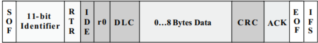
Figure 2.2: Standard CAN: 11-Bit Identifier [4]
