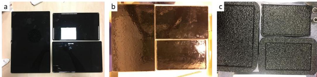
Figure 14: Demolded specimens, a) 1.0 wt% COOH-MWCNT-epoxy, b) 1.2 wt% MWCNT-epoxy, c) 2.0 wt% MWCNT-epoxy
