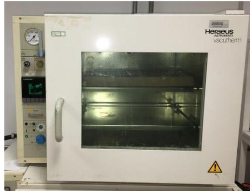
*Figure 9: Cure oven with vacuum system*
