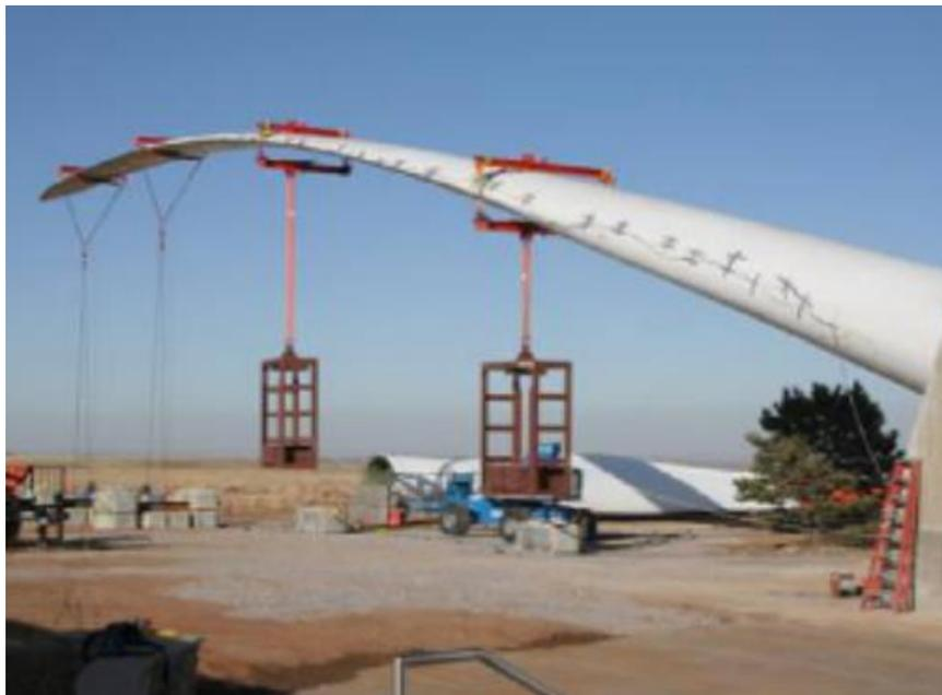
Figure 1.9. Multiple Point Method without Whiffletree System [15]
