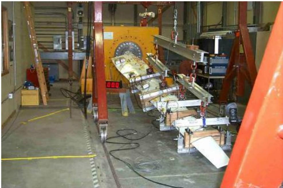
*Figure 2.9. Whiffletree arrangement on 9 meters wind turbine blade [20]*
