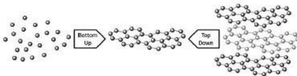
*Figure 1.3. A schematic of 'bottom-up' and 'top-down' graphene synthesis [3].*
