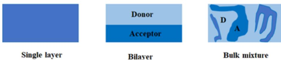
**Figure 1.8.** Active layer representations of single layer, bilayer and BHJ solar devices
