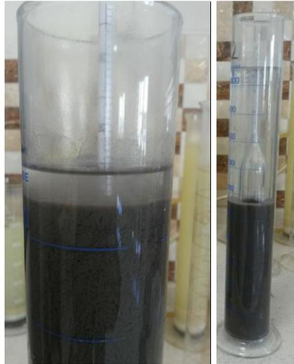
*Figure 5.25.* Hydrometer test for KFA
