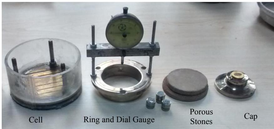
Figure 4.11. Swelling apparatus type-2
