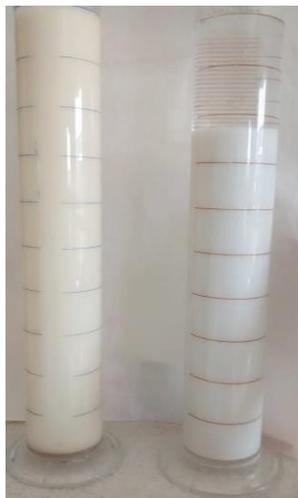
*Figure 4.35. View form hydrometer tests*
