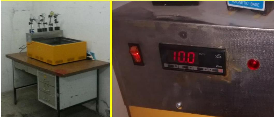
Figure 4.17. Water bath for 10°C tests
