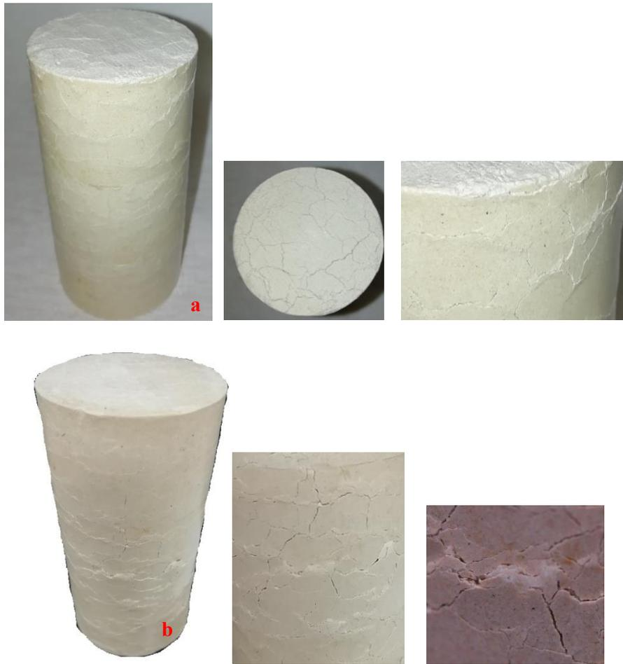
*Figure 6.12.* 40000ppm NS added 4% L treated specimen cured at 10°C for a- 4 months, b- 9 months
