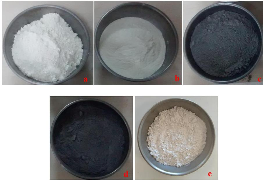
Figure 4.1. Materials (a-kaolinite, b-bentonite, c-soma fly ash, d-sivas-kangal fly ash, e-lime)
