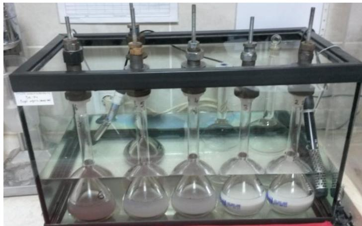
Figure 4.34.  $G_s$  samples in water tank
