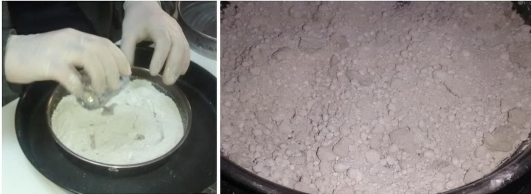
*Figure 4.7.* Addition of water to the dry mixture and mixing
