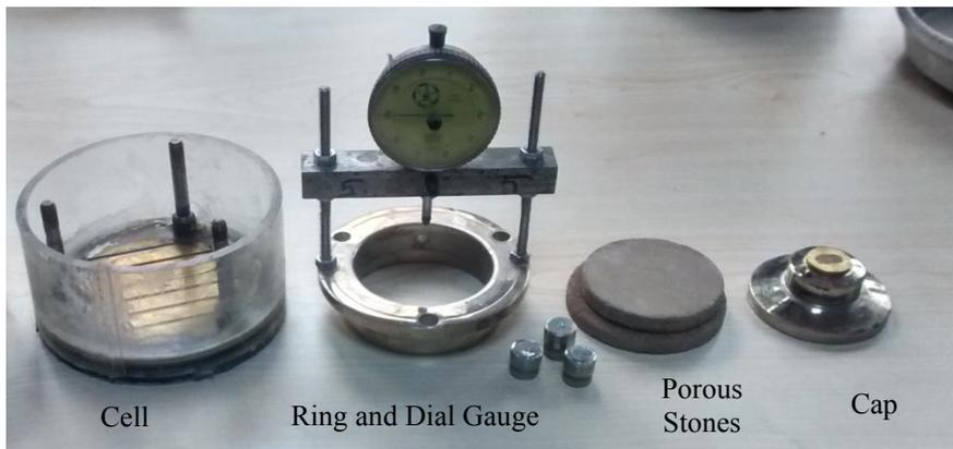
Figure 4.11. Swelling apparatus type-2
