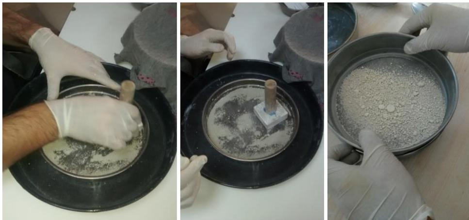
*Figure 4.8.* Crushing particles that stuck to each other with wooden blocks and sieving
