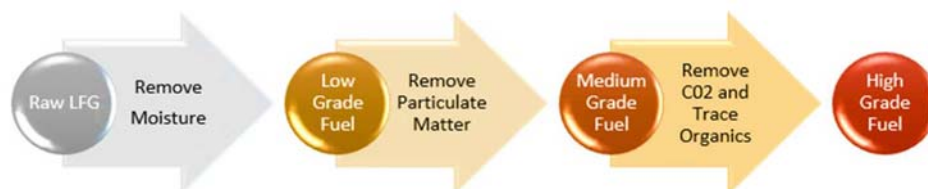
Figure 5 Treatment Steps of LFG
