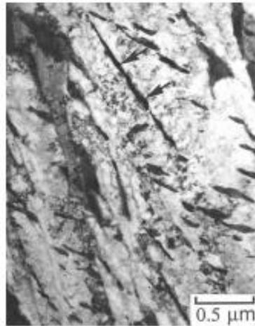
*Figure 2.4.* Formation of carbide precipitates inside of ferrite plates [9]
