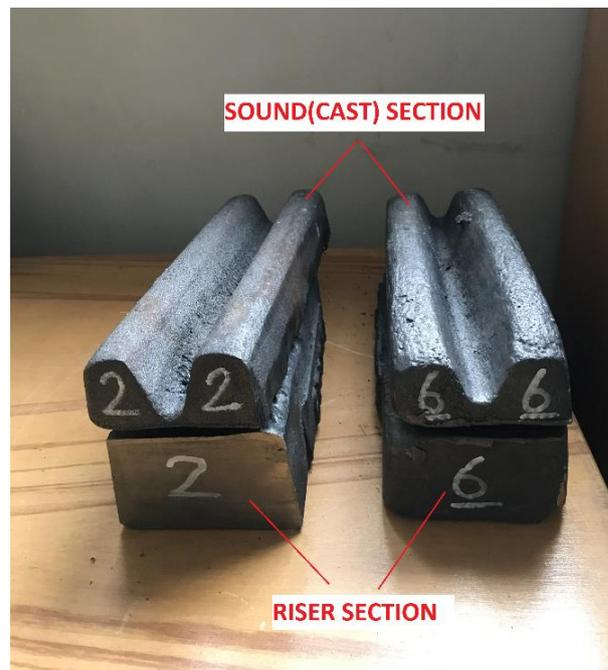
*Figure 3.1.* The figure of cast of (2) 4330M (6) Cu-alloyed 4330M steels (During pouring into molds, risers were on top. The photo taken after the risers and the casting were separated by cutting)
