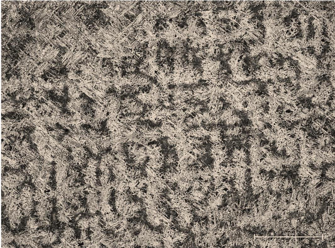
*Figure 4.5.* Dendrites observed in as-cast Cu-alloyed 4330M microstructure at a lower magnification.
