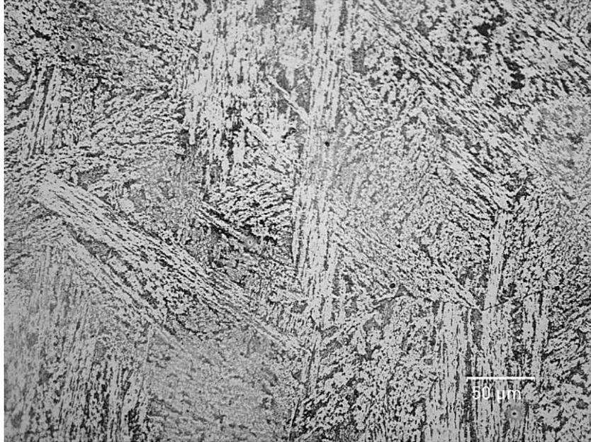
*Figure 4.3.* The as-cast microstructure of 4330M under optical microscopy
