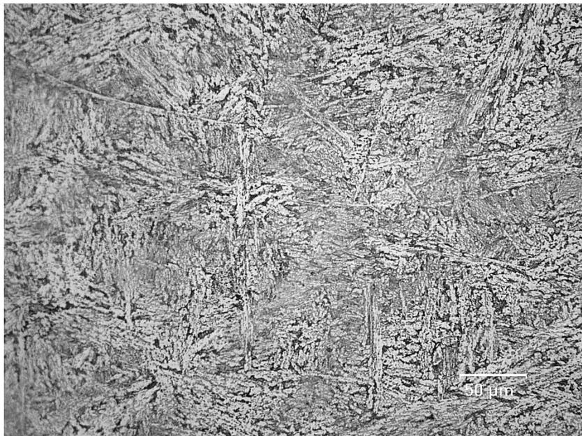
*Figure 4.4.* The as-cast microstructures of Cu-alloyed 4330M under optical microscopy
