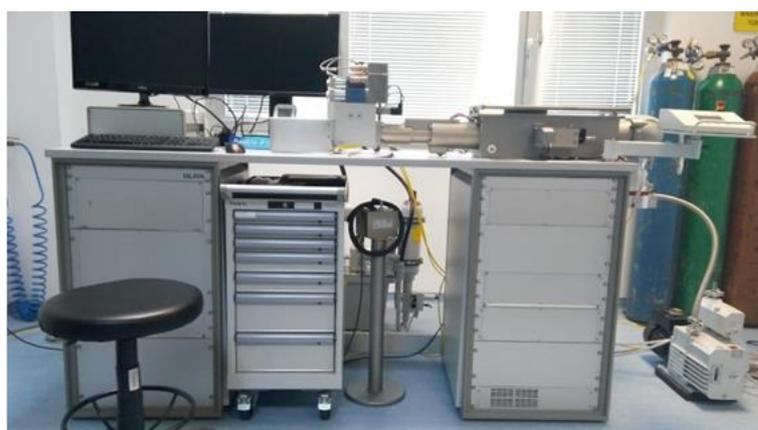
**Figure 3.1** TA-BAEHR DIL805A/D-Deformation Dilatomete
