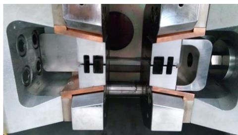
**Figure 3.9** Tensile test sample located in the Gleeble the chamber before test
