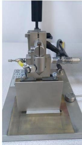
**Figure 3.4** Spot welding device for thermocouple welding to sample for temperature control of dilatometer
