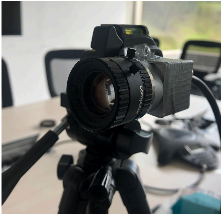
Figure 3.7: Basler Ace 720-540uc Video Camera
