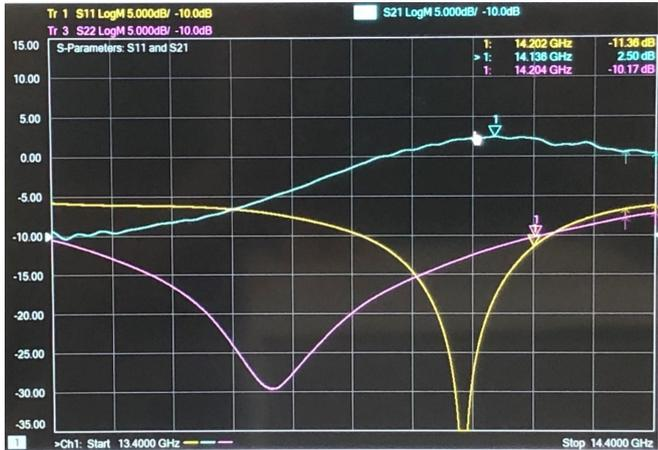
Figure 4.15: S-Parameter Measurement of PA After Replacement of SMA Connectors
