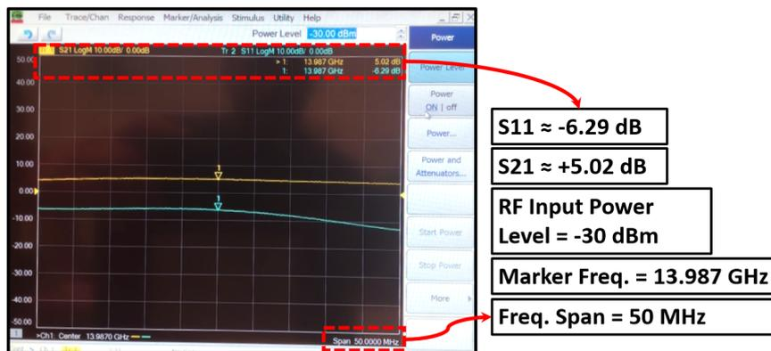
Figure 4.10: Gain and Input Matching Performance of the Power Amplifier Circuit Produced By LPKF
