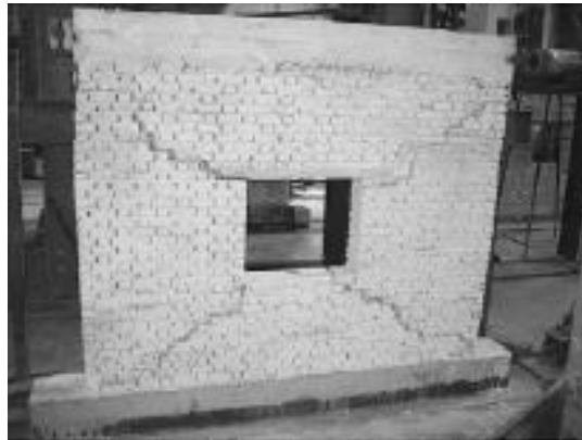
Figure 5.2. Unreinforced masonry wall specimen with window opening (Kalali and Kabir, 2012)
