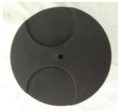
Figure 3.8. Modified Piston Head [42]
