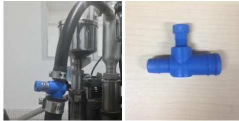
Figure 3.11. LPG Fuel Flow Control Valve
