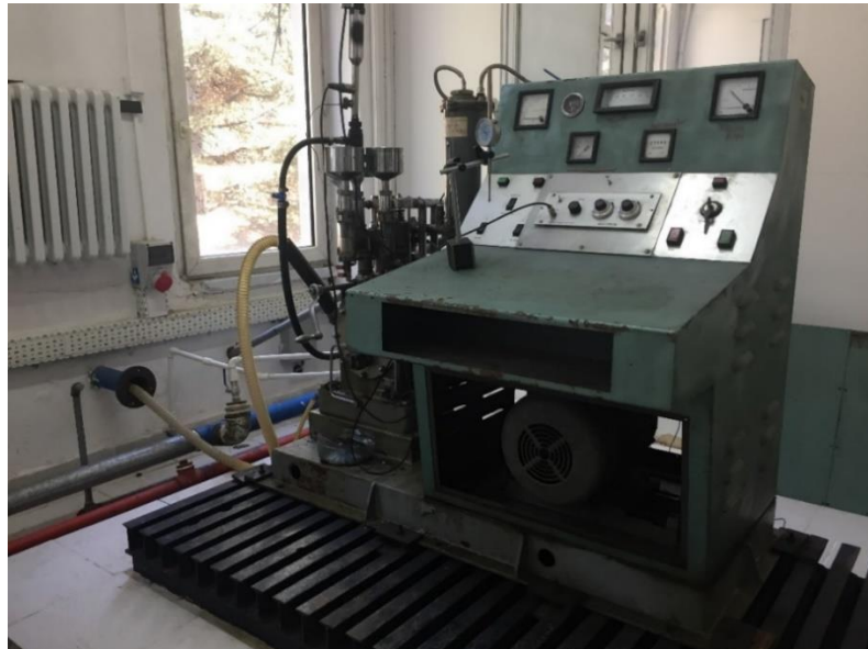
Figure 3.1. Cooperative Fuel Research Engine
