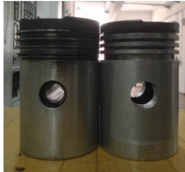
Figure 3.7. Piston design comparison of original (Right) and modified design (left) [42]
