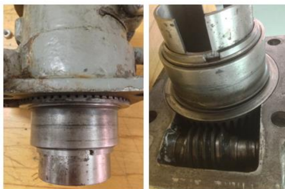
Figure 3.3. Compression Ratio Control Mechanism
