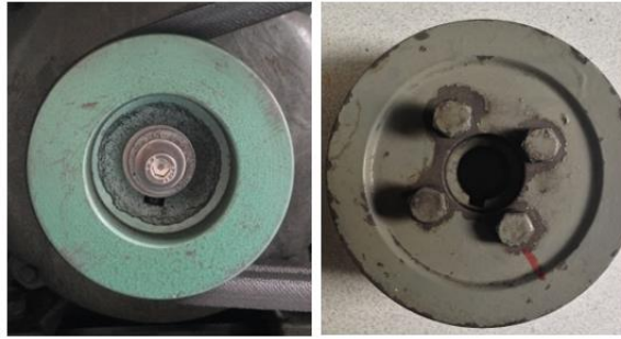
Figure 3.2. 100 mm pulley for RON (left) and 150 mm pulley for MON (right) measurements
