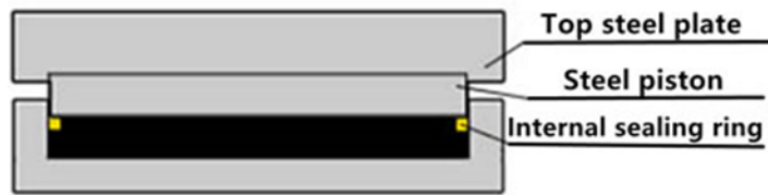
Fixed pot bearing structure
