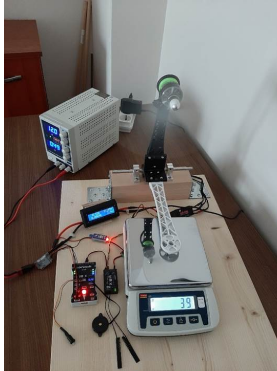
Figure 4.28: Thrust measurement setup for quadrotor motor-propeller pair
