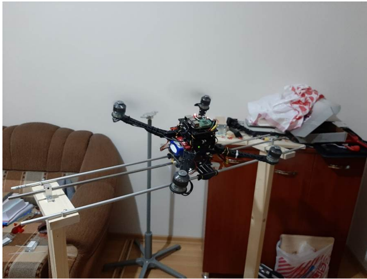
Figure 4.33: Single axis quadrotor test bench
