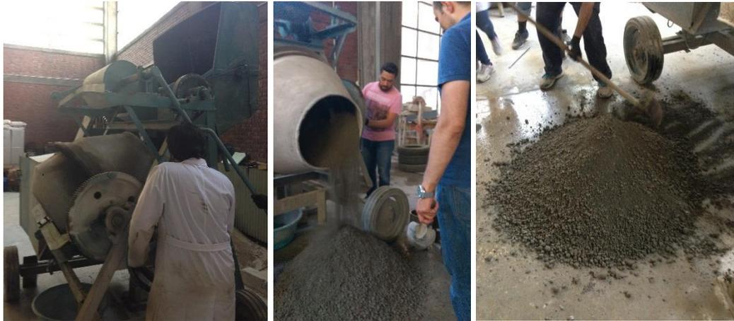
*Figure 3.3.* Mixing RCC mixture with rotary drum mixer and shovel on the ground
