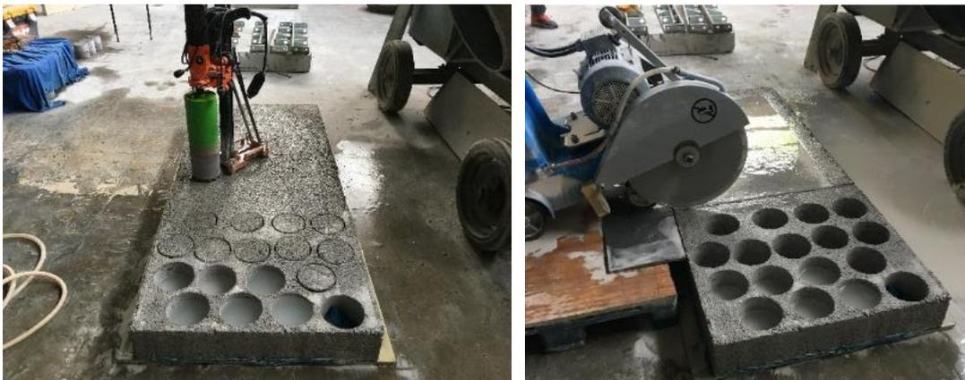
Figure 3.26 Taking the cores on the RCC plate and reducing the plate sizes with walk-behind concrete saw cutting machine
