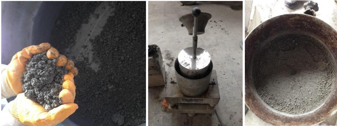
*Figure 3.4.* RCC mixture consistency and applied Vebe test
