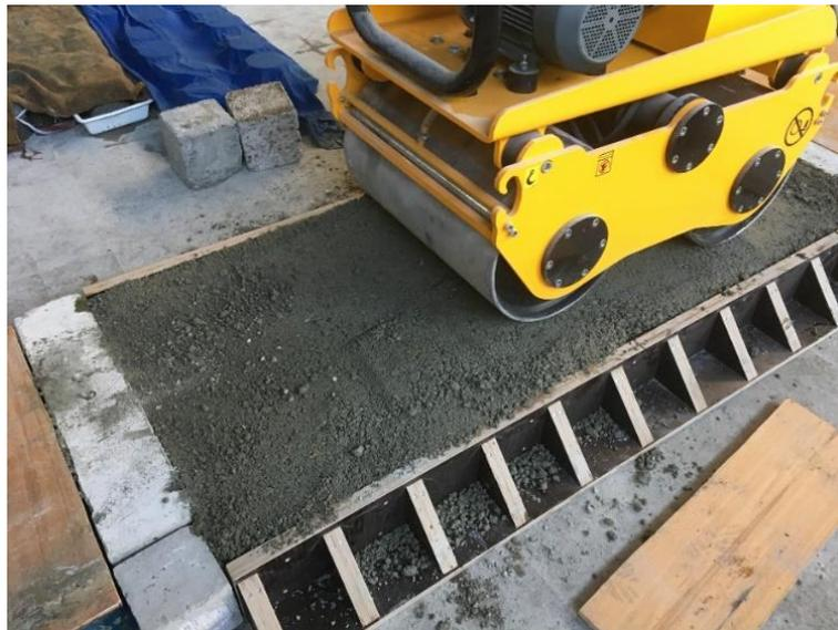
*Figure 3.18.* Surface undulations for some RCC mixtures during DDVHR application
