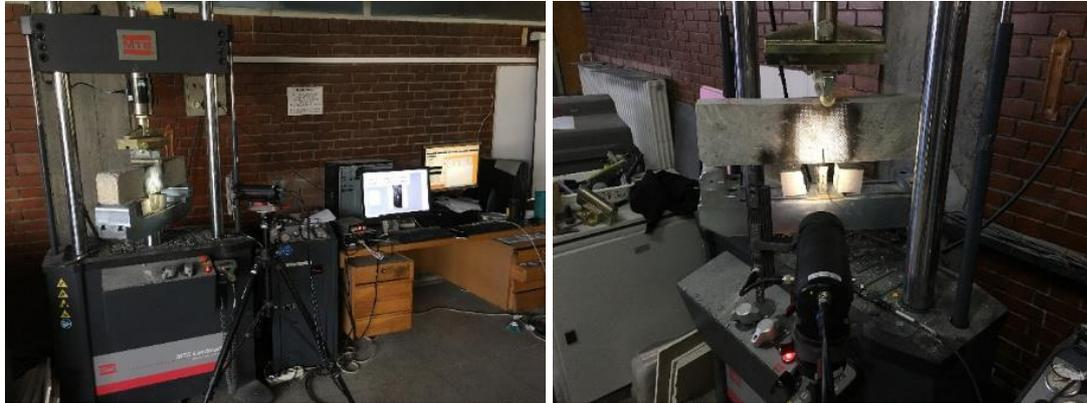
Figure 4.22. Three-point bending fracture test (RILEM TC 89-FMT 1990) on notched RCC specimen.
