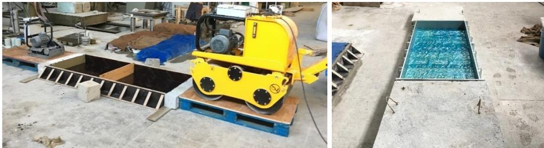
*Figure 3.15.* Wood and steel molds used for DDVHR
