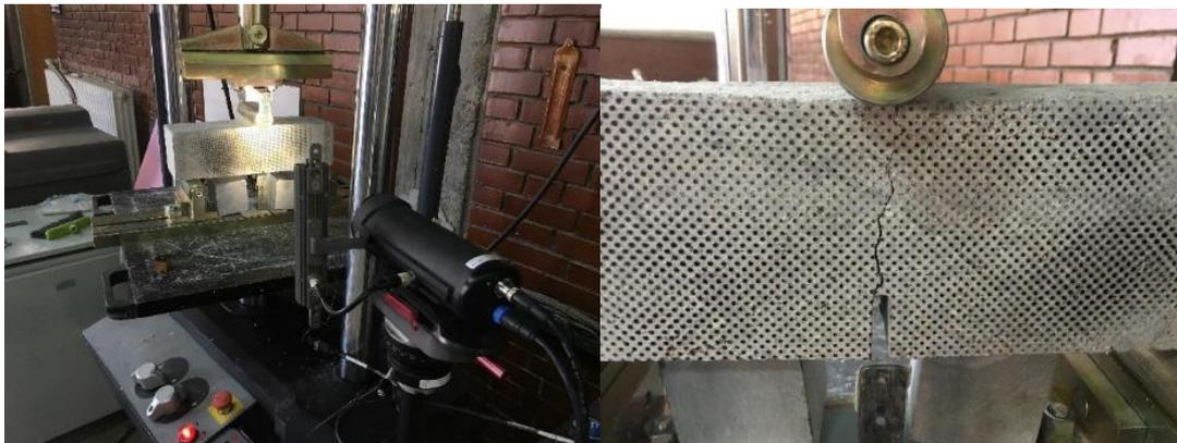
Figure 4.28. *Determination of fracture energy of RCC mixtures by three-point bending test applied on notched beam according to JCI-S-001-2003 standard*
