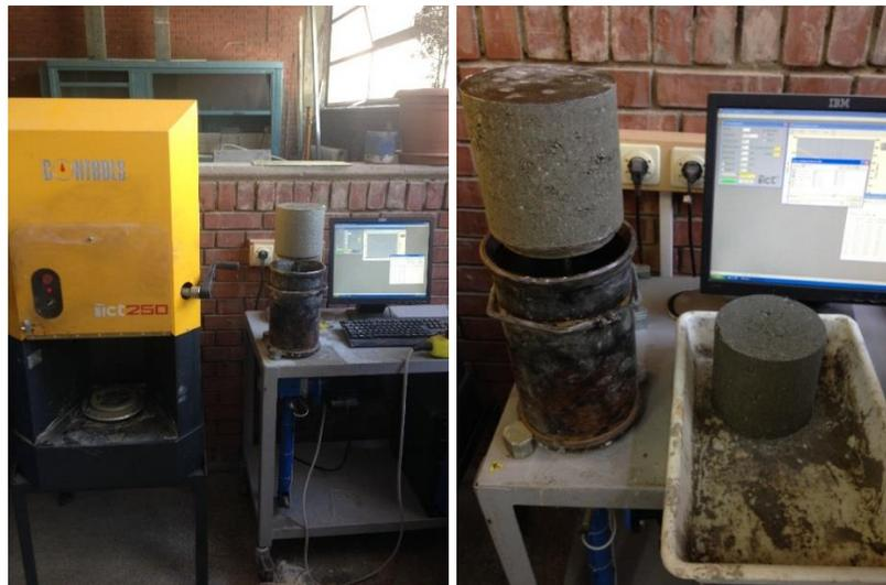
*Figure 3.8.* Compaction of RCC mixtures by SGC method.
