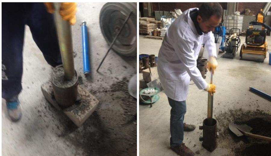
*Figure 3.5.* Compaction of RCC mixtures by modified proctor method (ASTM D1557)
