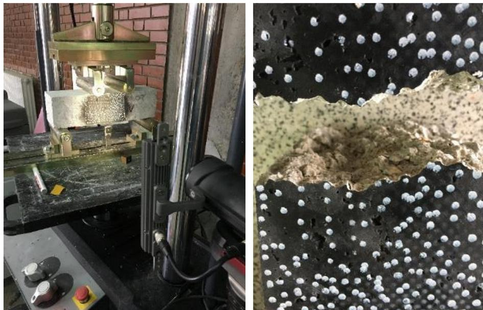
Figure 4.20. Determination of flexural strength of RCC mixtures according to ASTM C78.
