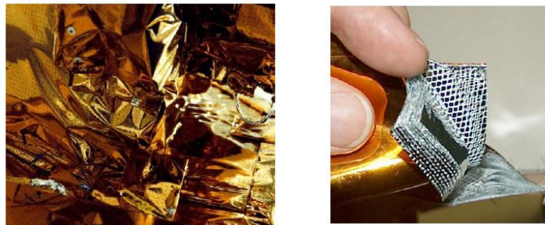
Figure 4.5 The Example of MLI Blanket [22]
