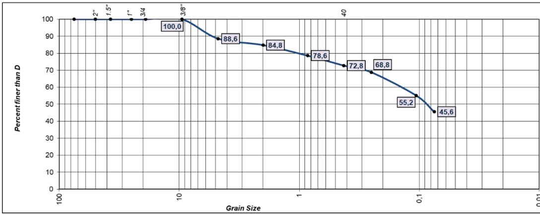
Figure 0.4. Particle size distribution plot of sample C1
