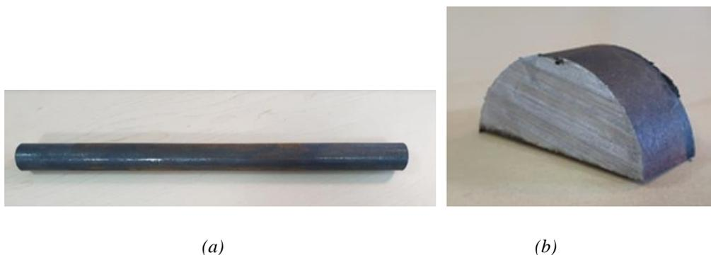
Figure 3.2. (a) the 100Cr6 bar and (b) the heat treatment specimen cut from it.
