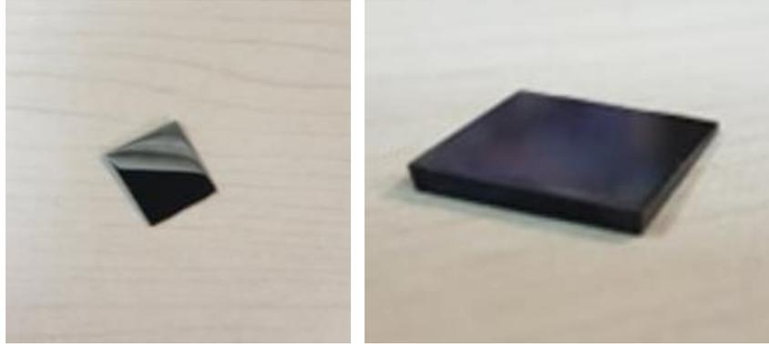
Figure 3.4. The XRD measurement specimen of 100Cr6 from different angles
