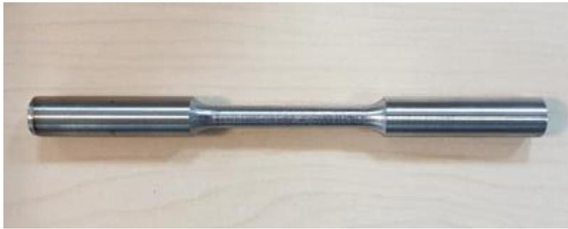
*Figure 3.5.* Tensile Test Specimen of 100Cr6 steel
