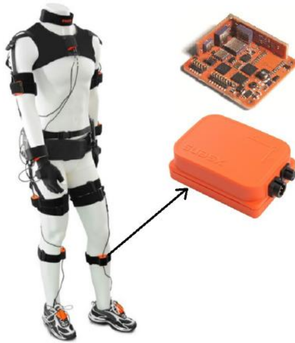
Figure 2.4. Xsens MVN BIOMECH© human motion capture system and the inertial sensor
