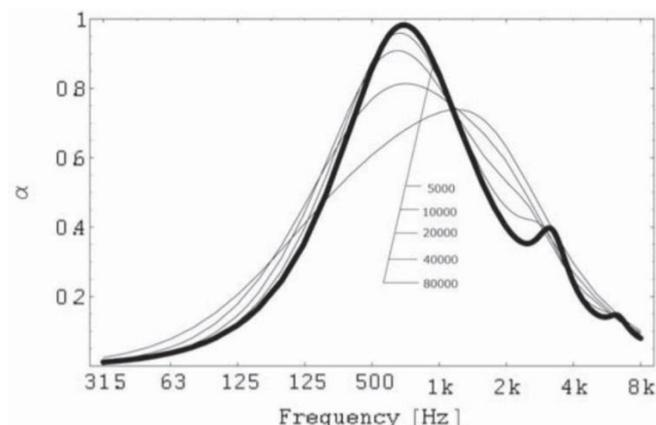
*Figure 2.53.* Comparison of sound absorption coefficients of a perforated panel with 0.3mm hole diameter, 0.3mm thickness, 0.8% perforation ratio and 50mm cavity depth but different porous material. Flow resistance of porous backing material differs between 5 to 8 kPa.s.m-1 (Sakagami et al. 2011).
