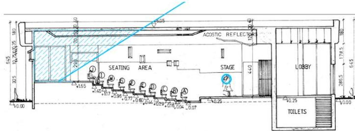
Figure 3.12. Ceiling surfaces suitable for sound absorber application
