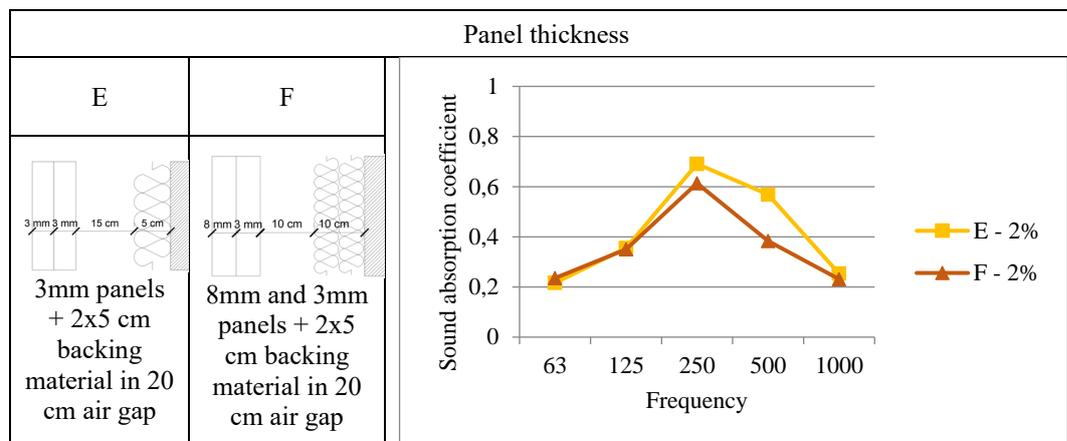
The perforated panel with 2% perforation ratio and 2-mm rather narrow slot width was expected to provide higher sound absorption at low frequencies compared to the panel with 12% perforation ratio. Hence, the effects of air gap and porous material with different slot widths as 2mm and 12 mm were determined. Final configuration for the perforated panel proposal is established at the end of these analyses.
