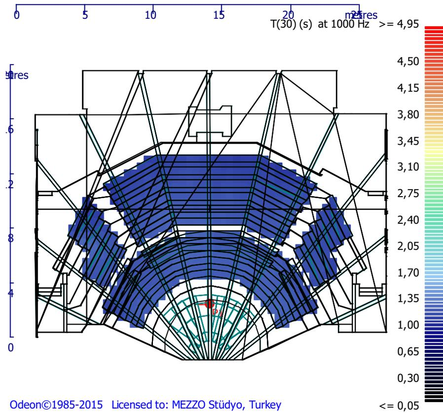
Figure 4.10. Reverberation time (T(30)) distribution map for 1000 Hz -current situation
