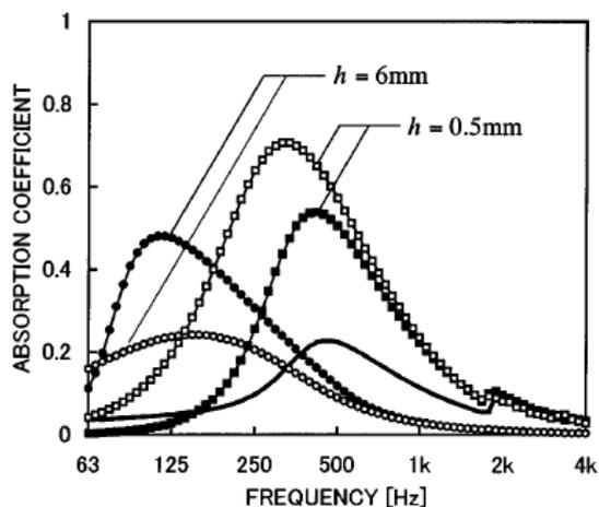
Figure 2.44. Effects of vibration and panel thickness on sound absorption coefficients. ( - ): 6mm thick perforated panel with 4.9% perforation ratio. Results for with ( -●-) and without ( -○-) the vibration effect for 6mm thick perforated plate with 0.2% perforation ratio. With ( -■-) and without ( -□-) the vibration effect for 0.5mm thick perforated plate with 0.2% perforation ratio (Takahashi & Tanaka, 2002).
