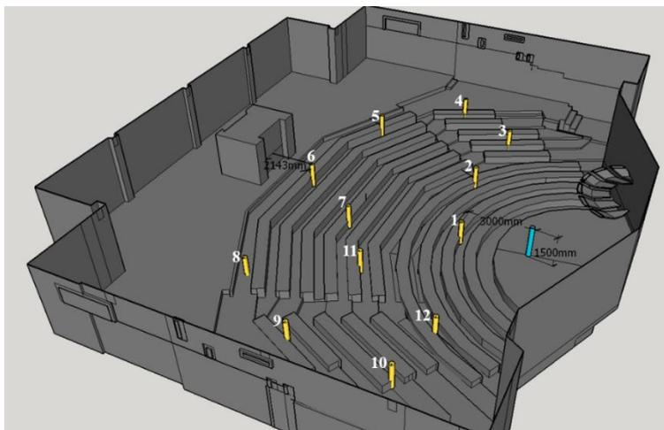
Figure 3.18. Representation of source and microphone positions in the hall
