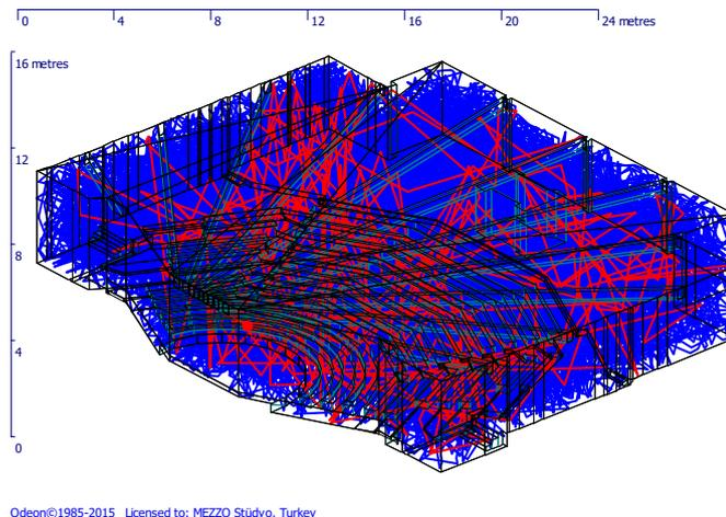
Figure 3.13. ODEON ray tracing view for the Amphitheatre
