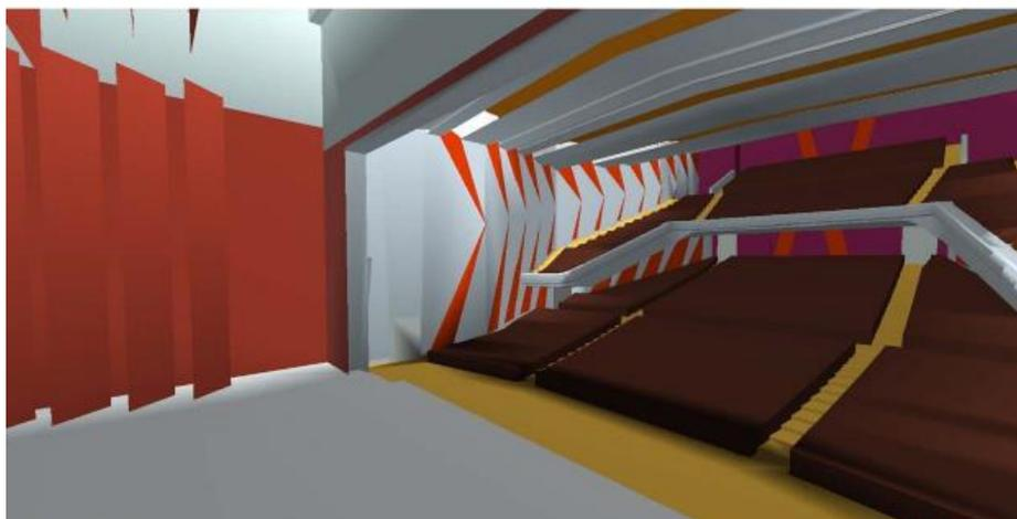
*Figure 2.18.* 3D OpenGL view of multi-functional auditorium, exported from ODEON room acoustics simulation software (Sü Gül, Meriç Nursal, Bora, Çalışkan, 2016).
