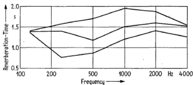
Figure 2.11. Reverberation times for the Beattie Theatre. Without active acoustic system (below), with active acoustic system as single feedback system (middle), with the phase modulated active acoustic system (above) (Guelke & Broadhurst, 1971).
