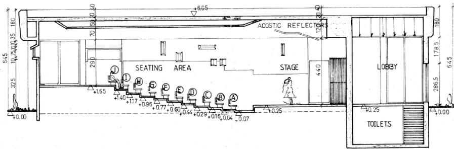
Figure 3.6. Longitudinal section of the Amphitheatre (Hejjo, 1986)
