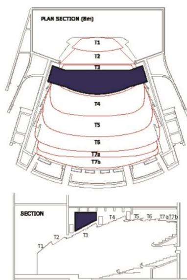
Figure 2.4. Location of the coupled volume in plan (above) and section views (below) (Sü-Gül & Çalışkan, 2010)
