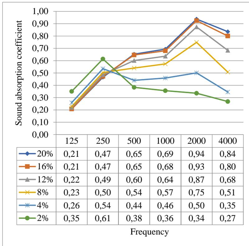
Figure 4.3. Sound absorption coefficients of perforated panel system with 20-cm air gap and 2 x 5 cm 48-52 kg/m<sup>3</sup> rock wool.
