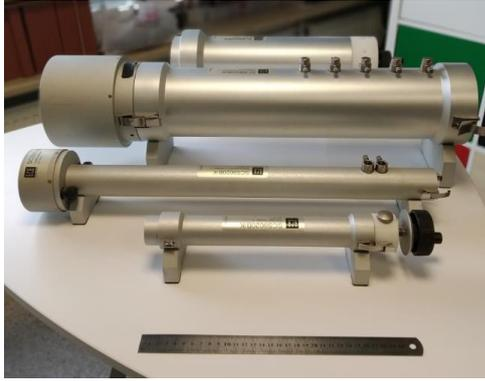
*Figure 3.9.* Impedance tubes for sound absorption coefficient measurements
