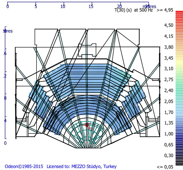
Figure 4.8. Reverberation time (T(30)) distribution map for 500 Hz -current situation
