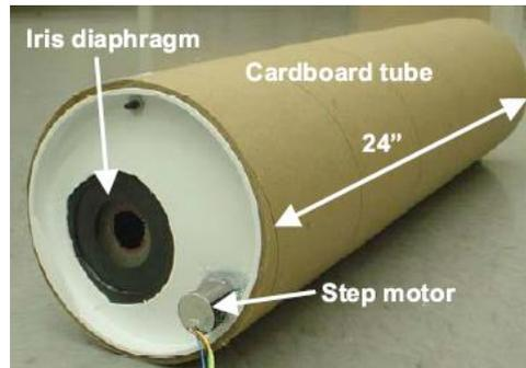
Figure 2.29. Helmholtz resonator with variable opening (Estève & Johnson (2004).
