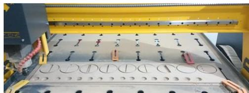
*Figure 3.8.* Manufacture of perforated panel samples by a CNC router
