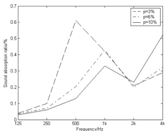
Figure 2.37. Effects of perforation ratio on sound absorption coefficients of perforated panels (Hou et al. 2010).
