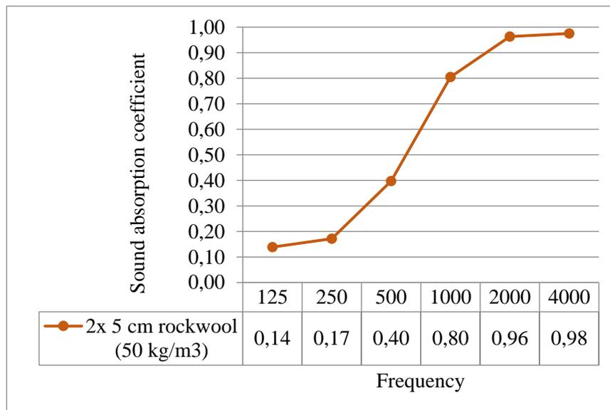
Figure 4.2. Sound absorption coefficients of 2 x 5 cm 48-52 kg/m<sup>3</sup> rock wool.
