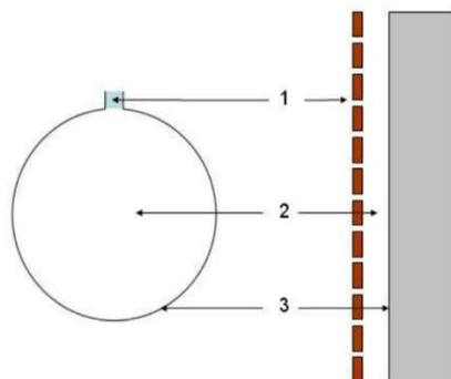
*Figure 2.28.* Comparison of Helmholtz resonator and perforated panel sections. 1 represents the hole of perforated panel and neck of Helmholtz resonator. 2 is the air gap behind the perforated panel and cavity of the resonator. 3 is the rigid wall behind the panel and cavity surface (Negro et al. 2010).
