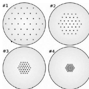
Figure 2.34. Schematic pictures of samples of perforated panels. #1:  $b=14,18\text{mm}$ , #2:  $b=8\text{mm}$ , #3:  $b=3,5\text{mm}$ , #4:  $b=2,5\text{mm}$ .  $b$  is the center to center distance between holes (Tayong, 2013).
