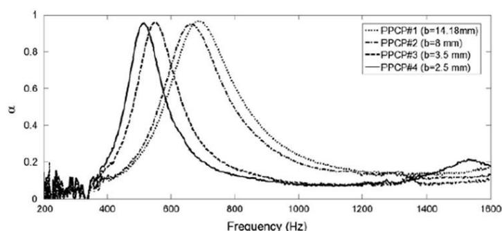
Figure 2.35. Impedance tube measurements of samples with 20mm air cavity (Tayong, 2013).
