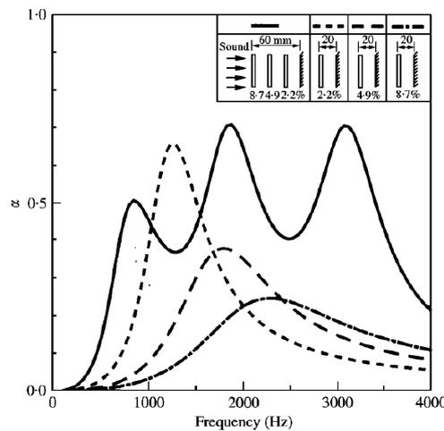
Figure 2.36. Resonance frequencies of the multi-layer sound absorber and its compartments (Lee & Chen, 2001).
