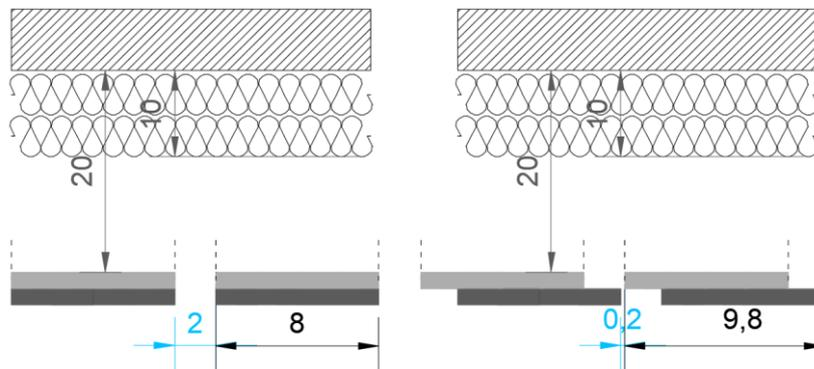
Figure 3.2. Schematic description of variability in perforations
