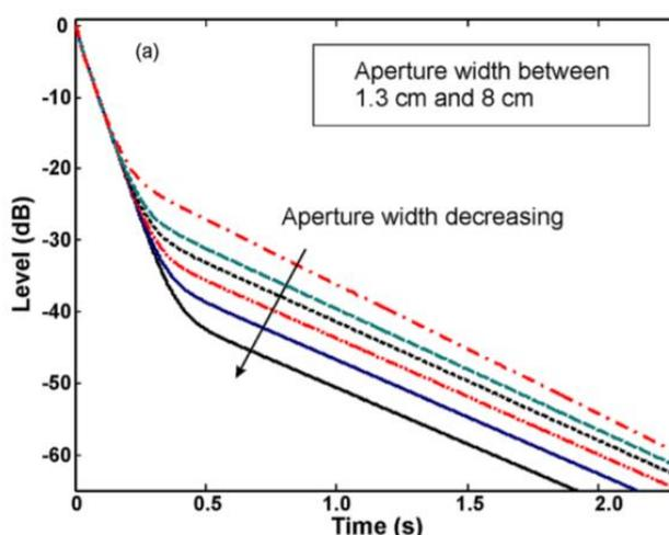
Figure 2.6. Decreasing aperture size and energy decay profiles depending on diffusion equation model (Xiang et al. 2013).
