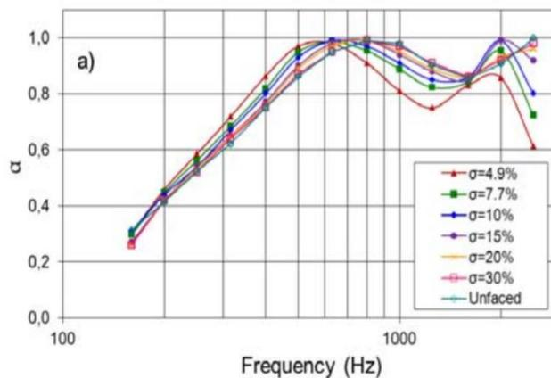
Figure 2.39. Sound absorption coefficients of perforated panels with different perforation ratios (Borelli, Schenone & Pittaluga, 2013).
