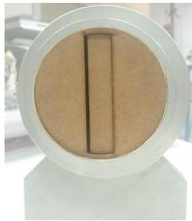
*Figure 3.10.* Samples placed in impedance tube for sound absorption coefficient measurements
