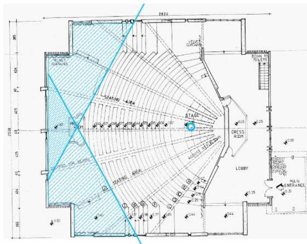
Figure 3.11. Wall surfaces suitable for sound absorber application
