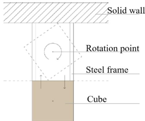
Figure 2.24. Schematic description of variable acoustic cube (derived from; Kousi, Gyftopoulos, Karagiannis & Sotiropoulou, 2016).
