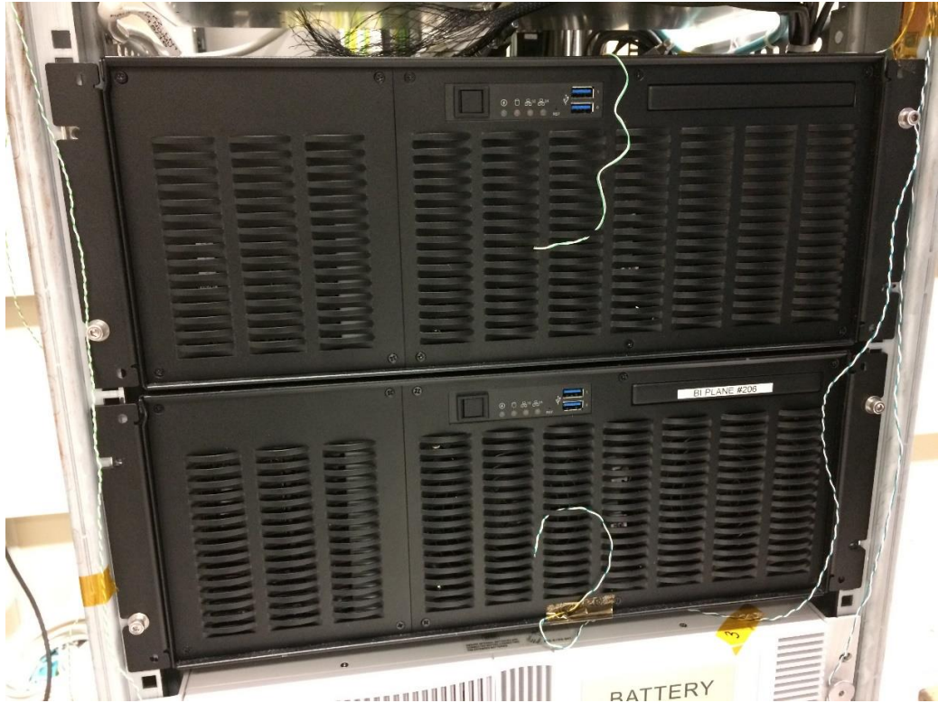
Figure 2.2. Inlet thermocouples on Workstation – 1 and Workstation – 2
