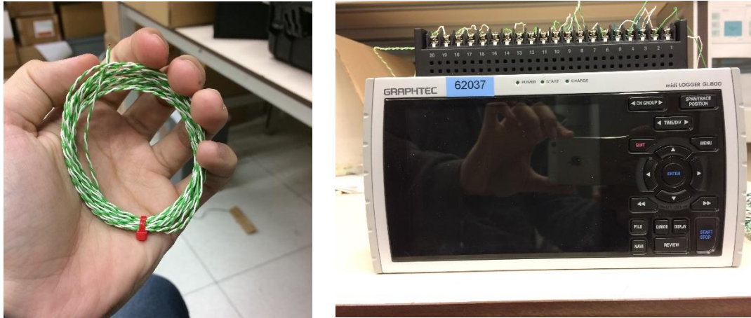
Figure 2.1. Type-K thermocouple and Graphtec data logger
