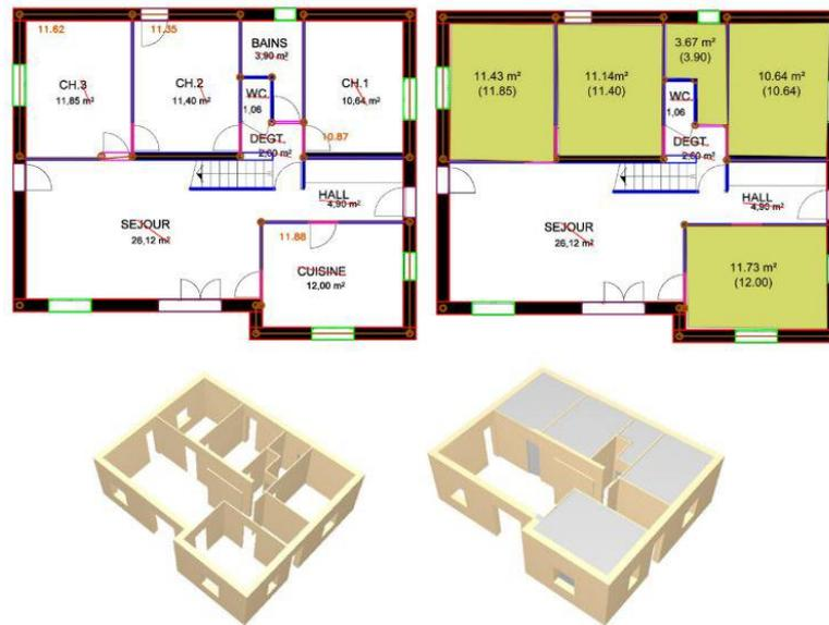
Figure 2.5. Recognition of building elements and 3D reconstruction (Gimenez et al., 2016)
