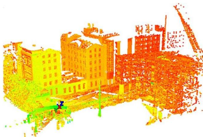
*Figure 2.7.* Laser scanning of a building under construction (Tang et.al, 2010)
