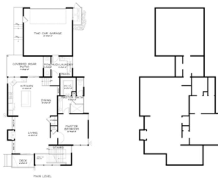
Figure 3.5. Floor plan drawing and corresponding label image
