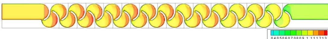
Figure 3.16. Fluid depth of Type 2 considering max. flow rate conditions – Top view
