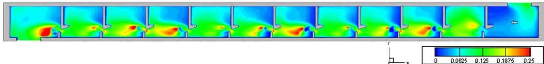
*Figure 1.11. Turbulent kinetic energy,  $k$  values in  $m^2/s^2$  at  $0.75h$  fluid depth of the previous study on conventional vertical slot pass by Özkaya, 2014*
