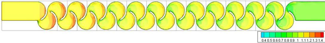
Figure 3.241. Fluid depth of Type 27 considering max. flow rate conditions – Top view
