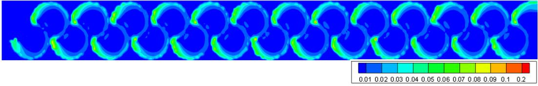
Figure 3.100. TKE of Type 11 considering min. flow rate conditions at 0.75h water level
