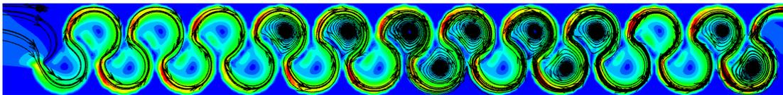
Figure 3.120. Streamlines of Type 13 considering max. flow rate conditions at 0.75h water level
