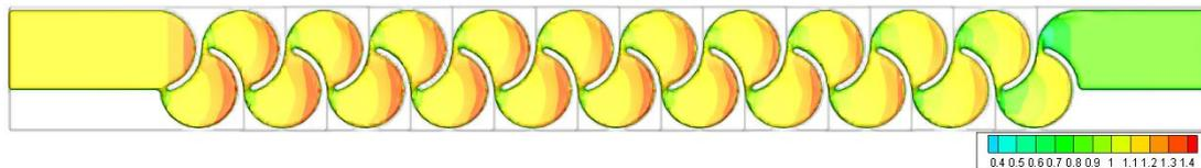
Figure 3.169. Fluid depth of Type 19 considering max. flow rate conditions – Top view
