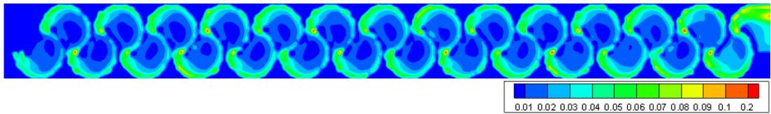
Figure 3.49. TKE of Type 5 considering max. flow rate conditions at 0.75h water level
