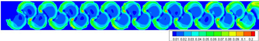
Figure 3.40. TKE of Type 4 considering max. flow rate conditions at 0.75h water level
