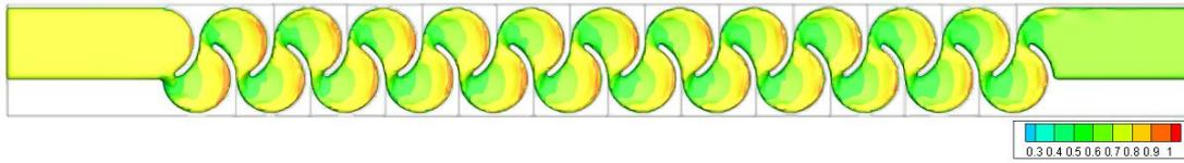
Figure 3.141. Fluid depth of Type 16 considering min. flow rate conditions – Top view
