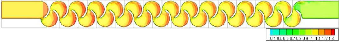
Figure 3.160. Fluid depth of Type 18 considering max. flow rate conditions – Top view
