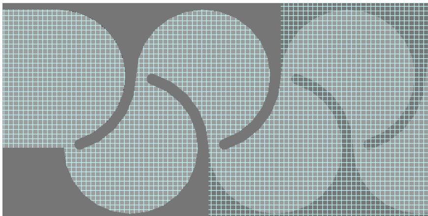
Figure 3.4. Plan view of mesh with 0.09 m cell size
