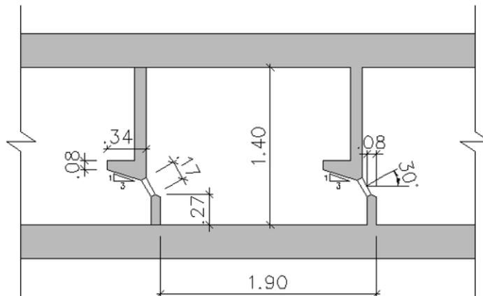
Figure 2.2. Determined conventional vertical slot fish type dimensions (in m) (Özkaya, 2014)
