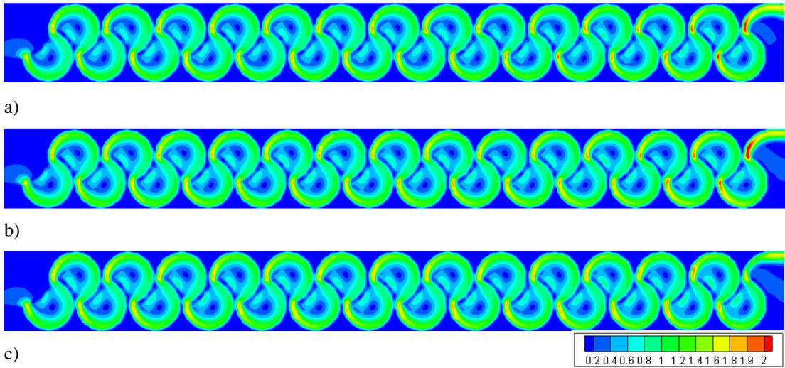
Figure 3.110. Flow velocities of Type 12 considering max. flow rate conditions at water levels of: a) 0.25h, b) 0.50h, c) 0.75h
