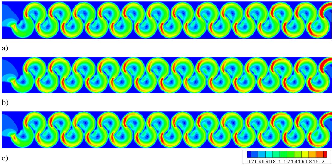
Figure 3.155. Flow velocities of Type 17 considering max. flow rate conditions at water levels of: a) 0.25h, b) 0.50h, c) 0.75h
