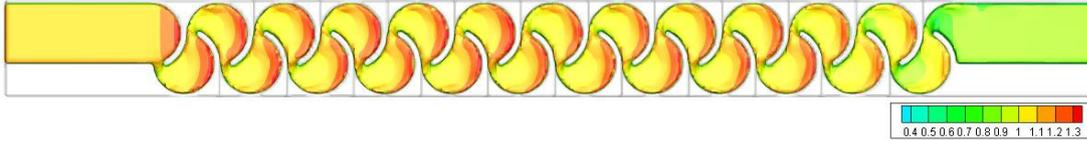
Figure 3.34. Fluid depth of Type 4 considering max. flow rate conditions – Top view
