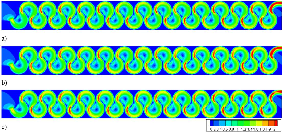
Figure 3.164. Flow velocities of Type 18 considering max. flow rate conditions at water levels of: a) 0.25h, b) 0.50h, c) 0.75h
