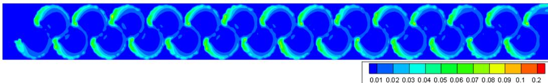
Figure 3.109. TKE of Type 12 considering min. flow rate conditions at 0.75h water level
