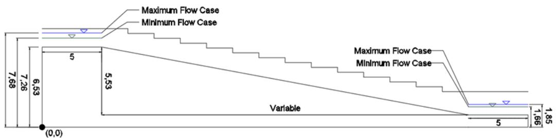
Figure 3.2. Typical fish pass section demonstrating water levels (measurements are in m)
