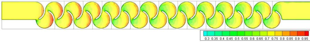
Figure 3.240. Fluid depth of Type 27 considering min. flow rate conditions – Top view
