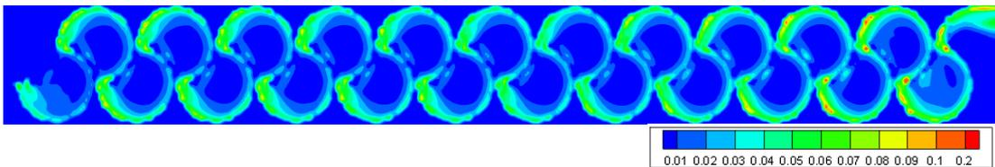
Figure 3.211. TKE of Type 23 considering max. flow rate conditions at 0.75h water level
