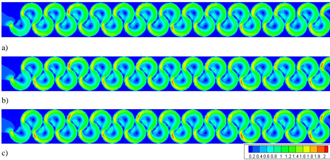
Figure 3.134. Flow velocities of Type 15 considering min. flow rate conditions at water levels of: a) 0.25h, b) 0.50h, c) 0.75h
