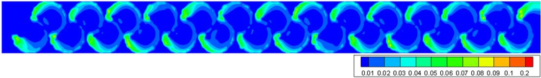
Figure 3.19. TKE of Type 2 considering min. flow rate conditions at 0.75h water level
