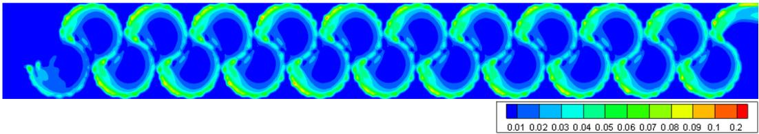
Figure 3.226. TKE of Type 25 considering min. flow rate conditions at 0.75h water level
