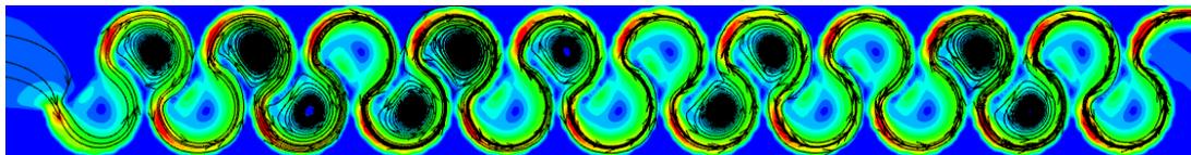
Figure 3.225. Streamlines of Type 25 considering min. flow rate conditions at 0.75h water level
