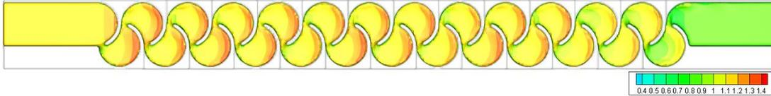
Figure 3.124. Fluid depth of Type 14 considering max. flow rate conditions – Top view
