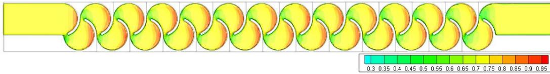
Figure 3.213. Fluid depth of Type 24 considering min. flow rate conditions – Top view
