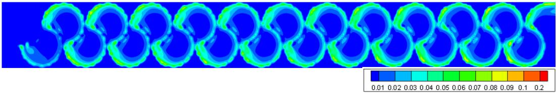
Figure 3.235. TKE of Type 26 considering min. flow rate conditions at 0.75h water level
