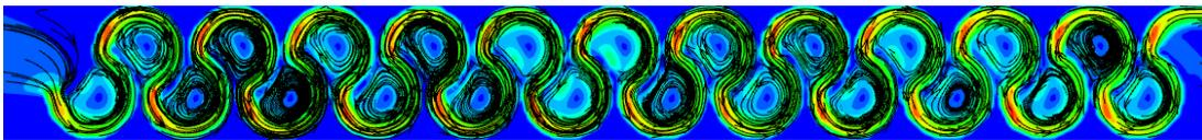
Figure 3.36. Streamlines of Type 4 considering min. flow rate conditions at 0.75h water level
