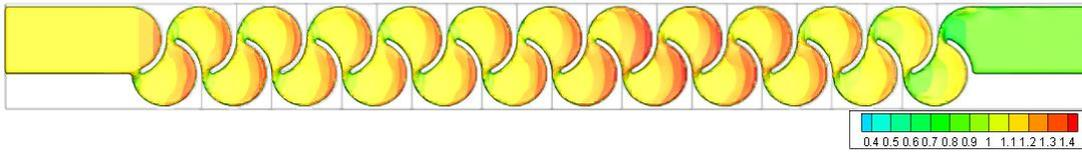
Figure 3.205. Fluid depth of Type 23 considering max. flow rate conditions – Top view
