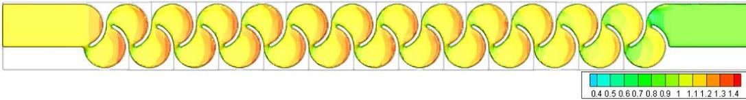
Figure 3.214. Fluid depth of Type 24 considering max. flow rate conditions – Top view
