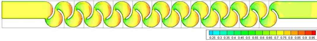
Figure 3.33. Fluid depth of Type 4 considering min. flow rate conditions – Top view
