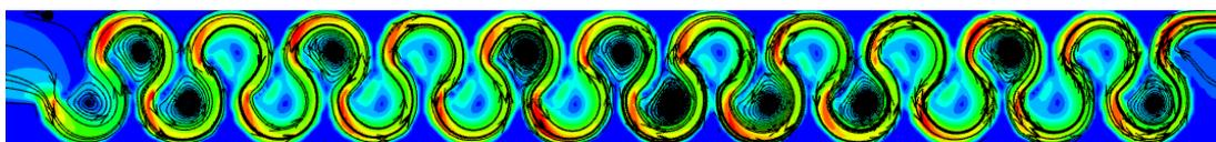
Figure 3.63. Streamlines of Type 7 considering min. flow rate conditions at 0.75h water level
