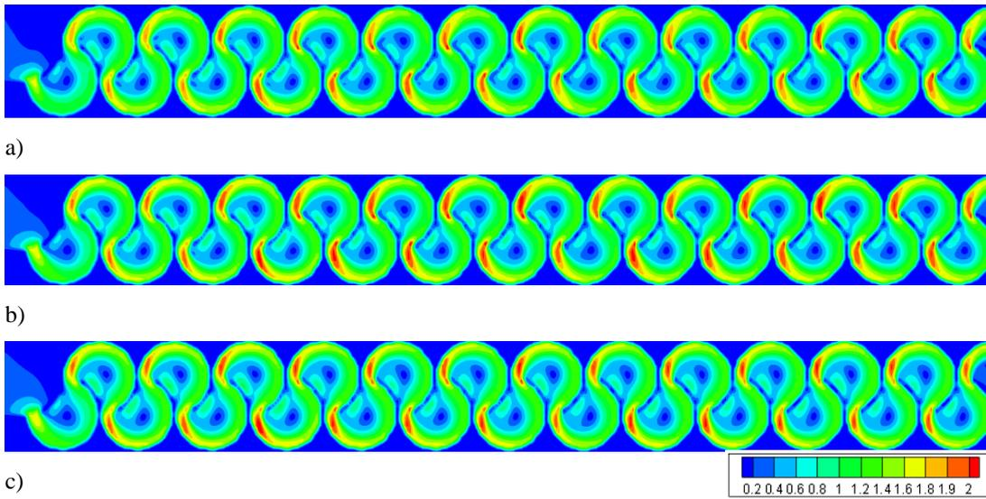
Figure 3.242. Flow velocities of Type 27 considering min. flow rate conditions at water levels of: a) 0.25h, b) 0.50h, c) 0.75h
