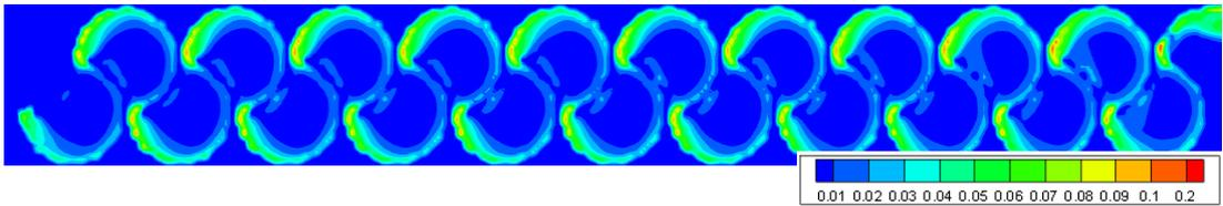
Figure 3.175. TKE of Type 19 considering max. flow rate conditions at 0.75h water level
