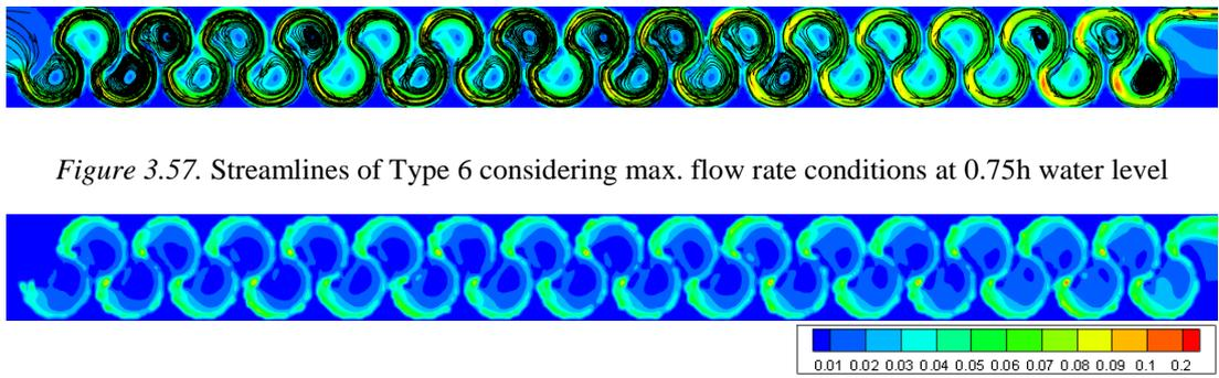
Figure 3.57. Streamlines of Type 6 considering max. flow rate conditions at 0.75h water level
