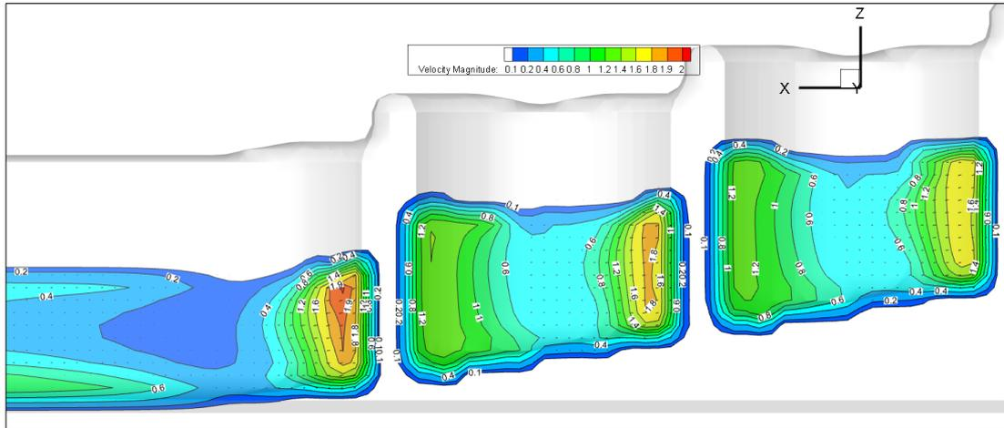
Figure 3.250. Velocity magnitude contours (xy plane) of section  $x_2$
