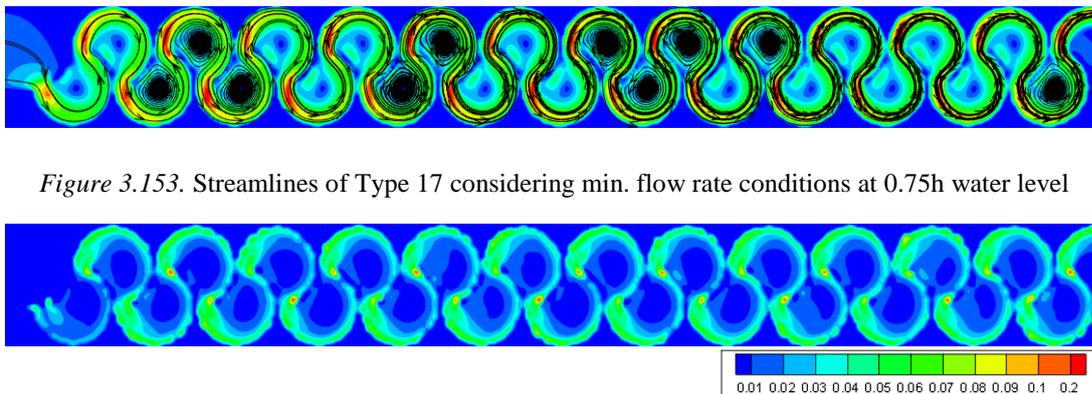
Figure 3.153. Streamlines of Type 17 considering min. flow rate conditions at 0.75h water level
