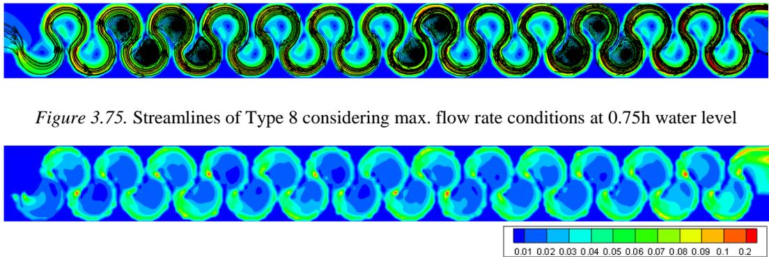
Figure 3.75. Streamlines of Type 8 considering max. flow rate conditions at 0.75h water level
