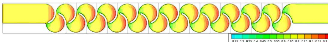
Figure 3.87. Fluid depth of Type 10 considering min. flow rate conditions – Top view
