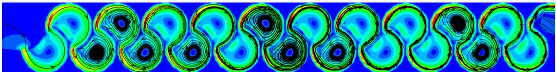
Figure 3.174. Streamlines of Type 19 considering max. flow rate conditions at 0.75h water level
