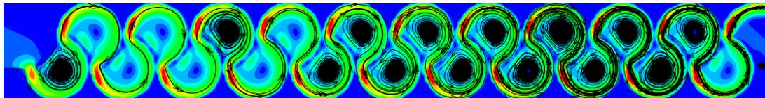
Figure 3.198. Streamlines of Type 22 considering min. flow rate conditions at 0.75h water level
