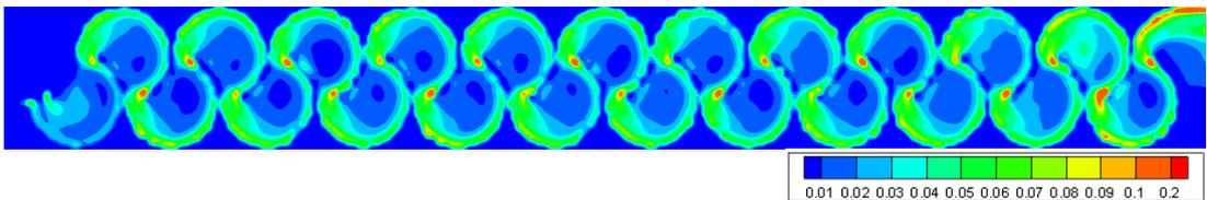
Figure 3.148. TKE of Type 16 considering max. flow rate conditions at 0.75h water level
