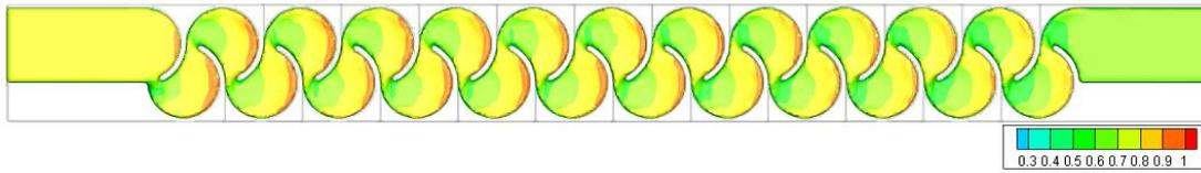
Figure 3.231. Fluid depth of Type 26 considering min. flow rate conditions – Top view
