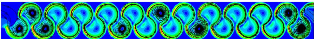
Figure 3.93. Streamlines of Type 10 considering max. flow rate conditions at 0.75h water level
