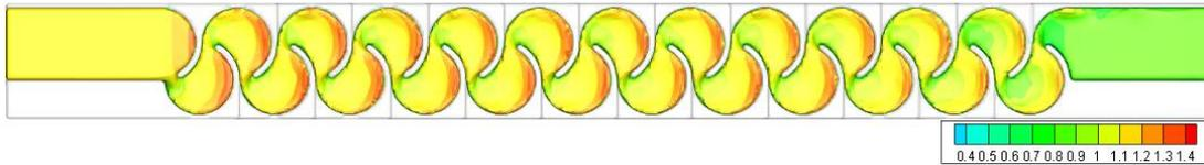
Figure 3.142. Fluid depth of Type 16 considering max. flow rate conditions – Top view
