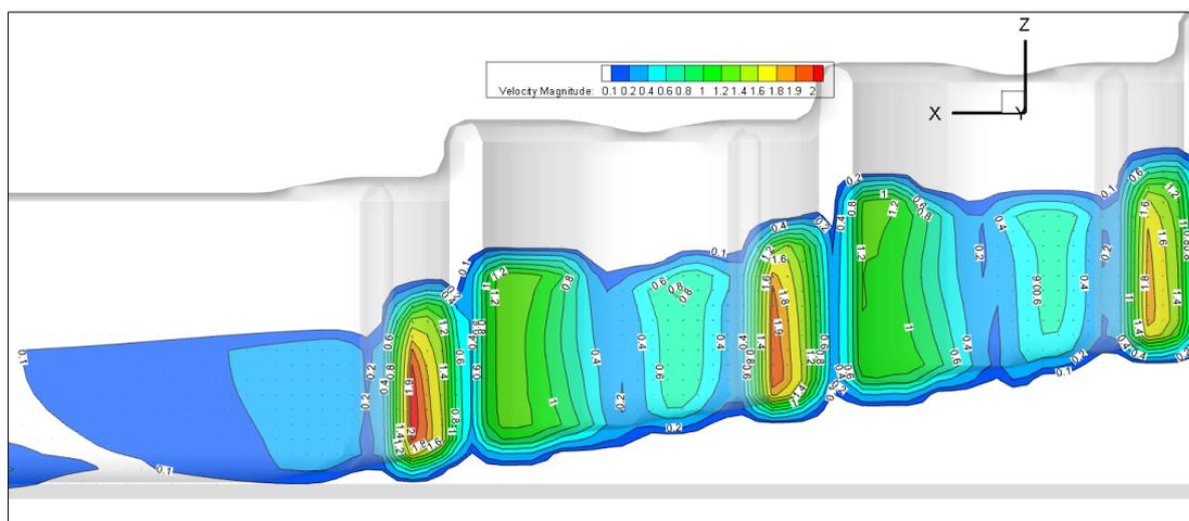
Figure 3.249. Velocity magnitude contours (xy plane) of section  $x_1$
