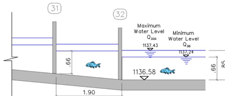
Figure 2.4. Water levels at the conventional vertical slot fish pass entrance (Özkaya, 2014)
