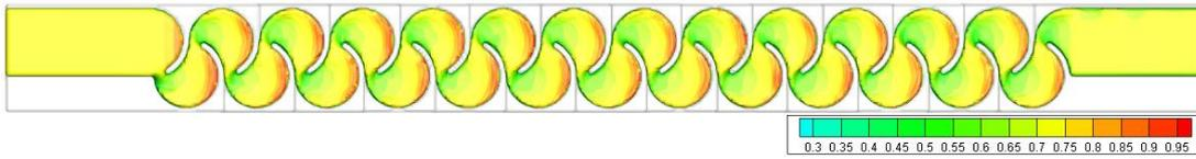
Figure 3.150. Fluid depth of Type 17 considering min. flow rate conditions – Top view
