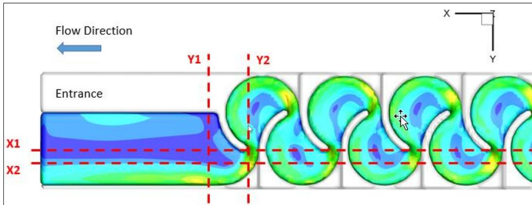
Figure 3.248. Sections taken form entrance of fish pass
