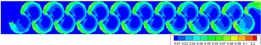
Figure 3.202. TKE of Type 22 considering max. flow rate conditions at 0.75h water level
