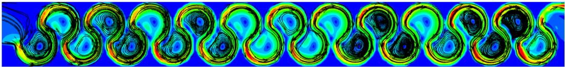
Figure 3.39. Streamlines of Type 4 considering max. flow rate conditions at 0.75h water level
