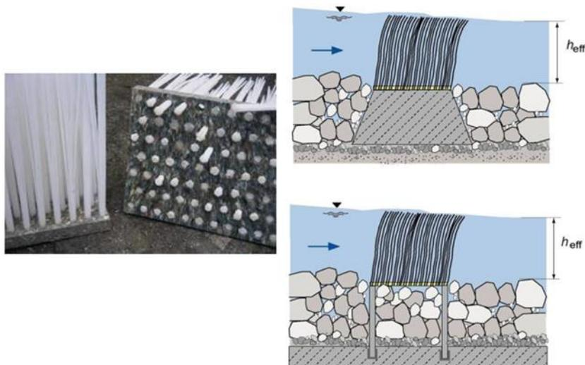
Figure 1.4. Brush package consisting of a carrier plate to which the brush bundle is placed (Left), brush package fixing on concrete foundation and pedestal bearing plate (Right) (DWA-M 509)
