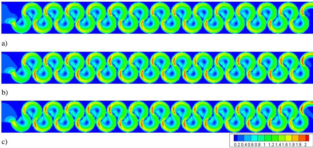
Figure 3.161. Flow velocities of Type 18 considering min. flow rate conditions at water levels of: a) 0.25h, b) 0.50h, c) 0.75h
