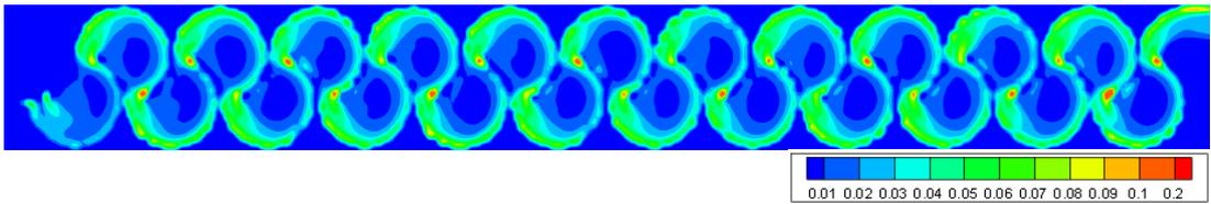
Figure 3.145. TKE of Type 16 considering min. flow rate conditions at 0.75h water level
