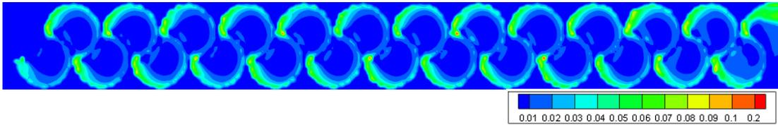
Figure 3.103. TKE of Type 11 considering max. flow rate conditions at 0.75h water level
