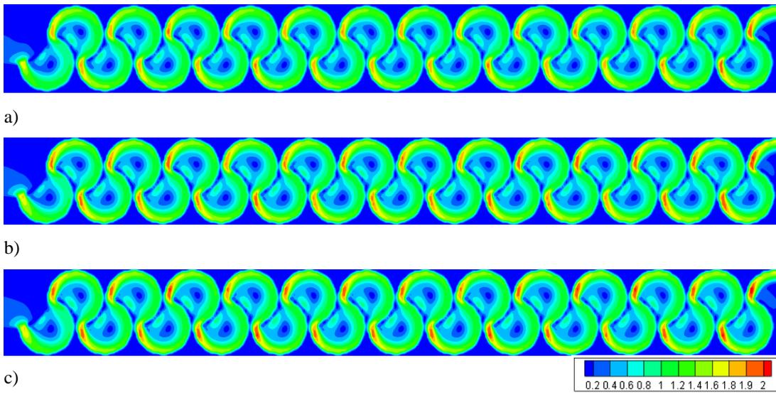
Figure 3.215. Flow velocities of Type 24 considering min. flow rate conditions at water levels of: a) 0.25h, b) 0.50h, c) 0.75h
