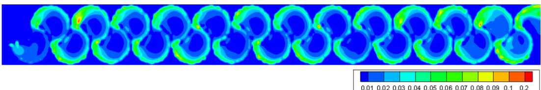
Figure 3.130. TKE of Type 14 considering max. flow rate conditions at 0.75h water level
