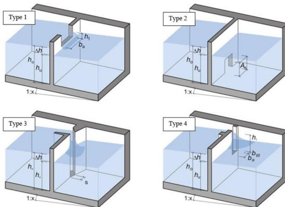
Figure 1.1. Opening types on the cross - walls of pool fish passes (DWA-M 509)
