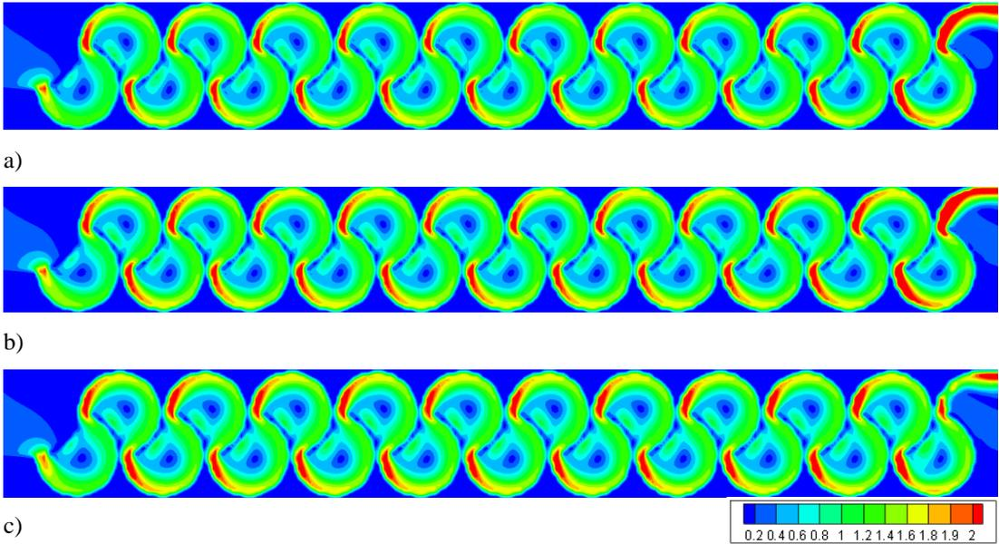
Figure 3.200. Flow velocities of Type 22 considering max. flow rate conditions at water levels of: a) 0.25h, b) 0.50h, c) 0.75h
