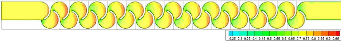
Figure 3.132. Fluid depth of Type 15 considering min. flow rate conditions – Top view
