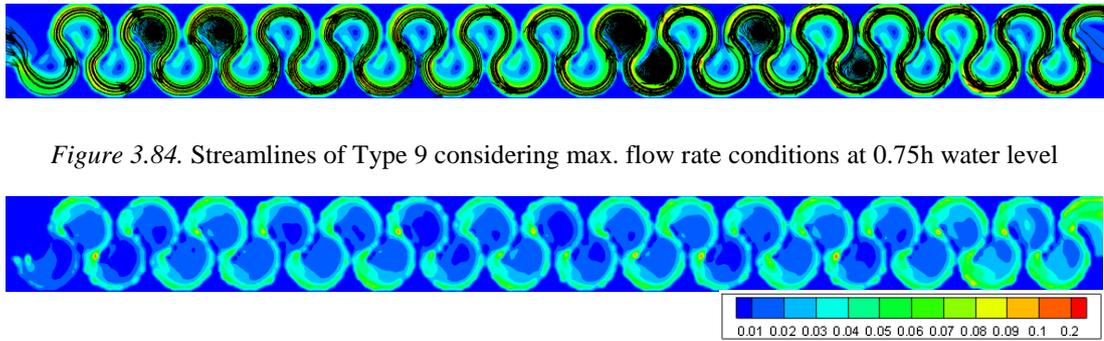
Figure 3.85. TKE of Type 9 considering max. flow rate conditions at 0.75h water level
