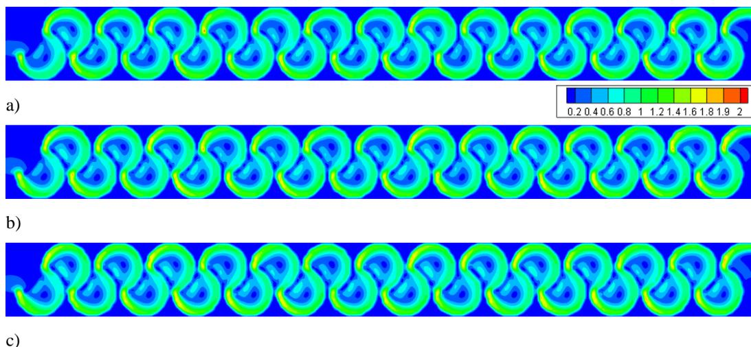
Figure 3.17. Flow velocities of Type 2 considering min. flow rate conditions at water levels of: a) 0.25h, b) 0.50h, c) 0.75h
