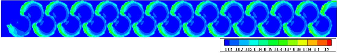
Figure 3.217. TKE of Type 24 considering min. flow rate conditions at 0.75h water level
