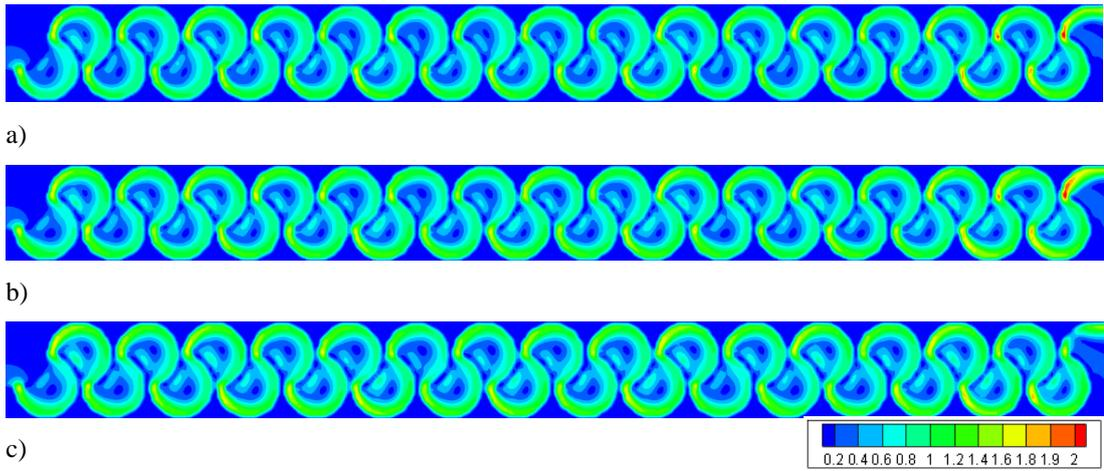
Figure 3.29. Flow velocities of Type 3 considering max. flow rate conditions at water levels of: a) 0.25h, b) 0.50h, c) 0.75h
