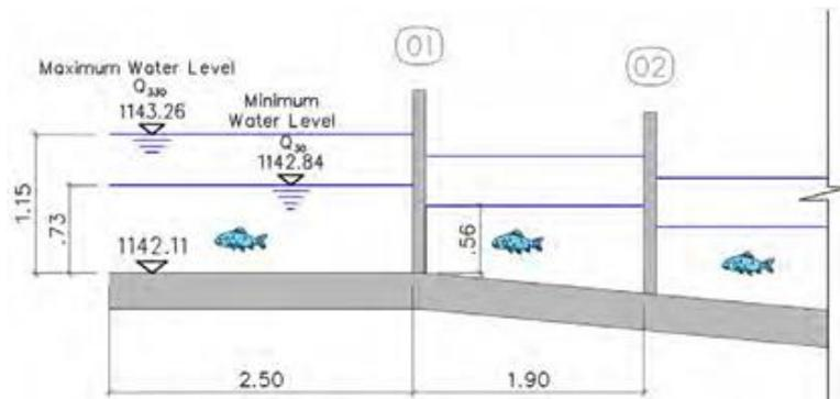
Figure 2.3. Water levels at the conventional vertical slot fish pass exit (Özkaya, 2014)
