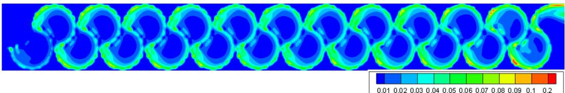
Figure 3.238. TKE of Type 26 considering max. flow rate conditions at 0.75h water level
