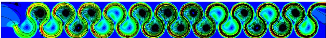
Figure 3.237. Streamlines of Type 26 considering max. flow rate conditions at 0.75h water level
