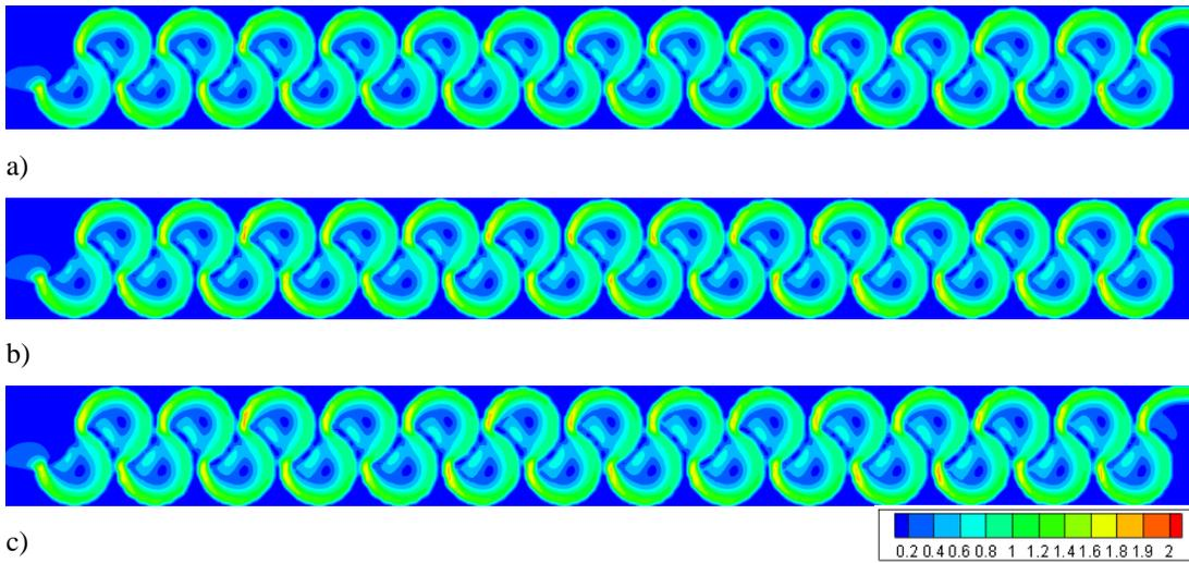
Figure 3.107. Flow velocities of Type 12 considering min. flow rate conditions at water levels of: a) 0.25h, b) 0.50h, c) 0.75h
