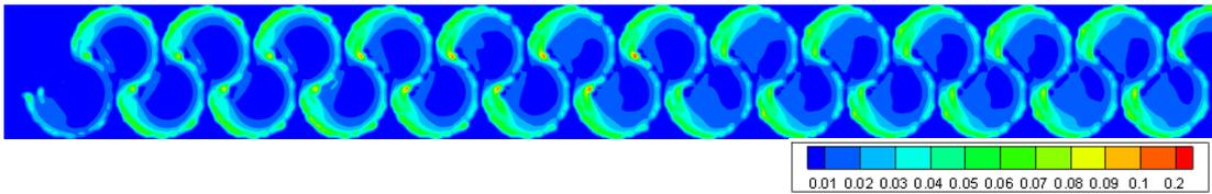
Figure 3.244. TKE of Type 27 considering min. flow rate conditions at 0.75h water level
