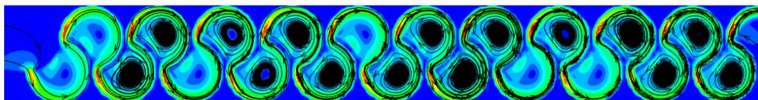
Figure 3.171. Streamlines of Type 19 considering min. flow rate conditions at 0.75h water level
