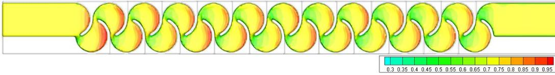
Figure 3.114. Fluid depth of Type 13 considering min. flow rate conditions – Top view
