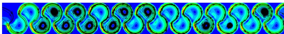
Figure 3.90. Streamlines of Type 10 considering min. flow rate conditions at 0.75h water level
