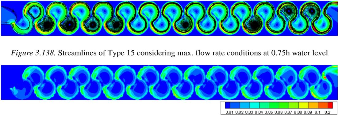
Figure 3.139. TKE of Type 15 considering max. flow rate conditions at 0.75h water level
