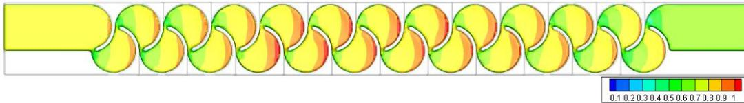
Figure 3.177. Fluid depth of Type 20 considering min. flow rate conditions – Top view
