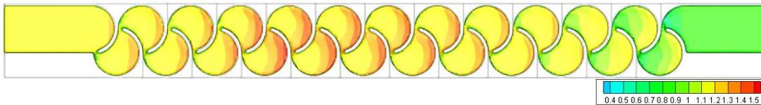
Figure 3.178. Fluid depth of Type 20 considering max. flow rate conditions – Top view
