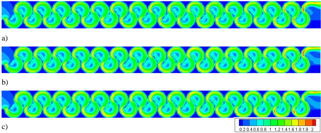
Figure 3.56. TKE of Type 1 considering max. flow rate conditions at 0.75h water level
