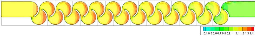
Figure 3.232. Fluid depth of Type 26 considering max. flow rate conditions – Top view
