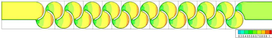
Figure 3.168. Fluid depth of Type 19 considering min. flow rate conditions – Top view
