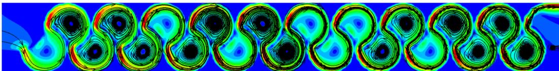
Figure 3.201. Streamlines of Type 22 considering max. flow rate conditions at 0.75h water level
