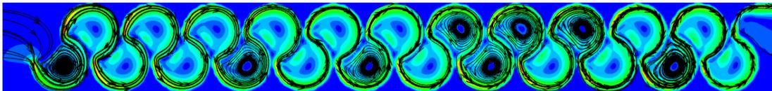
Figure 3.183. Streamlines of Type 20 considering max. flow rate conditions at 0.75h water level
