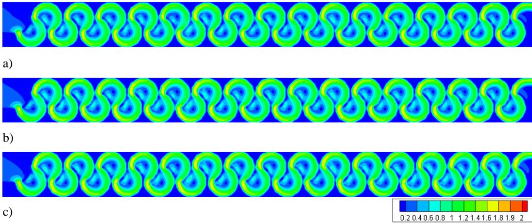
Figure 3.53. Flow velocities of Type 6 considering min. flow rate conditions at water levels of: a) 0.25h, b) 0.50h, c) 0.75h
