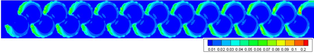
Figure 3.181. TKE of Type 20 considering min. flow rate conditions at 0.75h water level
