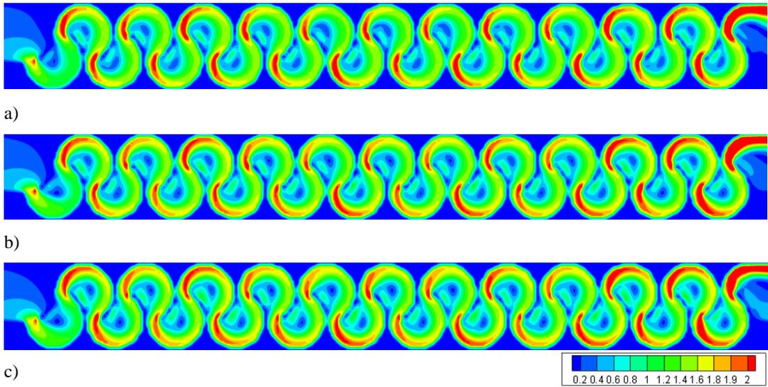
Figure 3.65. Flow velocities of Type 7 considering max. flow rate conditions at water levels of: a) 0.25h, b) 0.50h, c) 0.75h
