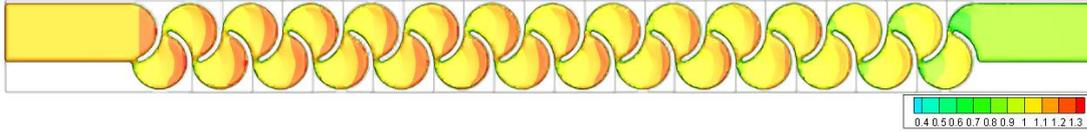
Figure 3.106. Fluid depth of Type 12 considering max. flow rate conditions – Top view
