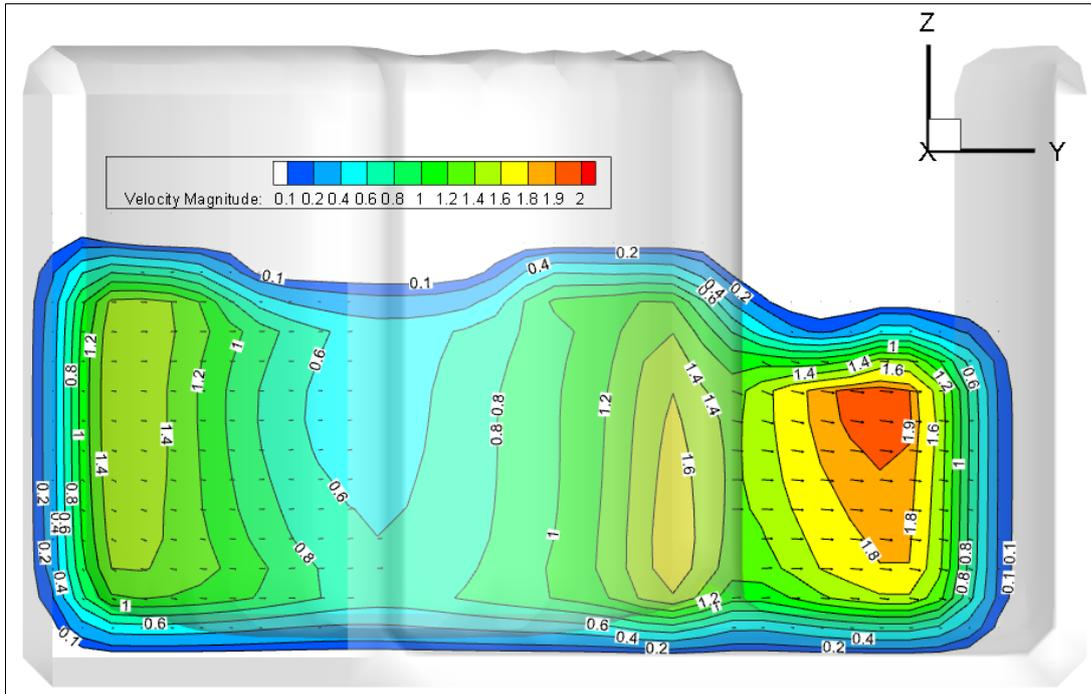
Figure 3.252. Velocity magnitude (xy plane) of section  $y_2$
