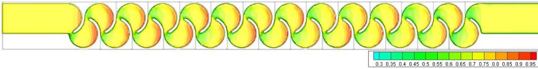
Figure 3.123. Fluid depth of Type 14 considering min. flow rate conditions – Top view
