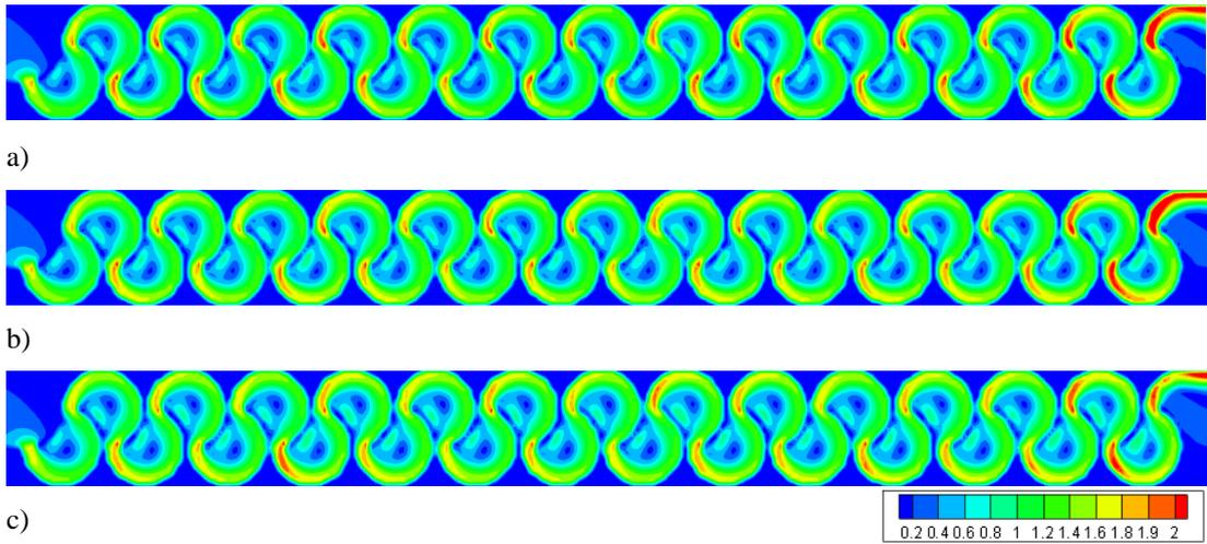
Figure 3.47. Flow velocities of Type 5 considering max. flow rate conditions at water levels of: a) 0.25h, b) 0.50h, c) 0.75h
