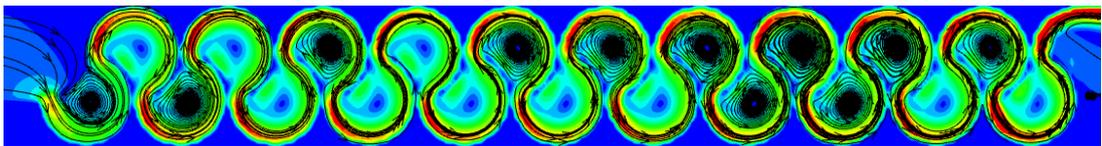
Figure 3.228. Streamlines of Type 25 considering max. flow rate conditions at 0.75h water level
