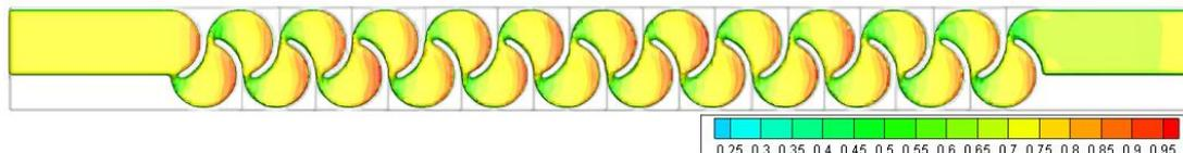
Figure 3.6. Fluid depth of Type 1 considering min. flow rate conditions – Top view
