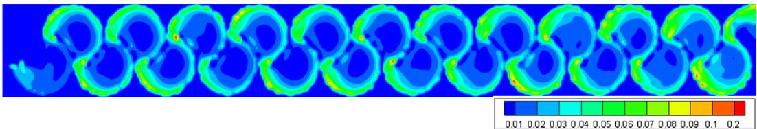
Figure 3.121. TKE of Type 13 considering max. flow rate conditions at 0.75h water level
