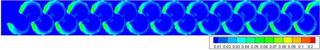
Figure 3.190. TKE of Type 21 considering min. flow rate conditions at 0.75h water level
