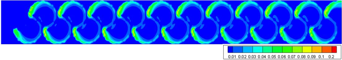
Figure 3.172. TKE of Type 19 considering min. flow rate conditions at 0.75h water level
