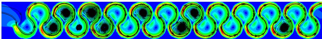
Figure 3.234. Streamlines of Type 26 considering min. flow rate conditions at 0.75h water level
