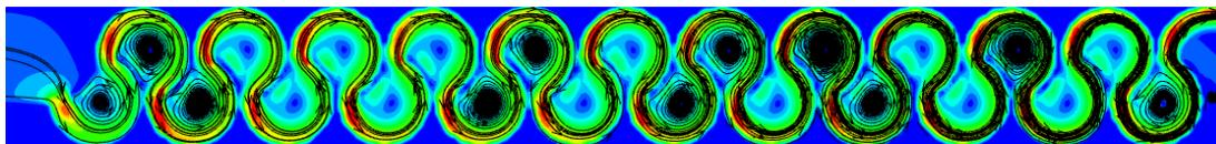
Figure 3.144. Streamlines of Type 16 considering min. flow rate conditions at 0.75h water level
