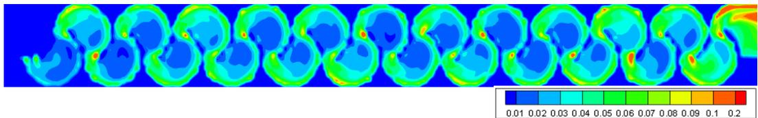
Figure 3.67. TKE of Type 7 considering max. flow rate conditions at 0.75h water level
