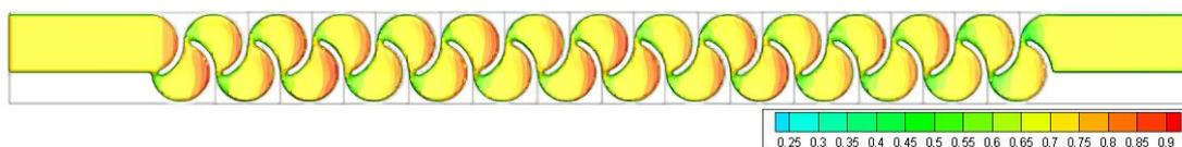
Figure 3.15. Fluid depth of Type 2 considering min. flow rate conditions – Top view
