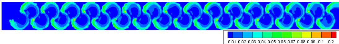
Figure 3.55. TKE of Type 6 considering min. flow rate conditions at 0.75h water level
