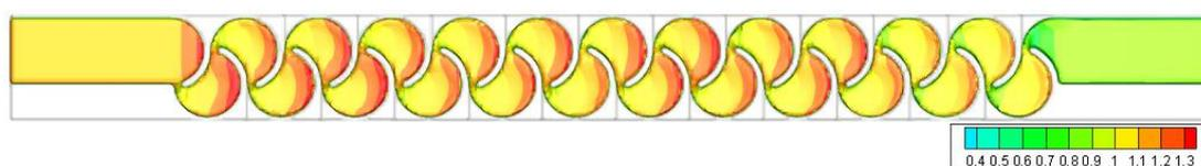
Figure 3.7. Fluid depth of Type 1 considering max. flow rate conditions – Top view
