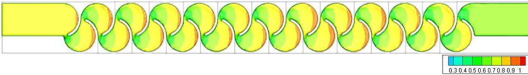
Figure 3.204. Fluid depth of Type 23 considering min. flow rate conditions – Top view
