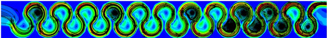
Figure 3.66. Streamlines of Type 7 considering max. flow rate conditions at 0.75h water level
