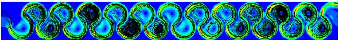
Figure 3.12. Streamlines of Type 1 considering max. flow rate conditions at 0.75h water level
