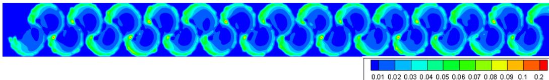
Figure 3.46. TKE of Type 5 considering min. flow rate conditions at 0.75h water level
