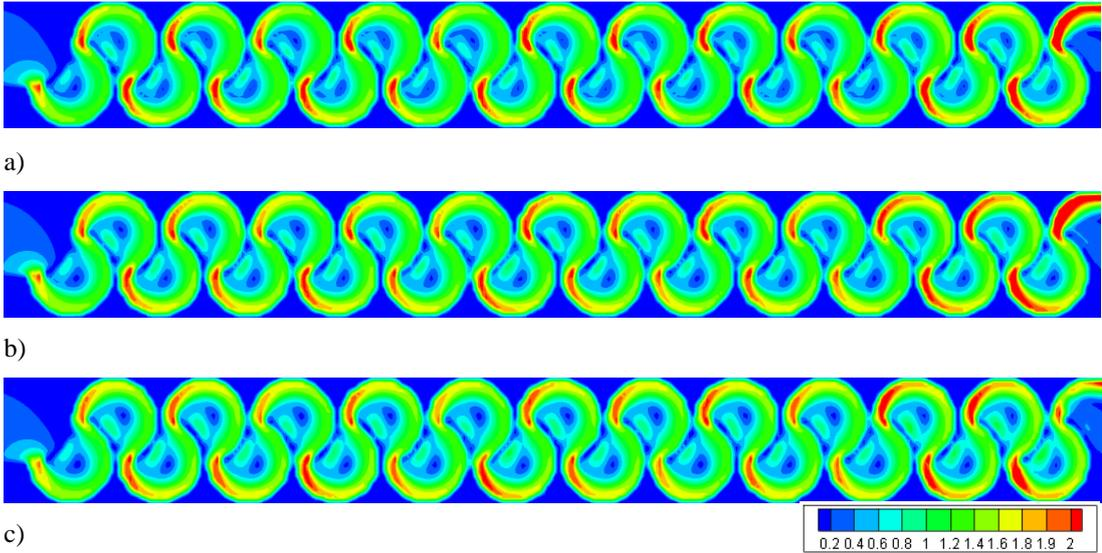
Figure 3.38. Flow velocities of Type 4 considering max. flow rate conditions at water levels of: a) 0.25h, b) 0.50h, c) 0.75h
