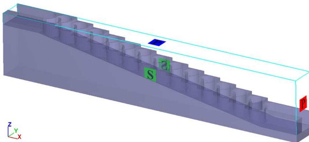
Figure 3.3. Boundary conditions for a typical fish pass
