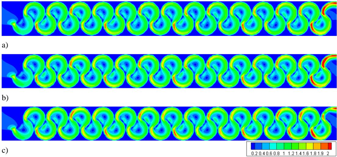
Figure 3.137. Flow velocities of Type 15 considering max. flow rate conditions at water levels of: a) 0.25h, b) 0.50h, c) 0.75h
