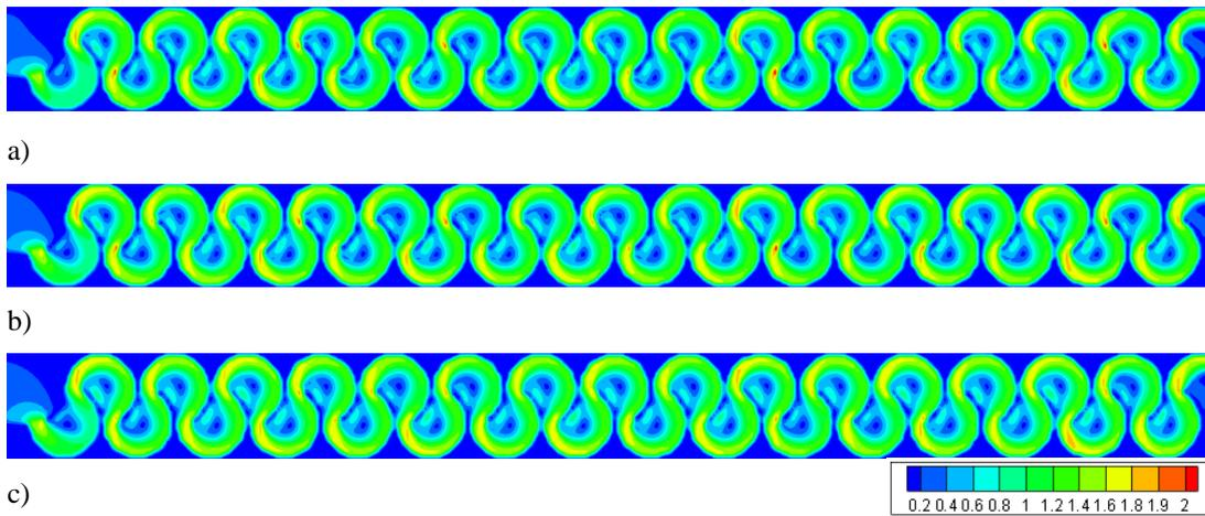
Figure 3.80. Flow velocities of Type 9 considering min. flow rate conditions at water levels of: a) 0.25h, b) 0.50h, c) 0.75h
