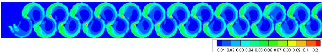
Figure 3.154. TKE of Type 17 considering min. flow rate conditions at 0.75h water level
