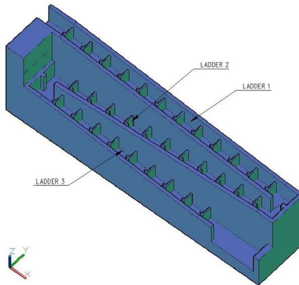
Figure 2.1. 3D solid model of the fish ladder (Özkaya, 2014)
