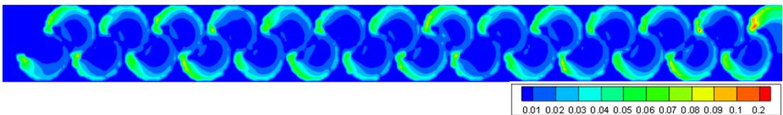
Figure 3.22. TKE of Type 2 considering max. flow rate conditions at 0.75h water level
