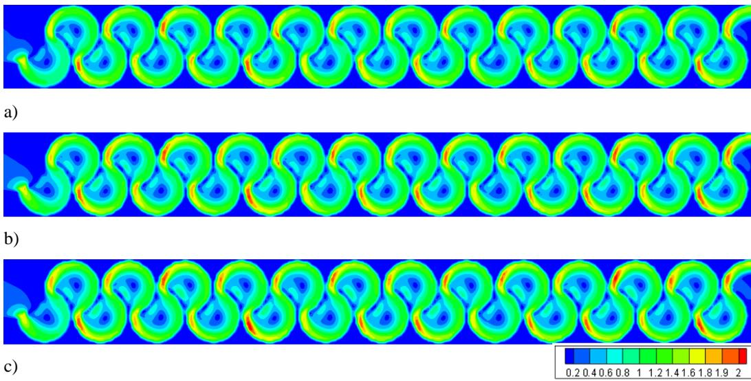
Figure 3.125. Flow velocities of Type 14 considering min. flow rate conditions at water levels of: a) 0.25h, b) 0.50h, c) 0.75h
