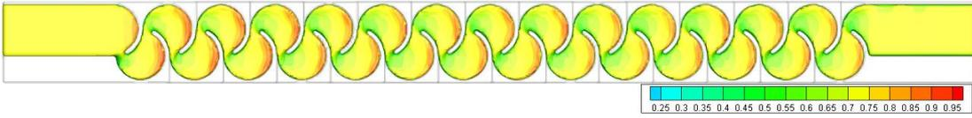
Figure 3.159. Fluid depth of Type 18 considering min. flow rate conditions – Top view
