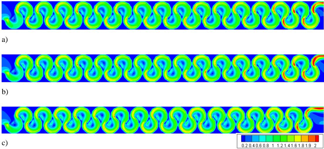
Figure 3.83. Flow velocities of Type 9 considering max. flow rate conditions at water levels of: a) 0.25h, b) 0.50h, c) 0.75h
