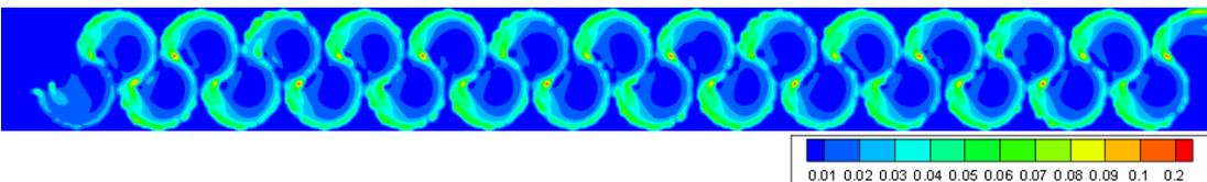
Figure 3.163. TKE of Type 18 considering min. flow rate conditions at 0.75h water level
