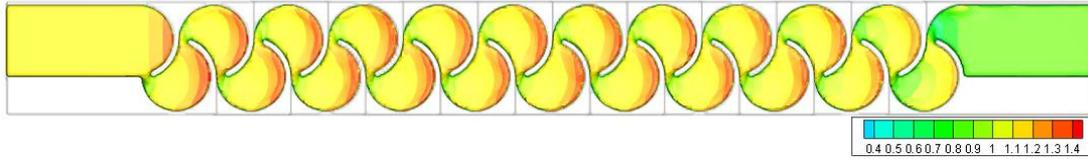
Figure 3.196. Fluid depth of Type 22 considering max. flow rate conditions – Top view
