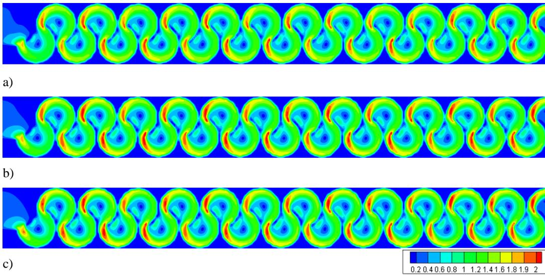
Figure 3.152. Flow velocities of Type 17 considering min. flow rate conditions at water levels of: a) 0.25h, b) 0.50h, c) 0.75h
