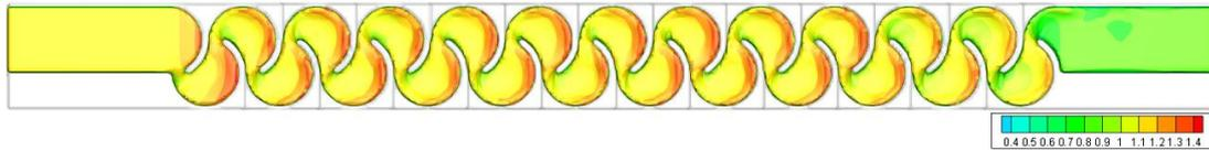
Figure 3.61. Fluid depth of Type 7 considering max. flow rate conditions – Top view
