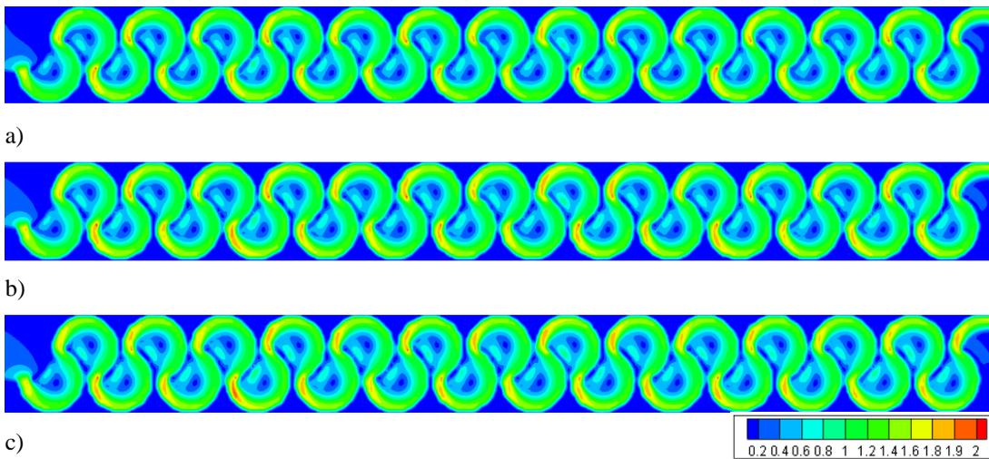
Figure 3.44. Flow velocities of Type 5 considering min. flow rate conditions at water levels of: a) 0.25h, b) 0.50h, c) 0.75h
