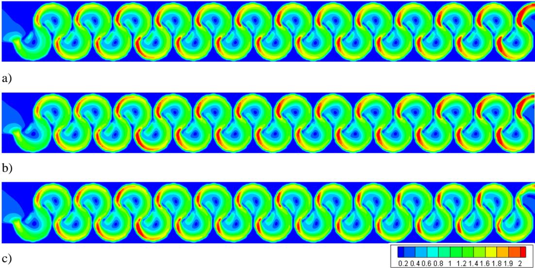
Figure 3.245. Flow velocities of Type 27 considering max. flow rate conditions at water levels of: a) 0.25h, b) 0.50h, c) 0.75h
