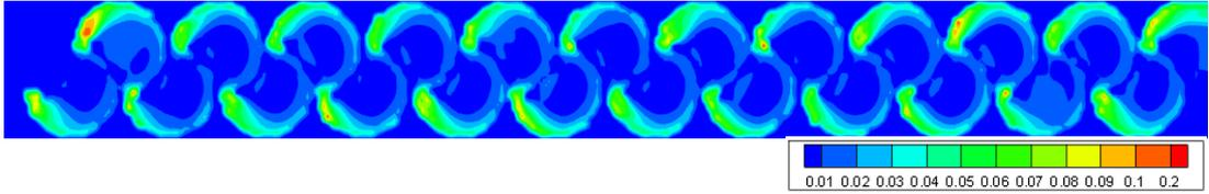
Figure 3.10. TKE of Type 1 considering min. flow rate conditions at 0.75h water level
