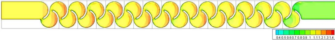
Figure 3.133. Fluid depth of Type 15 considering max. flow rate conditions – Top view
