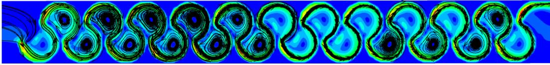
Figure 3.9. Streamlines of Type 1 considering min. flow rate conditions at 0.75h water level
