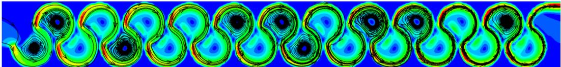
Figure 3.210. Streamlines of Type 23 considering max. flow rate conditions at 0.75h water level
