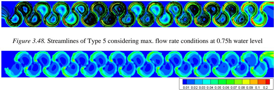
Figure 3.48. Streamlines of Type 5 considering max. flow rate conditions at 0.75h water level
