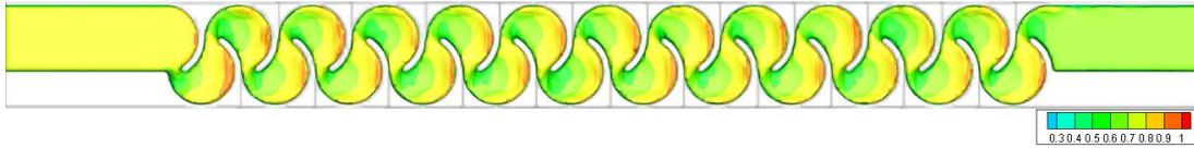
Figure 3.60. Fluid depth of Type 7 considering min. flow rate conditions – Top view
