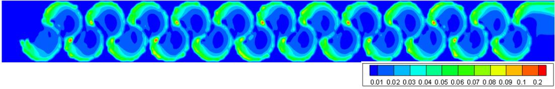
Figure 3.37. TKE of Type 4 considering min. flow rate conditions at 0.75h water level
