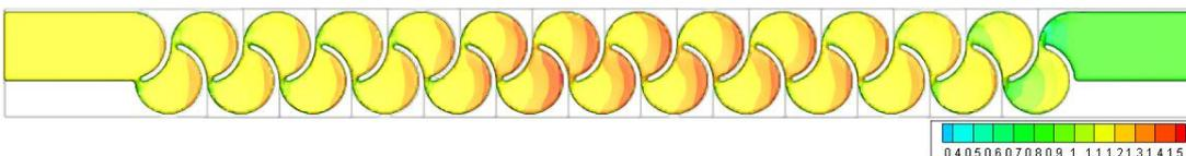
Figure 3.187. Fluid depth of Type 21 considering max. flow rate conditions – Top view
