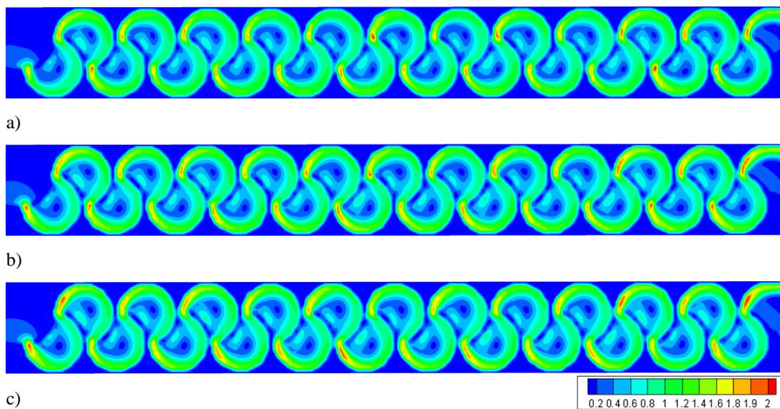
Figure 3.8. Flow velocities of Type 1 considering min. flow rate conditions at water levels of: a) 0.25h, b) 0.50h, c) 0.75h
