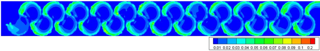
Figure 3.127. TKE of Type 14 considering min. flow rate conditions at 0.75h water level
