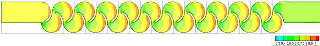
Figure 3.222. Fluid depth of Type 25 considering min. flow rate conditions – Top view
