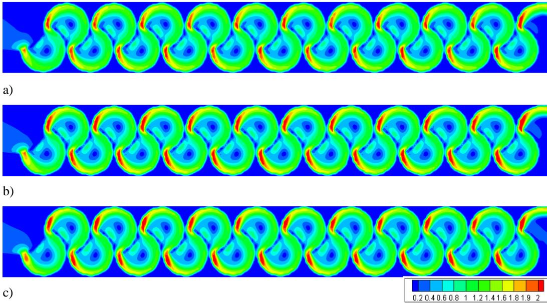
Figure 3.197. Flow velocities of Type 22 considering min. flow rate conditions at water levels of: a) 0.25h, b) 0.50h, c) 0.75h
