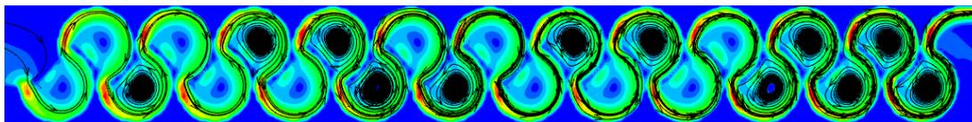
Figure 3.207. TKE of Type 23 considering min. flow rate conditions at 0.75h water level
