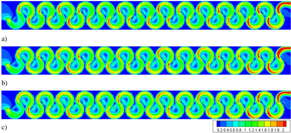
Figure 3.74. Flow velocities of Type 8 considering max. flow rate conditions at water levels of: a) 0.25h, b) 0.50h, c) 0.75h
