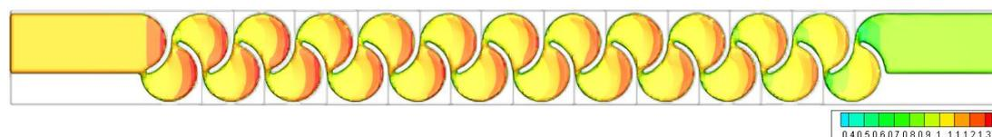
Figure 3.88. Fluid depth of Type 10 considering max. flow rate conditions – Top view
