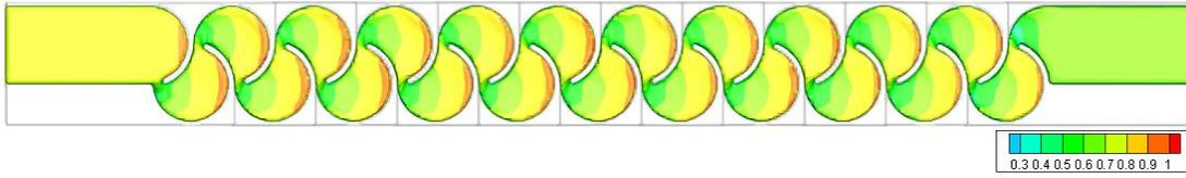
Figure 3.195. Fluid depth of Type 22 considering min. flow rate conditions – Top view
