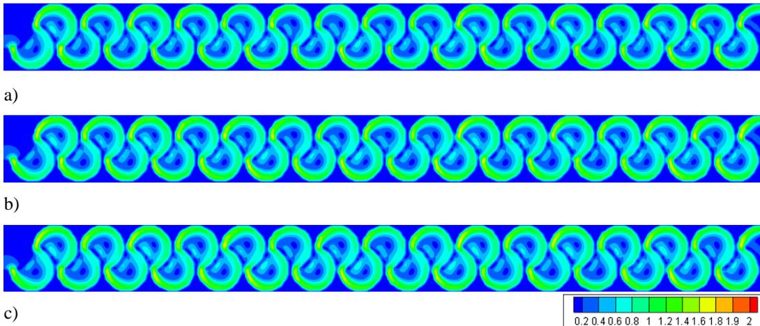
Figure 3.26. Flow velocities of Type 3 considering min. flow rate conditions at water levels of: a) 0.25h, b) 0.50h, c) 0.75h
