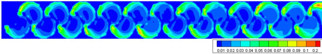
Figure 3.13. TKE of Type 1 considering max. flow rate conditions at 0.75h water level
