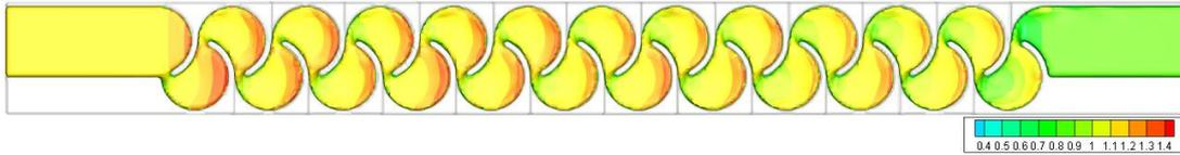
Figure 3.115. Fluid depth of Type 13 considering max. flow rate conditions – Top view
