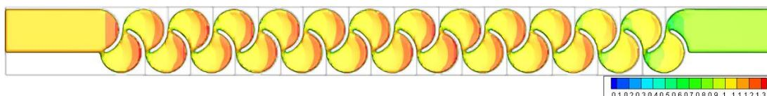
Figure 3.97. Fluid depth of Type 11 considering max. flow rate conditions – Top view
