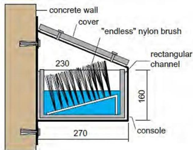
Figure 1.5. The eel ladder at Zeltingen dam on Moselle River (DWA-M 509)
