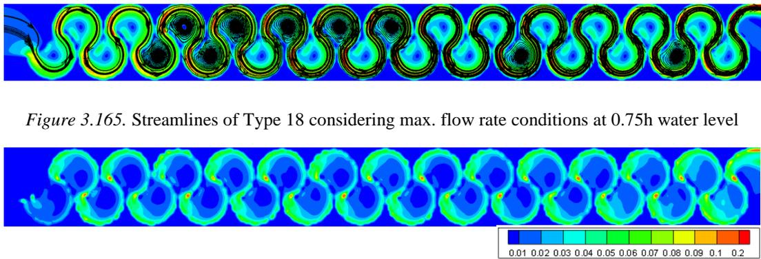
Figure 3.166. TKE of Type 18 considering max. flow rate conditions at 0.75h water level
