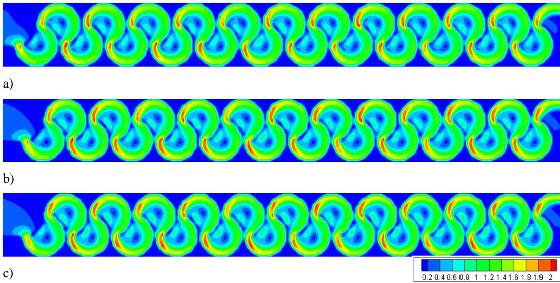
Figure 3.35. Flow velocities of Type 4 considering min. flow rate conditions at water levels of: a) 0.25h, b) 0.50h, c) 0.75h
