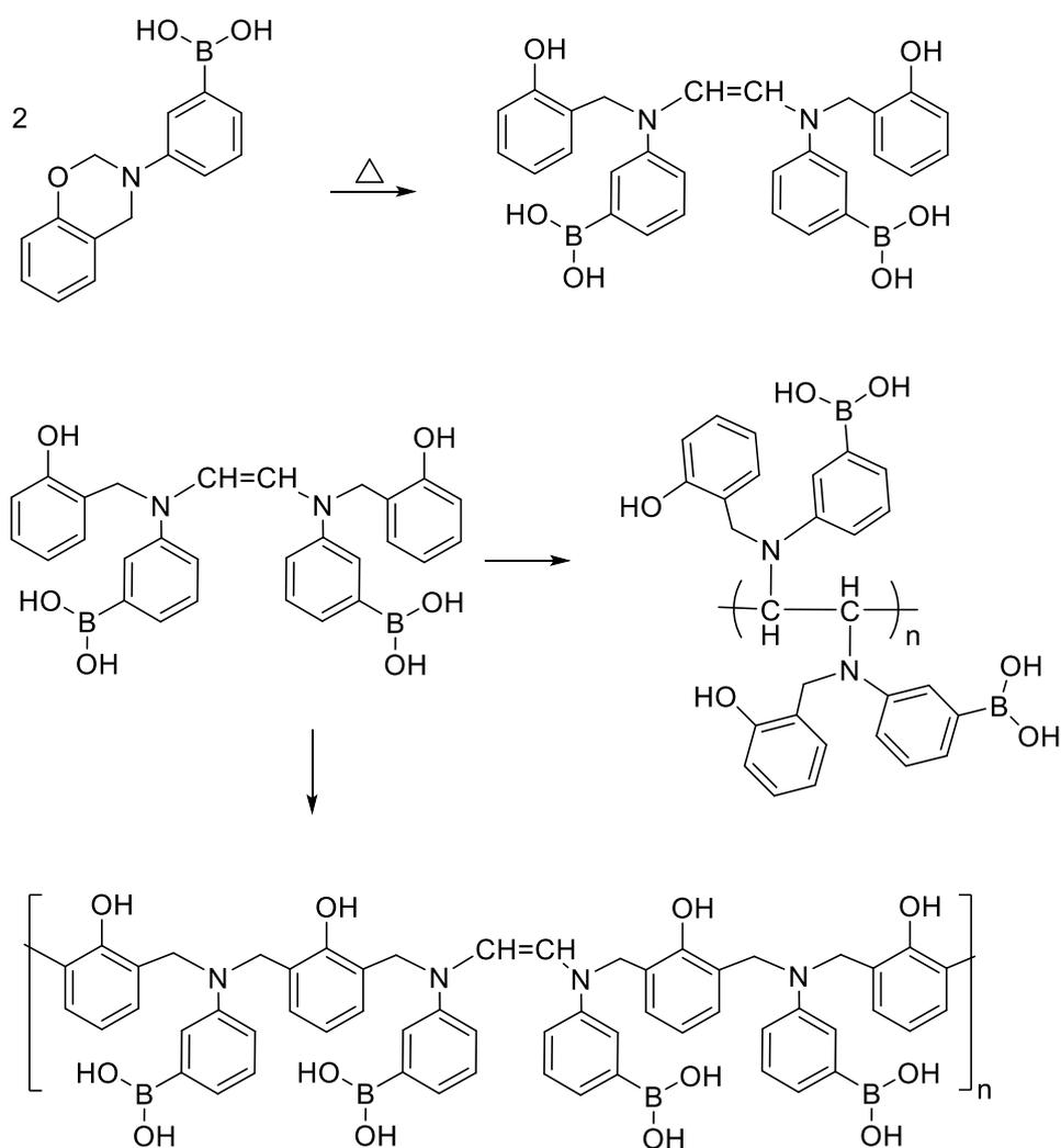
Scheme 3.5. Generation and polymerization of benzoxazine dimers
