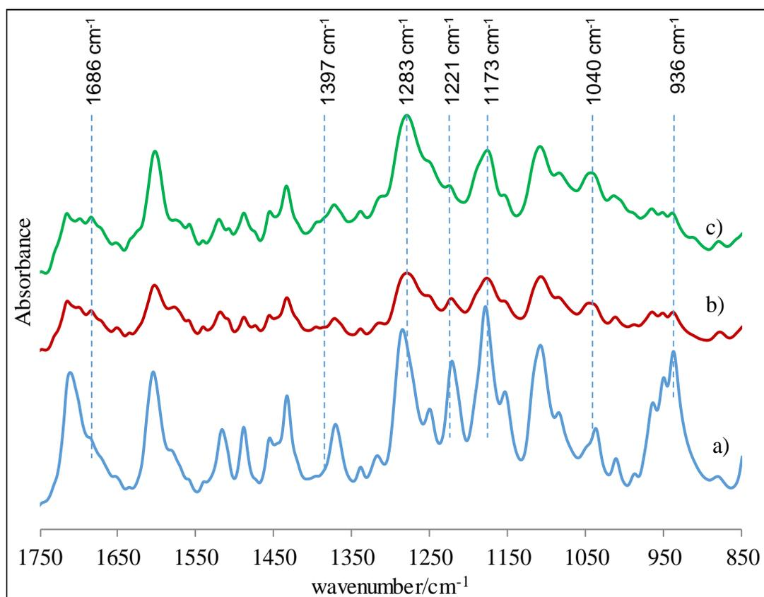
Figure 3.17. FTIR spectra of a) Pab monomer, b) PPab polymer and c) PPab/15BPDBA composite
