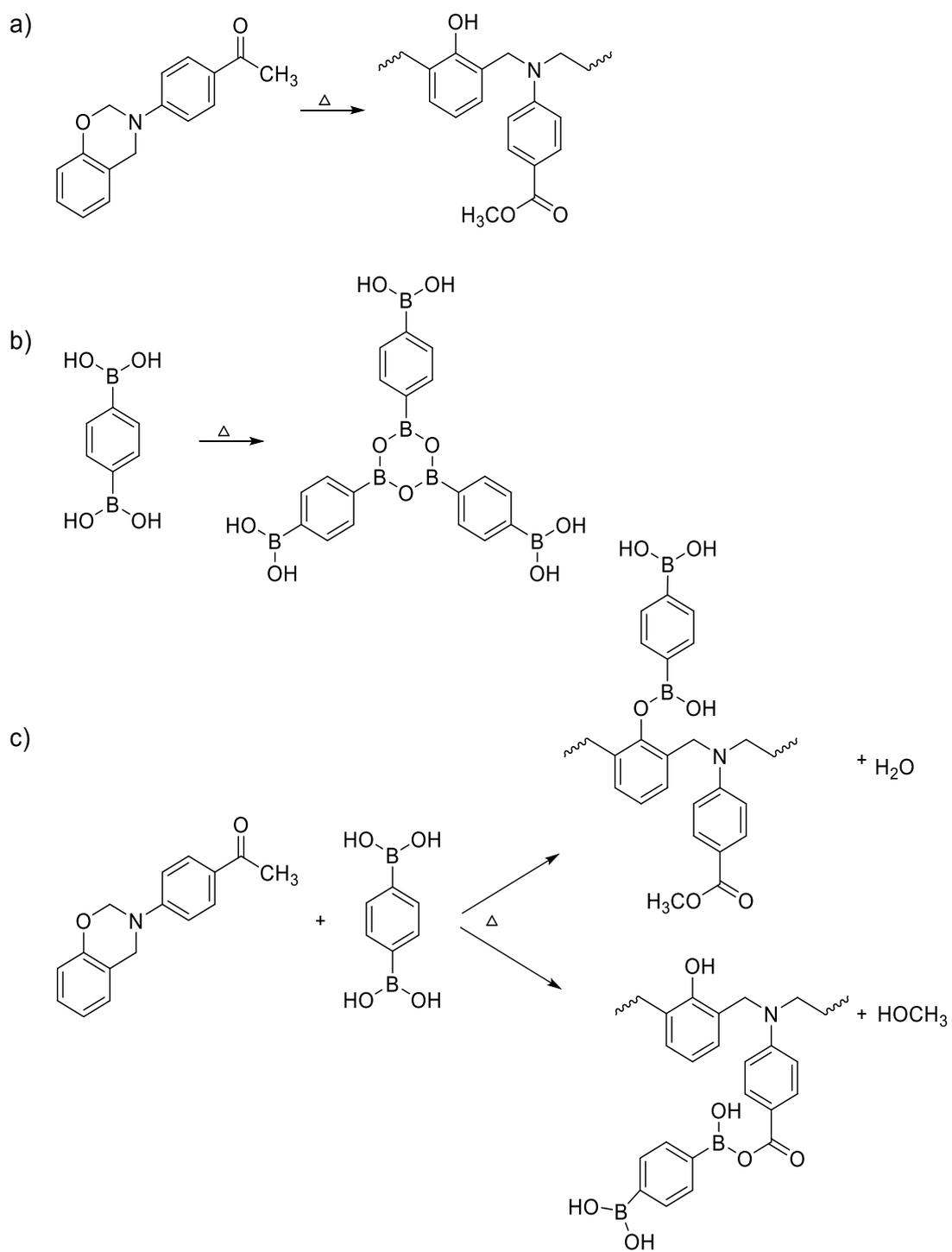
Scheme 3.8. Interactions during curing process of PPab/BDBA composites
