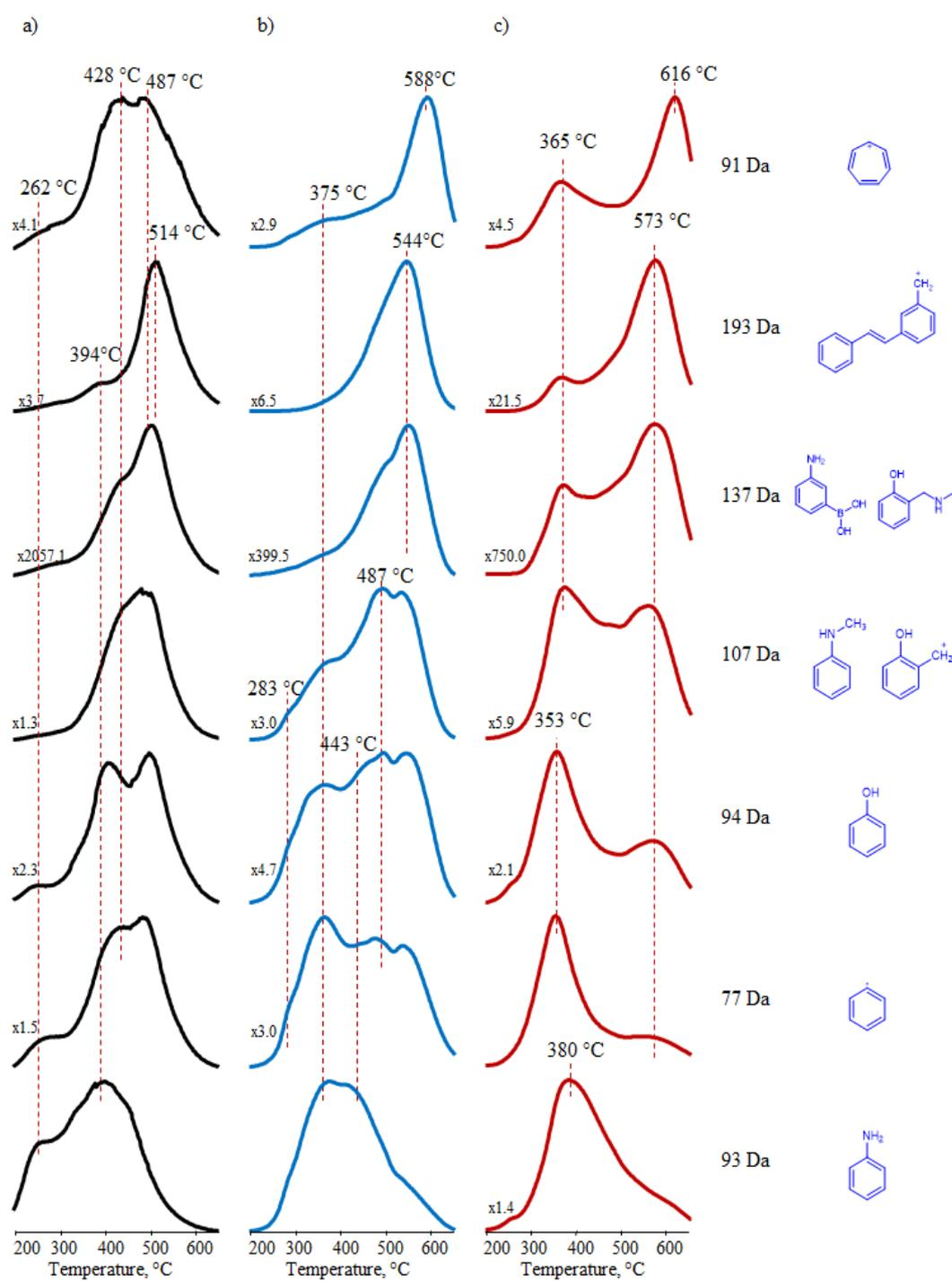
Figure 3.7. Single ion evolution profiles of a) PBz, b) PBz-50PBA and c) PBz-100APBA
