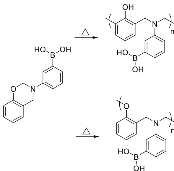
*Scheme 3.4.* Ring opening polymerization of Bz-100APBA
