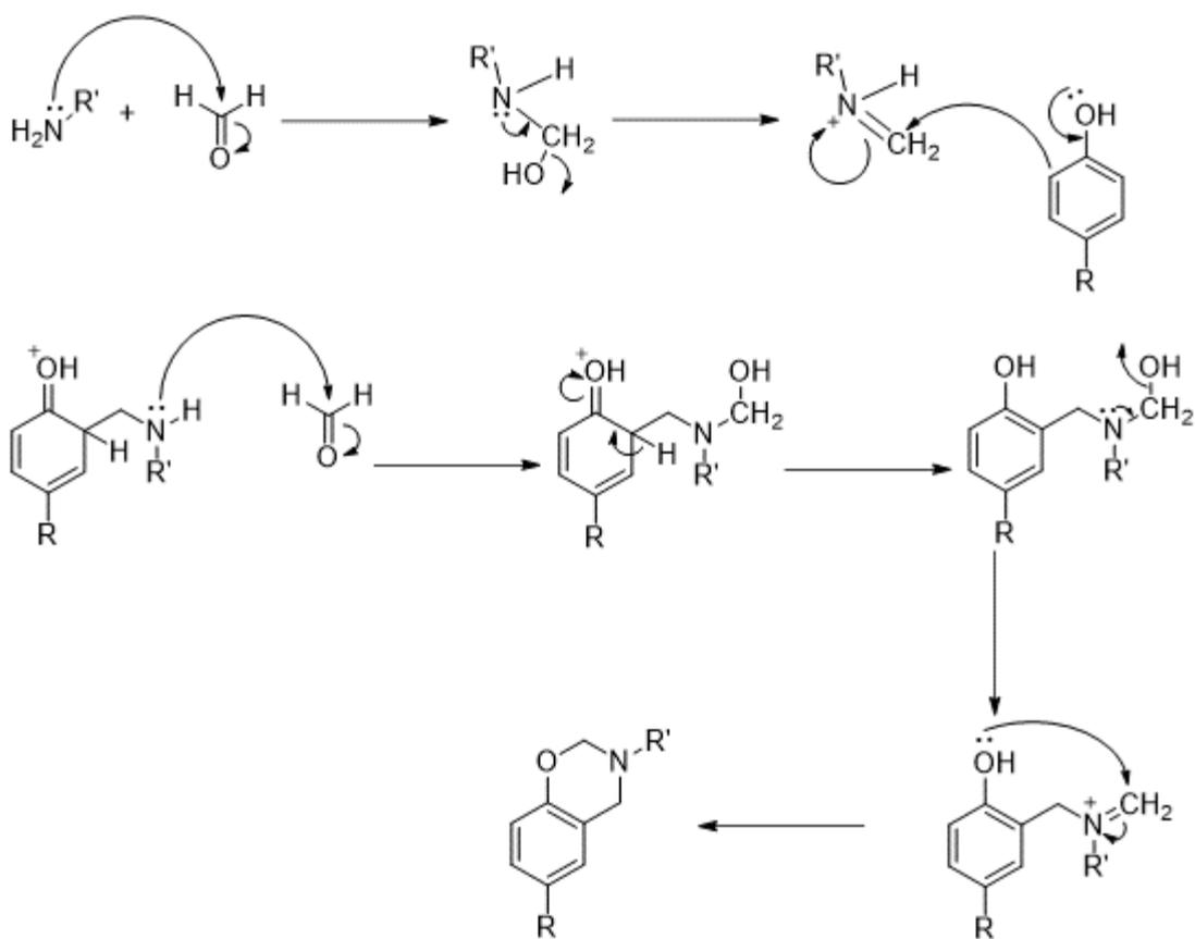
Scheme 1.3. Suggested mechanism for the synthesis of benzoxazine monomer
