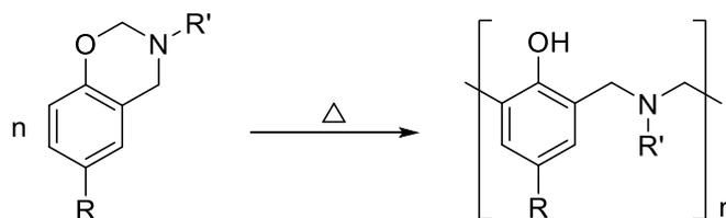
*Scheme 1.1.* Structure of benzoxazine monomer and polybenzoxazine
