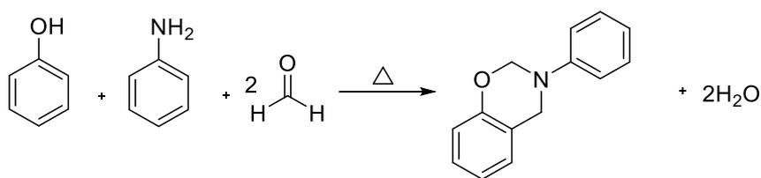
Scheme 3.1. Synthesis of benzoxazine based on phenol and aniline
