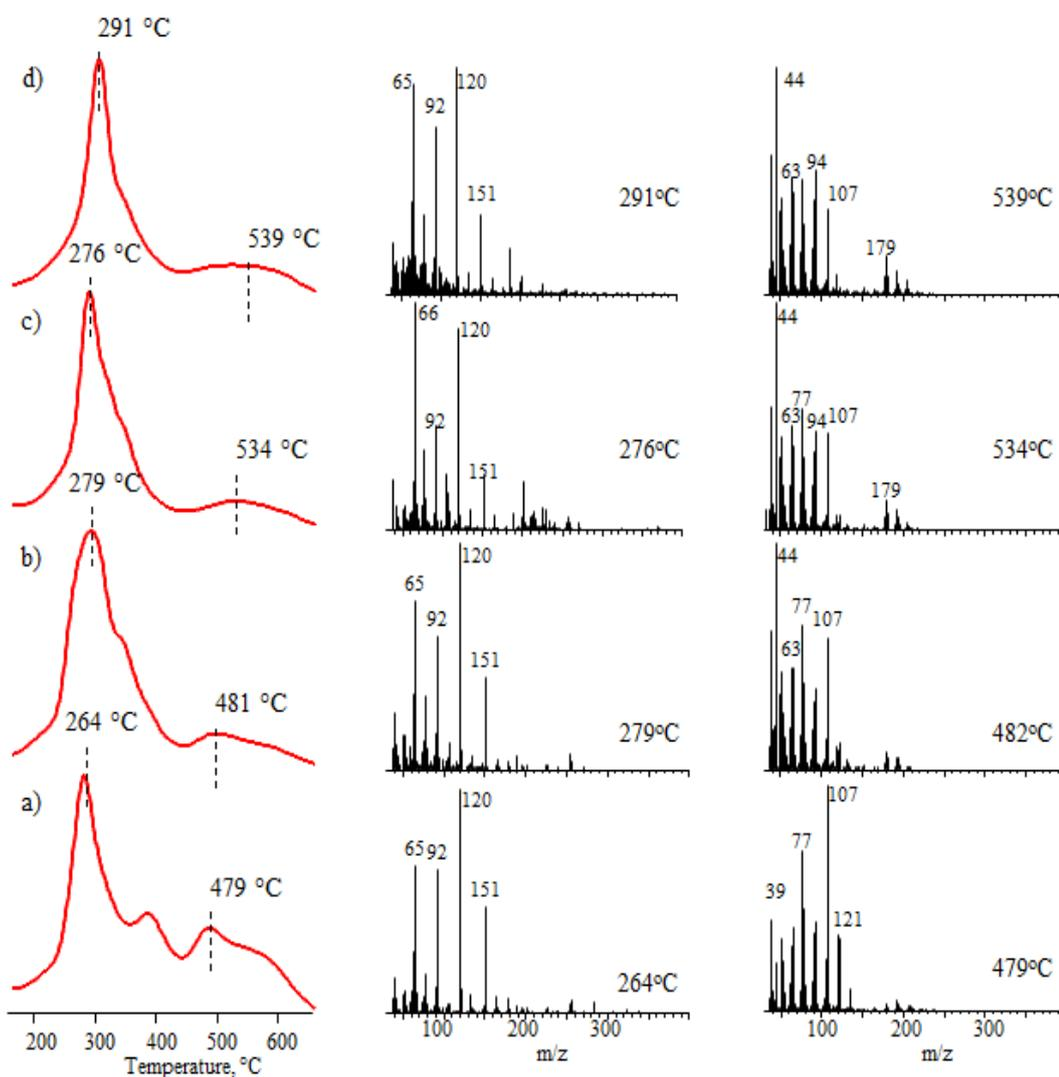
Figure 3.15. Total ion current curves and mass spectra of a) PPab, b) PPab/5BDBA, c) PPab/10BDBA and d) PPab/15BDBA
