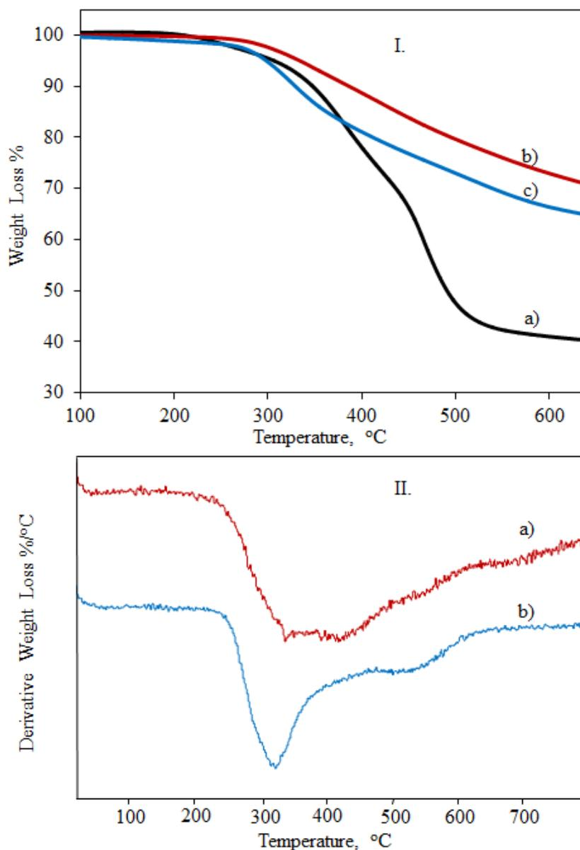
Figure 3.5. I. TGA curves of a) Bz, b) Bz-50APBA and c) Bz-100APBA monomers, II. DTA curves of a) PBz-50APBA and b) PBz-100 polymers
