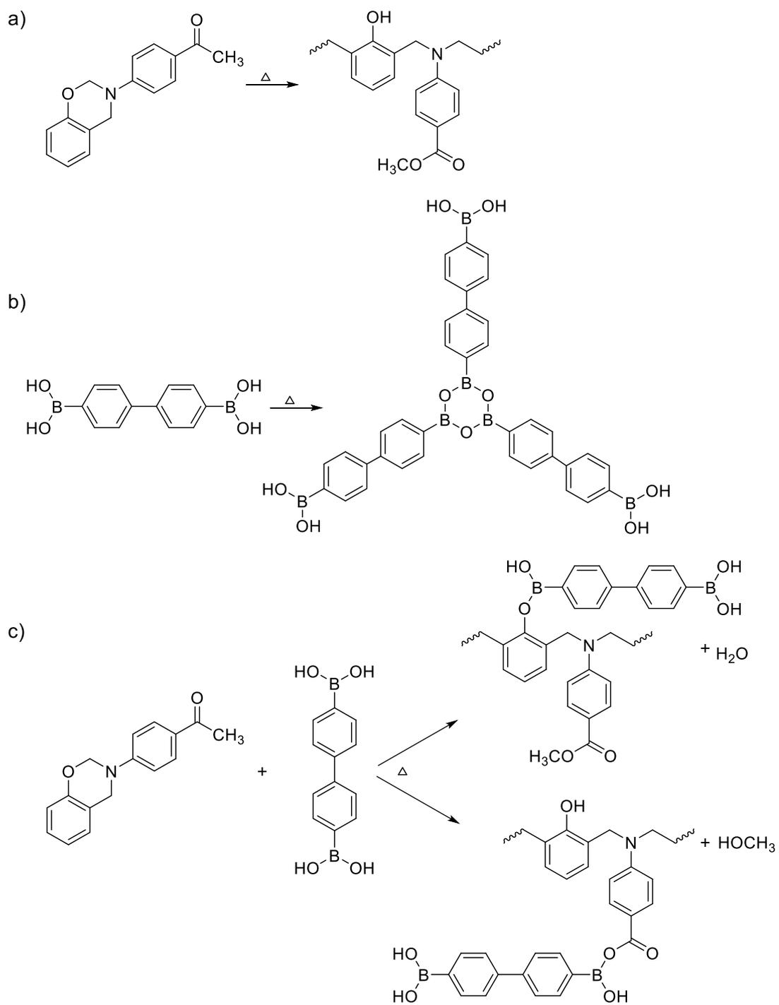
*Scheme 3.9.* Interactions during curing process of PPab/BPDBA composites
