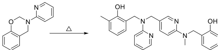
*Scheme 1.12.* Ring opening polymerization of benzoxazines
