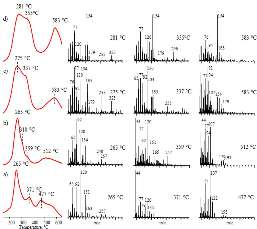
Figure 3.20. Total ion current curves and mass spectra of a) PPab, b) PPab/5BPDBA, c) PPab/10BPDBA and d) PPab/15BPDBA
