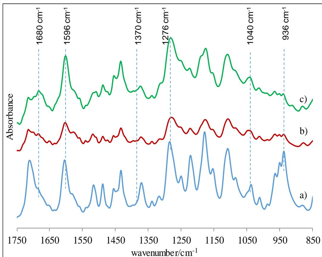
Figure 3.22. FTIR spectra of a) Pab monomer, b) PPab polymer and c) PPab/10HPBA composite
