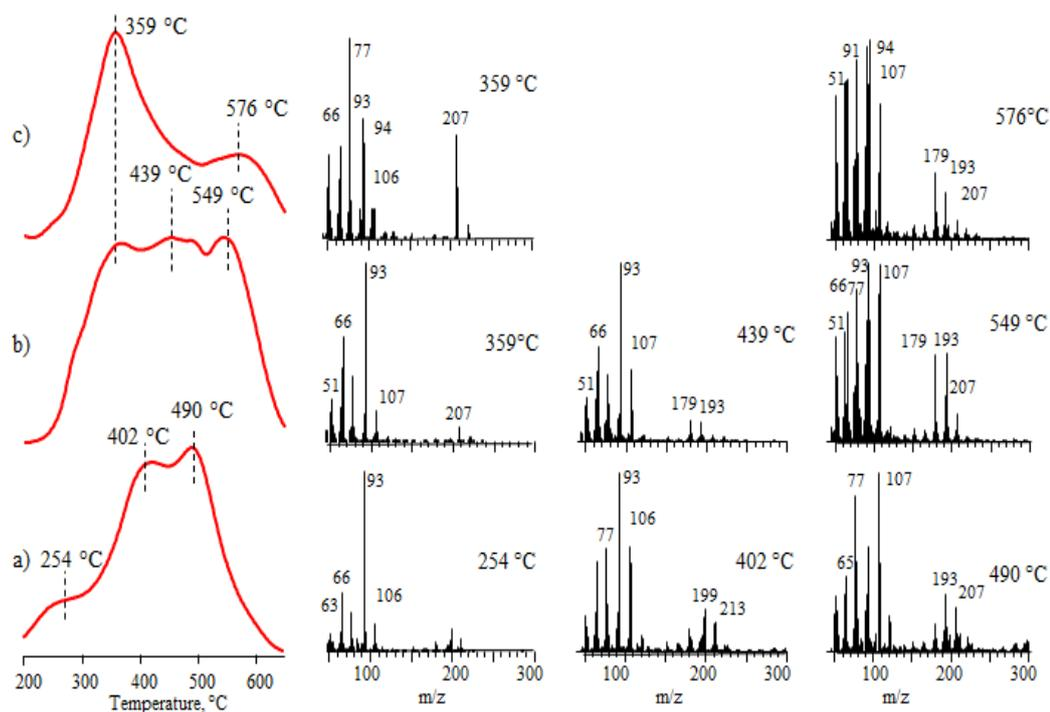
Figure 3.6. Total ion current curves and mass spectra of a) PBz, b) PBz-50PBA and c) PBz-100APBA
