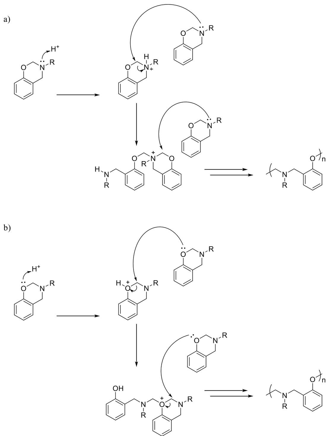
Scheme 1.11. Phenoxyl type of polymerization mechanisms of benzoxazine
