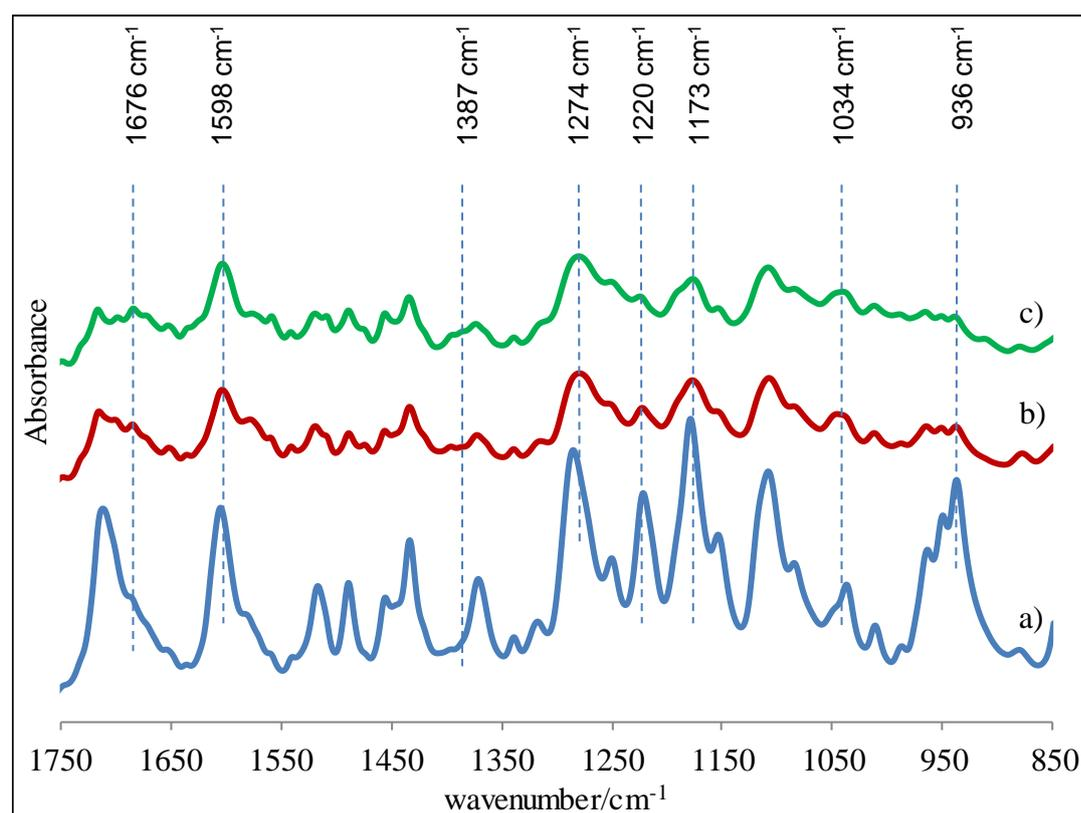
Figure 3.12. FTIR spectra of a) Pab monomer, b) PPab polymer and c) PPab/15BDBA composite
