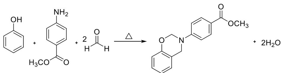
*Scheme 3.6.* Synthesis of benzoxazine based on phenol and 4-aminomethyl benzoate
