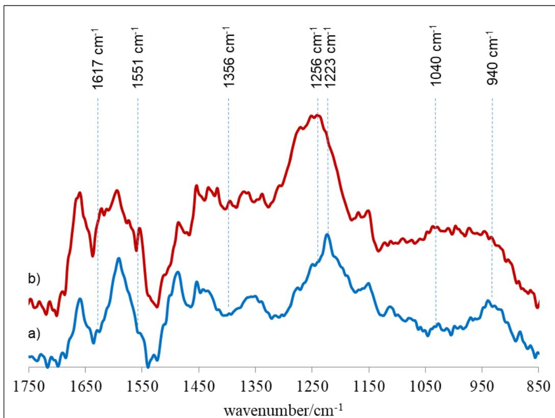
Figure 3.3. FTIR spectra of a) Bz-100APBA monomer and the b) PBz-100 polymer
