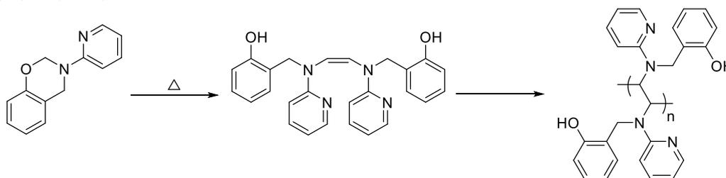
*Scheme 1.13.* Polymerization of benzoxazines based on dimer formation
