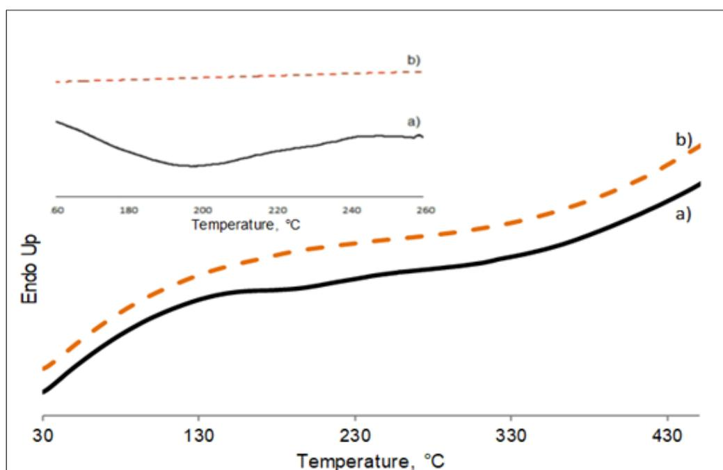
Figure 3.4. DSC curves of a) Bz-100APBA monomer and the b) PBz-100 polymer
