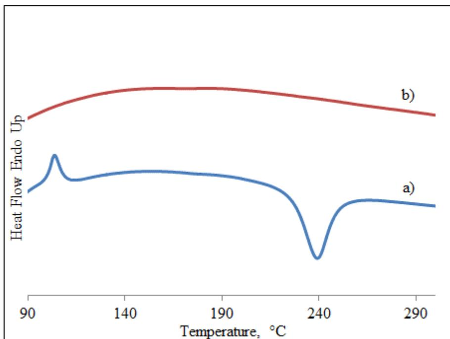
Figure 3.11. DSC spectra of a) Pab monomer and b) PPab polymer
