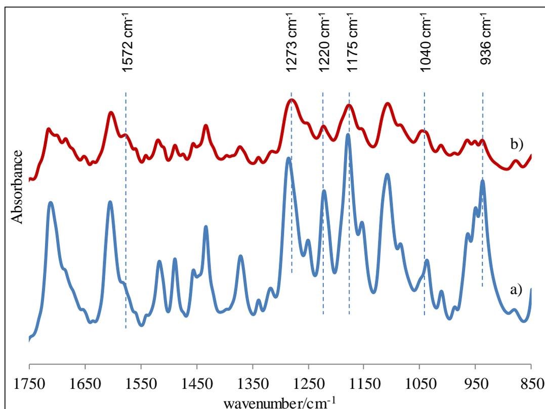
Figure 3.10. FTIR spectra of a) Pab monomer and b) PPab polymer
