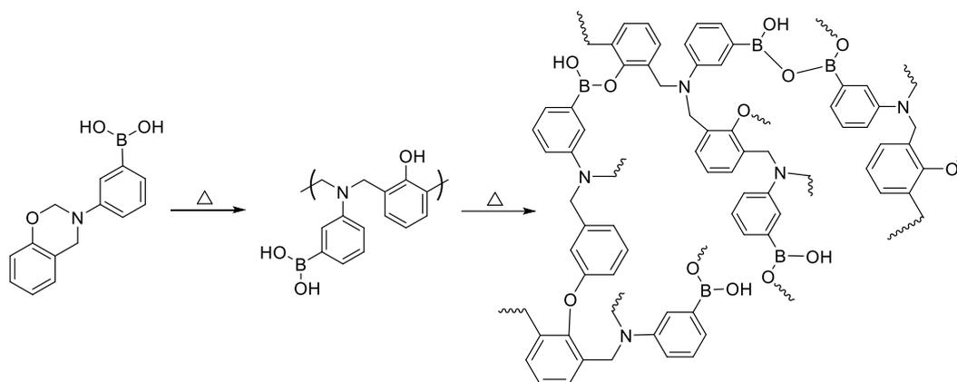
Scheme 3.3. Crosslinking during polymerization of Bz-100APBA monomer
