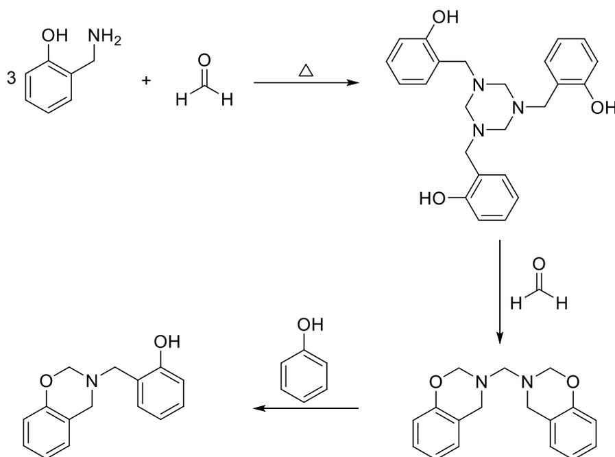
*Scheme 1.5.* The synthetic method of benzoxazines by Holly and Cope
