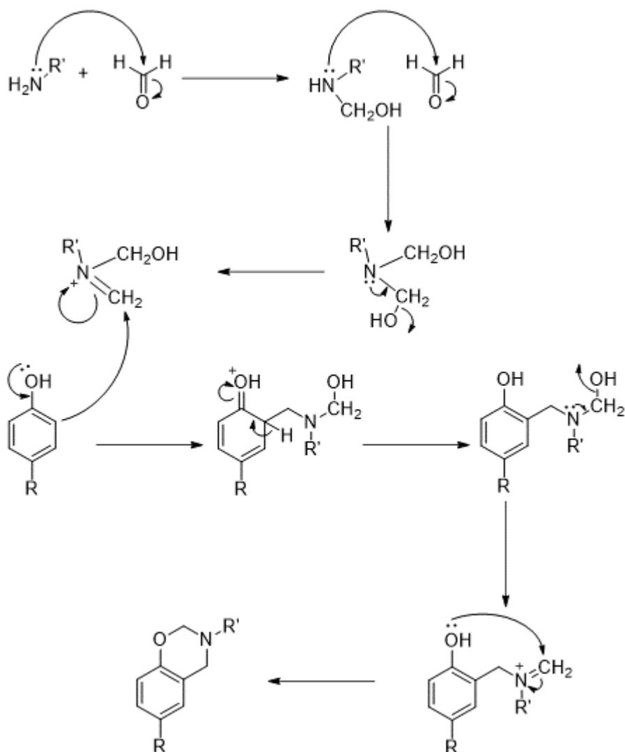
*Scheme 1.4.* Suggested mechanism for the synthesis of benzoxazine monomer
