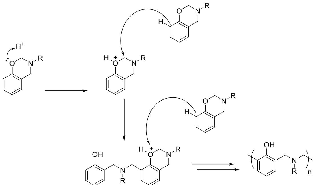
*Scheme 1.10.* Phenolic type of polymerization mechanism of benzoxazine
