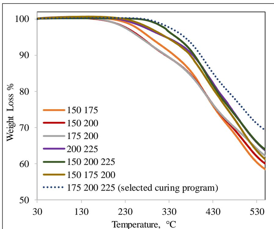
Figure 3.2. TGA curves different temperature programs applied to Bz-100APBA
