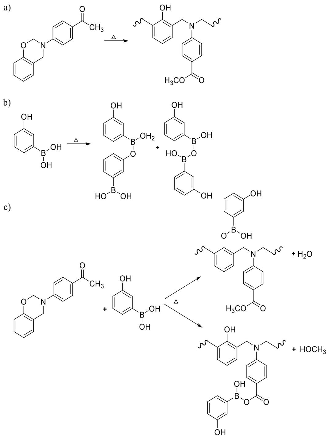
*Scheme 3.10.* Interactions during curing process of PPab/HPBA composites
