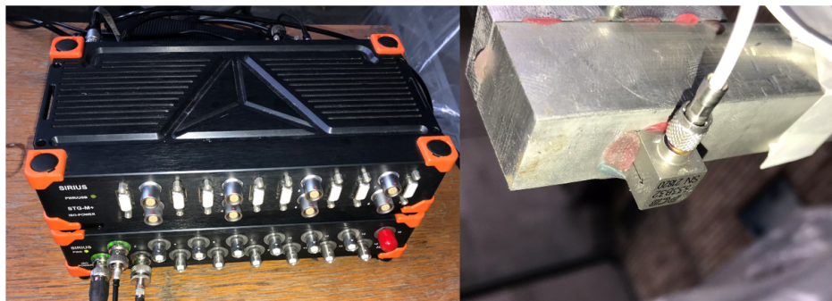
Figure 5.30: Data Acquisition Device and Accelerometer-2
