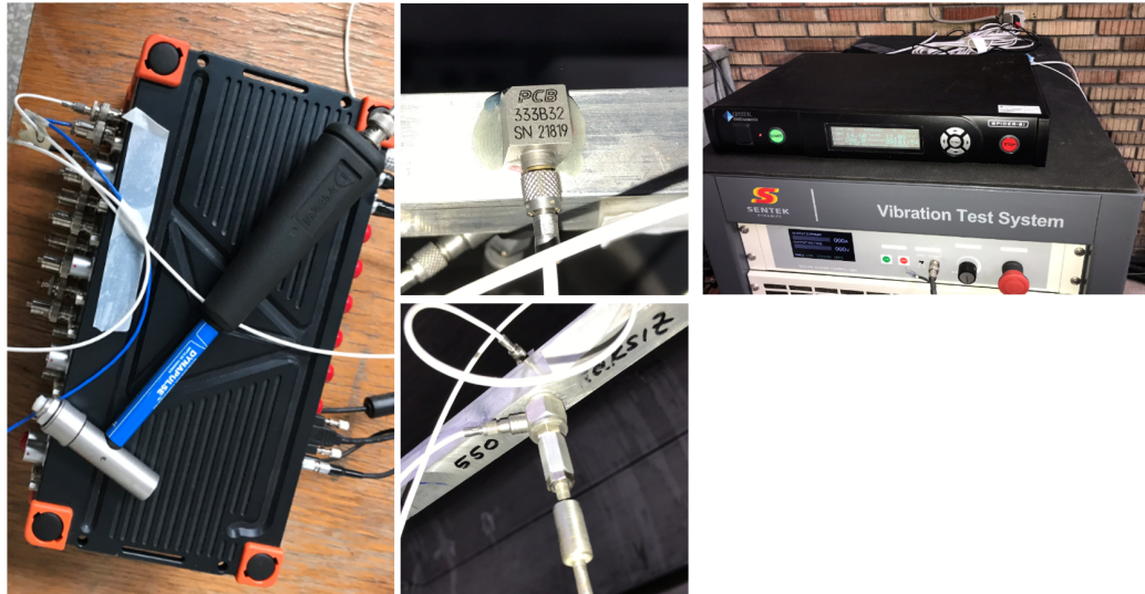
Figure 5.31: Impact Hammer, Accelerometer-1, Accelerometer-3, and Dynamic Shaker Control
