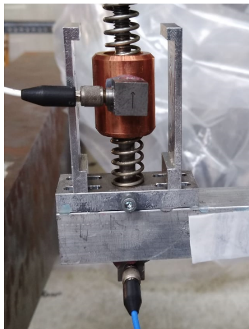
Figure 5.38: TVA attachment to beam
