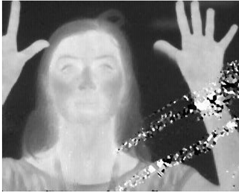
Figure 4.32. Indoor image taken by 320x256 heterojunction FPA.
