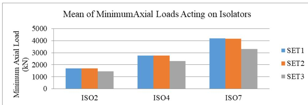
Figure 4.11. Mean Average Minimum Axial Loads Acting on Isolators of each GM Set Obtained from NTHA
