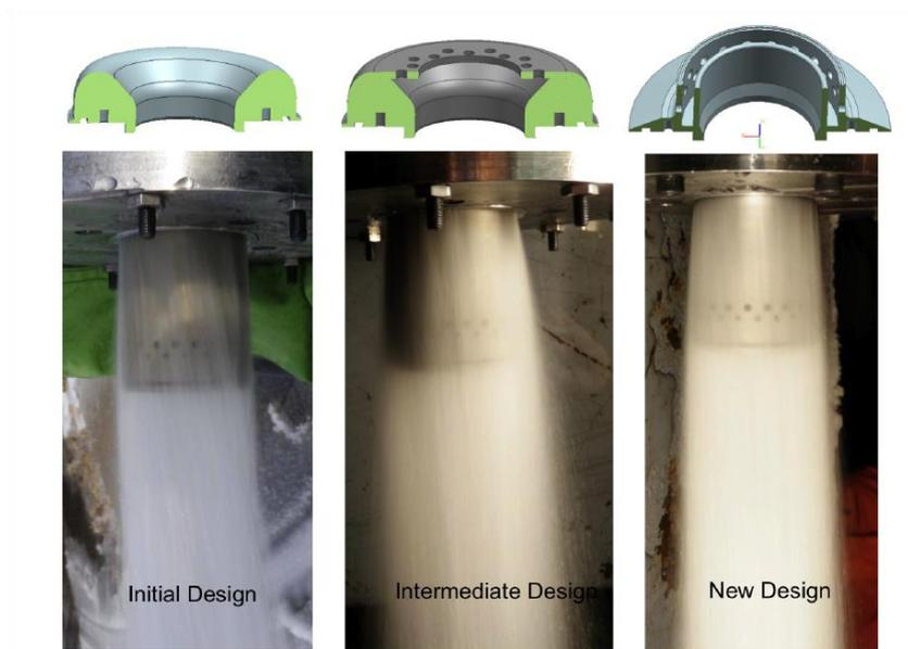
Figure 1.15. Uniformity of the Jet Introduced by Bedard [8]
