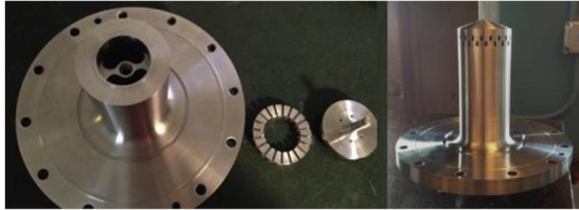
Figure 1.14 Components of Pintle Injector Designed by Badard et al [8]
