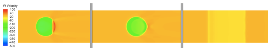
Figure 1.24 Comparison of Velocity Contours in the Vicinity of Bleed Hole for P/P_{\infty}=0.254 [48]
