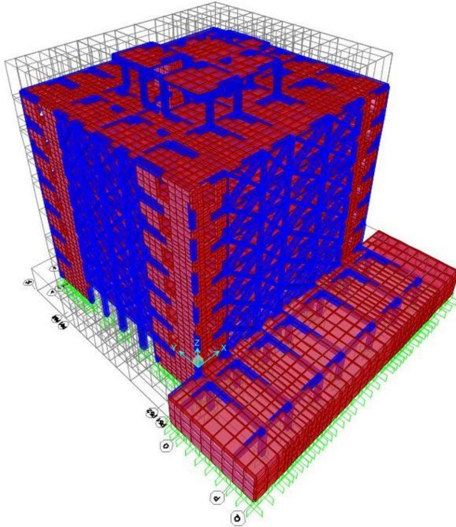
*Figure 4.15.* Finite element model with strut members
