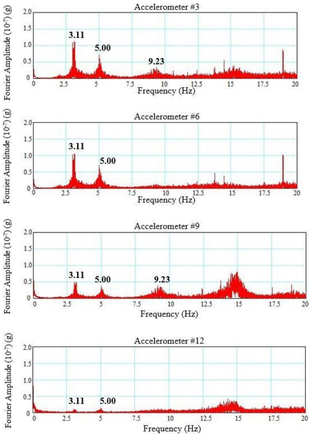
Figure 4.3. Fourier amplitude spectra for the NS direction
