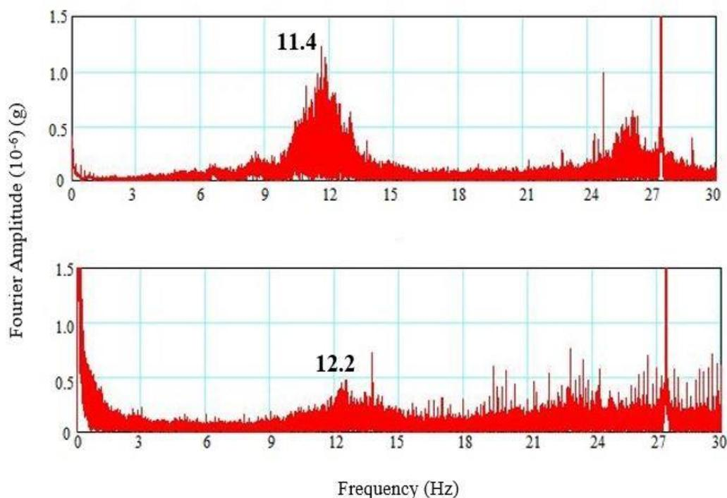
Figure 5.6. Floor frequency for the ground and second floors
