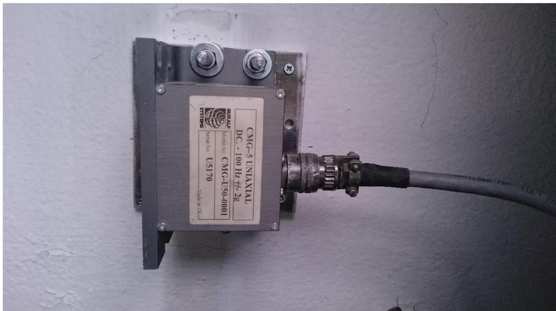
Figure 3.5. Uniaxial accelerometer
