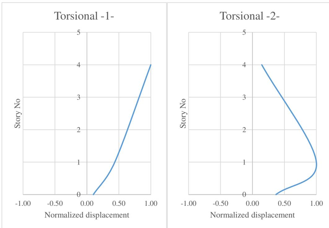
Figure 4.7. The first and second torsional mode shapes
