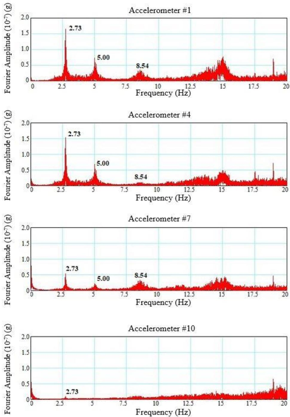
Figure 4.2. Fourier amplitude spectra for the EW direction
