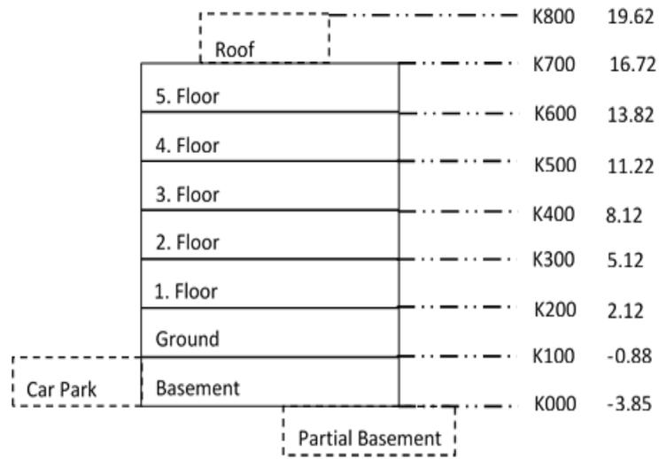
Figure 3.2. Floor labels and elevations (in m)
