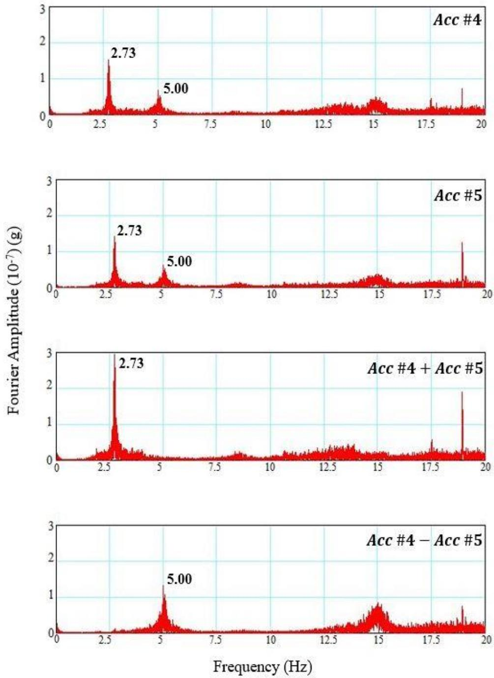
Figure 4.4. Fourier amplitude spectra for two parallel accelerometers
