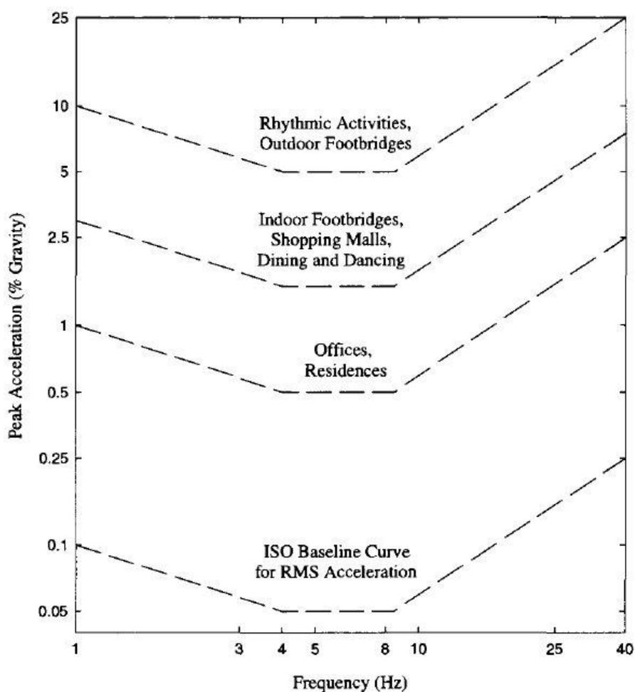
Figure 2.2. Recommended peak acceleration for human tolerance (ISO 2631-2)
