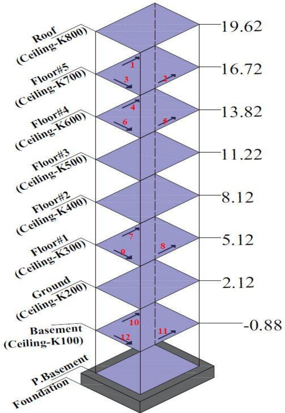
Figure 3.7. Instrumentation scheme for the horizontal direction
