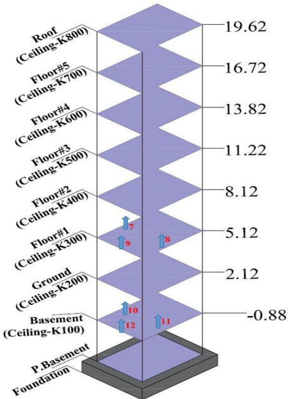
Figure 3.8. Instrumentation scheme for the vertical direction
