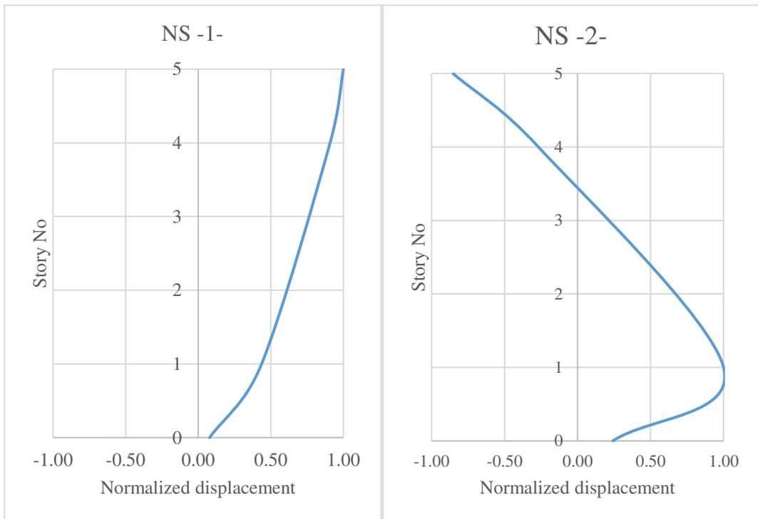
Figure 4.6. The first and second translational mode shapes for the NS direction
