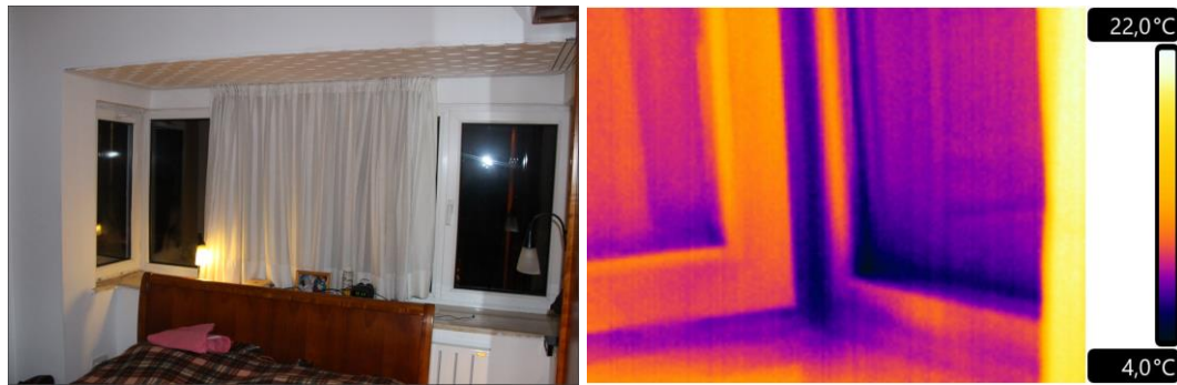
Figure 4.8. The window frames, especially the edges where window frame and building wall come together are the coldest zones with surface temperatures 15°C colder than the indoor air temperature. That temperature difference signals the risk of condensation and air tightness problems occurring at the coldest zones ( T_{in} = 19.5^{\circ}\text{C} , RH= 45%).
