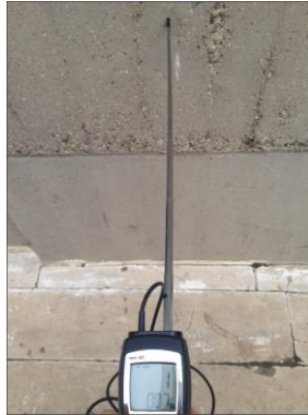
Figure 2.6. Using handheld anemometer to measure wind velocity near wall surface
