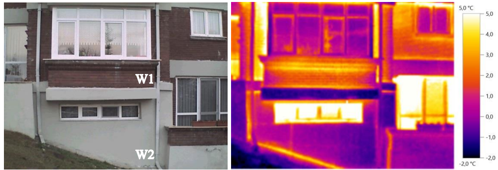
Figure 4.9. Surface temperature of W2 being close to the outside air temperature shows the improvement in thermal resistance while being still 1-2°C higher than the outside air temperature ( T_{\text{out}} = -3.1^{\circ}\text{C} , RH= 65%).
