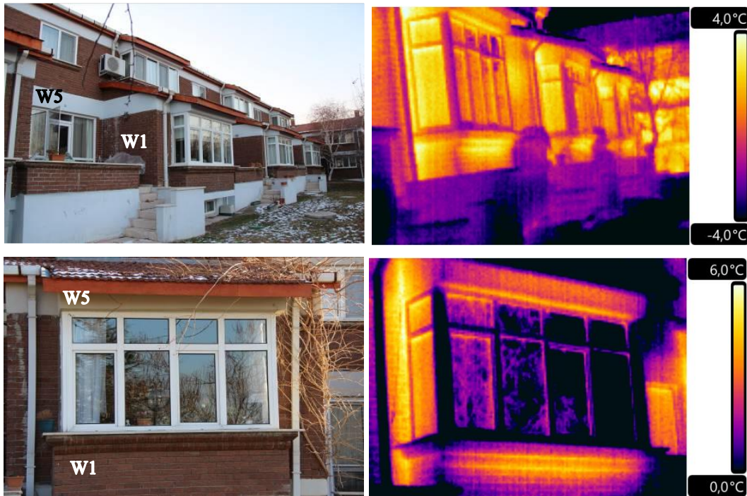
Figure 4.4. The warm edges reaching 6°C difference higher than the outside air temperature exhibit the significant heat loss through the edges where the window frames come together with the structure. The warmer surfaces of the uninsulated reinforced concrete beam (W5) and the insulated cavity brick wall (W1) where the radiator is positioned behind the parapet signal the inadequate thermal resistance of those walls ( T_{out} = 0.3^{\circ}\text{C} , RH= 60%).
