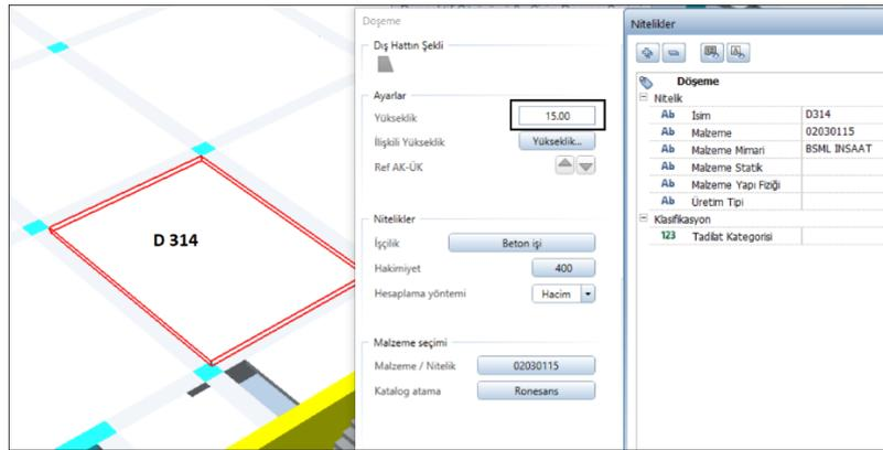
Figure 4.12. Incorrect Floor Thickness in Allplan Model
