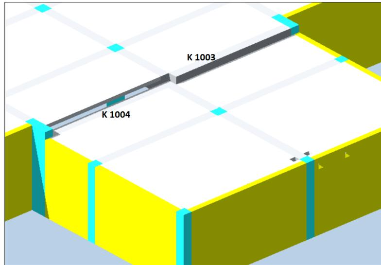
*Figure 4.13. Incorrect Floor Level in Allplan Model*
