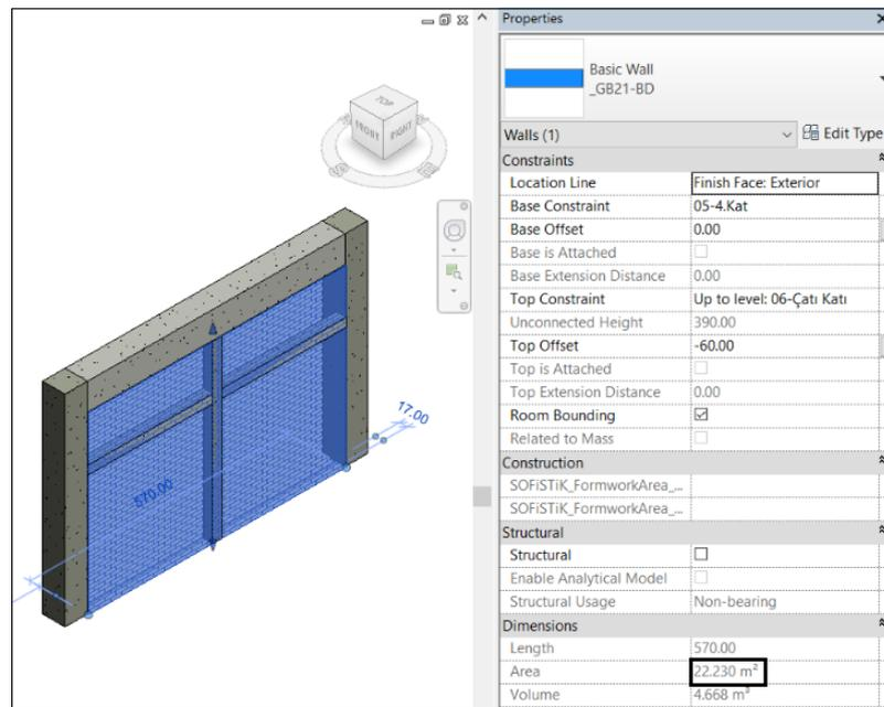
Figure 3.9. Area of an Architectural Wall (before Using Join Feature of Revit)
