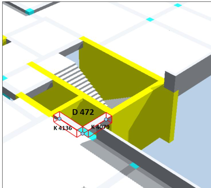
Figure 4.7. Missing Floor in Allplan Model
