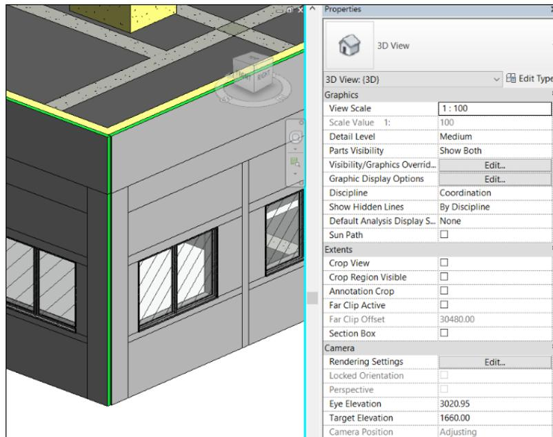
Figure 3.19. An Improper Joint of Insulation Elements in 3D Plan (after Join Command)
