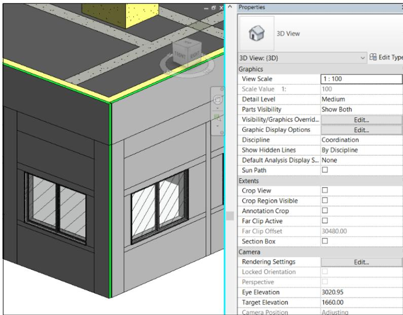
Figure 3.17. An Improper Joint of Insulation Elements in 3D Plan
