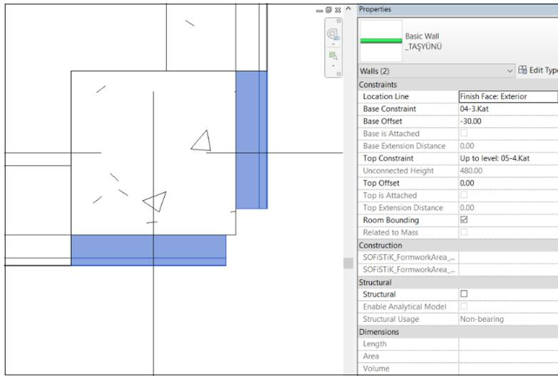
Figure 3.21. Elements after Deleting Split Sections in 2D Plan
