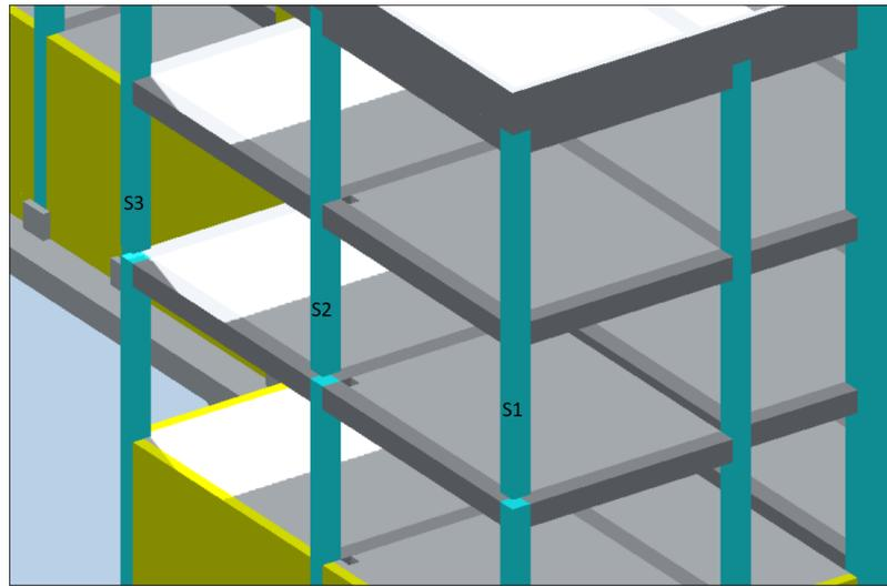
*Figure 4.2. Modeling Mistake in the Height of the Columns in Allplan Model*
