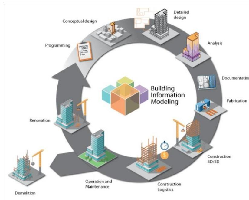
Figure 2.2. Usage of BIM throughout the Lifecycle of a Building
