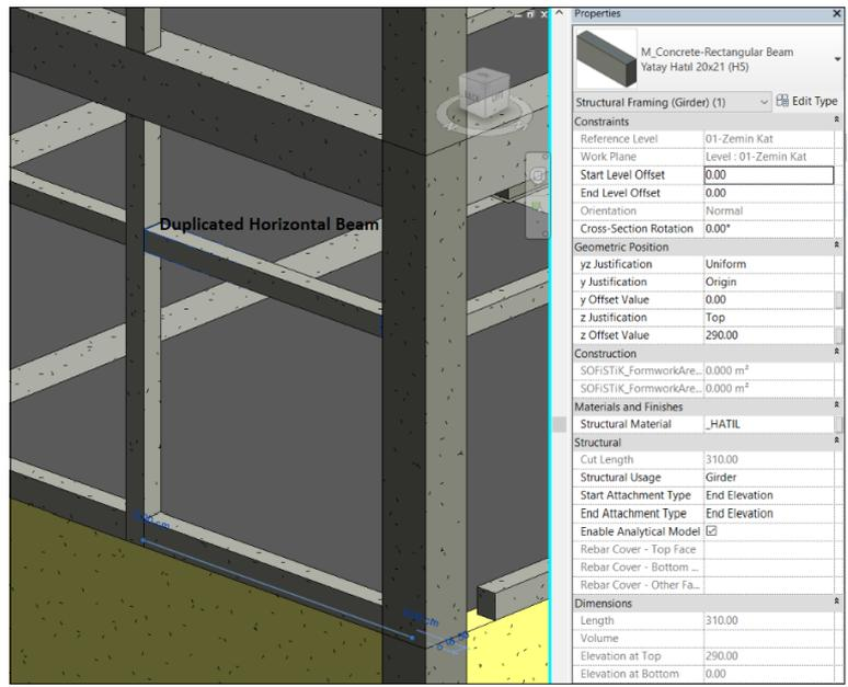
Figure 4.21. Duplicated Horizontal Beam in Revit Model
