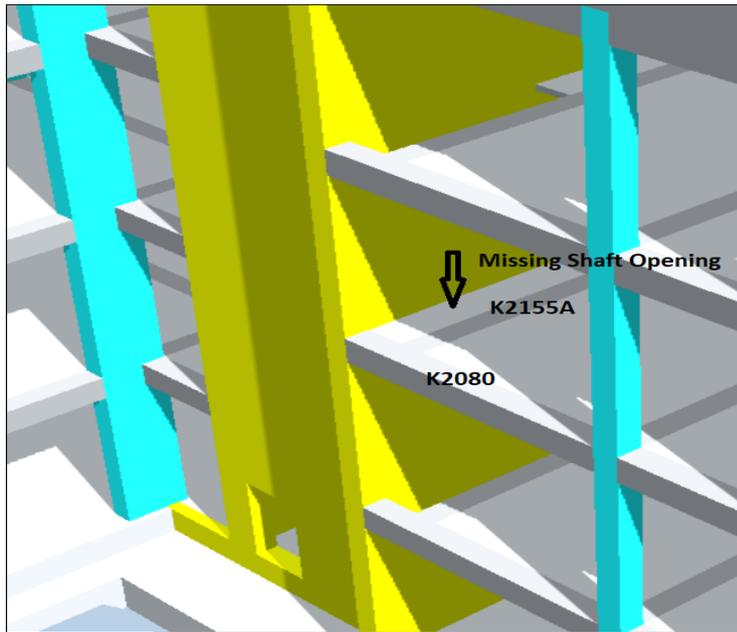
Figure 4.6. Missing Shaft Opening in Allplan Model
