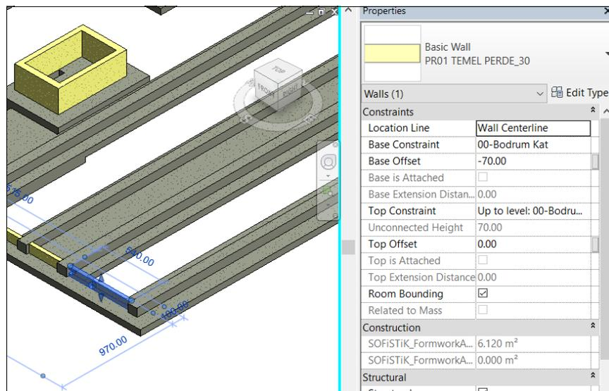
Figure 3.2. Vertical opening in Foundation Walls
