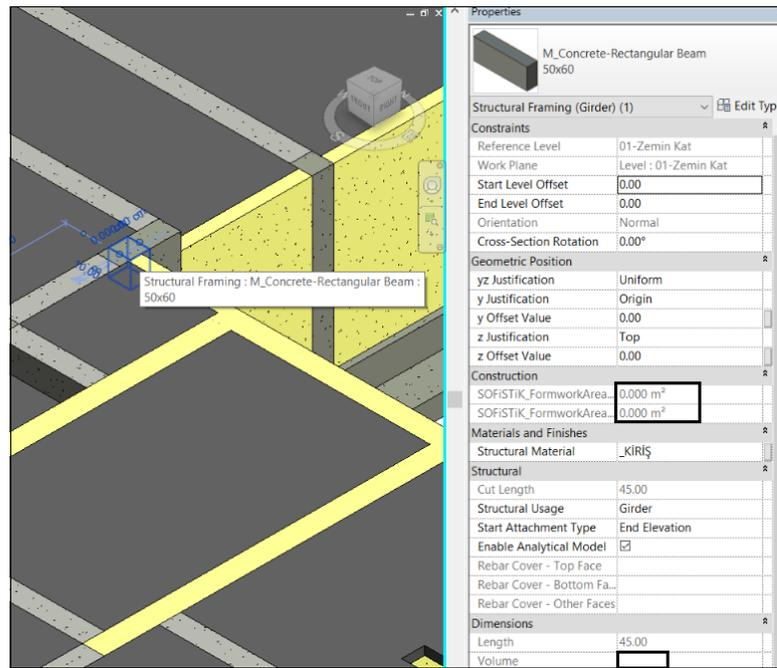
Figure 3.5. A Beam in Column Having No Volume and No Formwork Area
