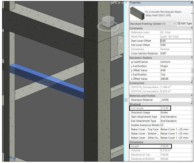
Figure 4.22. Beam having Unequal Length and Cut Length
