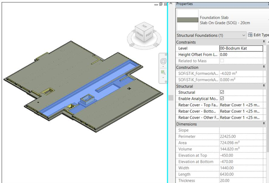
Figure 4.1. Foundation with Slab on Grade
