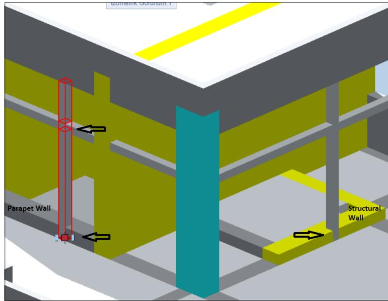
Figure 4.19. Incorrect Level of Vertical Beams and Improper Joint of Beams in Allplan Model
