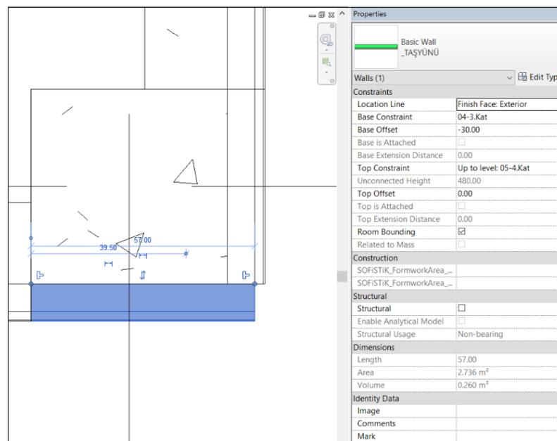
Figure 3.16. An Improper Joint of Insulation Elements in 2D Plan
