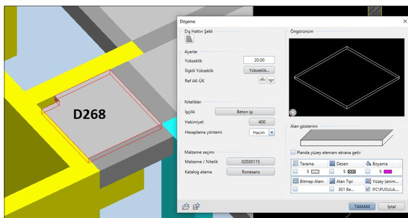
Figure 4.16. Incorrect Floor Thickness in D268 Floor in Allplan Model
