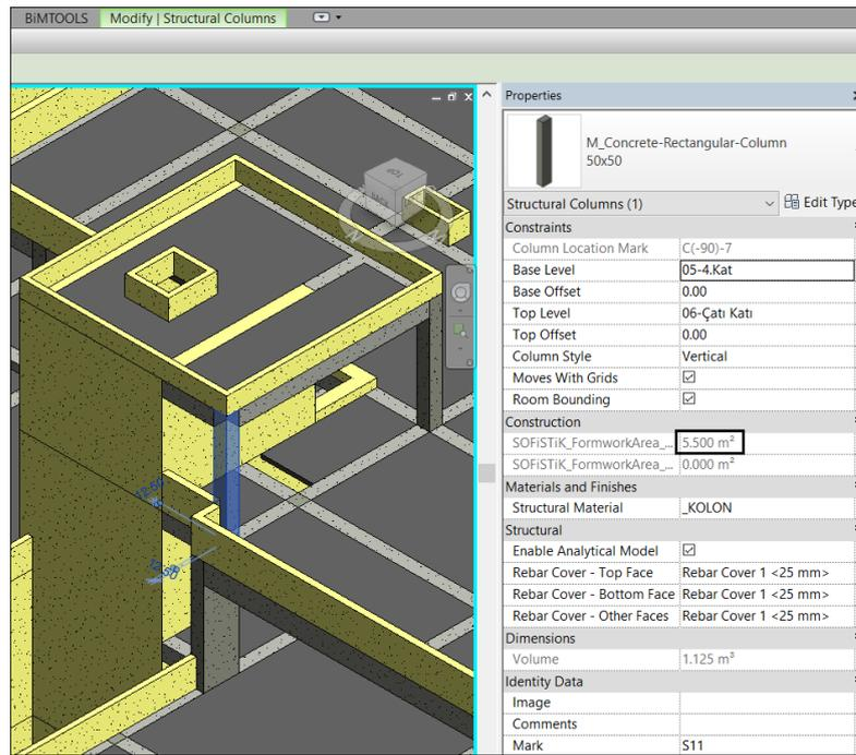
Figure 4.4. Incorrect Formwork Area of S11 Column in Revit Model
