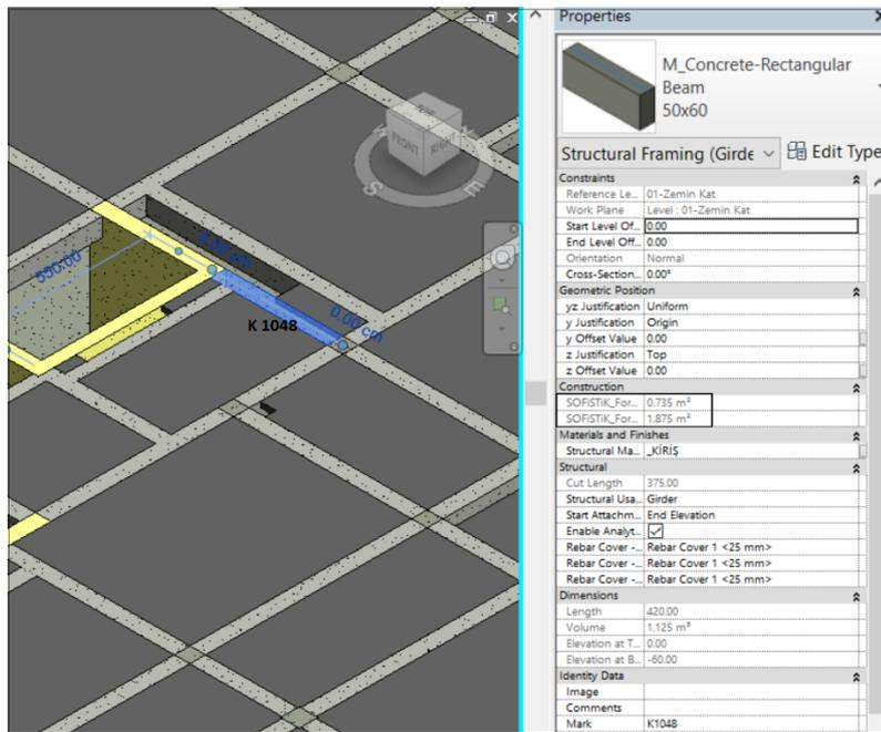
Figure 4.14. Beam Having Shaft Opening at One Side in Revit Model
