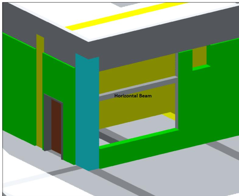
Figure 4.20. Incorrect Length of Horizontal Beam in Allplan Model
