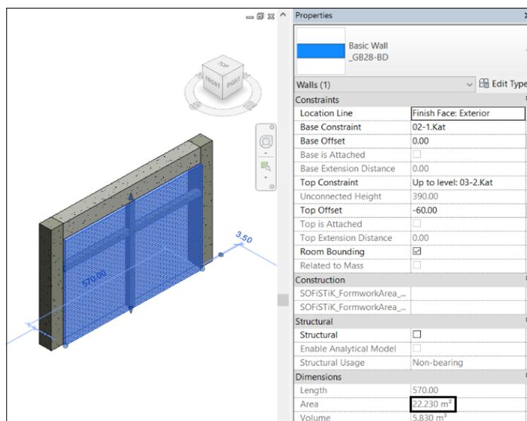
Figure 3.11. Area of an Architectural Wall (Exterior Face not Aligned with Structural Frame - before Using Join Feature of Revit)
