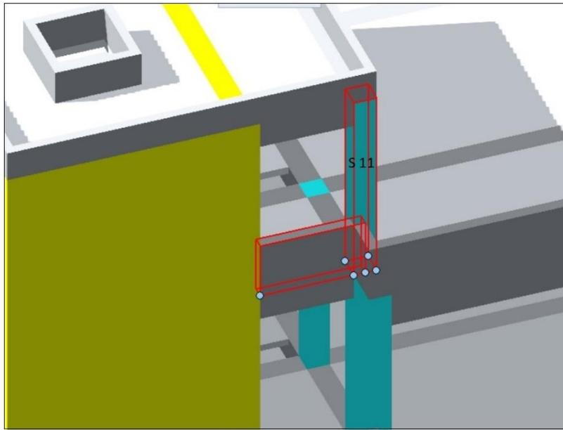
*Figure 4.3. Modeling Mistake in Joint of Column and Parapet Wall in Allplan Model*
