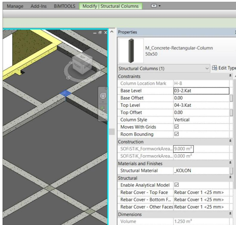
Figure 4.5. Incorrect Formwork Area of S65 Column in Revit Model
