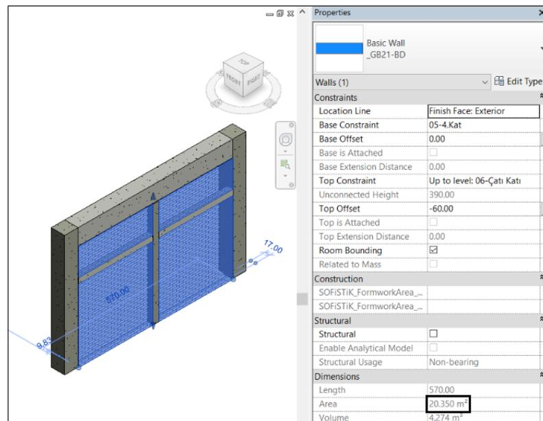
Figure 3.10. Area of an Architectural Wall (after Using Join Feature of Revit)
