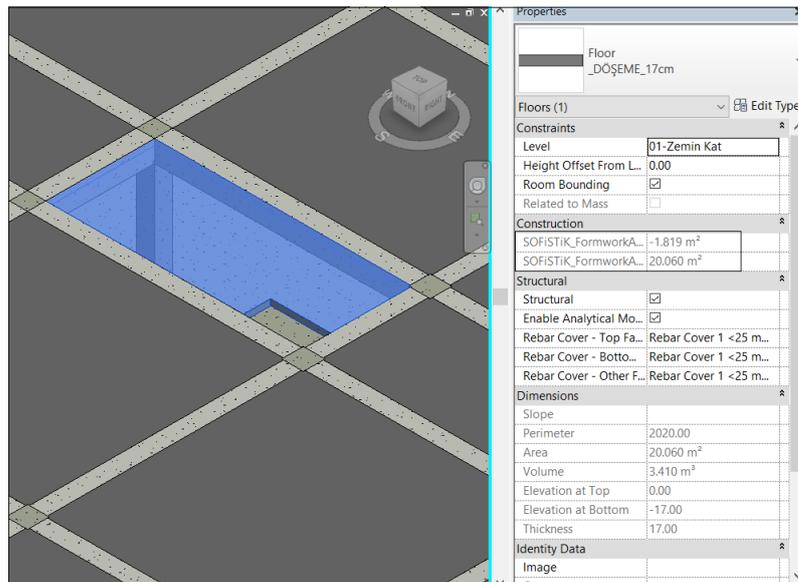
Figure 4.17. Incorrect Formwork Area of D138 Floor Having Shaft Opening in Revit Model
