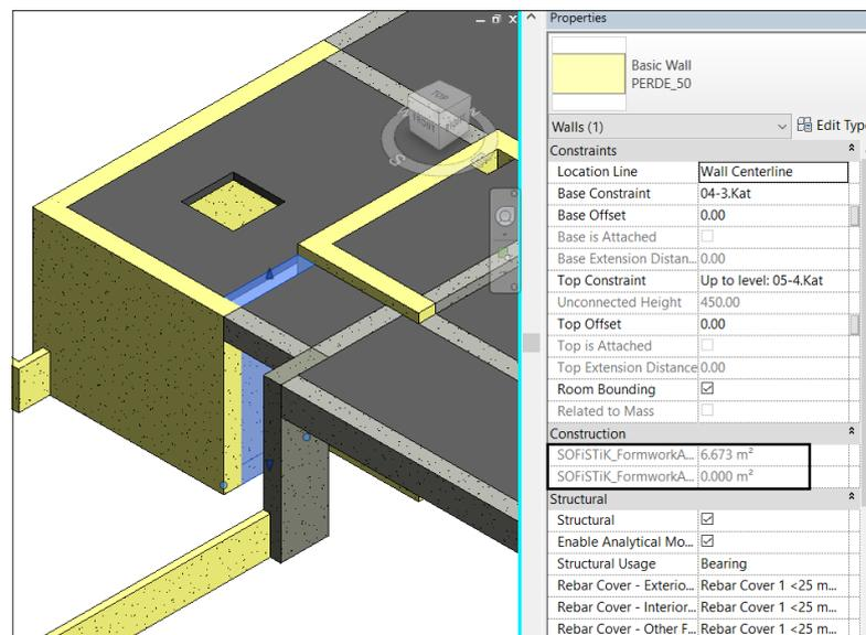
Figure 4.8. Miscalculated Formwork Area of Structural Wall in Revit Model
