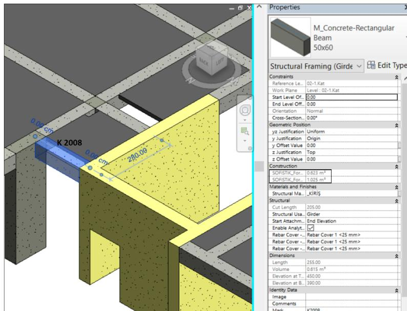
Figure 4.15. Beam Joining with Structural Wall in Revit Model
