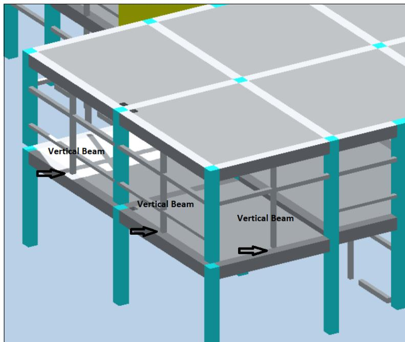
*Figure 4.18. Incorrect Height of Vertical Beams in Allplan Model*
