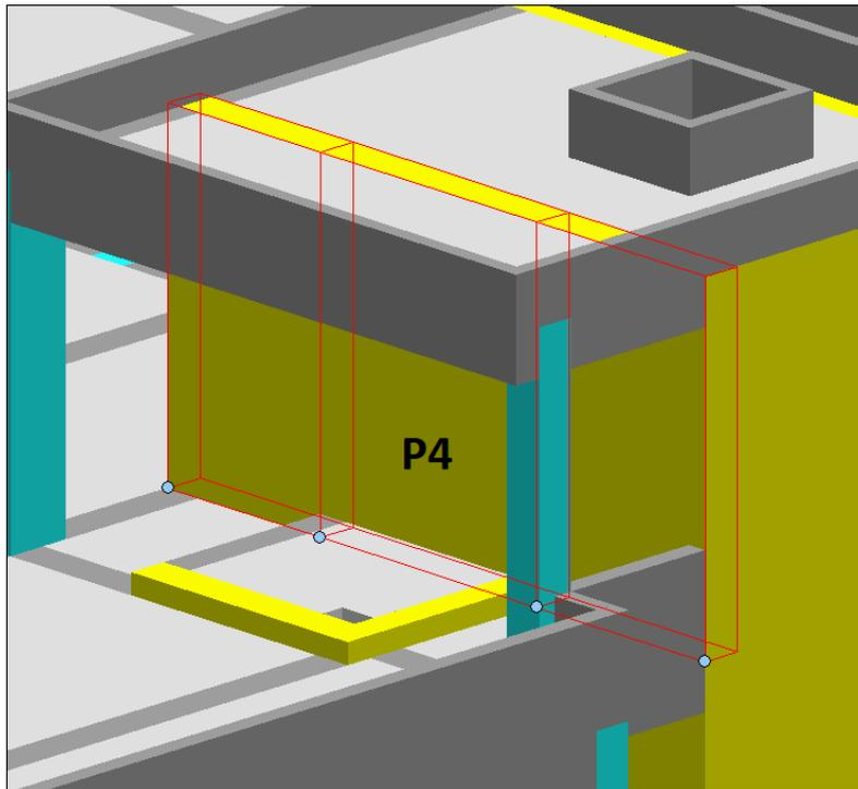
*Figure 4.11. Incorrect Level of Structural Wall in Allplan Model*
