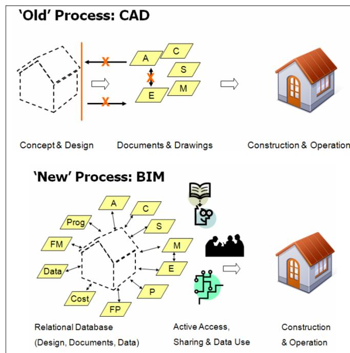
Figure 2.3. Comparison between Conventional CAD and New BIM Approach
