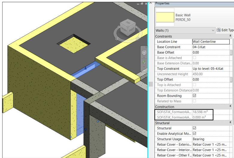
Figure 4.9. Corrected Formwork Area of Structural Wall in Revit Model
