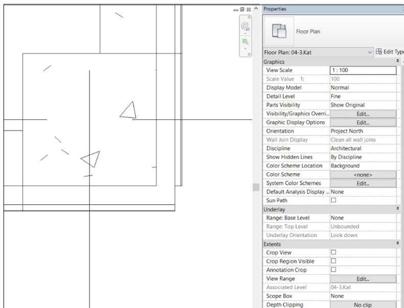
Figure 3.18. An Improper Joint of Insulation Elements in 2D Plan (after Join Command)
