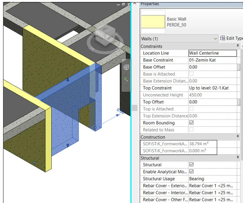
Figure 4.10. Miscalculated Formwork Area of Structural Wall in Revit Model
