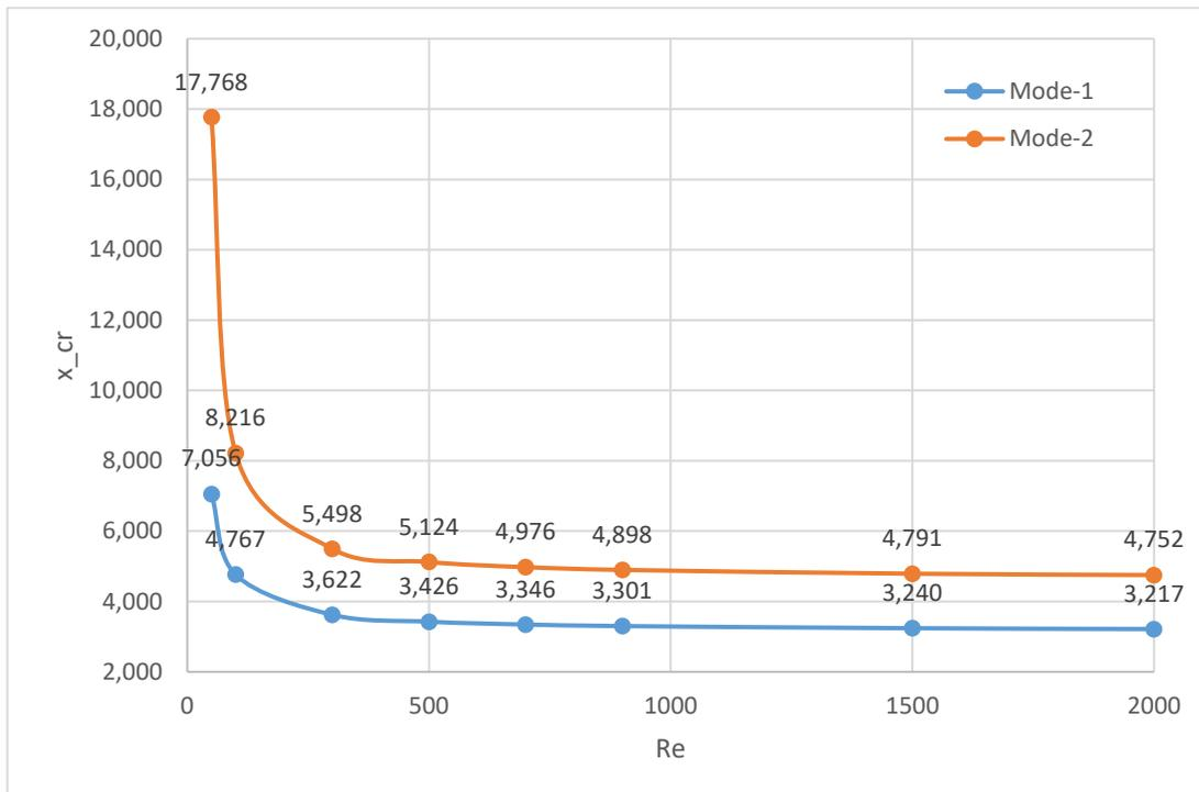
Figure 2.27. Change of the Tip of The Neutral Curve with Reynolds Number
