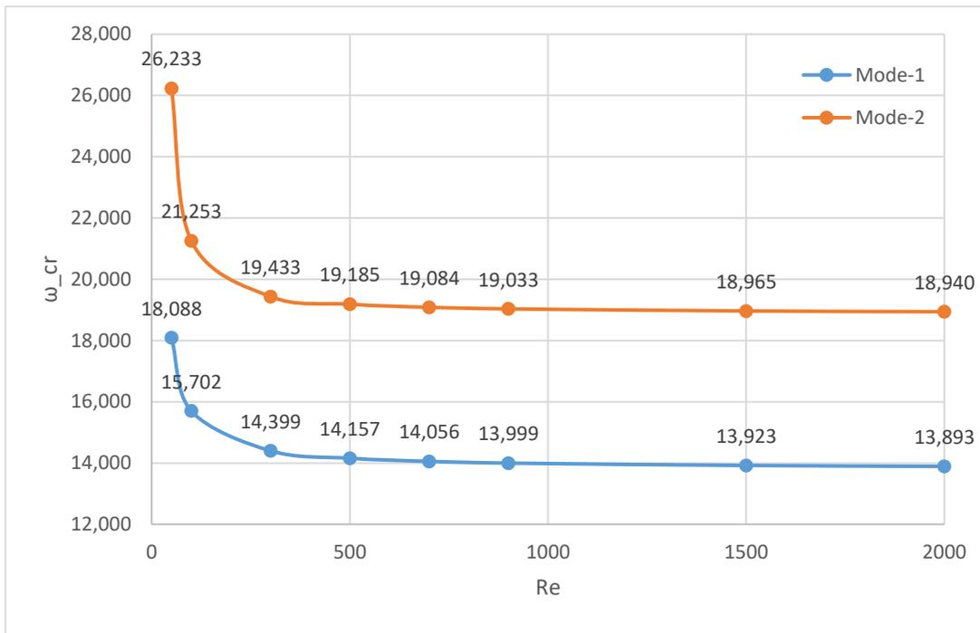
Figure 2.29. Change of the Critical Disturbance Frequency with Reynolds Number
