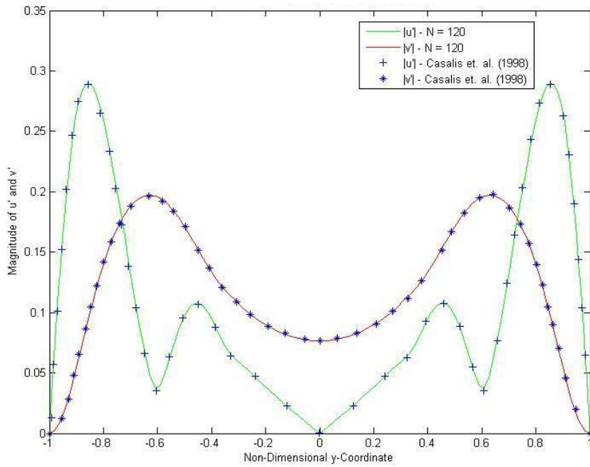
Figure 2.13. Magnitude of Perturbation Velocity Components,  $Re = 900, x = 10, \omega = 30$  – Mode-1
