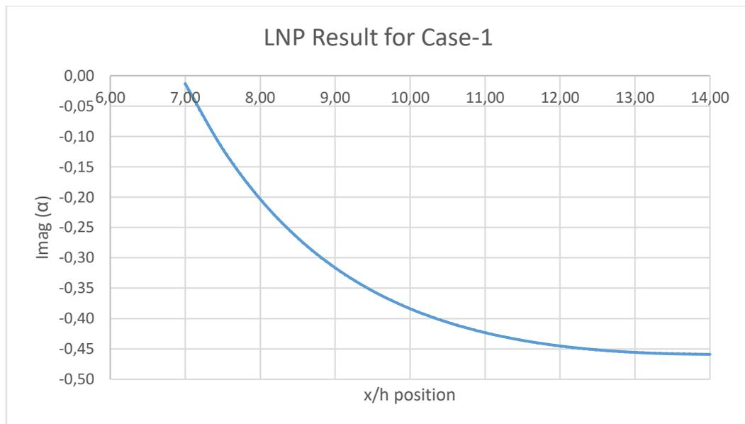
Figure 3.4. Change of Imaginary Part of Complex Wavenumber for Case-1
