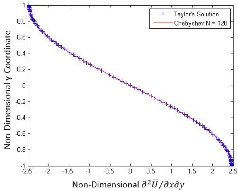
Figure 2.8.  $\partial^2 \bar{U}^* / \partial x^* \partial y^*$  Comparison (Independent of x-Direction)
