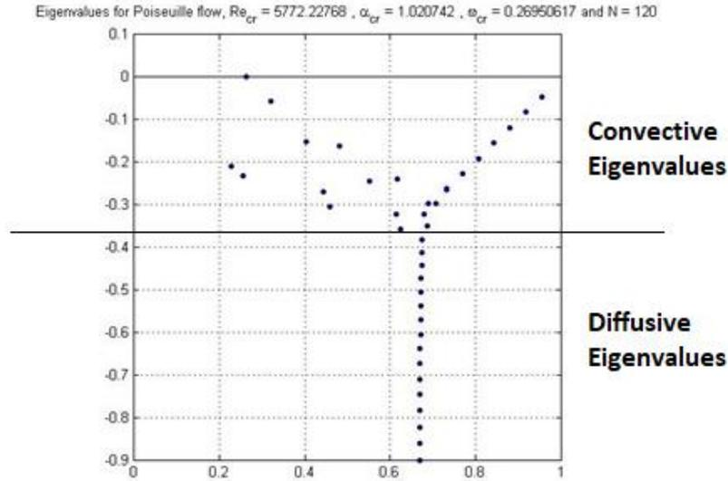
Figure 2.10. Temporal Stability Spectrum for Plane Poiseuille Flow at Critical Conditions  $Re_c$  and  $\alpha_c$
