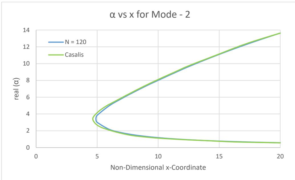
Figure 2.19. Comparison Of The Neutral Curves For Wavenumber – Mode-2
