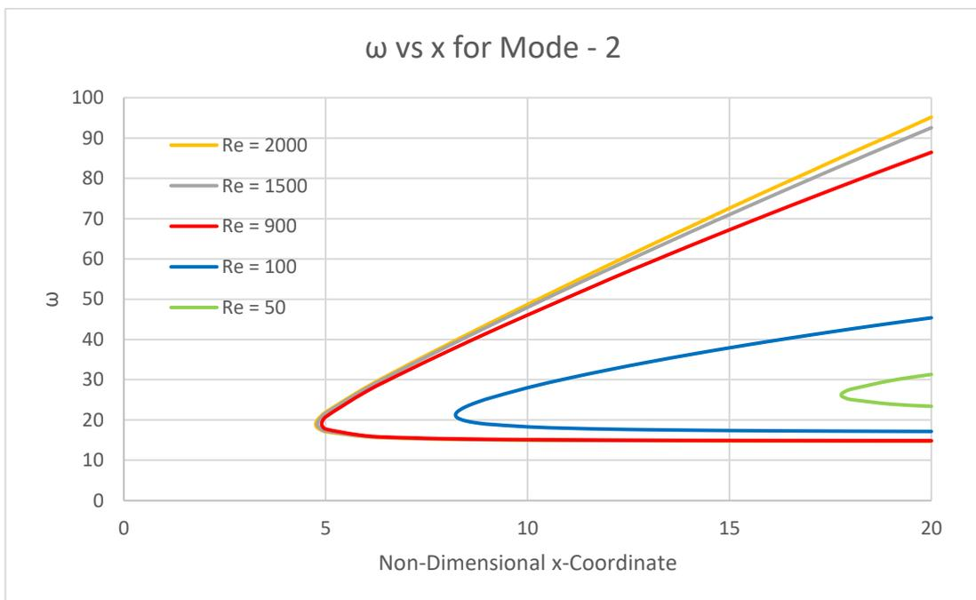
Figure 2.24. Natural Curves of Disturbance Frequency for Different Reynolds Numbers – Mode-2
