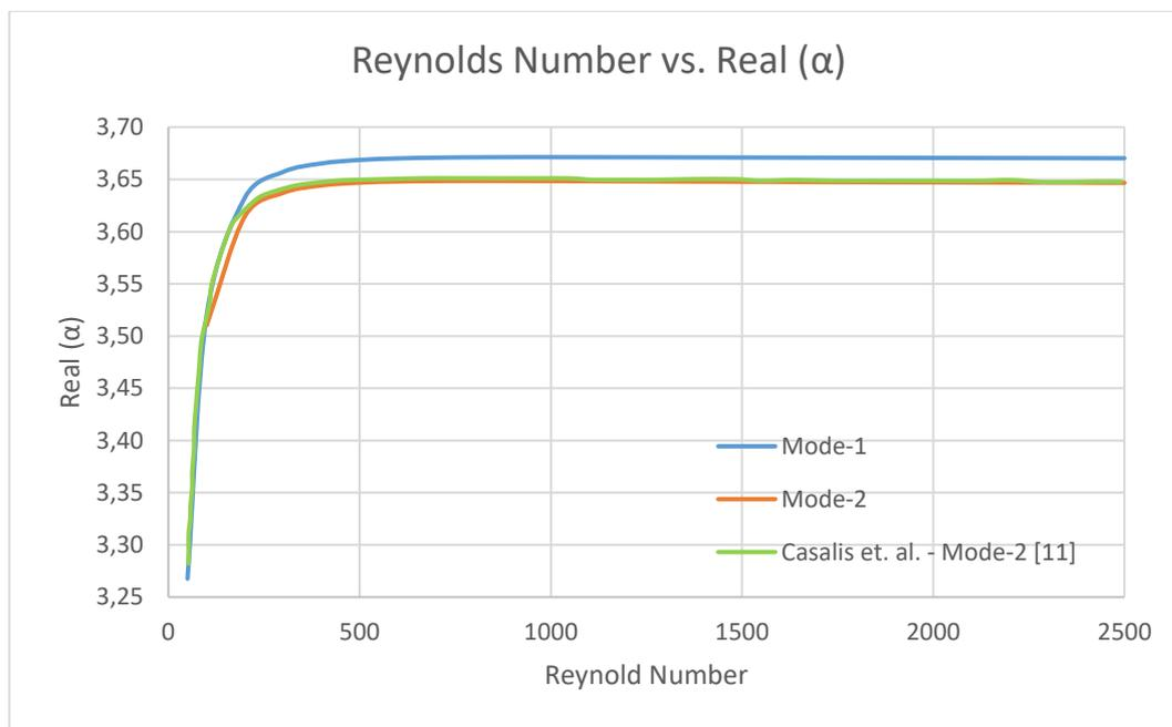
Figure 2.25. Change of Real Part of Complex Wavenumber
