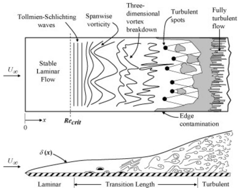
Figure 1.5. Laminar to Turbulent Transition in Boundary Layer [21]
