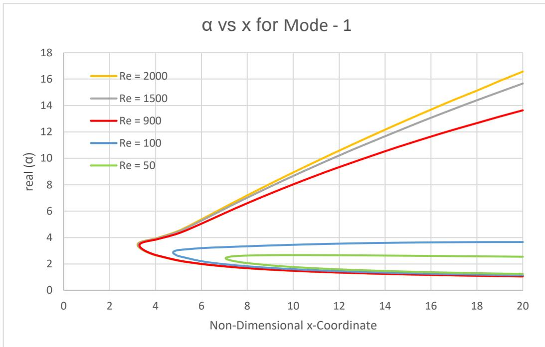
Figure 2.21. Neutral Curves of Wavenumber for Different Reynolds Numbers – Mode-1
