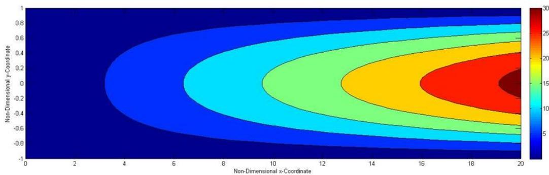
Figure 2.4. Mean Velocity Magnitude Contours for  $L/h = 20$
