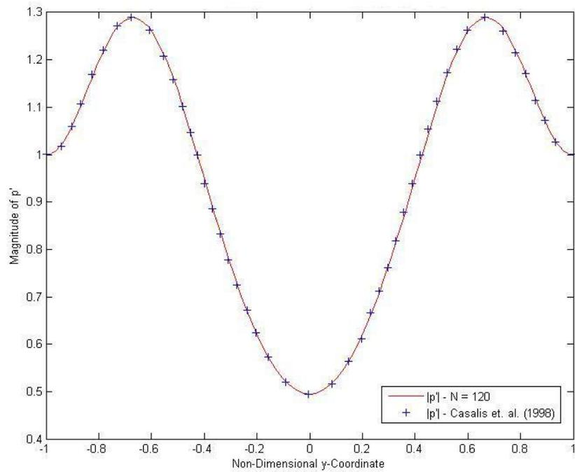
Figure 2.16. Magnitude of Perturbation Pressure for  $Re = 900, x = 10, \omega = 30$  – Mode-2
