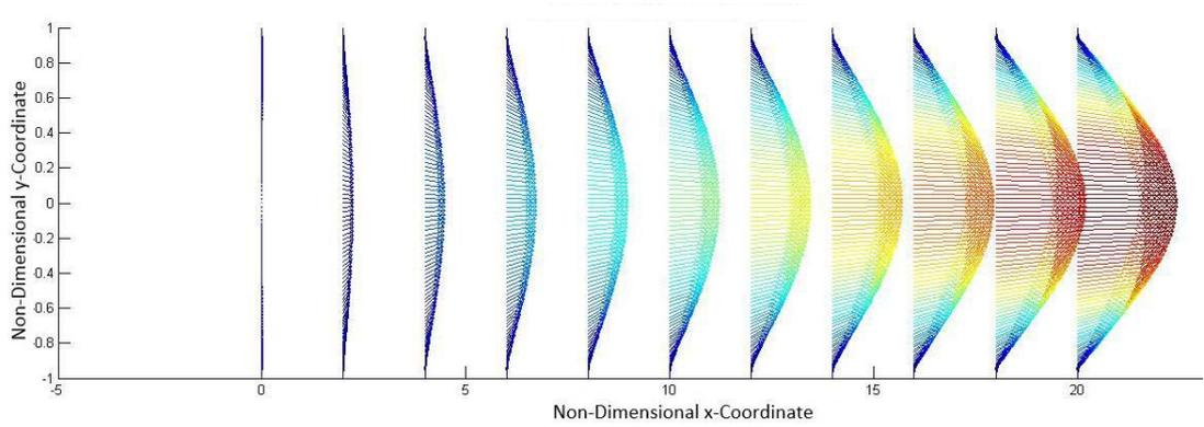
Figure 2.5. Mean Velocity Vectors for  $L/h = 20$
