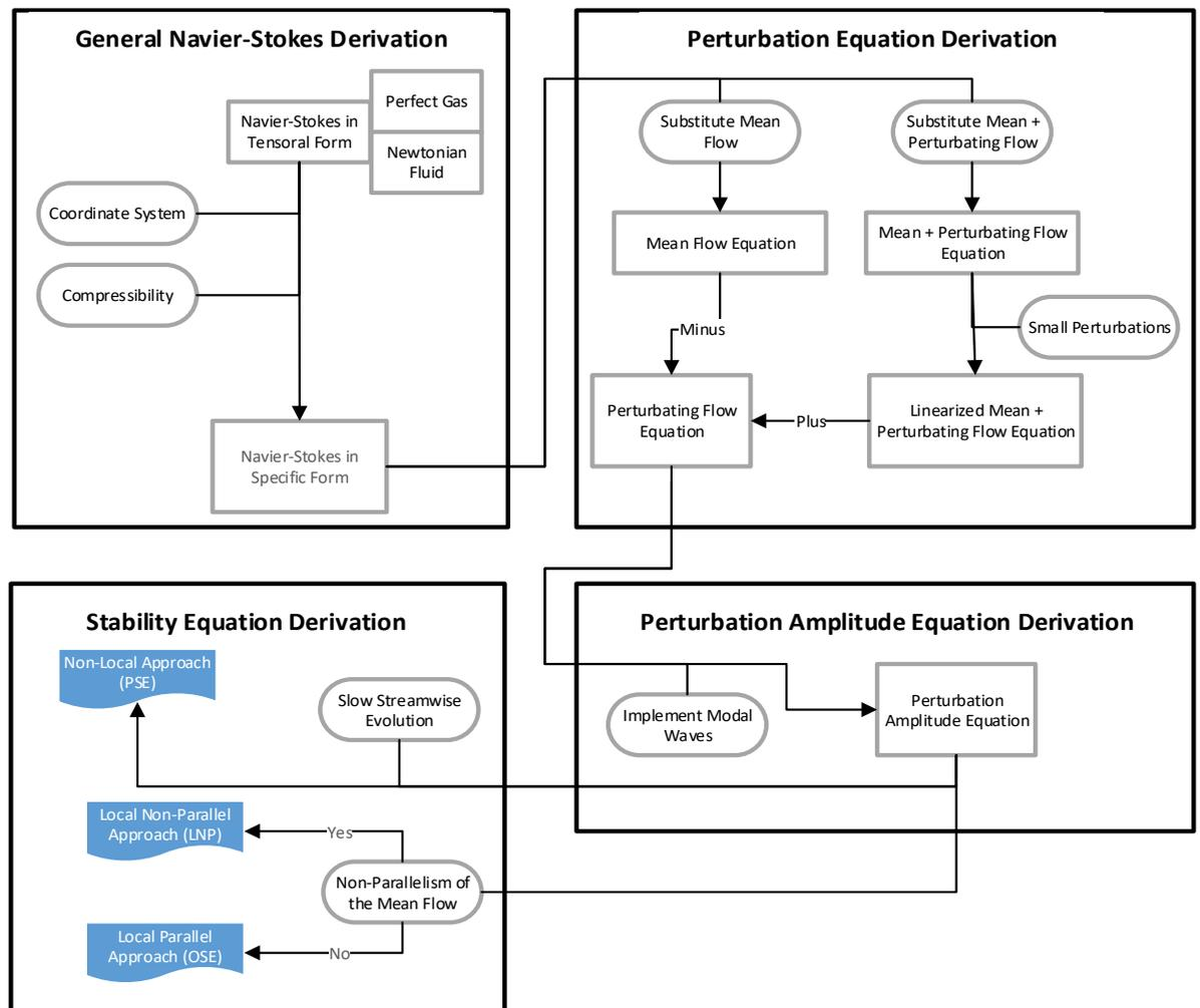
Figure 2.2. Block Diagram of the Derivation of Stability Equations
