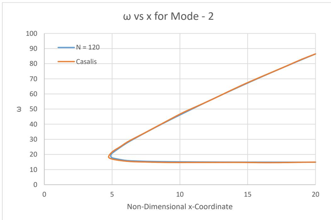
Figure 2.20. Comparison Of The Neutral Curves For Disturbance Frequency – Mode-2
