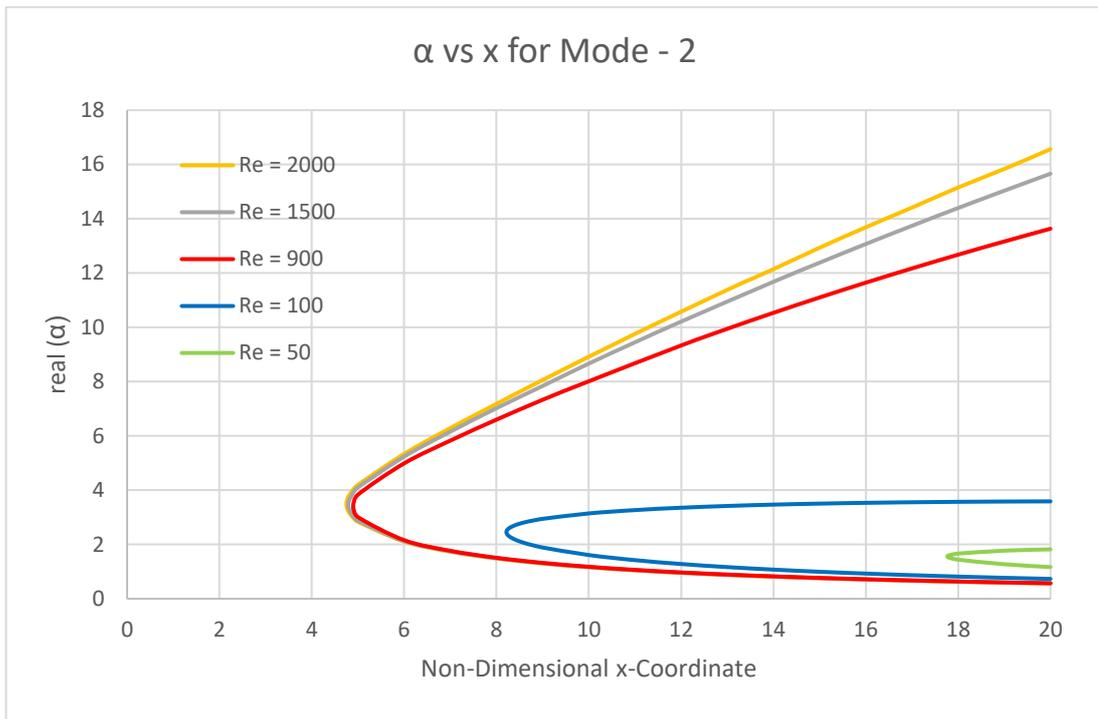
Figure 2.23. Natural Curves of Wavenumber for Different Reynolds Numbers – Mode-2
