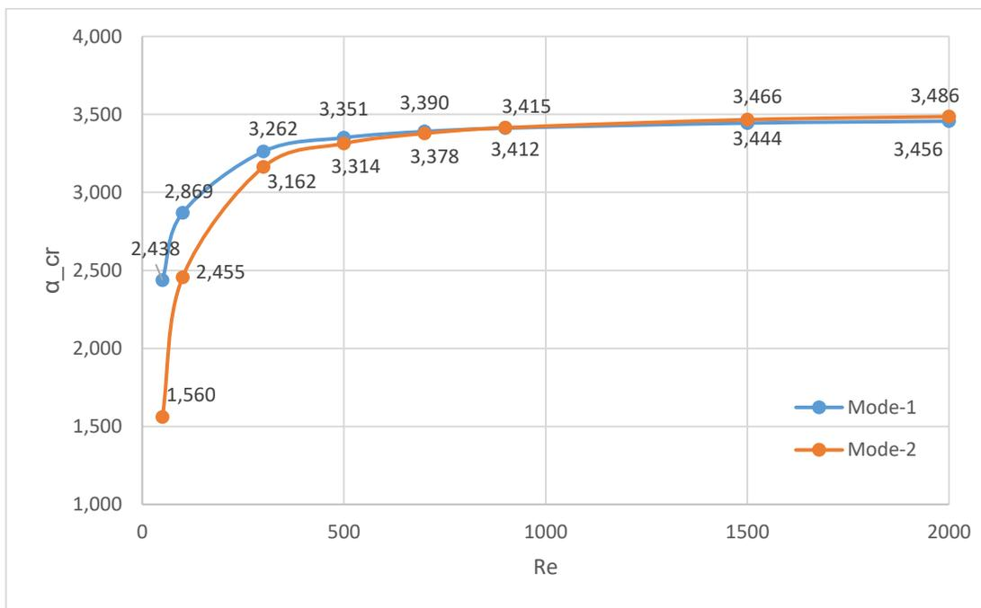
Figure 2.28. Change of the Critical Wavenumber with Reynolds Number
