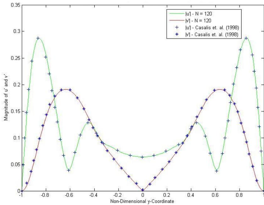
Figure 2.14. Magnitude of Perturbation Velocity Components,  $Re = 900, x = 10, \omega = 30$  – Mode-2
