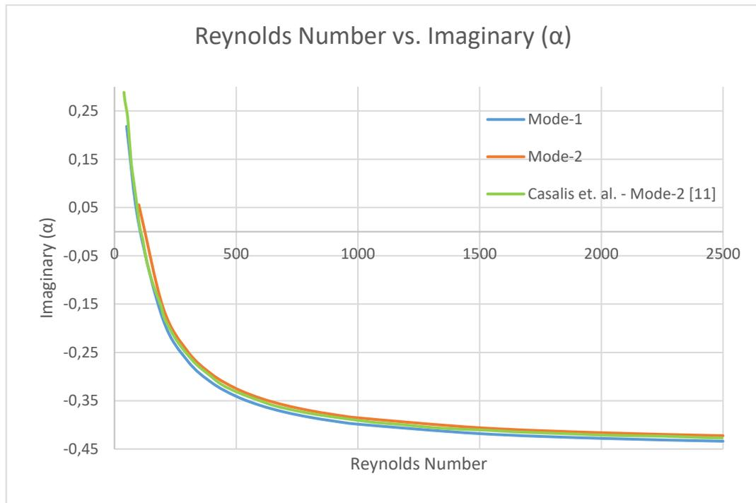
Figure 2.26. Change of Imaginary Part of Complex Wavenumber
