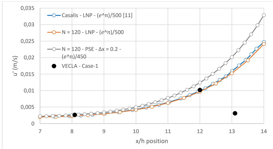
Figure 3.5. Fluctuating Streamwise Velocity – Case-1
