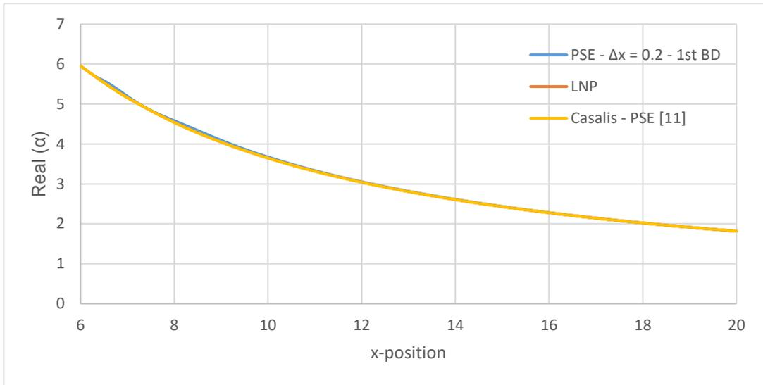
Figure 3.1. Change of Real Part of Wavenumber Along x
