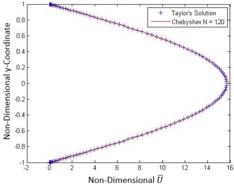
Figure 2.6.  $\bar{U}^*$  Comparison at  $x/h = 10$
