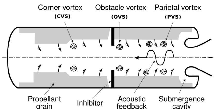
Figure 1.1. Vortex-Shedding – Acoustic Wave Interaction [4]
