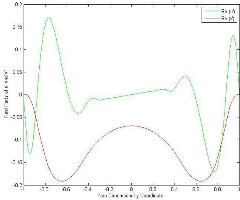
Figure 2.11. Real Parts of Perturbing Velocity Components for  $Re = 900, x = 10, \omega = 30$  – Mode-1
