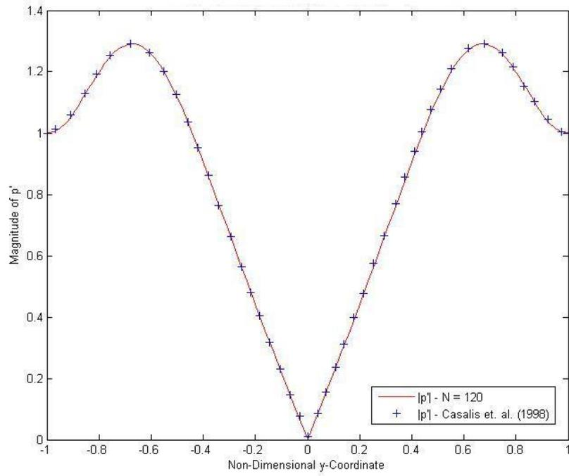
Figure 2.15. Magnitude of Perturbation Pressure for  $Re = 900, x = 10, \omega = 30$  – Mode-1
