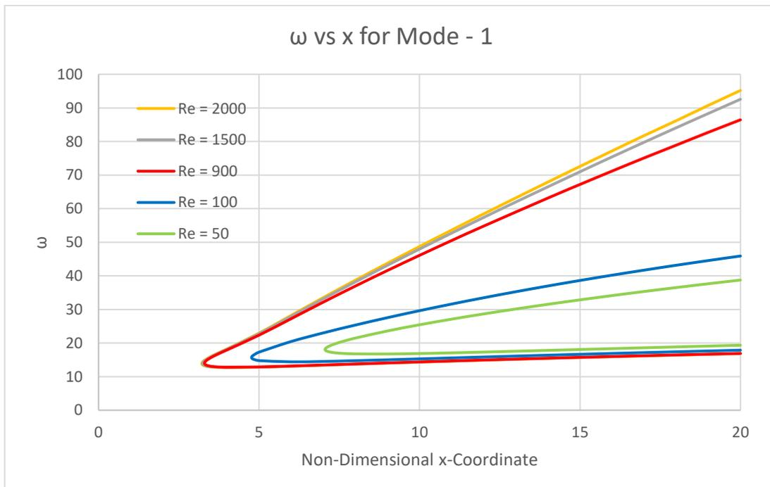
Figure 2.22. Natural Curves of Disturbance Frequency for Different Reynolds Numbers – Mode-1
