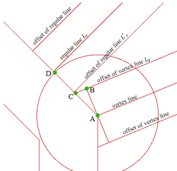
Figure 4.20: A safety distance equal to a regular line's offset distance is added to the barring circle to avoid overlapping of offset areas.
