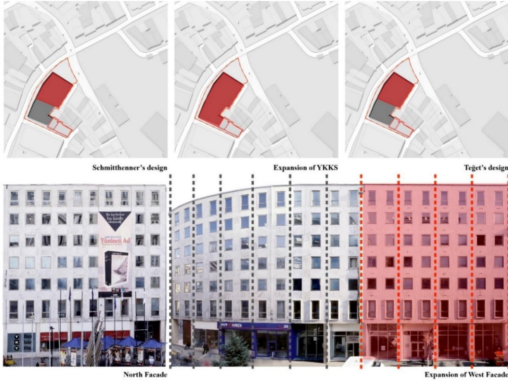
Figure 2.9. Expansion of the Yapı Kredi Building with the adjacent building.
