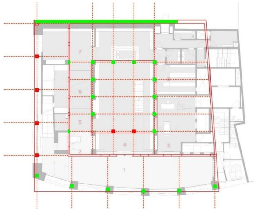
Figure 3.7. The superimposition of the old Yapı Kredi Bank's and YKKS building's structures.
