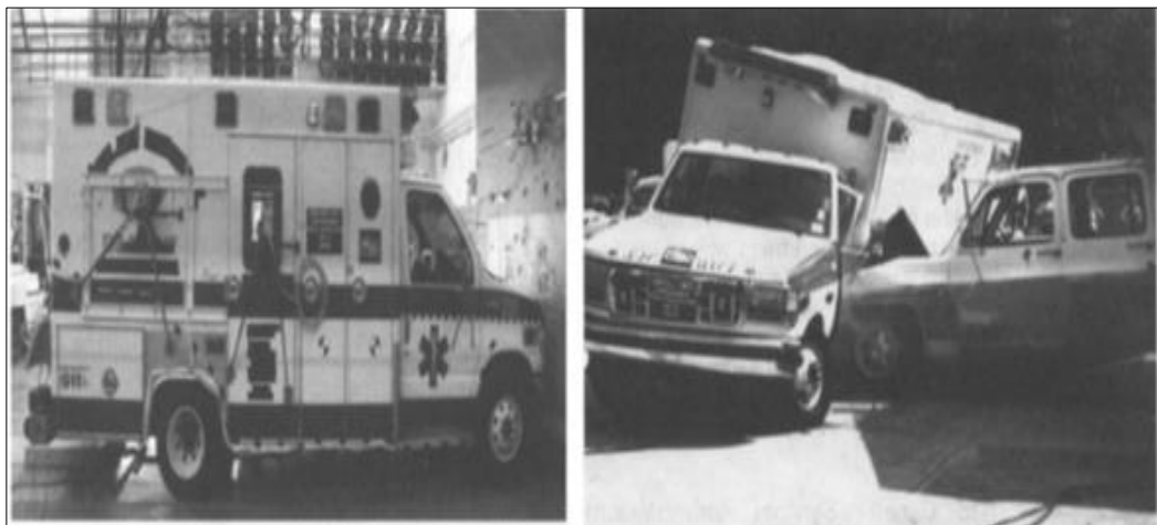
Figure 2.7. Fixed barrier front-impact test and side-impact test [18]
