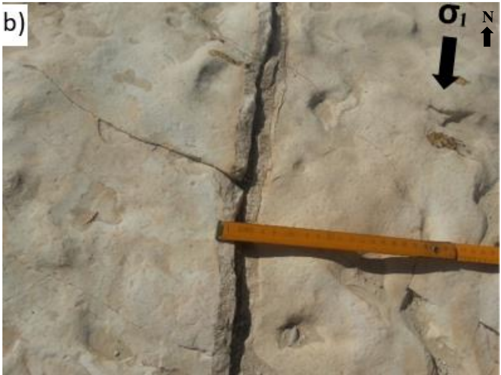
Figure 2.11. Field views from tension joints taken from the structural station located at the back limb of the Gemrik Anticline where the wall damage zone of the Bozova Fault is distant: (a) A view illustration how joint survey was performed in the field. The extended, foldable wooden ruler, which is one meter long, is placed perpendicular to the strikes of the tension joints and average density is 4 to 5 joints per meter; (b) a close-up view from 3-cm-width calcite filled vein.
