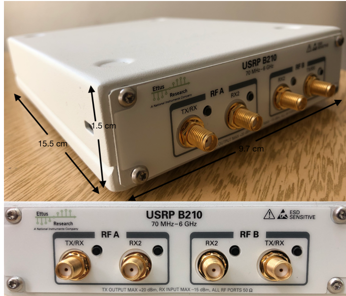
Figure 2.2: The USRP B210 with steel kit. There are one transmit and one receive channel on " RF A " and another transmit and receive channels on " RF B ".
