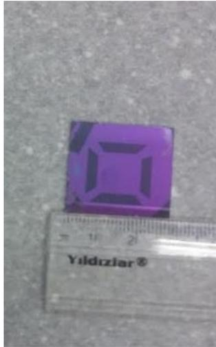
Figure 4.24. Picture of undoped and shaped Si layer on SOI wafer
