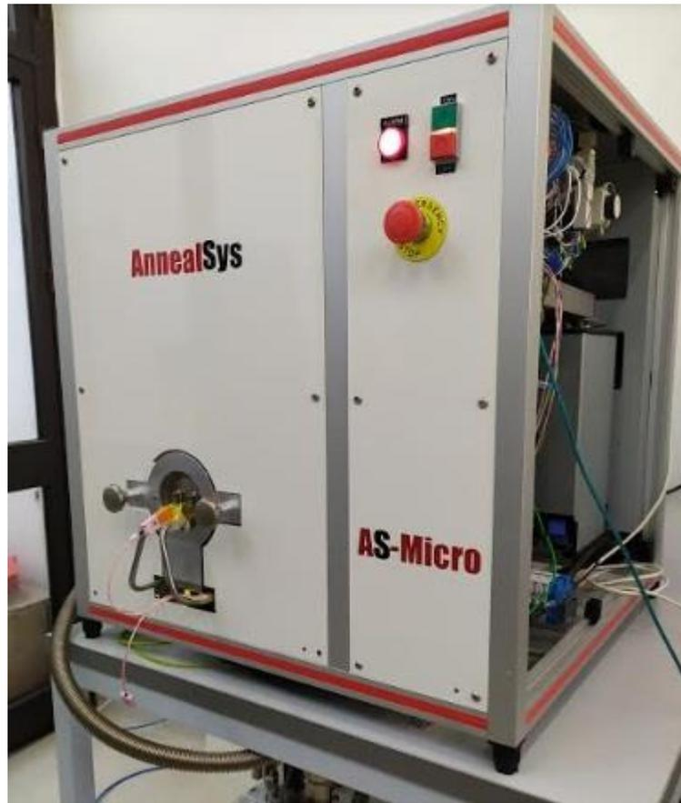
*Figure 3.4.* Picture of RTA oven in GUNAM
