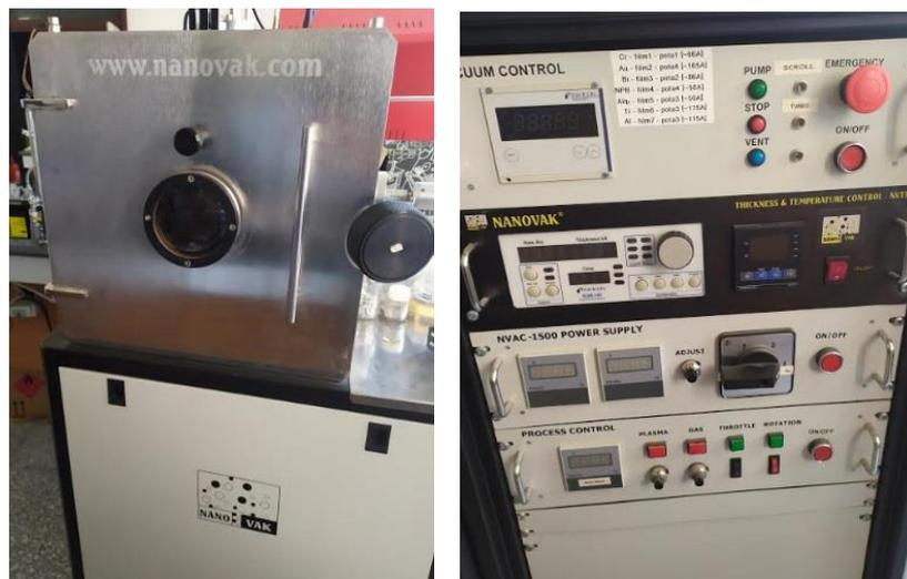
Figure 3.7. Picture of Nanovak thermal evaporation system in SPMG laboratory
