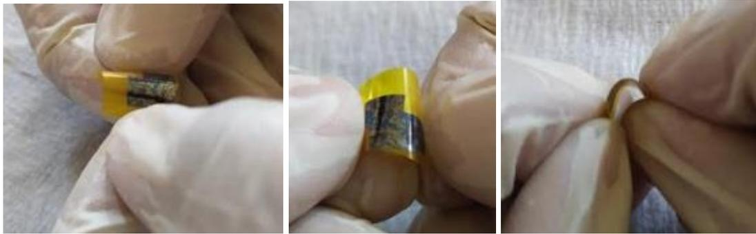
*Figure 4.37.* Flexibility of 30  $\mu\text{m}$  thick silicon layer coated with SOG on kapton tape. L=10mm
