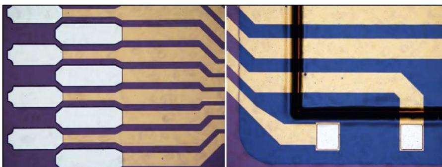
Figure 3.20. Electrode pads are opened after the parylene RIE process.
