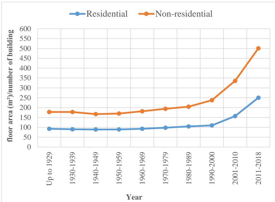
Figure 4.47. Annual variation of total floor area (m<sup>2</sup>) per number of building with respect to function of building
