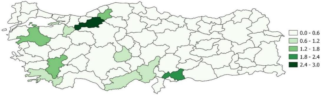
Figure 4.36. Percentage of calcium silicate brick (CSB) for infill walls in Turkey at province level
