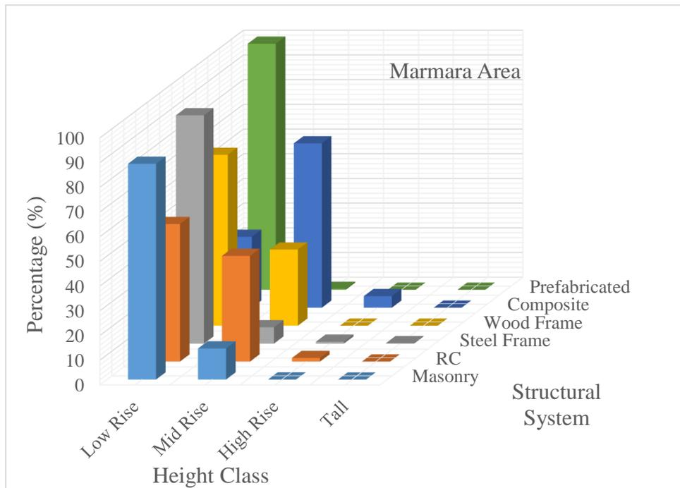
Figure B.9. Percentage of low, mid, high-rise and tall residential buildings with respect to structural system in Eastern Anatolia and Marmara Areas
