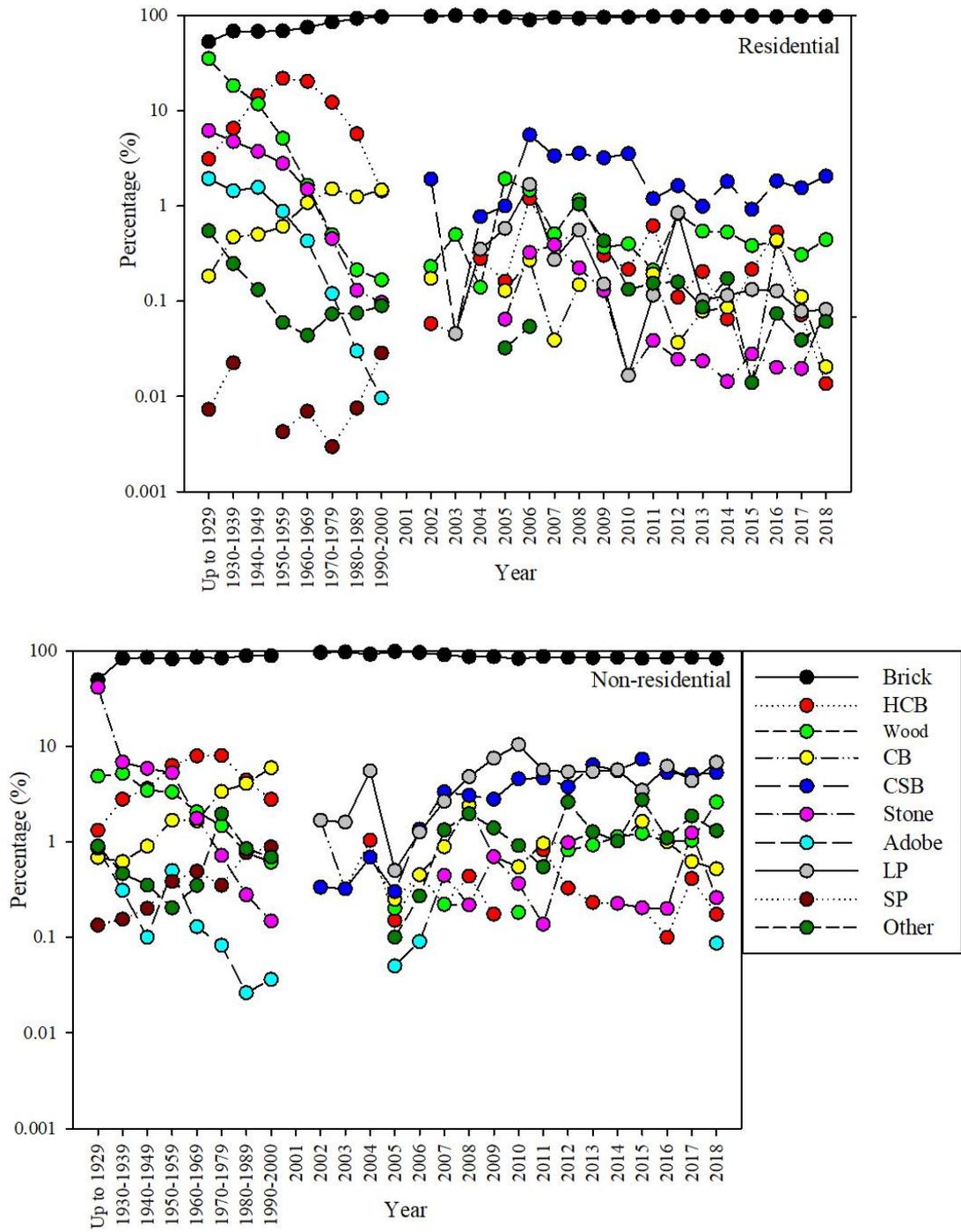
Figure B.20. Annual variation of material of infill wall percentage with respect to the use of building in İstanbul
