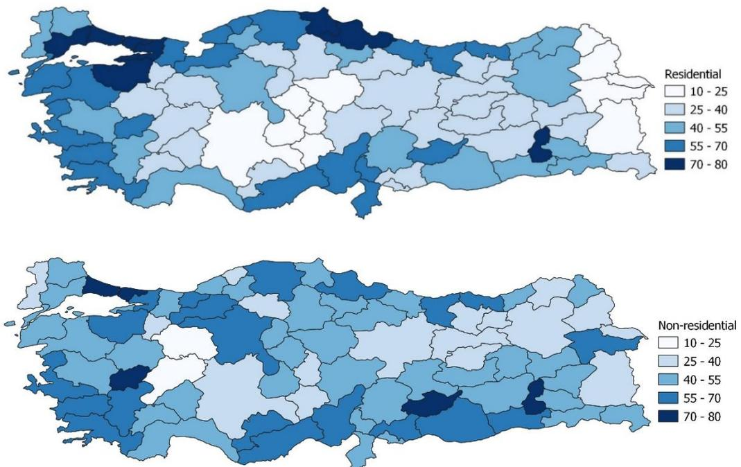
Figure 4.8. The percentage of RC structural system for residential and non-residential buildings at province level
