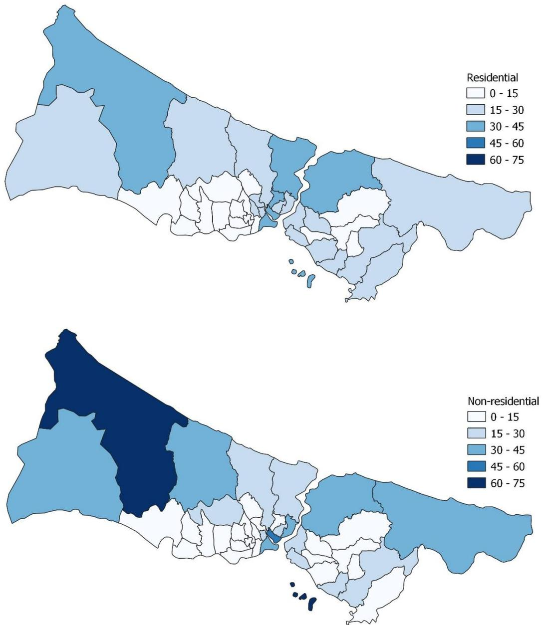
Figure 4.14. Masonry structural system percentages in residential and non-residential buildings in İstanbul at district level
