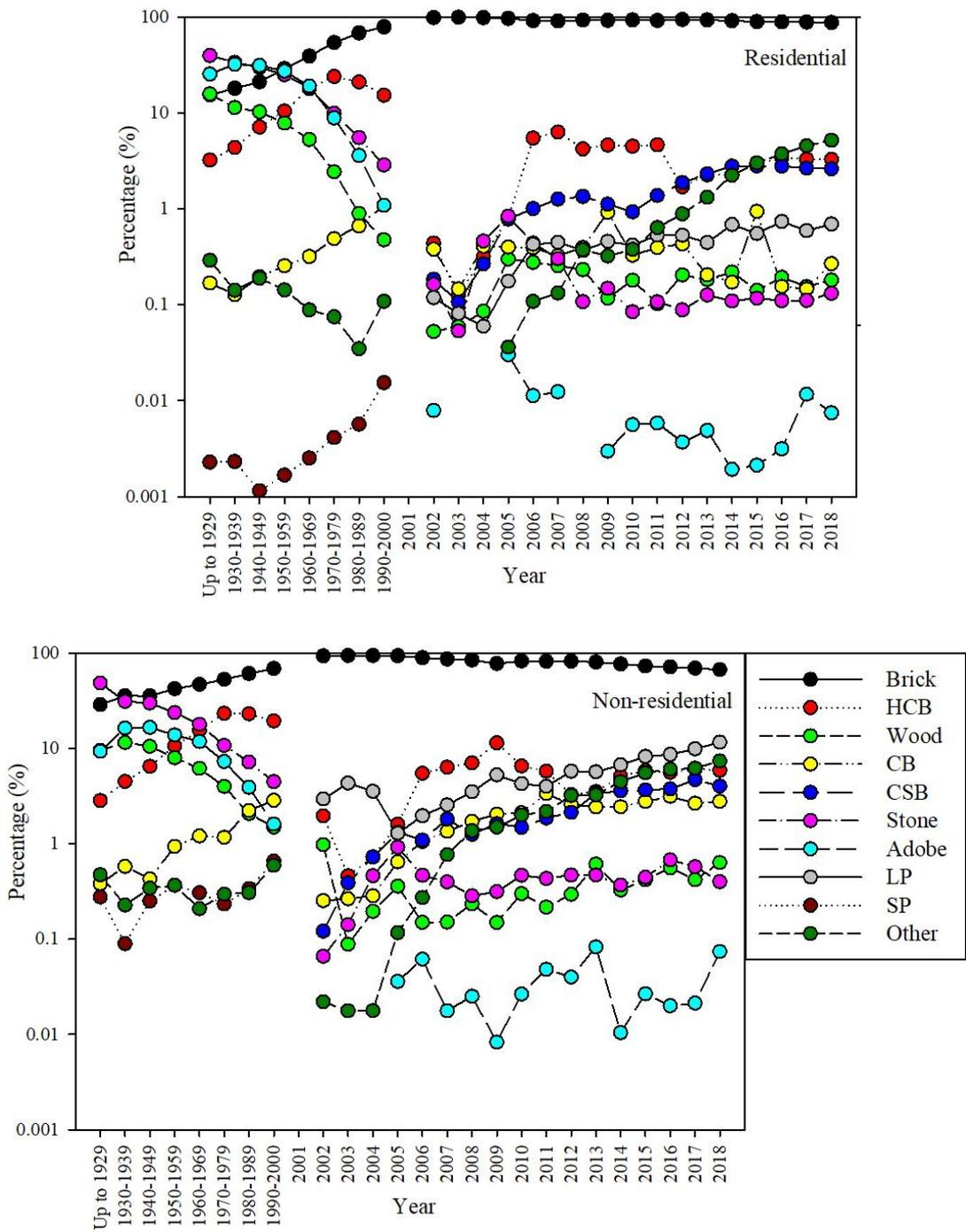
Figure B.17. Annual variation of material of infill wall in Turkey with respect to the use of building
