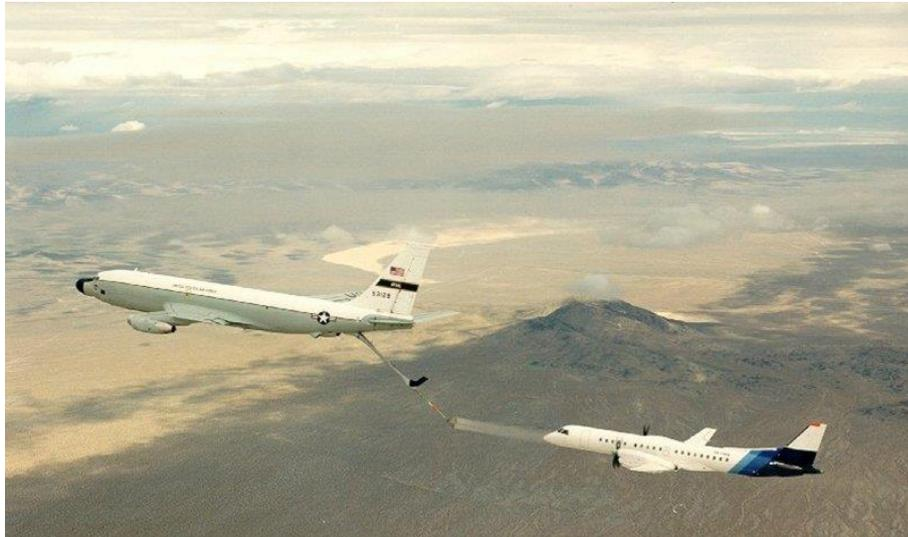
*Figure 1.2.* Icing tests in simulated clouds produced by icing tanker [9]
