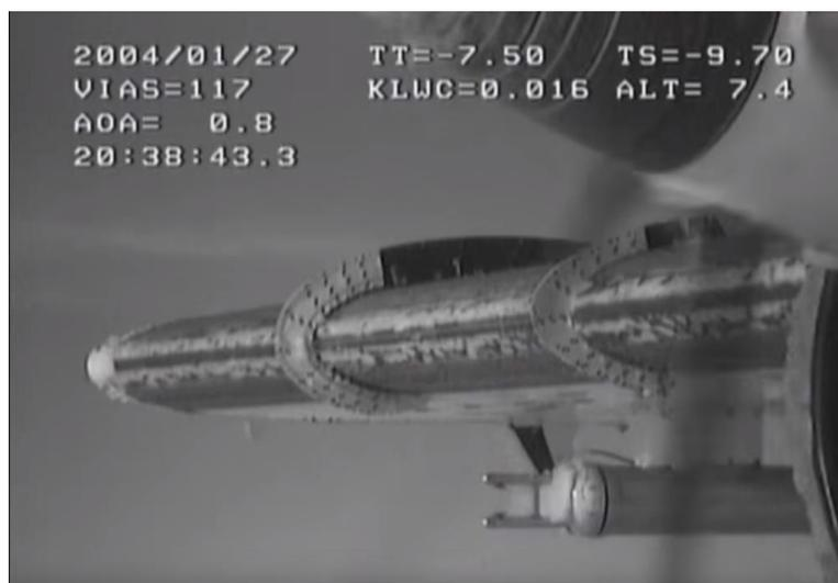
*Figure 1.1.* In-flight icing tests [17]
