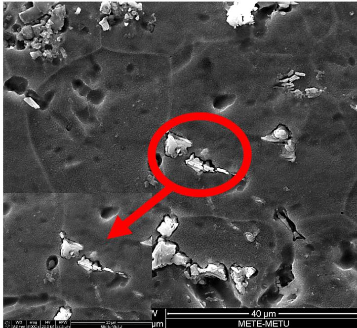
Figure 6.73 SEM image of white precipitates along the grain boundaries in hot-rolled 10wt.% 7075/B<sub>4</sub>C composite
