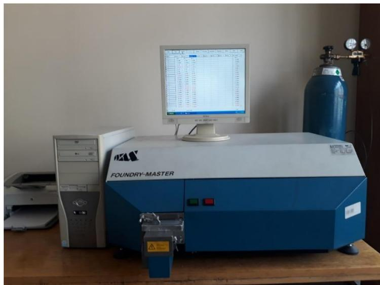
Figure 5.24 WAS Foundry Master optical emission spectroscopy used for chemical analysis
