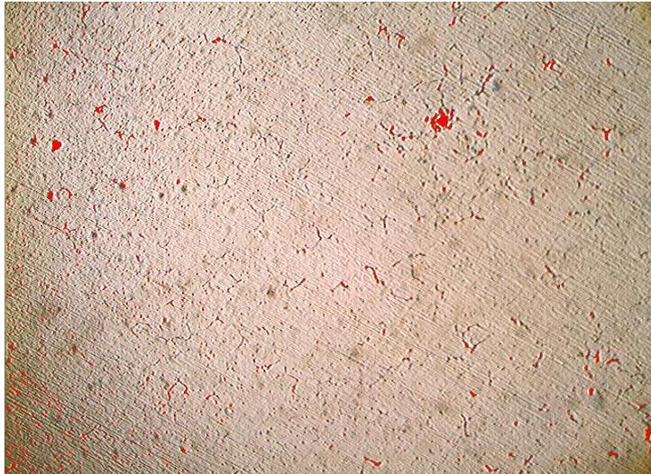
Figure 6.45 Porosity (red) in the microstructure of as-squeeze cast 7075 alloy produced under 15Hz frequency at 635°C SSM temperature (100x)
