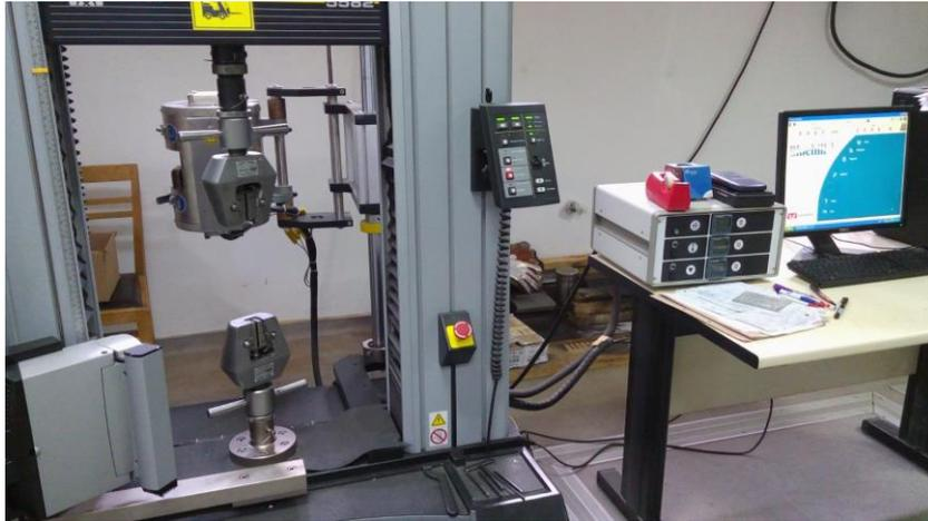
Figure 5.35 Instron Electromechanical Testing Device
