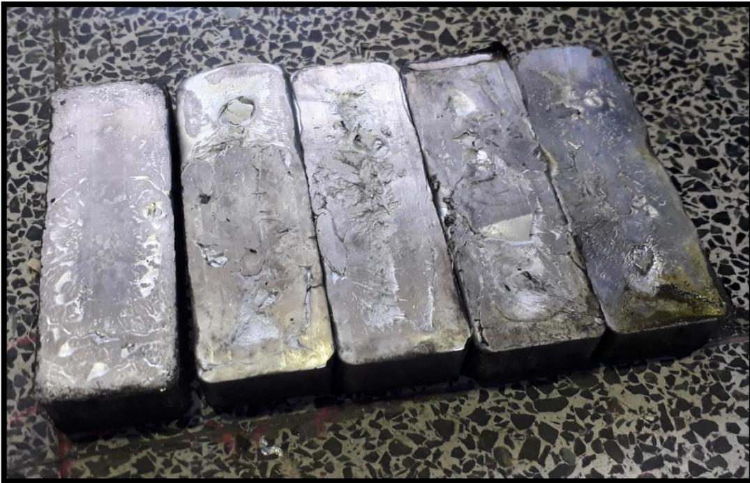
Figure 5.16 Semi-solid squeeze cast 7075 samples at different SSM temperatures
