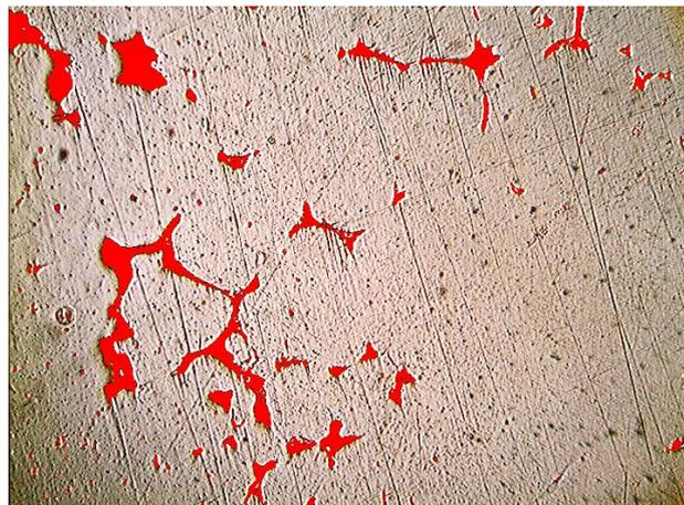
Figure 6.42 Porosity (red) in the microstructure of sand cast and T6-treated 7075 alloy produced under 15Hz frequency at 635°C SSM temperature (100x)
