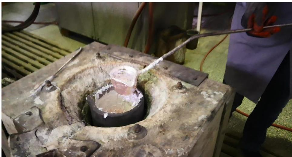
Figure 5.10 Transferring of liquid 7075 alloy and application of vibration in the ladle
