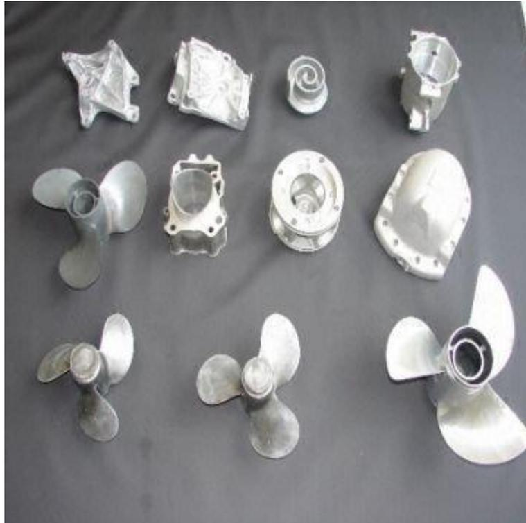
Figure 2.25 Various squeeze casting products
