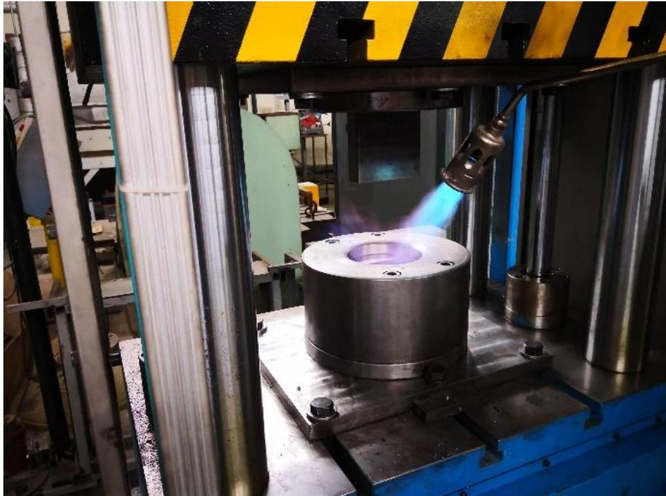
Figure 5.9 Pre-heating of metal mold by torch
