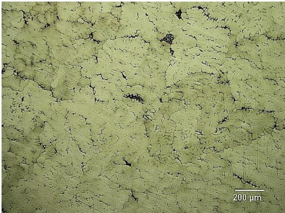
Figure 6.23 Microstructures of squeeze cast and T6-treated 7075 alloy produced with no-vibration at 670°C obtained by optical microscopy (200x)
