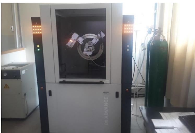
Figure 5.34 Bruker brand XRD device setup
