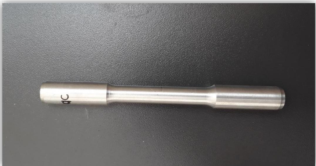
Figure 5.21 As machined tensile test specimen of squeeze casting experiment
