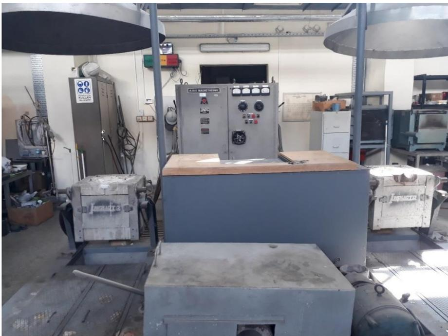
Figure 5.5 Induction furnace (25 kg steel capacity) where 7075 alloy was prepared
