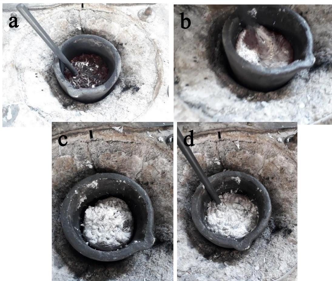
Figure 5.18 The stages of 7075/B<sub>4</sub>C mixture during composite making; a)initial addition of B<sub>4</sub>C powder after mixing of; b)5 minutes; c) 15 minutes; d)30 minutes
