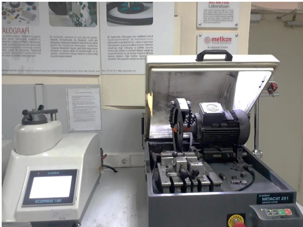
Figure 5.28 METACUT 251 Specimen cutter (right) and the mounting device (left)
