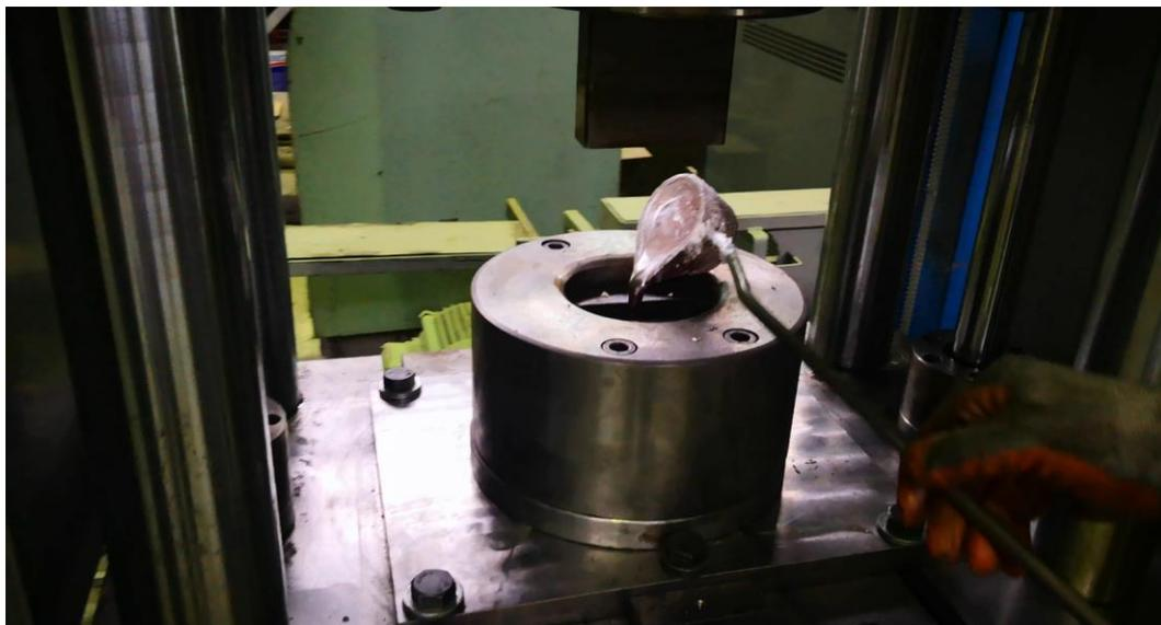
Figure 5.12 Casting of the semi-solid slurry into the die cavity just before pressure application
