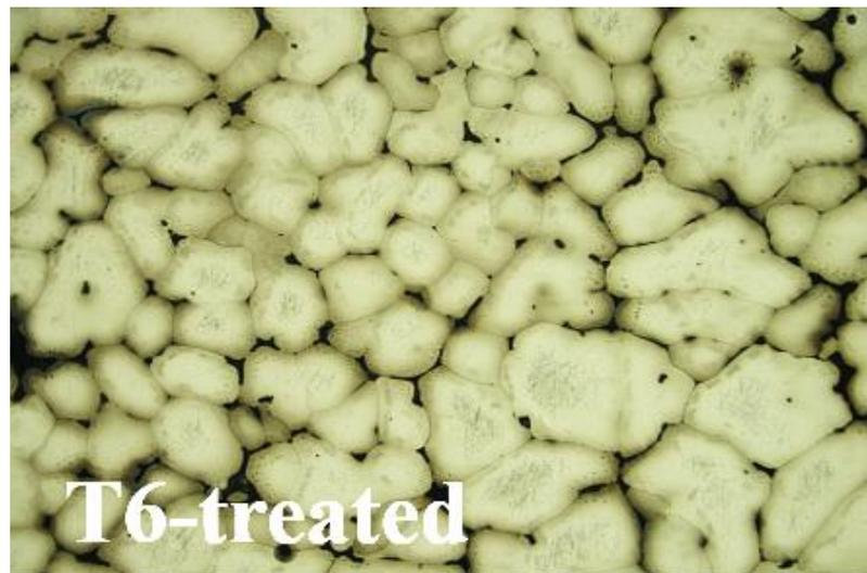
Figure 6.9 Microstructure of sand cast and T6 treated 7075 alloy produced under 15Hz frequency at 630°C SSM temperature obtained by optical microscopy (200x)
