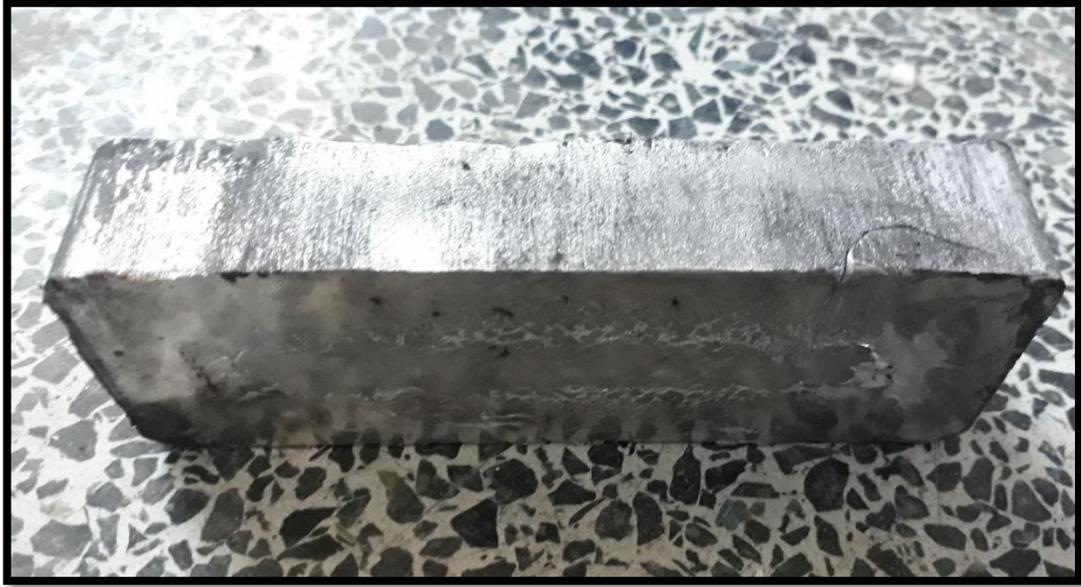
Figure 5.17 Single sample of 7075 alloy produced by squeeze casting
