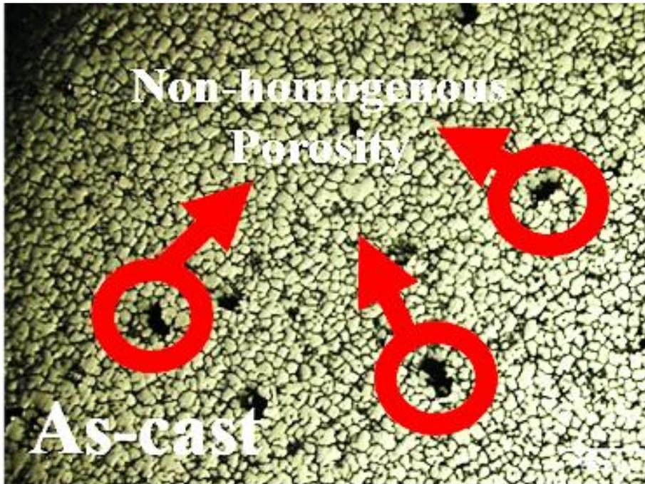
Figure 6.14 Microstructures of sand cast 7075 alloy produced under 15Hz frequency and 625°C SSM temperature obtained by optical microscopy (50x)
