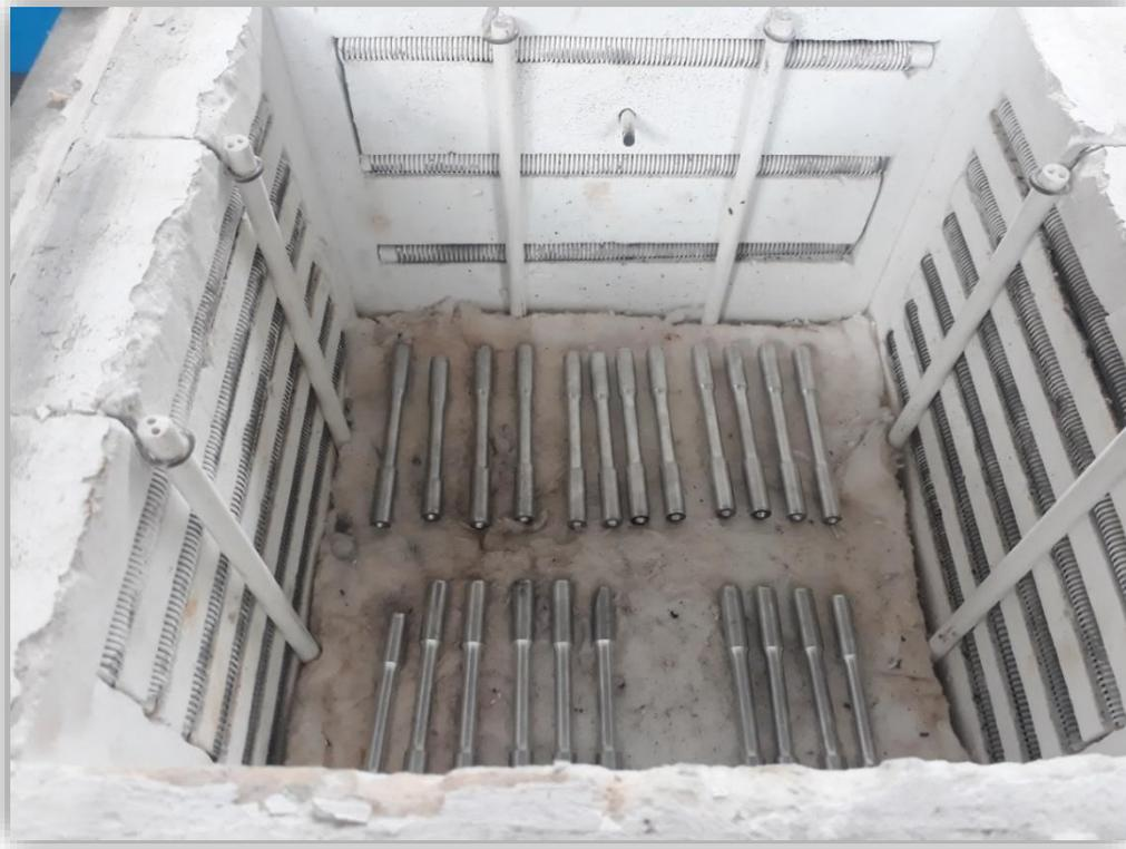
Figure 5.23 Tensile test specimens' placement in the electrical resistance furnace before solutionizing
