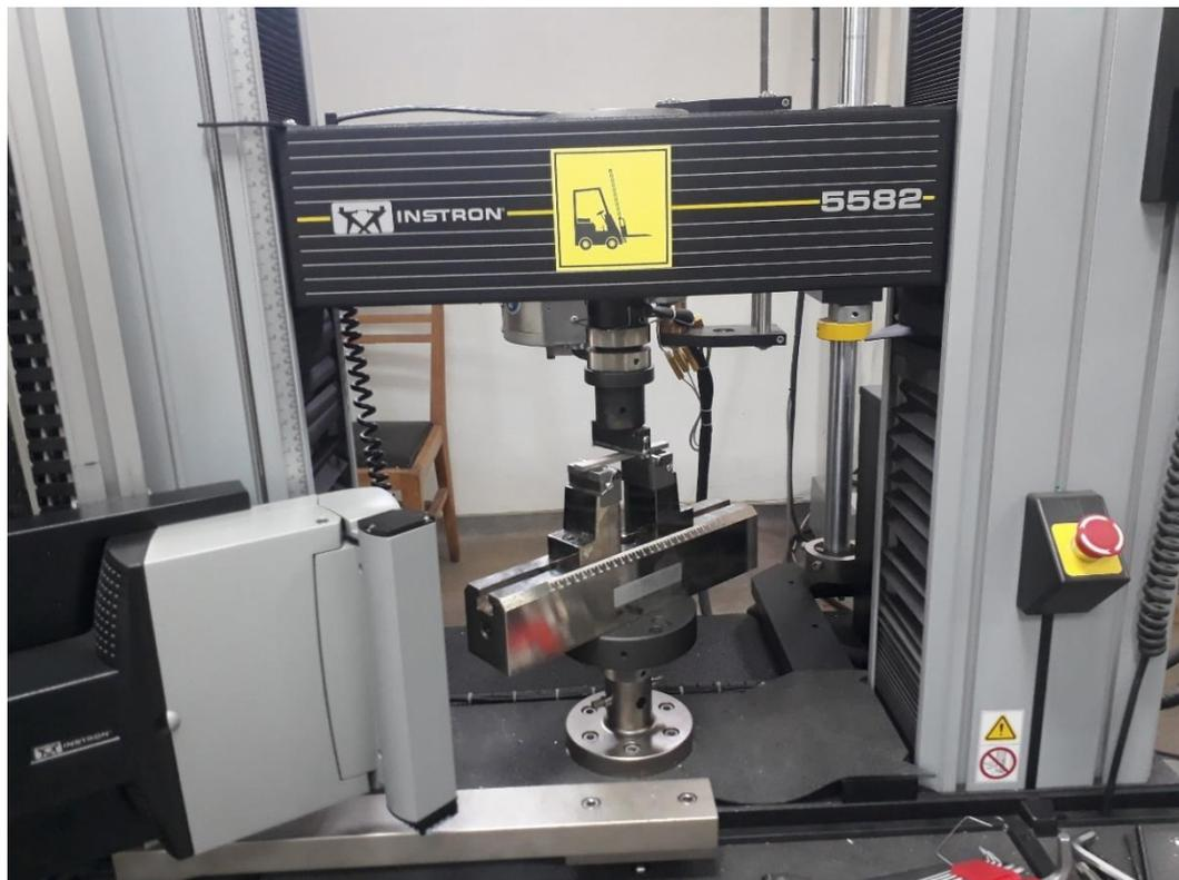
Figure 5.37 3-Point Bending Test on Instron Electromechanical Testing Device
