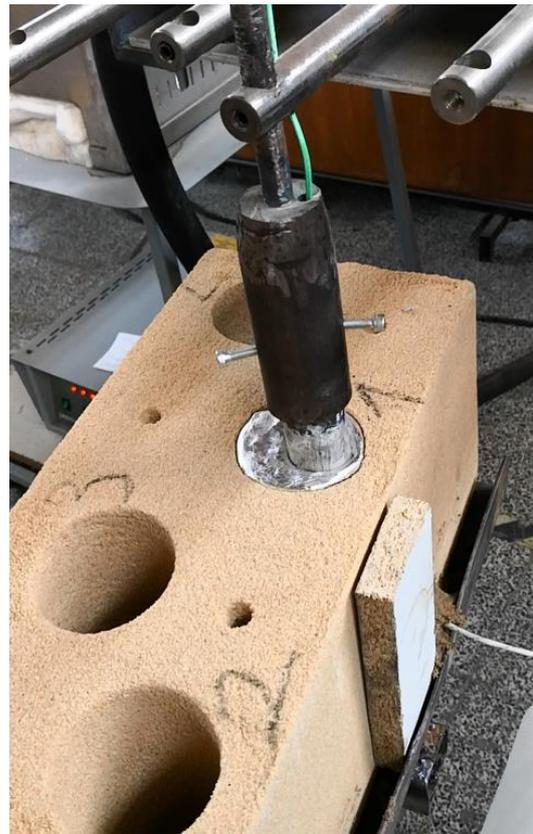
Figure 5.4 Temperature recording during solidification and the application of vibration
