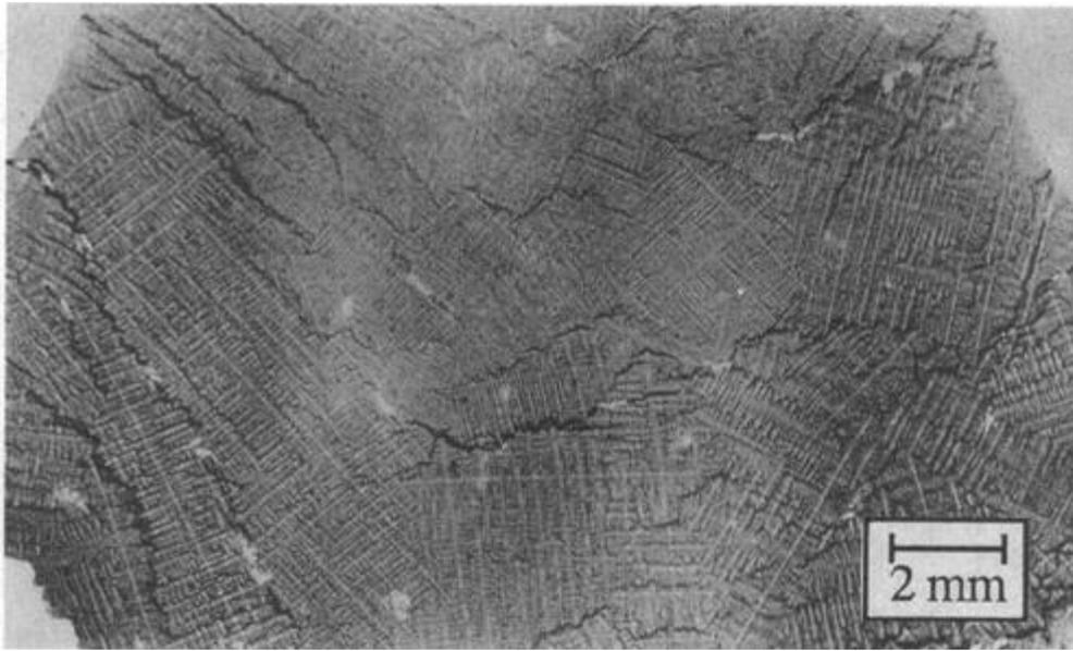
Figure 2.6 Radiography of Al-10Cu alloy filled with hot tears [8]
