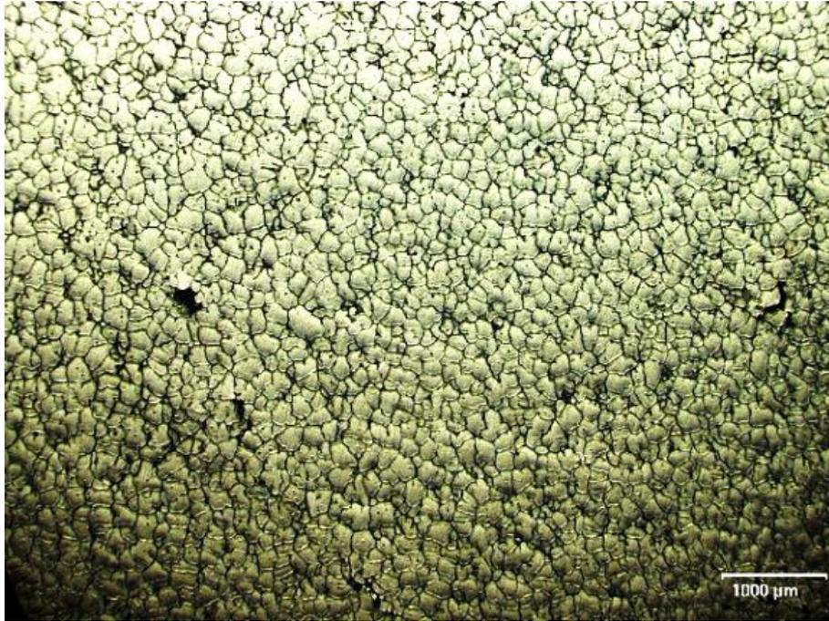
Figure 6.12 Microstructure of sand cast 7075 alloy produced under 15Hz frequency 635°C SSM temperature obtained by optical microscopy (50x)
