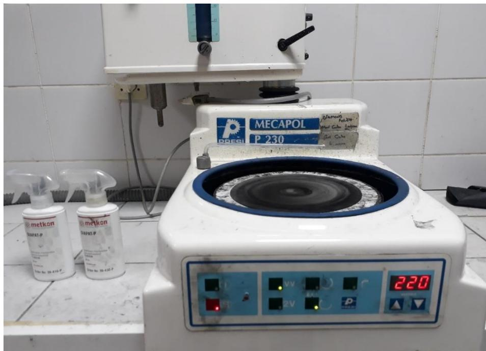
Figure 5.30 Rotating disc type polisher with  $6\mu$  by  $1\mu$  diamond solutions
