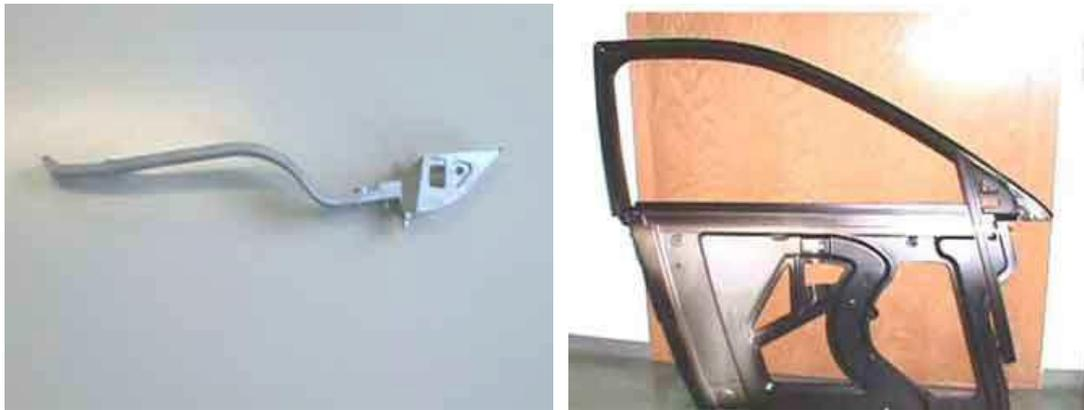
Figure 2.12 Rheocast thin walled structural parts in doors AUDI A3 [2]
