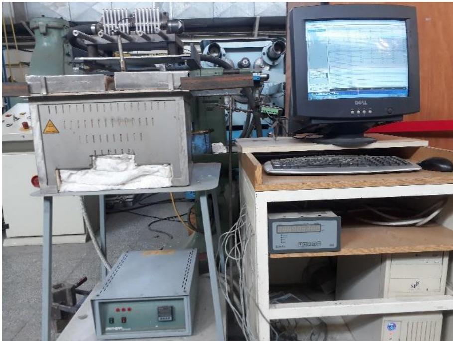
Figure 5.6 Vibration machine and thermal analysis set-up connected to each other
