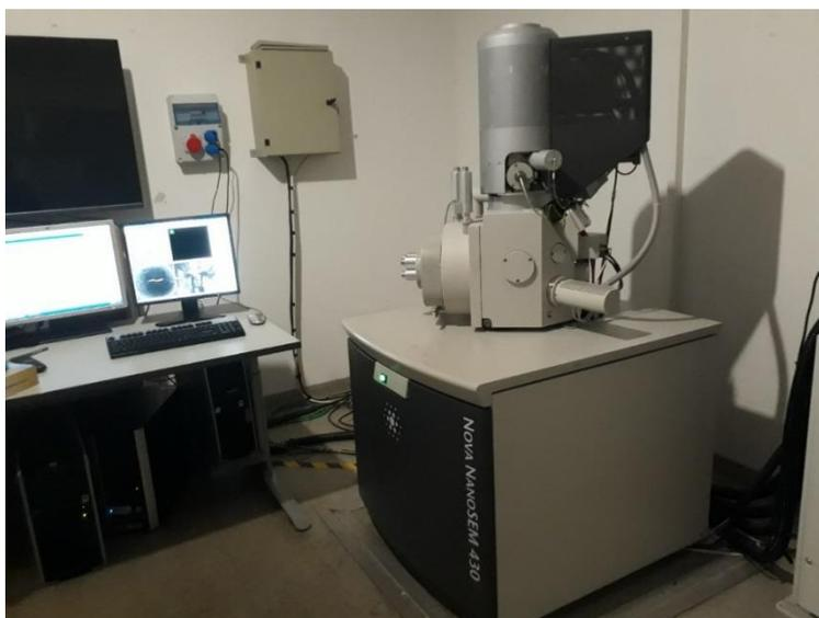
Figure 5.33 NOVA NANOSEM 430 Scanning electron microscopy setup
