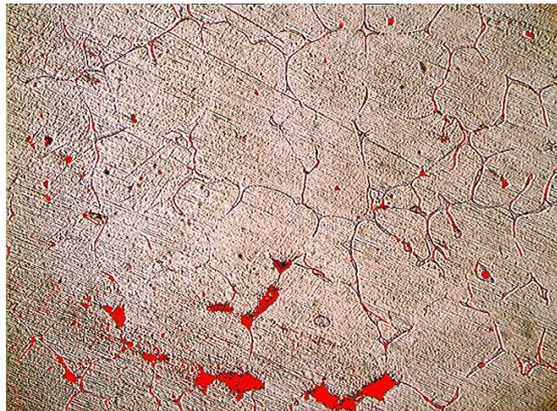
Figure 6.41 Porosity (red) in the microstructure of sand cast 7075 alloy produced under 15Hz frequency and 635°C SSM temperature (100x)
