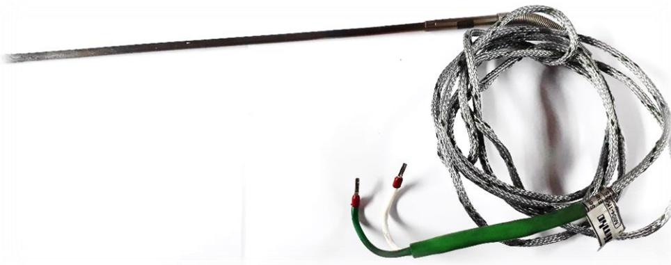
Figure 5.26 K-type thermocouple with metal casing
