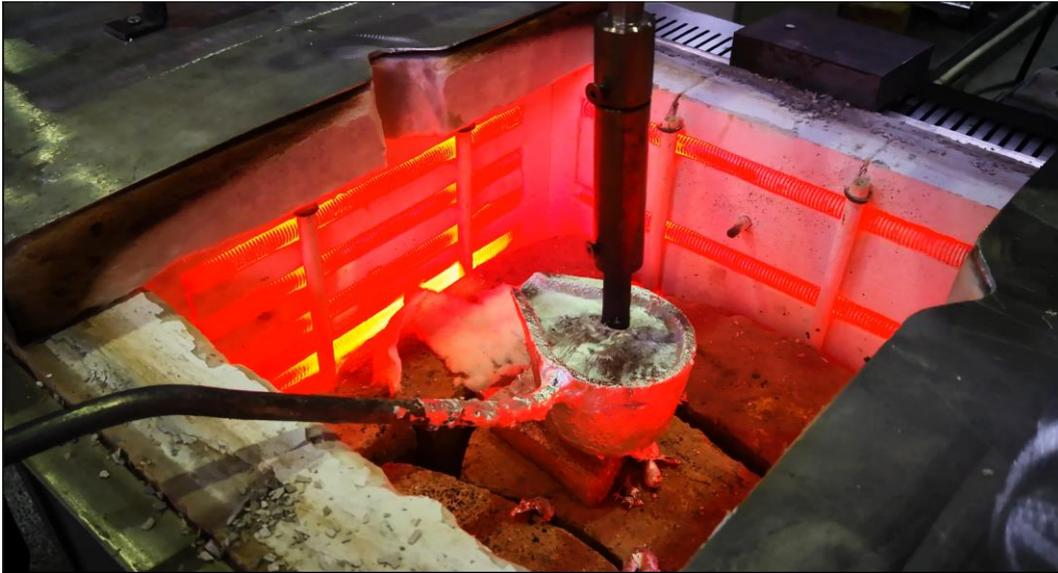
Figure 5.11 The application of vibration inside the ladle for conditioning
