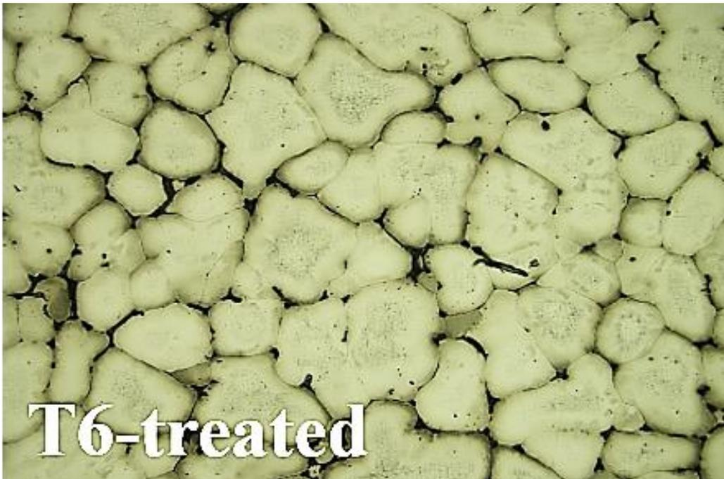
Figure 6.10 Microstructure of sand cast and T6 treated 7075 alloy produced under 15Hz frequency at 625°C SSM temperature obtained by optical microscopy (200x)
