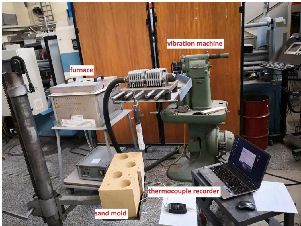
Figure 5.2 Whole experimental set-up used in sand-casting experiments consisting of electrical resistance furnace, vibration machine, sand mold and thermocouple recorder
