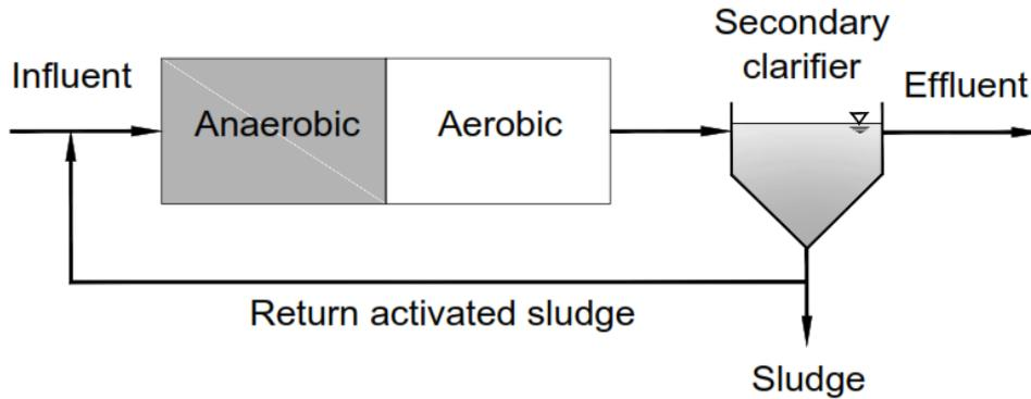
Figure 2-9 The Diagram of A/O Biological Phosphorous Removal Process Adapted from Figure 8-29 (a) (Stensel et al., 2014)
