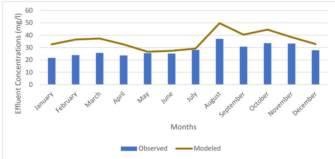
Figure 5-9 Effluent COD concentrations for 2017 Validation
