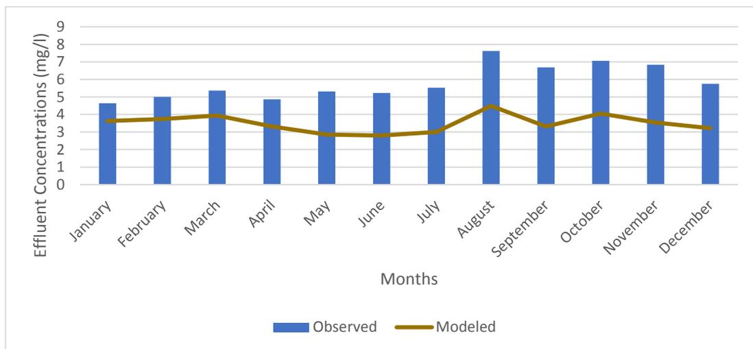
Figure 5-10 Effluent BOD concentrations for 2017 Validation
