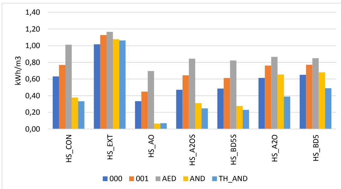
Figure 4-6 SEC2 Results for HS Wastewaters
