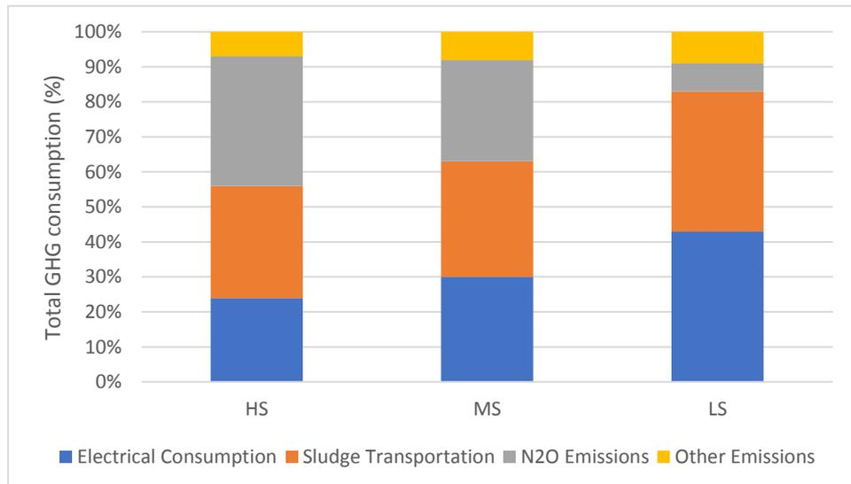
Figure 4-10 GHGs Average Contribution to The Total Carbon Footprint for Different WW Strengths
