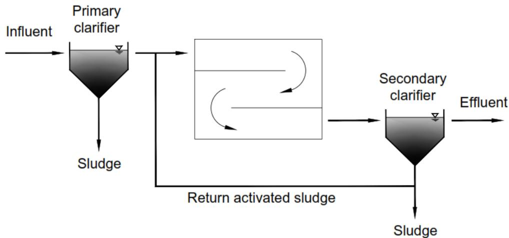
Figure 2-3 The Diagram of Plug-flow Adapted from Figure 8-15 (b) (Stensel et al., 2014)
