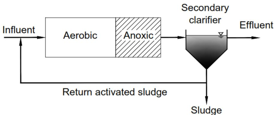
Figure 2-7 The Diagram of Post-Anoxic Biological Nitrogen Removal Process Adapted from Figure 8-21 (c) (Stensel et al., 2014)
