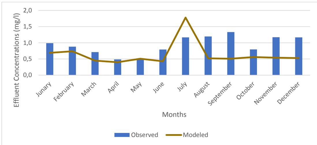
Figure 5-13 Effluent TP concentrations for 2017 Validation
