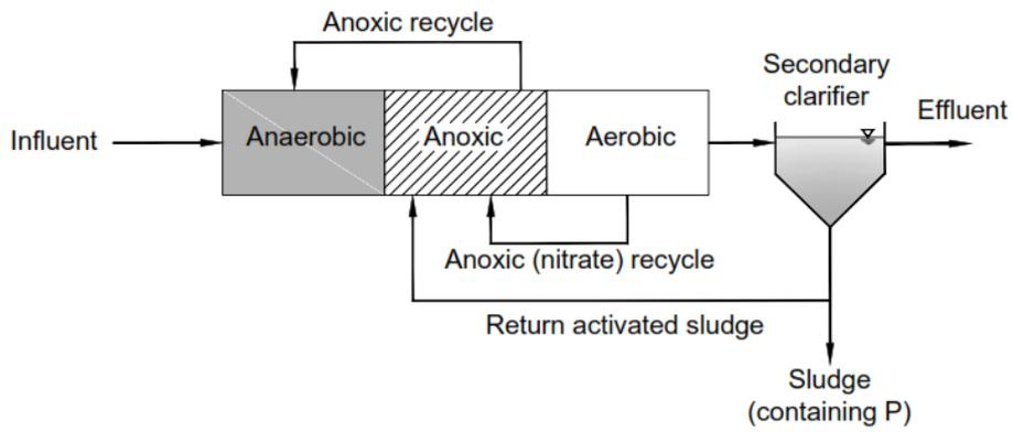
Figure 2-12 The Diagram UCT Process Adapted from Figure 8-29 (d) (Stensel et al., 2014)
