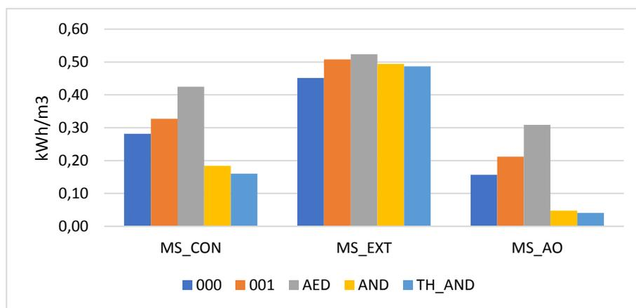
Figure 4-7 SEC1 Results of Conventional AS, Extended Aeration And A/O Processes for MS Wastewaters
