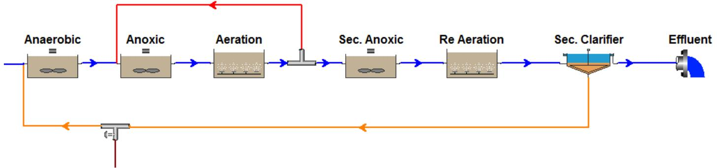
Figure B-5 BioWin Layout of Bardenpho-5 Process
