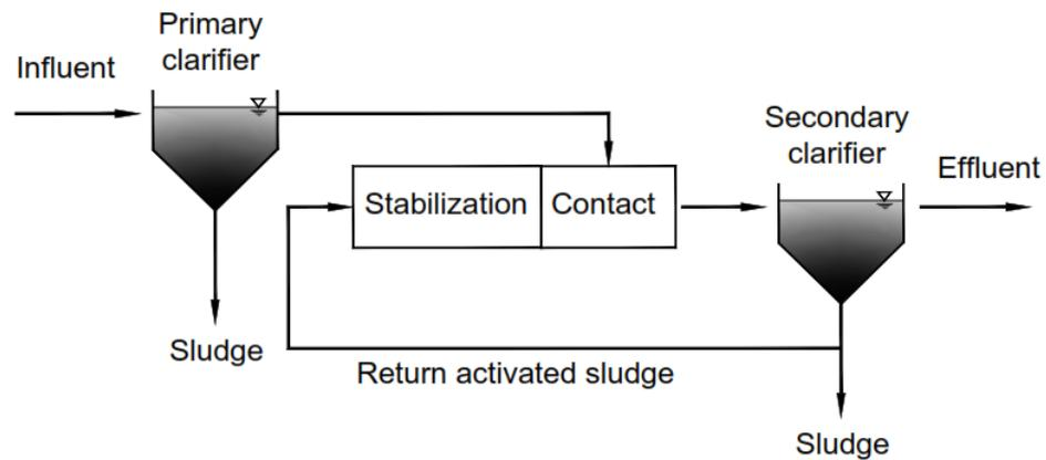
Figure 2-4 The Diagram of Contact-stabilization Adapted from Figure 8-15 (e) (Stensel et al., 2014)
