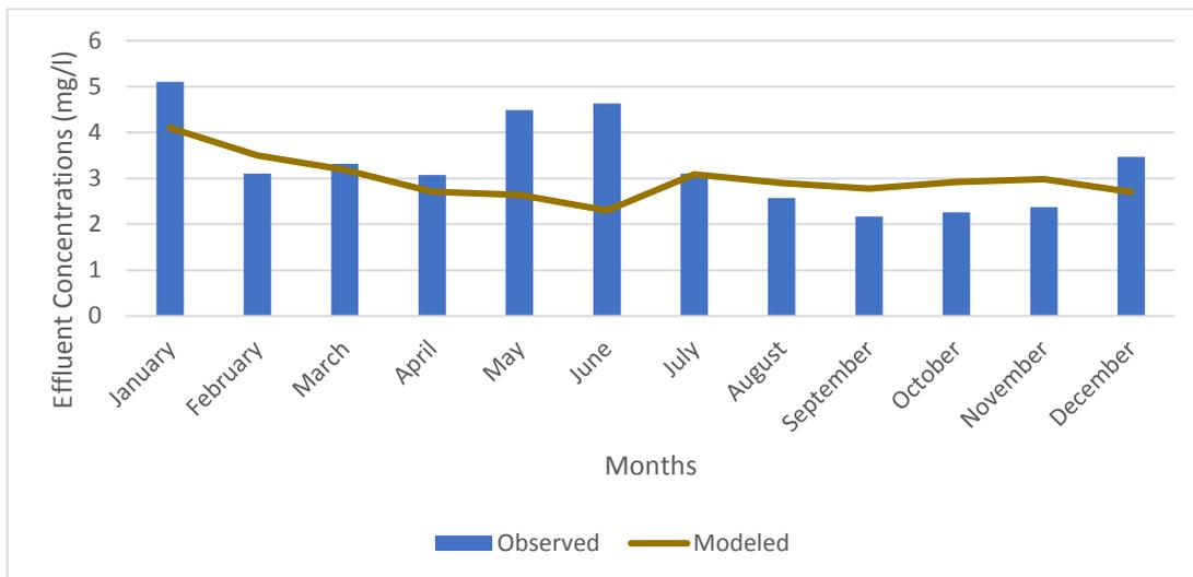
Figure 5-12 Effluent TN concentrations for 2017 Validation
