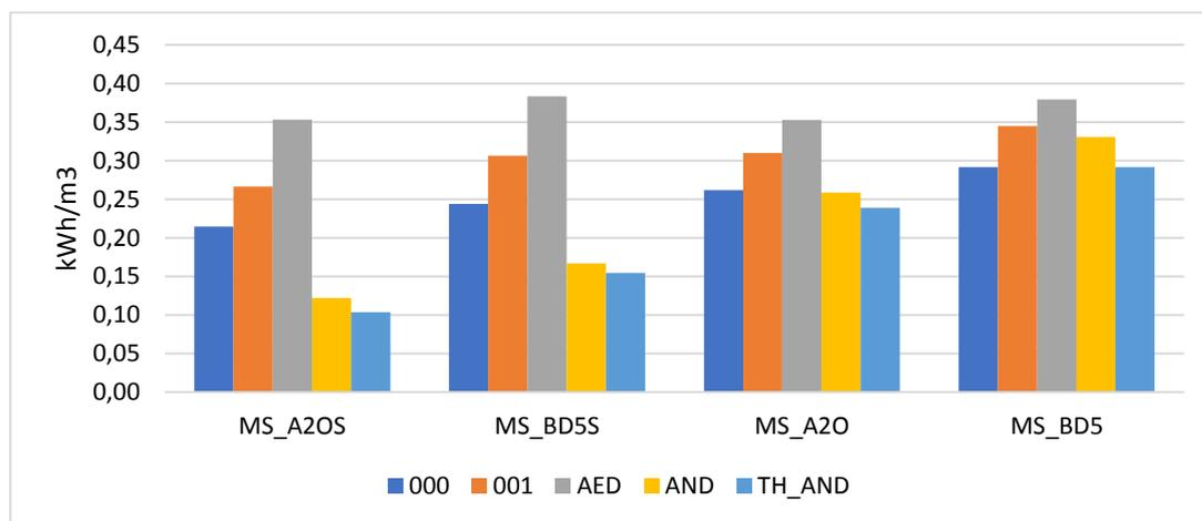
Figure 4-8 SEC1 Results of A2O And Bardenpho-5 Processes for MS Wastewaters
