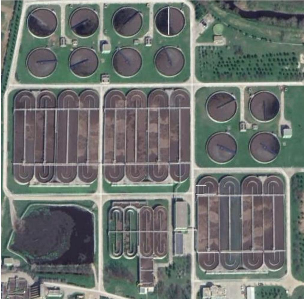
Figure 5-3 Top View of the Process Lines in the WWTP
