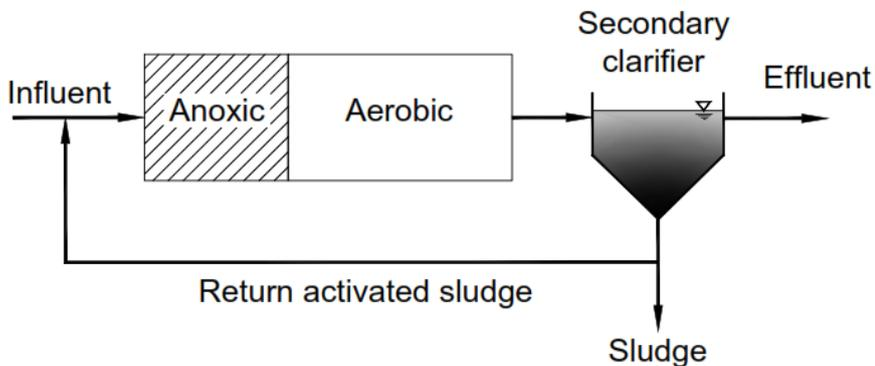
Figure 2-6 The Diagram of Pre-Anoxic Biological Nitrogen Removal Process Adapted from Figure 8-21 (a) (Stensel et al., 2014)
