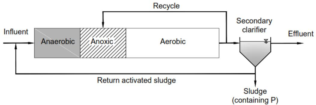
Figure 2-10 The Diagram of A2O Process Adapted from Figure 8-29 (b) (Stensel et al., 2014)
