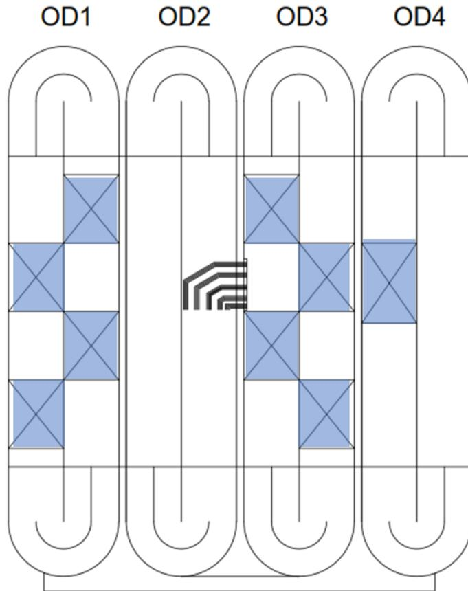
Figure 5-7 Picture taken from construction plan. Diffuser placement shown with blue boxes
