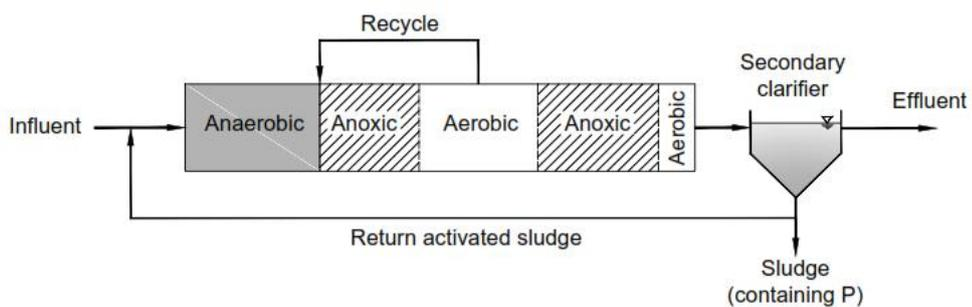
Figure 2-11 The Diagram of 5-Stage Bardenpho Process Adapted from Figure 8-29 (c) (Stensel et al., 2014)
