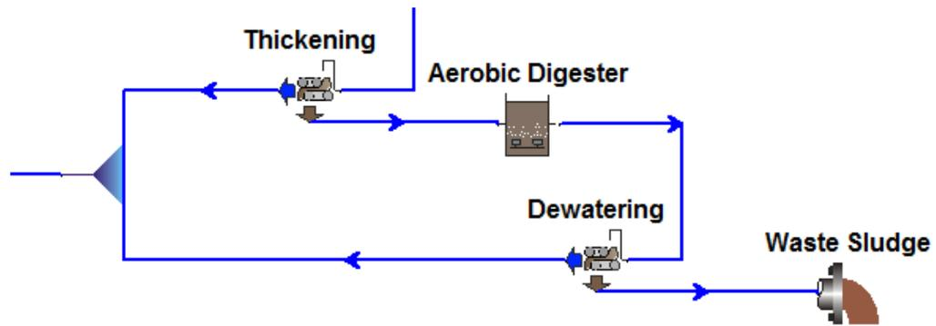
*Figure B-7 BioWin Layout Of Aerobic Sludge Process*
