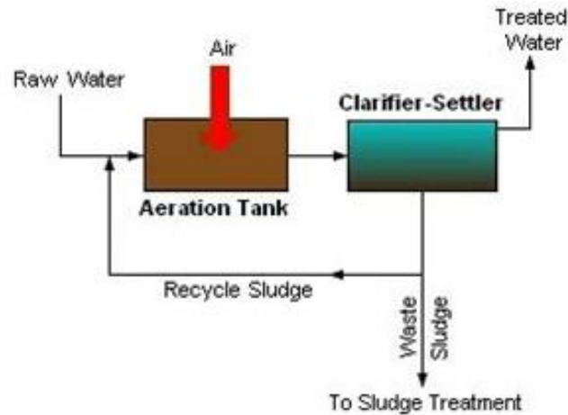
Figure 2-1. The Diagram of AS Process (Rieger et al., 2012)
