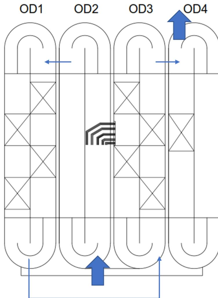
Figure 5-4 Oxidation Ditch Bioreactors Configuration of Bursa East WWTP
