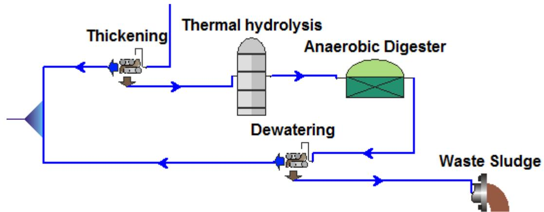
*Figure B-9 BioWin Layout of Anaerobic Sludge Process with Thermal Hydrolysis*
