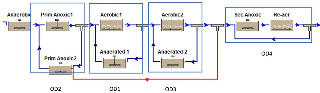
Figure 5-8 Oxidation Ditch Configuration
