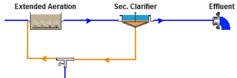
Figure B-2 BioWin Layout of Extended Aeration Process
