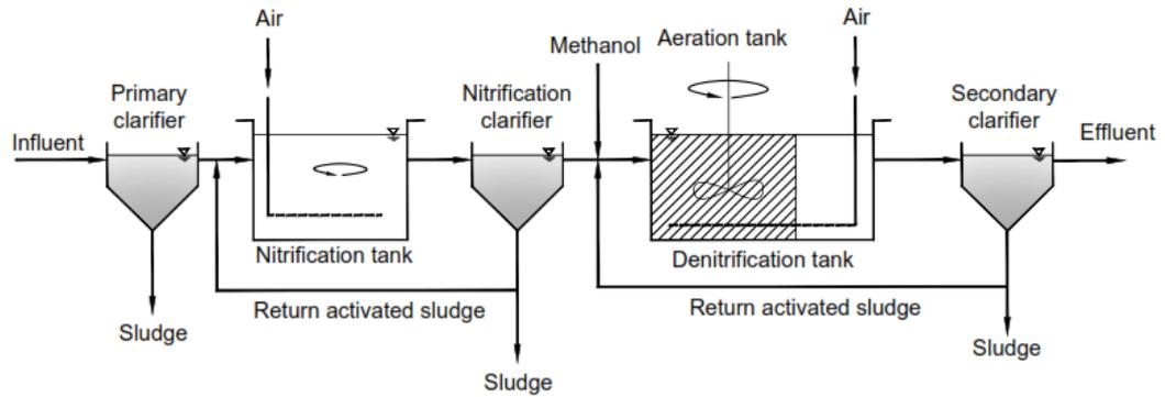
Figure 2-8 The Diagram of Two-Sludge Biological Nitrogen Removal Process Adapted from Figure 8-21 (e) (Stensel et al., 2014)
