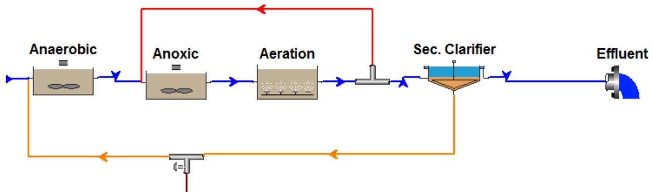
Figure B-4 BioWin Layout of A2O Process
