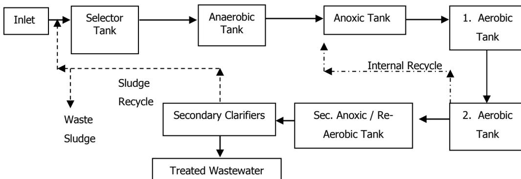
Figure 5-2 Wastewater Treatment Process Flow Diagram of Bursa East Municipal WWTP
