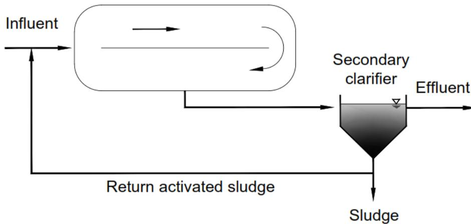
Figure 2-5 The Schematic Diagram of Oxidation Ditch Process Adapted from Figure 8-15 (j) (Stensel et al., 2014)
