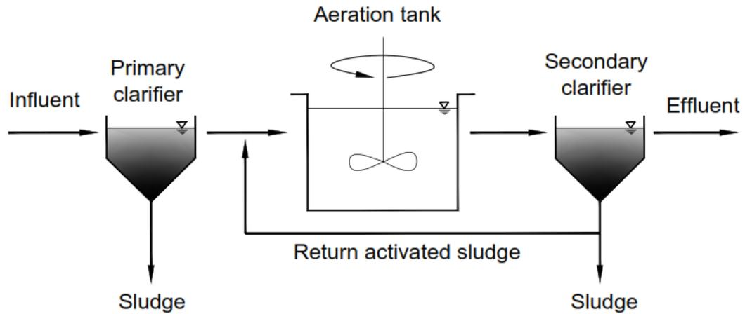
Figure 2-2 The Diagram of CMAS Adapted from Figure 8-1(a) (Stensel et al., 2014)
