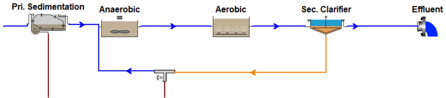
Figure B-3 BioWin Layout of A/O Process
