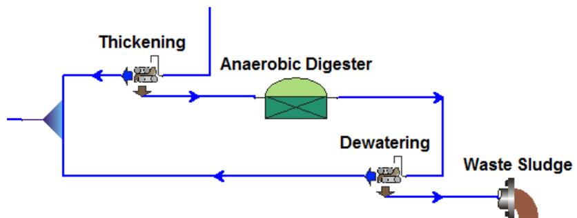
*Figure B-8 BioWin Layout of Anaerobic Sludge Process*
