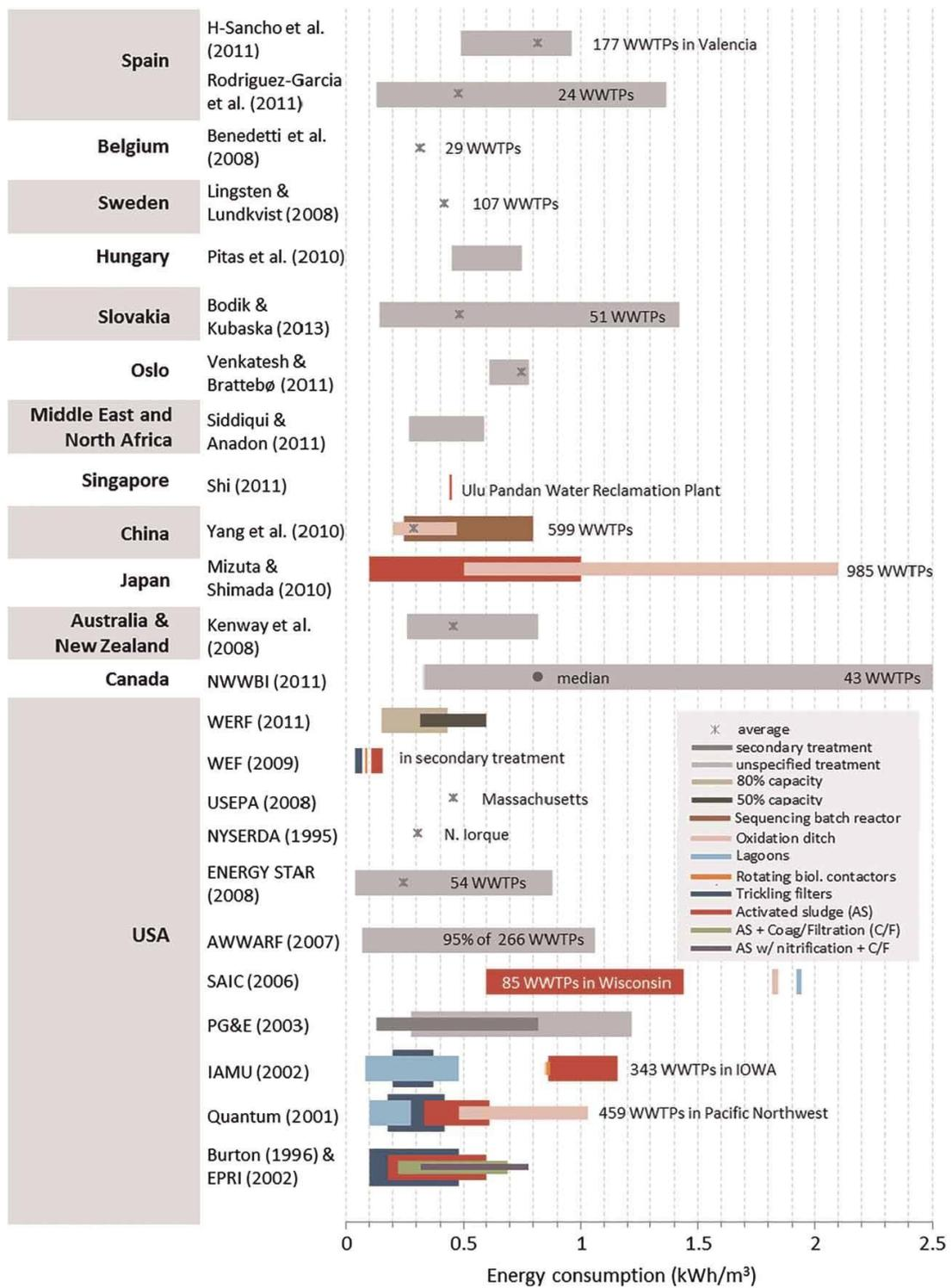
Figure 2-15 Energy Consumption per Treated Wastewater Volume in Different Countries (Silva et al., 2015)
