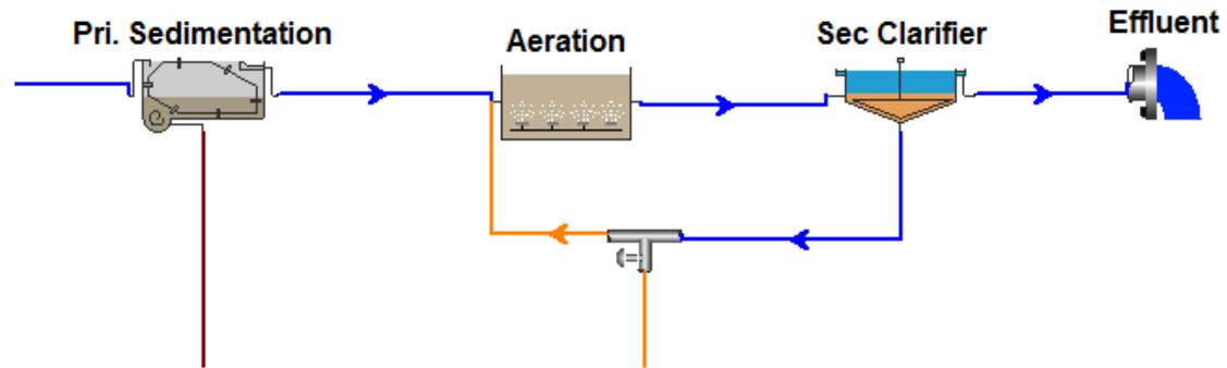
Figure B-1 BioWin Layout of Conventional AS Process
