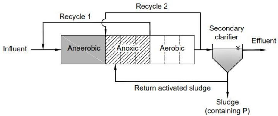
Figure 2-13 The Diagram of VIP Process Adapted from Figure 8-29 (e) (Stensel et al., 2014)
