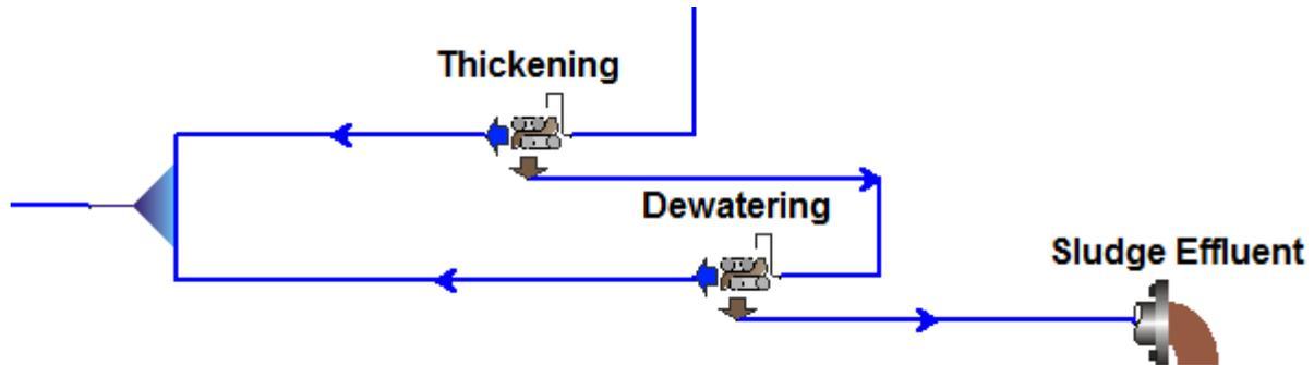
Figure B-6 BioWin Layout of Only Thickening and Dewatering Sludge Process
