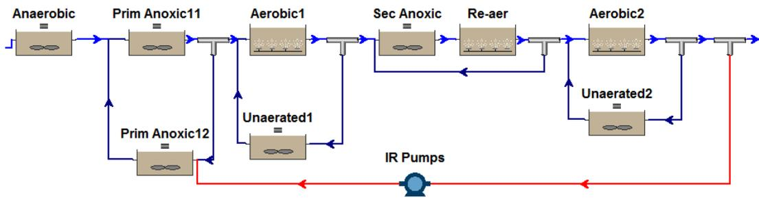
Figure 5-16 A2O configuration line up of Bursa East Municipal WWTP
