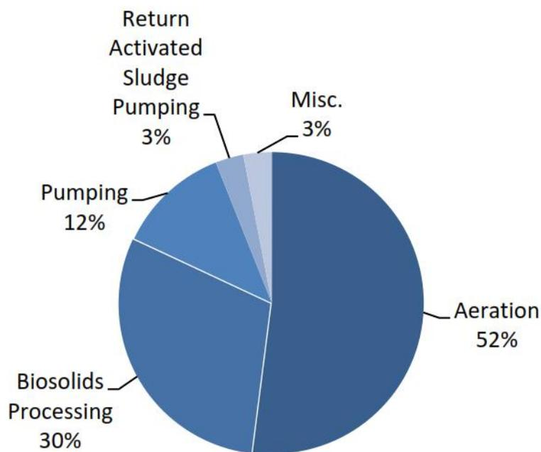
Figure 2-14 Typical Energy End-Uses in Municipal Wastewater Treatment (Pabi et al., 2013)
