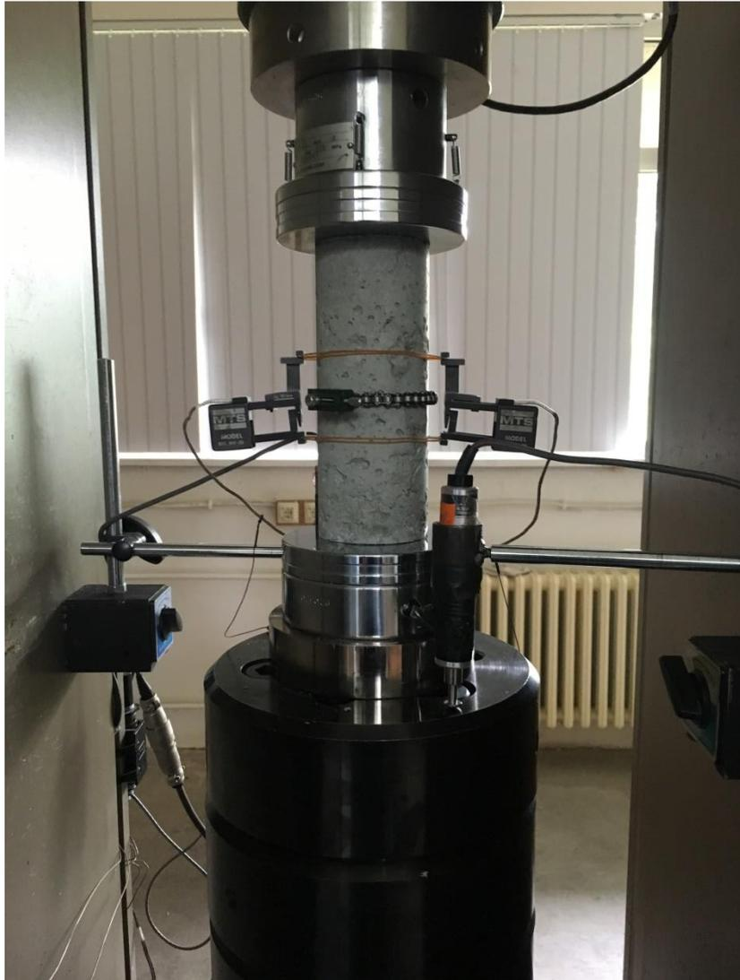
*Figure C.5. Example of the deformability test photos during the test*
