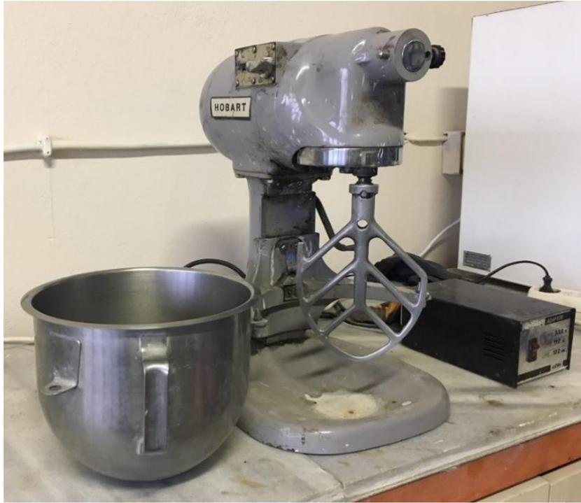
*Figure 3.8 Hobart N50 laboratory type mixer*
