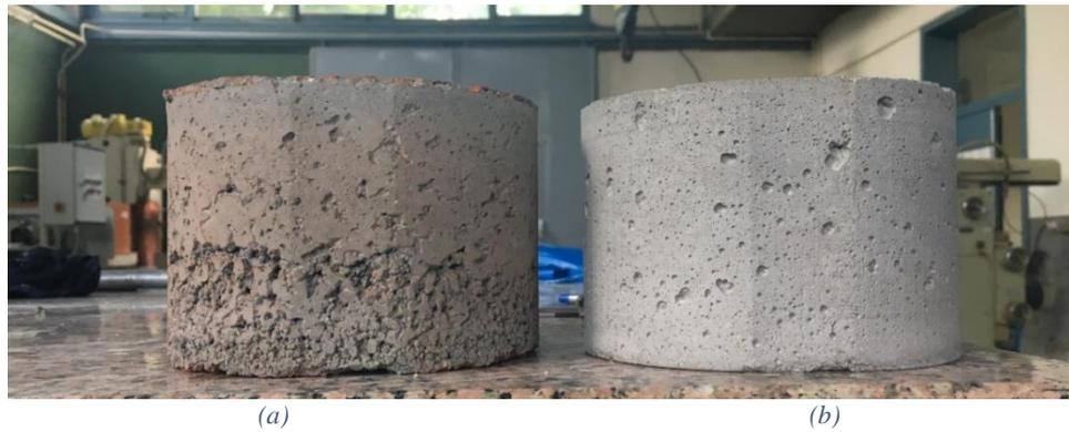
*Figure 5.11 Example of shotcrete specimen (a) with porous structure and (b) with targeted normal structure*
