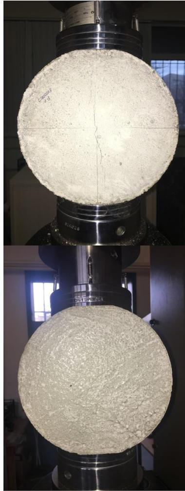
*Figure E.45 Examples of the FBD samples with 180 mm diameter*
