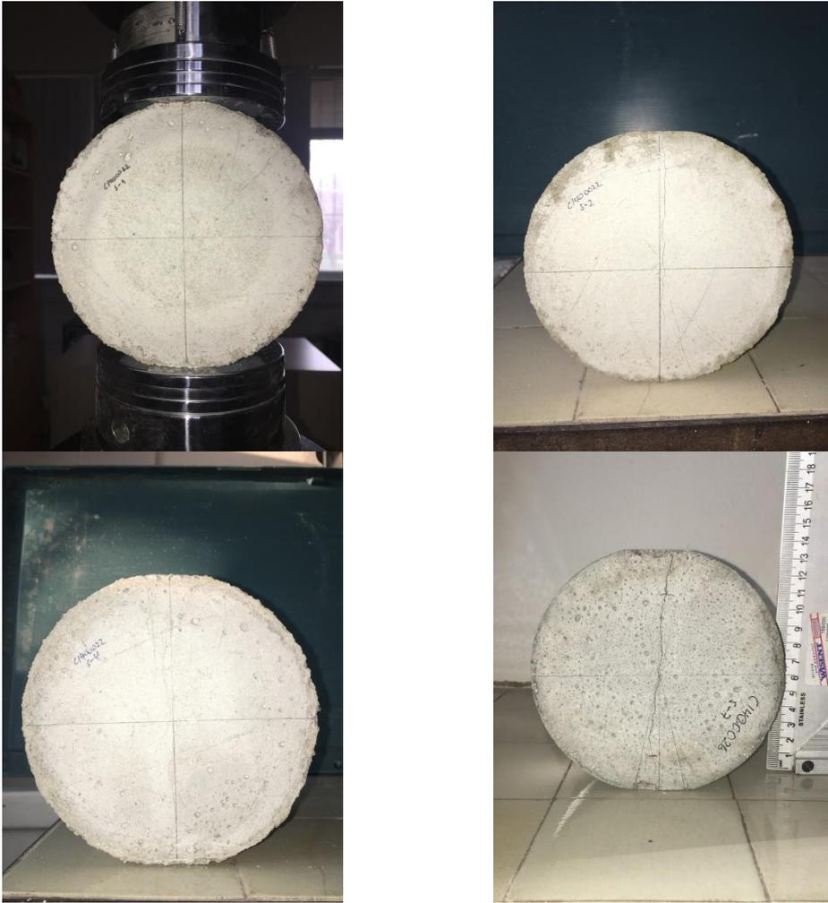
*Figure E.43 Examples of the FBD samples with 140 mm diameter*
