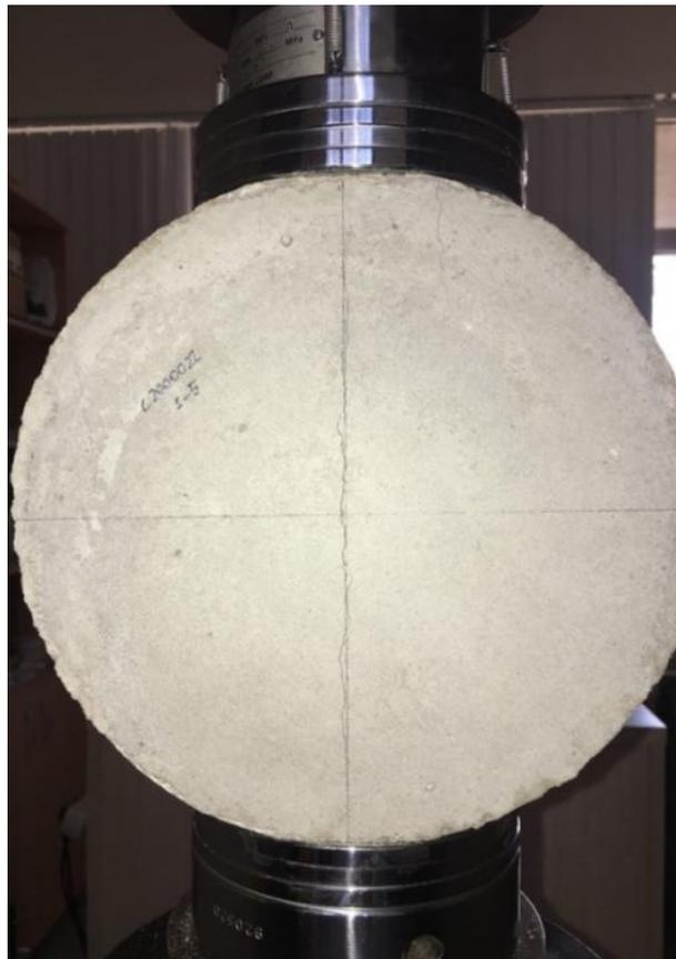
*Figure 6.1 C200-22\_s5 coded shotcrete sample during fracture toughness test*
