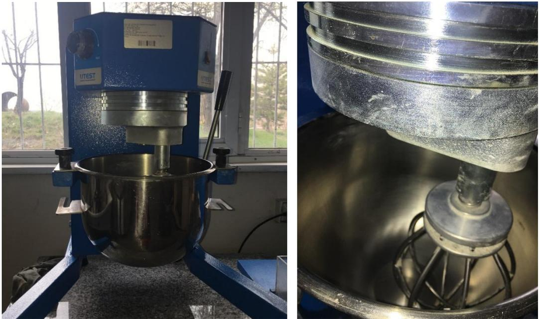
*Figure 3.9 UTEST laboratory type concrete mixer*
