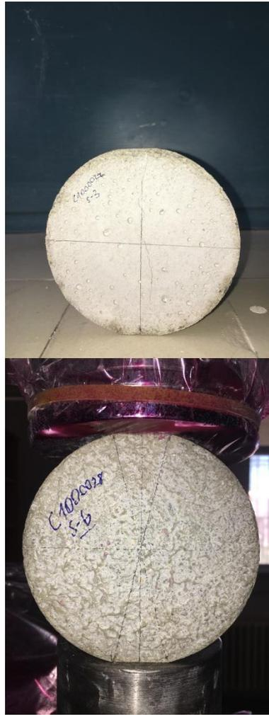
Figure E.41 Examples of the FBD samples with 100 mm diameter
