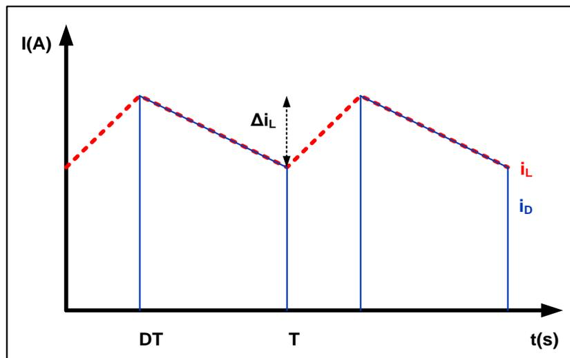
Figure 3.11. Boost Converter Diode (or Synchronous Rectifying MOSFET) Current Waveform
