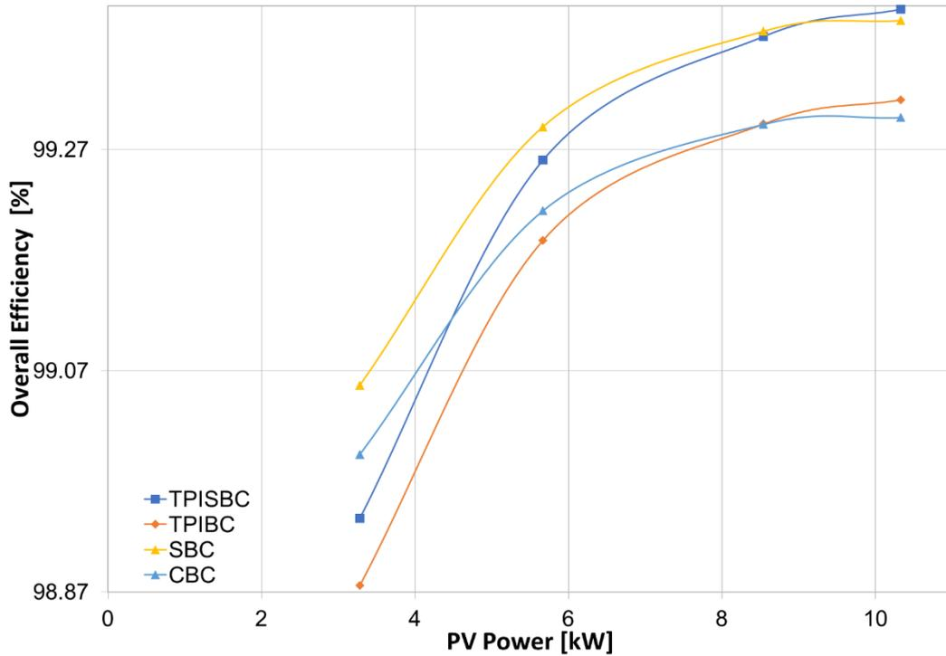
Figure 3.22. Effect of Operating Power on Overall Efficiency for Four Configuration Options: Two-Phase Interleaved Synchronous Boost Converter (TPISBC), Two-Phase Interleaved Boost Converter (TPIBC), Synchronous Boost Converter (SBC) and Conventional Boost Converter (CBC)
