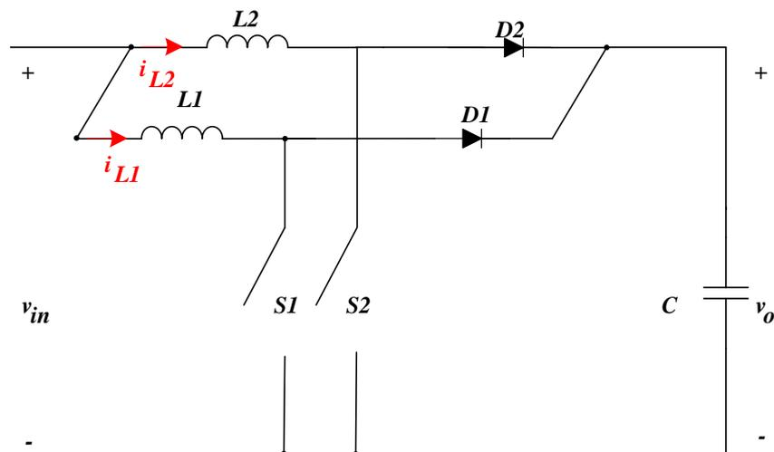
Figure 2.7. Two-Phase Boost Converter Diagram
