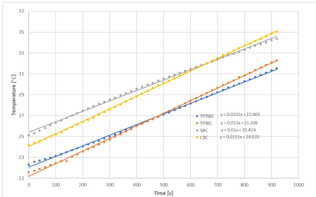
Figure 4.22. Temperature Profile of Boost Converter Configurations
