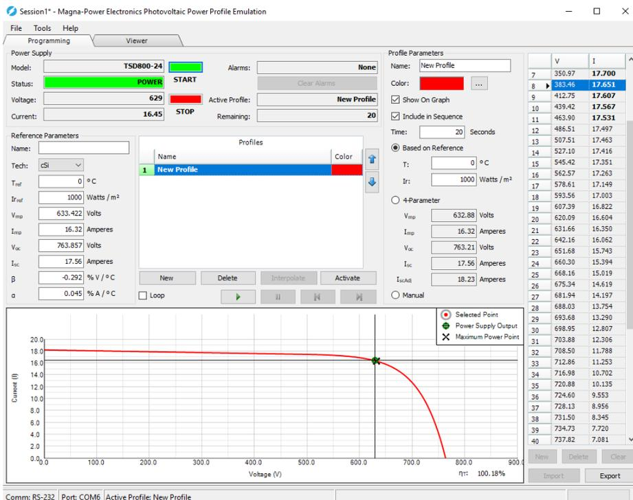
Figure 4.5. TPISBC Power Stage 1000 W/m<sup>2</sup> operation at MPP
