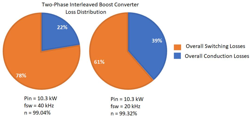
*Figure 3.7.* Loss Distribution of Two-Phase Interleaved Boost Converter at 20 kHz and 40 kHz at 10.3 kW Input Power
