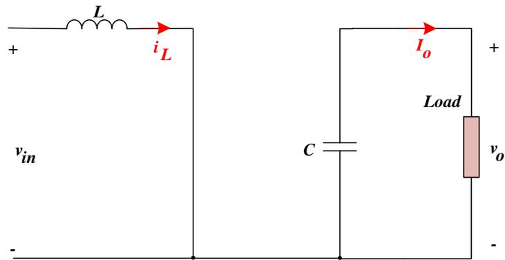
Figure 2.3. Conventional Boost Converter Operational Mode-1 Representation
