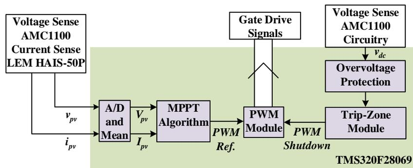
Figure 3.16. Main Control Block
