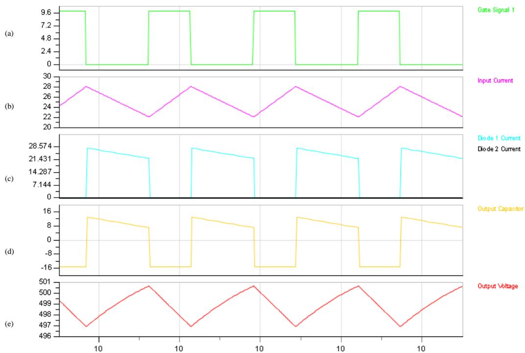
Figure 2.5. Conventional Boost Converter Critical Operational Waveforms Obtained with Power Electronics Simulator (24 us time division) Y-Axis: (a) 20 kHz Gate Signal (V), (b) Inductor Current (A), (d) Output Capacitor Current (A), (e) Output Voltage (V)
