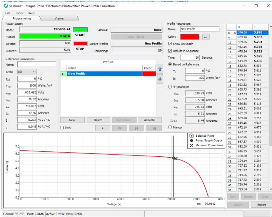
Figure 4.11. TPISBC Power Stage 325 W/m<sup>2</sup> operation at MPP
