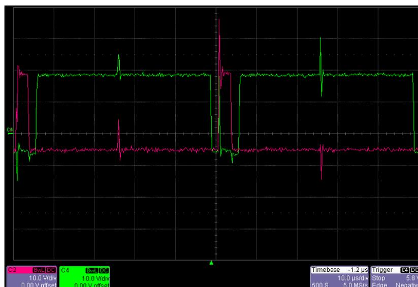
Figure 4.15. TPISBC Power Stage: One-Cycle High-Side and Low-Side MOSFET V<sub>GS</sub> waveforms
