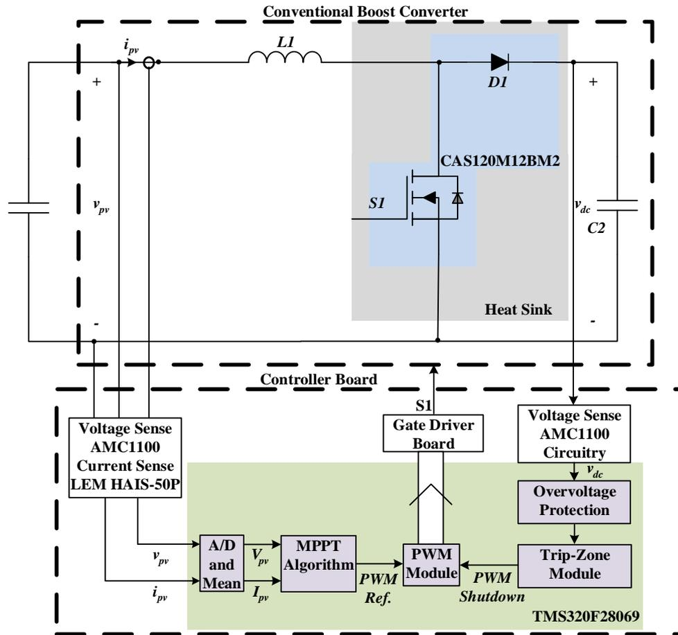
Figure 3.4. Conventional Boost Converter Power and Control Stages
