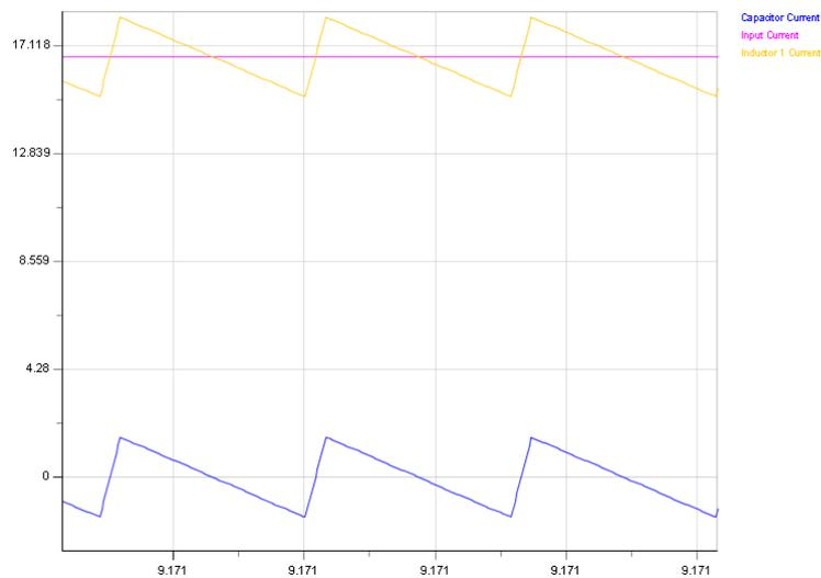
Figure 3.9. Conventional Boost Converter Input Current Waveforms Obtained with Power Electronics Simulator Y-Axis: (Pink) Input Current (A), (Blue) Capacitor Current (A), (Yellow) Inductor 1 Current (A)
