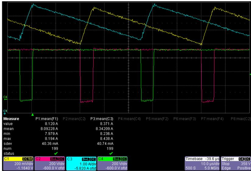
Figure 4.17. TPISBC Power Stage Operational Waveforms: C1- Inductor-1 (L1) Current Waveform (5A/V), C3 – Inductor-2 (L2) Current Waveform, C2 – S1  $V_{DS}$  waveform, C4 – S3  $V_{DS}$  waveform
