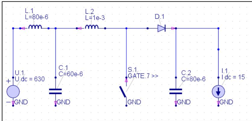
Figure 3.8. Simulation Circuit with Wire Inductance
