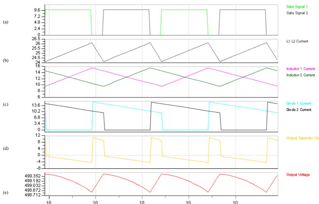
Figure 2.10. Two-Phase Interleaved Boost Converter Critical Operational Waveforms Obtained with Power Electronics Simulator (20  $\mu$ s time division) Y-Axis: (a) 20 kHz Gate Signals (V), (b) Input Current (A), (c) Inductor Currents (A), (d) Output Capacitor Current (A), (e) Output Voltage (V)
