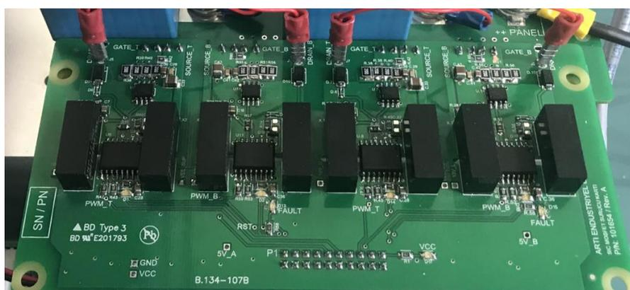
*Figure 3.13. Gate Driver Board Top-Side*
