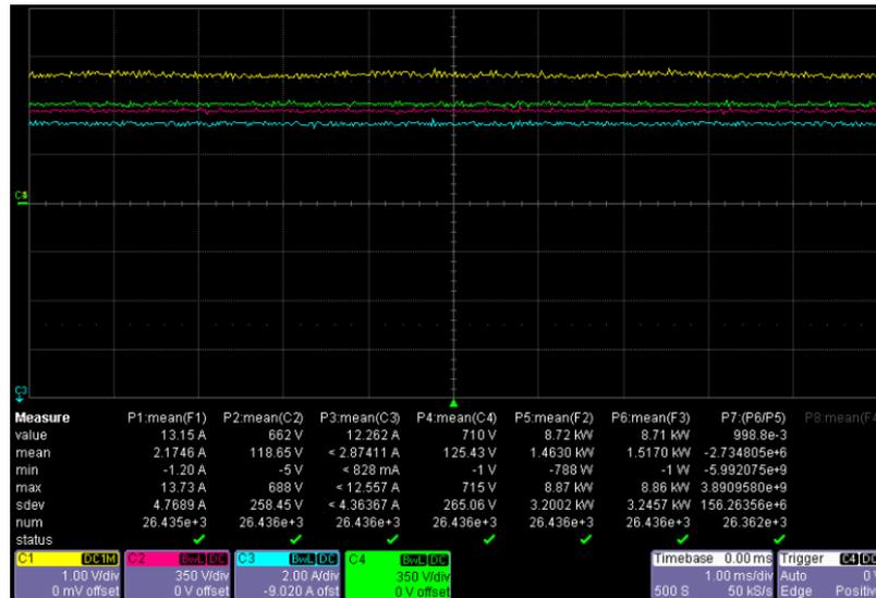
Figure 4.8. TPISBC Power Stage 825 W/m<sup>2</sup> operation at MPP: C1- Input Current (5A/V), C2-Input Voltage, C3-Output Current, C4-Output Voltage, P1 to P4-mean of channels C1 to C4, P5-Input Power, P6-Output Power, P7-Efficiency
