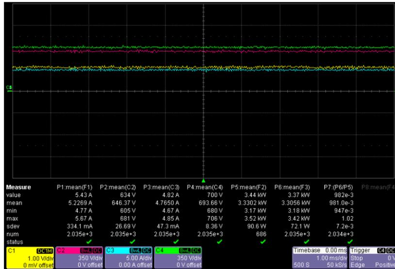
Figure 4.12. TPISBC Power Stage 325 W/m<sup>2</sup> operation at MPP: C1- Input Current (5A/V), C2-Input Voltage, C3-Output Current, C4-Output Voltage, P1 to P4-mean of channels C1 to C4, P5-Input Power, P6-Output Power, P7-Efficiency
