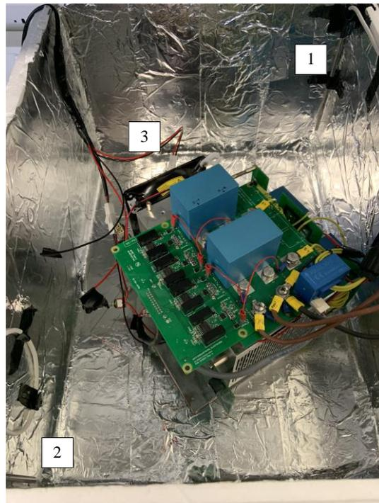
*Figure 4.21.* Calorimeter Setup 1: PT-100 Sensor 1, 2: PT-100 Sensor 2, 3: Heat Sink Fan
