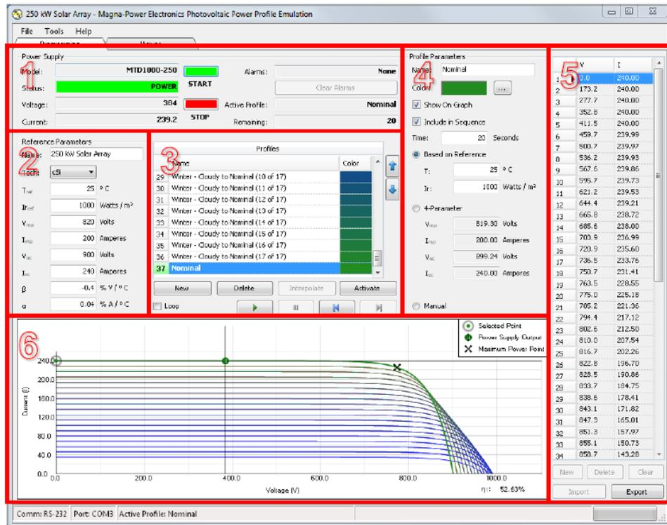
Figure 4.2. Main Window of Photovoltaic Power Profile Emulation Tool Software for Magna-Power TSD800-24 High Power DC Power Supply
