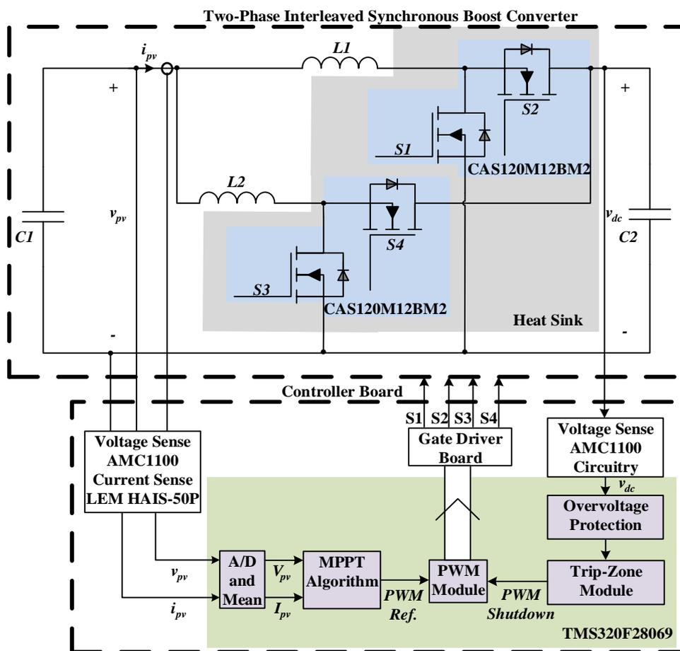
Figure 3.1. Two-Phase Interleaved Synchronous Boost Converter Power and Control Stages
