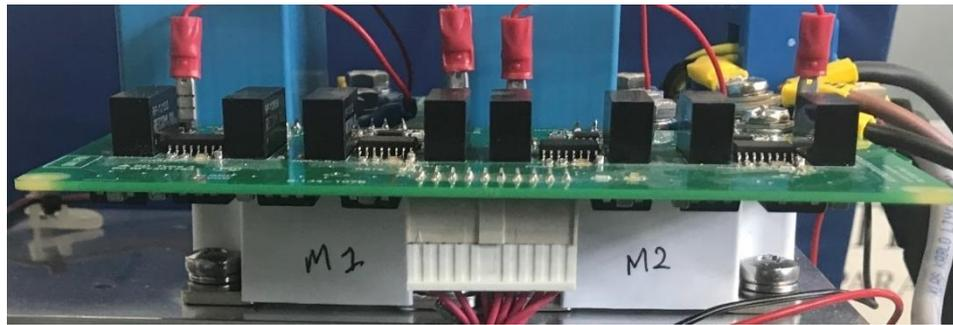
*Figure 3.14. Gate Driver Board as Plugged-In to the MOSFETs*
