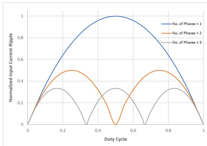
Figure 2.11. Normalized Input Current Ripple vs. Duty Cycle for Different Number of Phases
