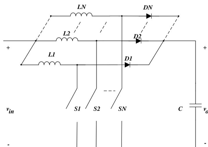
Figure 2.6. “N” Phase Boost Converter Diagram
