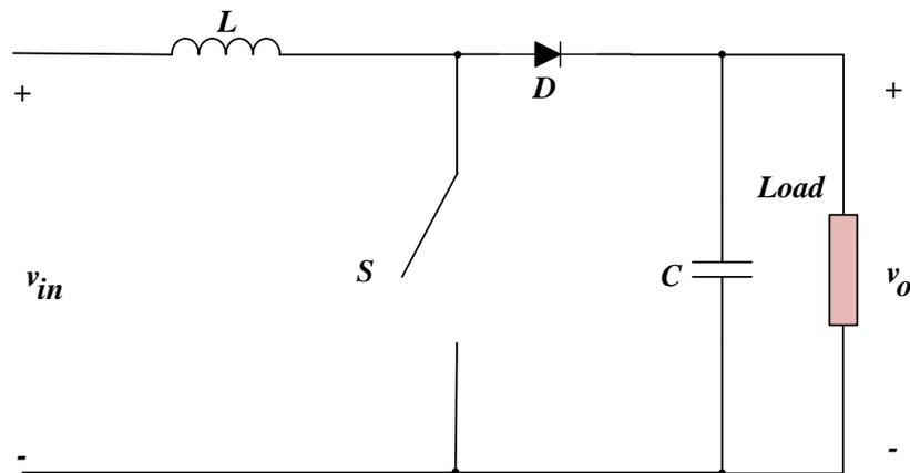
Figure 2.1. Conventional Boost Converter Diagram
