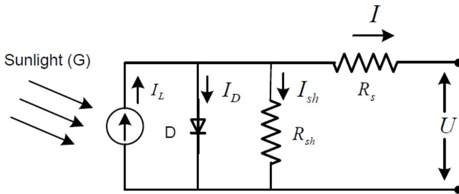
Figure 1 PV Cell Model
