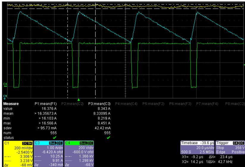
Figure 4.18. TPISBC Power Stage Operational Waveforms: C1- Input Current Waveform (5A/V), C3 – Inductor-1 (L1) Current Waveform, C4 – S1  $V_{DS}$  waveform
