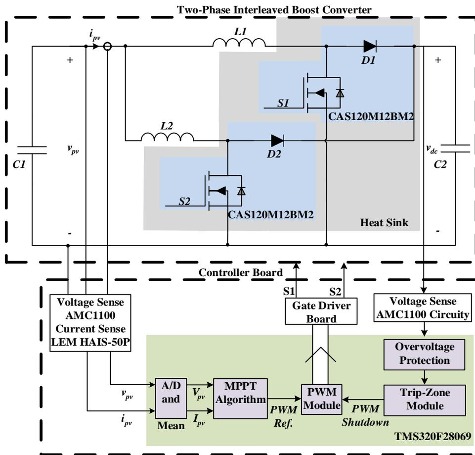
Figure 3.2. Two-Phase Interleaved Boost Converter Power and Control Stages
