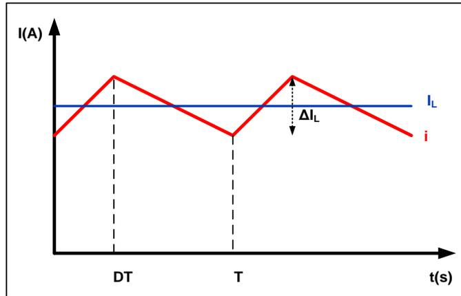
Figure 3.10. Boost Converter Inductor Current Waveform for CCM Operation
