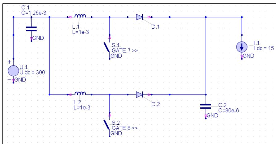
Figure 2.8. Simulated Two-Phase Interleaved Boost Converter Circuit Diagram, Input Voltage Source: 300 V, Output Current: 15A, C1: 1.26 mF, L1: 1mH, L2: 1mH, C2: 80 uF
