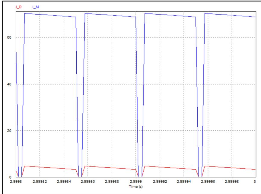
*Figure 3.25* Current Through Synchronous Boost Converter Upper MOSFET and Body Diode Obtained with Power Electronics Simulator: MOSFET Current in Blue (A), Diode Current in Red (A)
