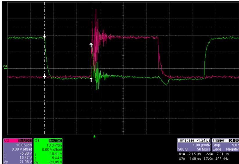
Figure 4.16. TPISBC Power Stage: Zoomed-In High-Side and Low-Side MOSFET  $V_{GS}$  waveforms with dead-band: C2 - Low-Side MOSFET  $V_{GS}$ , C4 - High-Side MOSFET  $V_{GS}$
