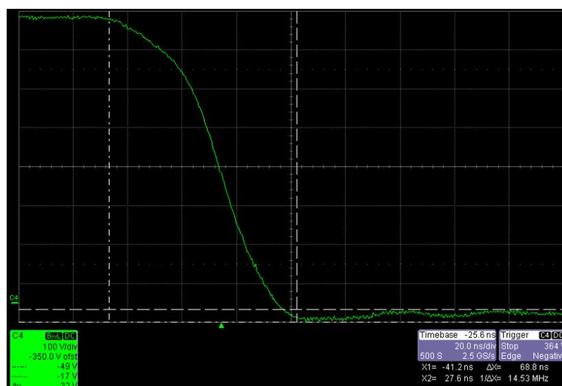
Figure 4.13. TPISBC Power Stage: Zoomed-in MOSFET VDS waveform during turn-on instant
