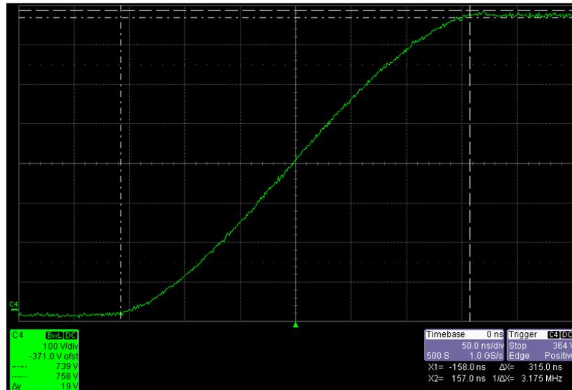
Figure 4.14. TPISBC Power Stage: Zoomed-in MOSFET V<sub>DS</sub> waveform during turn-off instant
