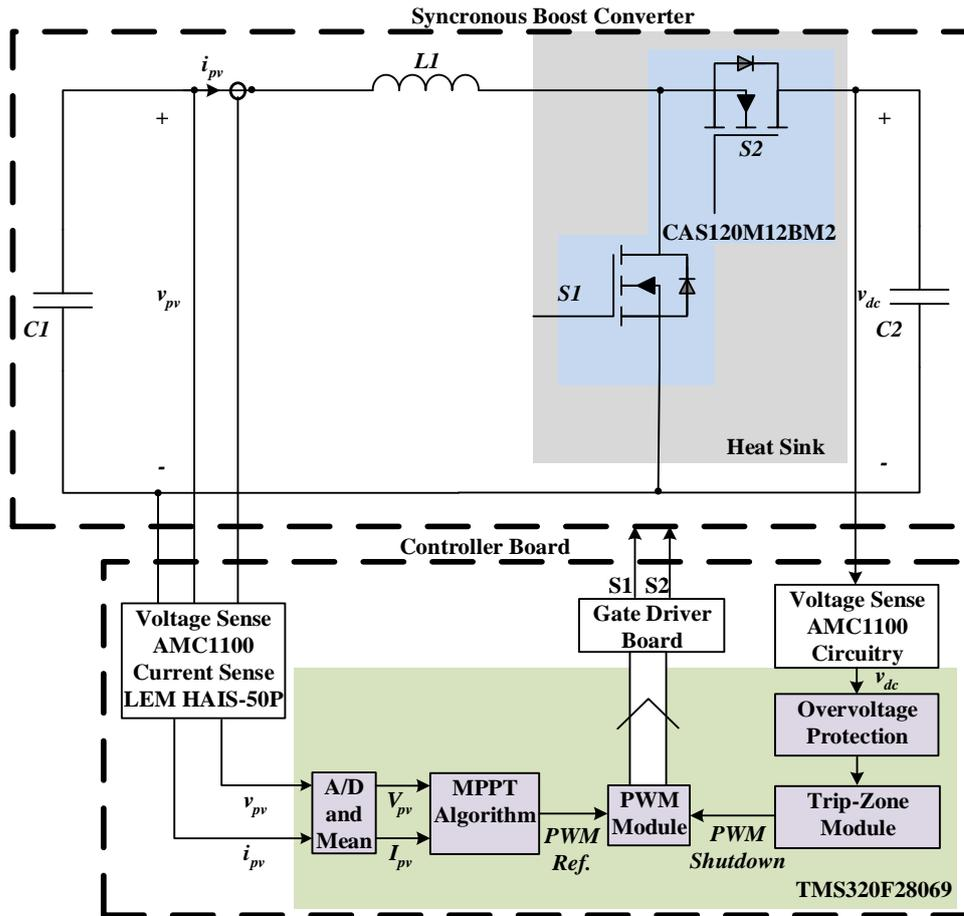
Figure 3.3. Synchronous Boost Converter Power and Control Stages
