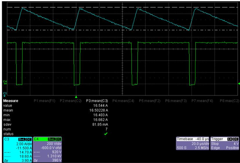
Figure 4.19. SBC Power Stage Operational Waveforms: C1- Input (Inductor) Current Waveform (5A/V), C4 – S1 V<sub>DS</sub> waveform
