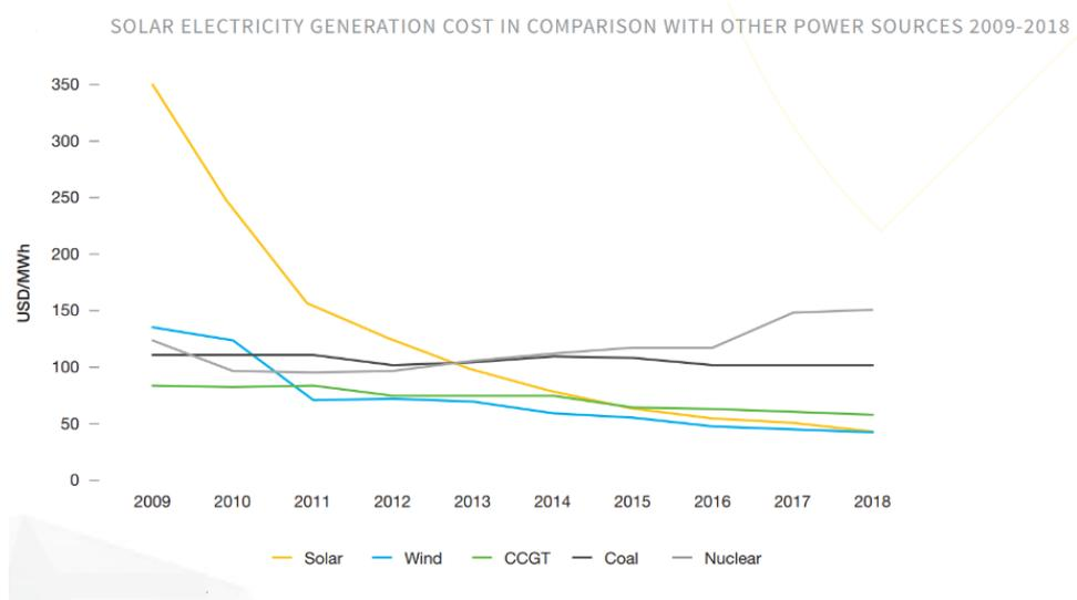
Figure 1.1. Electricity Generation Cost of Different Sources[1]
