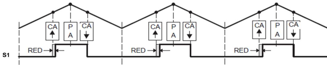
Figure 3.20. Conventional Boost Converter PWM Signal Generation Example
