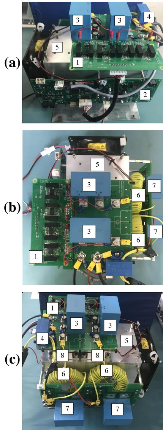
Figure 3.5. (a) Side-1 View (b) Top View (c) Side-2 View of the Boost Converter
