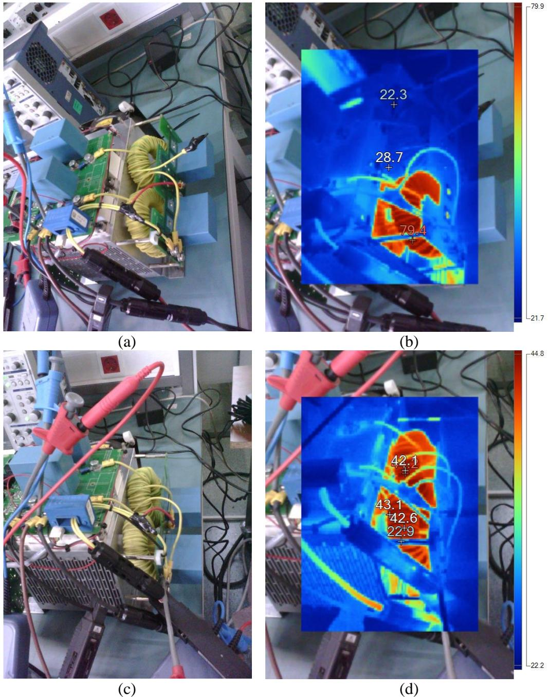
Figure 4.20. (a) Visible Light Image of SBC, (b) Infrared Image of SBC, (c) Visible Light Image of TPISBC, (d) Infrared Image of TPISBC
