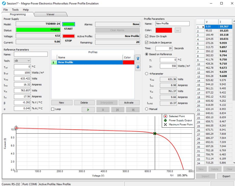
Figure 4.9. TPISBC Power Stage 550 W/m<sup>2</sup> operation at MPP
