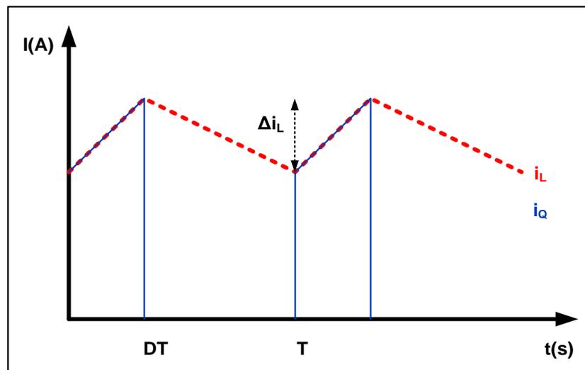
*Figure 3.12.* Boost Converter Switch Current Waveform
