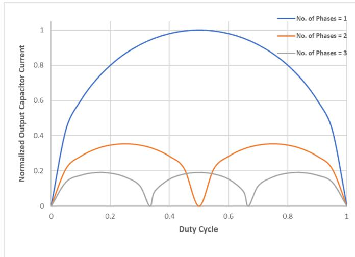
Figure 2.12. Normalized Output Capacitor Current Ripple vs. Duty Cycle for Different Number of Phases
