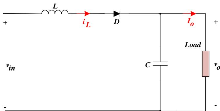
Figure 2.4. Conventional Boost Converter Operational Mode-2 Representation
