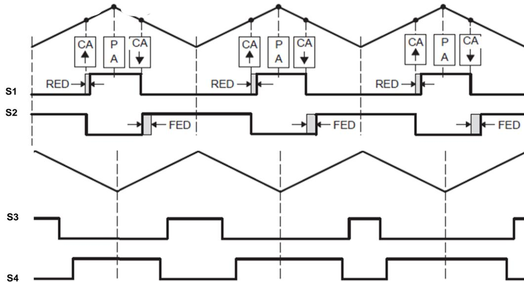
Figure 3.17. Two-Phase Interleaved Synchronous Boost Converter PWM Signal Generation Example
