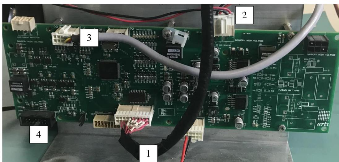
Figure 3.15. View of Control Board with the Necessary Connections
