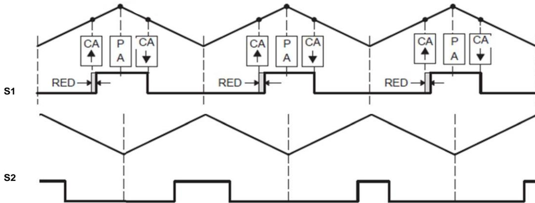
Figure 3.18. Two-Phase Interleaved Boost Converter PWM Signal Generation Example
