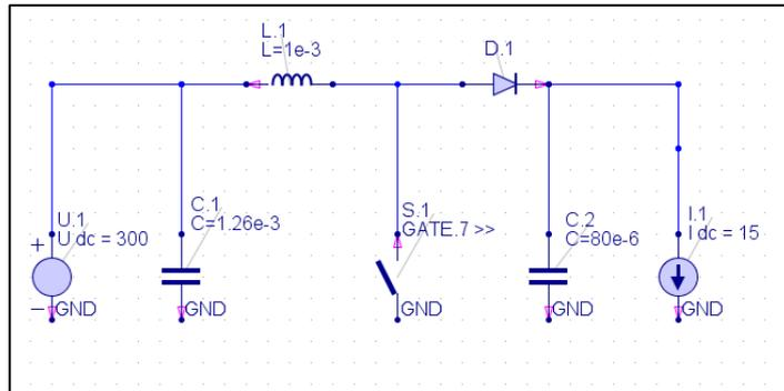
Figure 2.2. Simulated Boost Converter Circuit Diagram, Input Voltage Source: 300 V, Output Current: 15 A, C1: 1.26 mF, L1: 1 mH, C2: 80 uF
