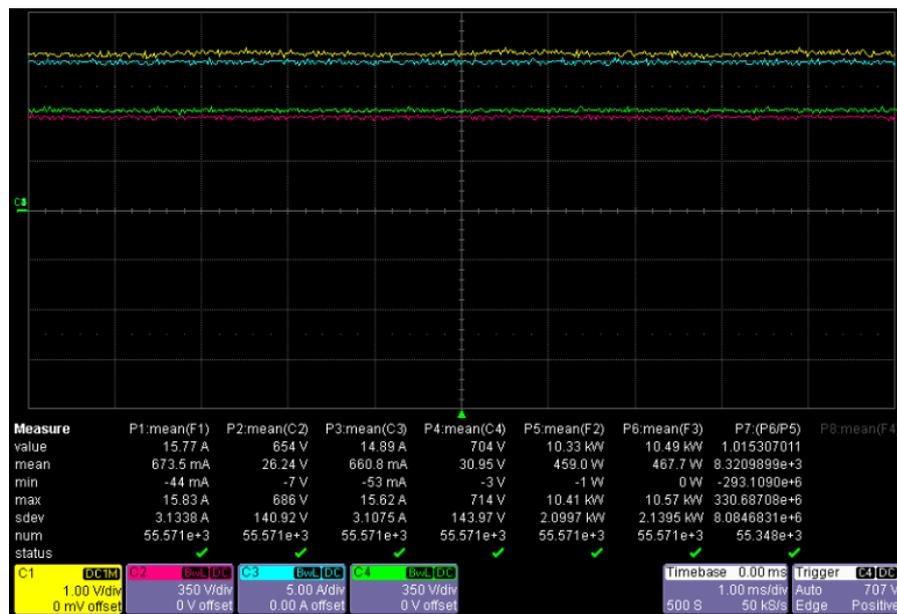
Figure 4.6. TPISBC Power Stage 1000 W/m<sup>2</sup> operation at MPP: C1- Input Current (5A/V), C2-Input Voltage, C3-Output Current, C4-Output Voltage, P1 to P4-mean of channels C1 to C4, P5-Input Power, P6-Output Power, P7-Efficiency
