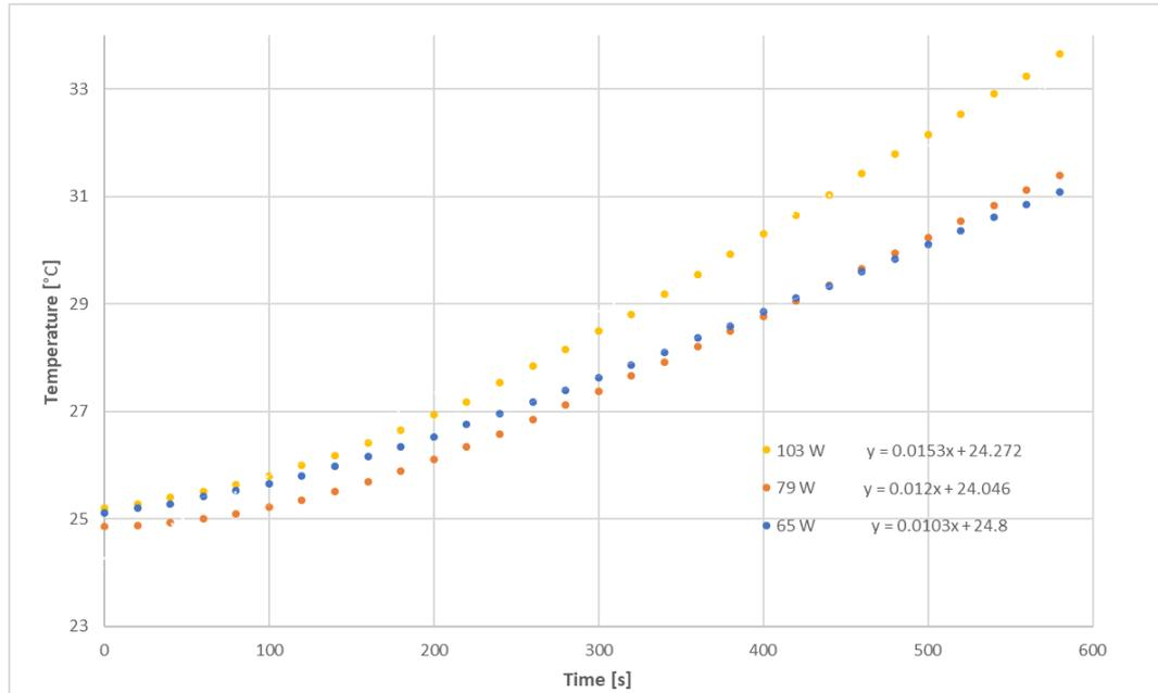
Figure 4.24. Temperature Profiles for Known Powers
