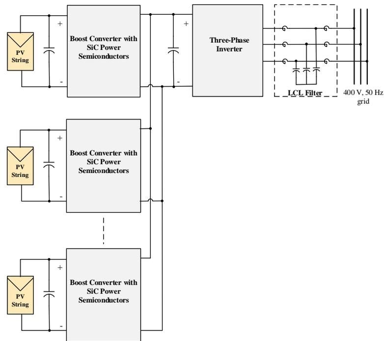
Figure 1.3. Photovoltaic System Integration with All-SiC MPPT Boost Converter
