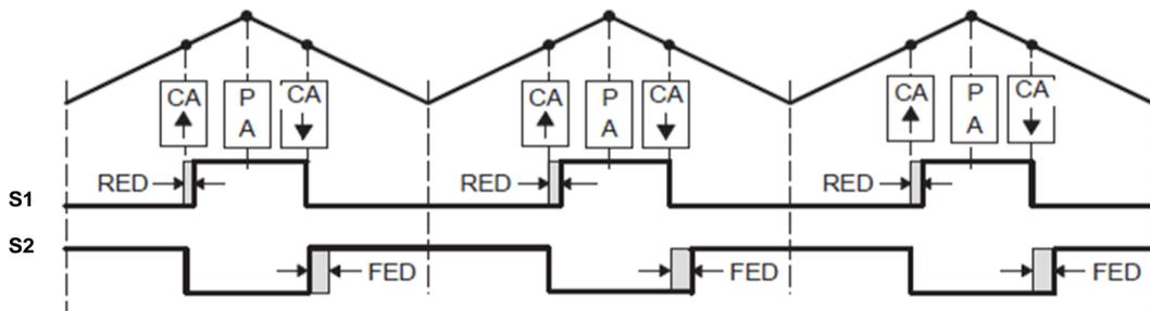
Figure 3.19. Synchronous Boost Converter PWM Signal Generation Example
