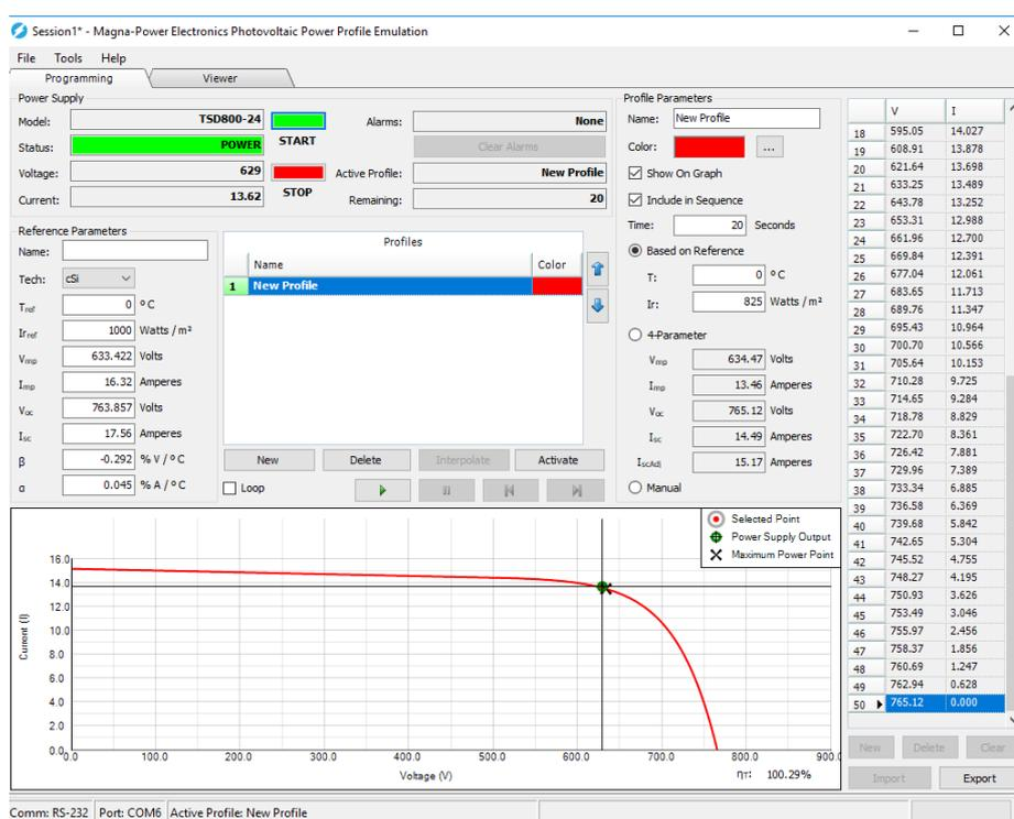
Figure 4.7. TPISBC Power Stage 825 W/m<sup>2</sup> operation at MPP
