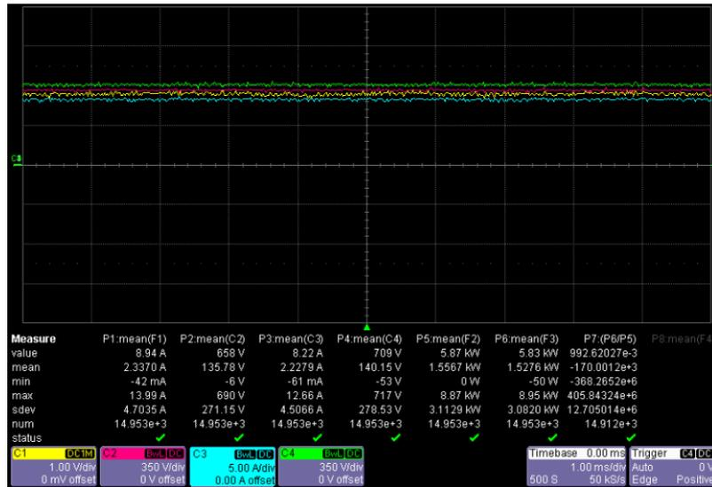
Figure 4.10. TPISBC Power Stage 550 W/m<sup>2</sup> operation at MPP: C1- Input Current (5A/V), C2-Input Voltage, C3-Output Current, C4-Output Voltage, P1 to P4-mean of channels C1 to C4, P5-Input Power, P6-Output Power, P7-Efficiency
