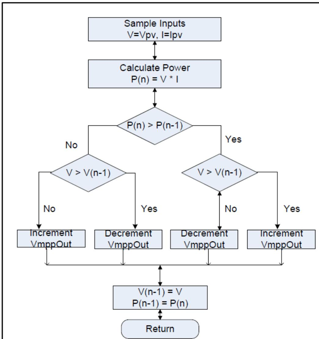
Figure 3.21. Perturb and Observe Algorithm [8]
