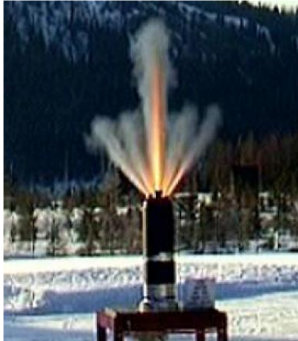
Figure 1.25. P80 pyrogen igniter static firing [12]
