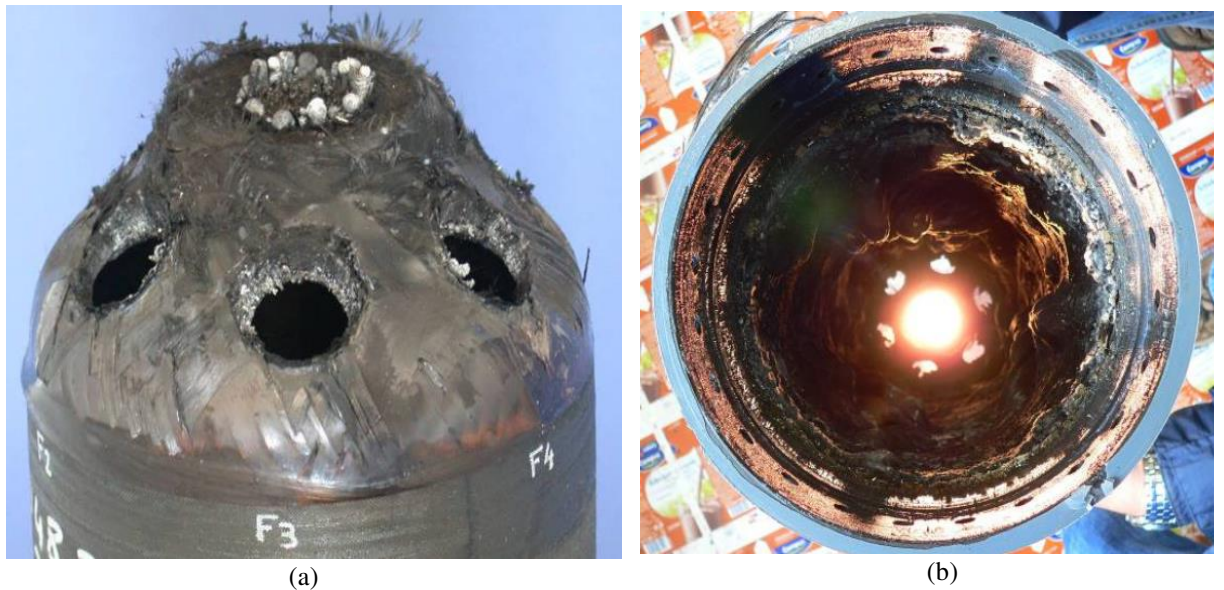
Figure 1.26. Z9 Igniter cases and nozzles after static Firing of Z9 (a) and Z23 (b) [12]
