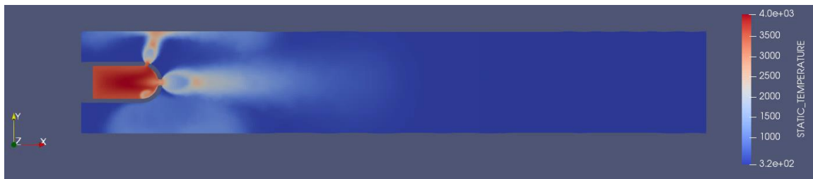
Figure 4.24. Temperature behavior of the test Case # 4 having 75° of radial nozzle angel, at the 10 th ms
