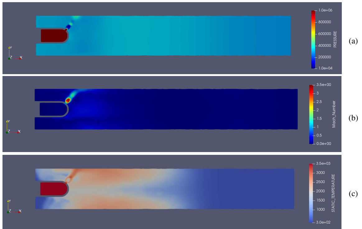
Figure 4.37. Pressure (a), Mach number (b) and static temperature (c) distributions of the test case ejecting only radial mass flow
