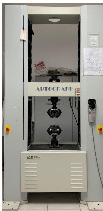
*Figure 10.* Shimadzu Autograph AG-IS 100kN universal testing machine.
