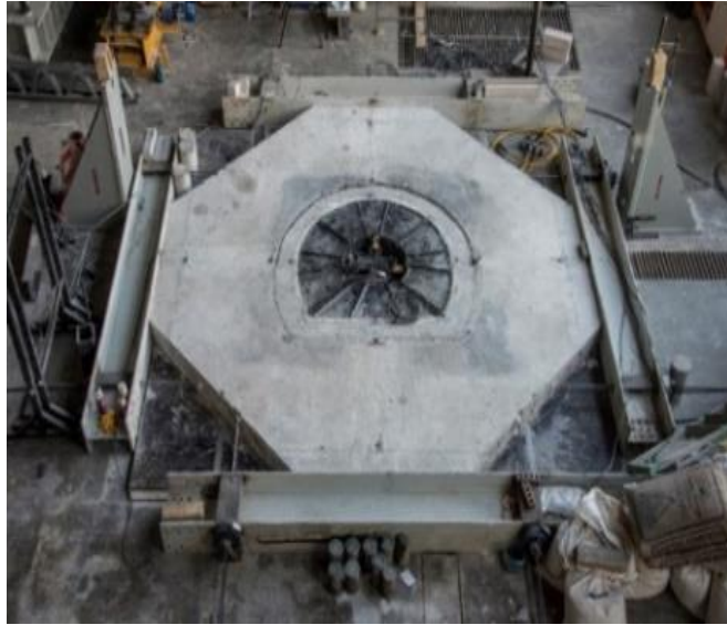
Figure 39. The setup of fourth experiment with partial in-situ confining stresses
