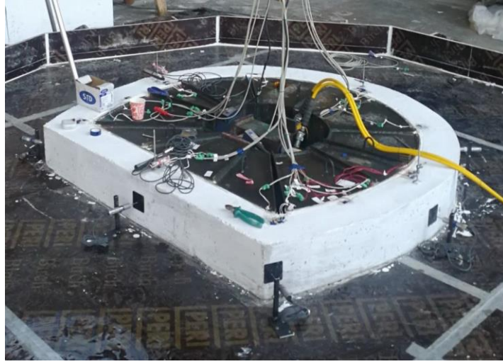
Figure 22. The setup of the first experiment with no rock confinement
