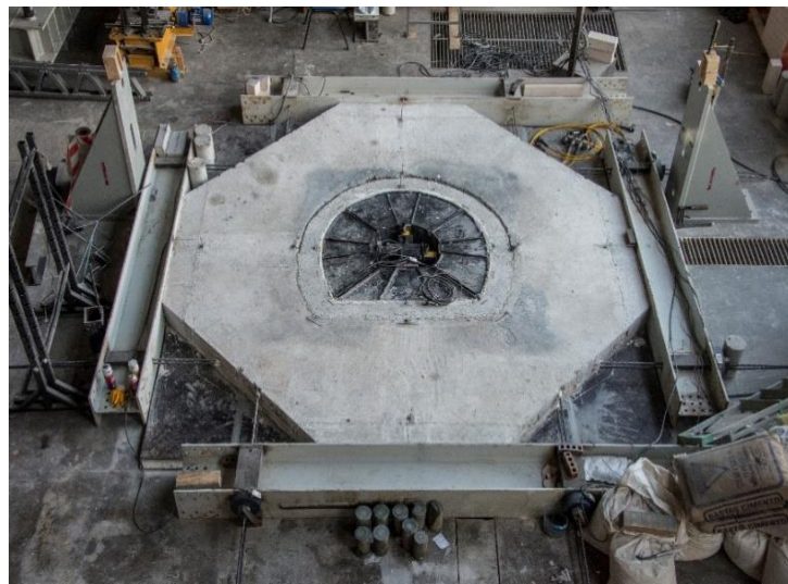
Figure 47. The setup of sixth experiment with partial in-situ confining stresses
