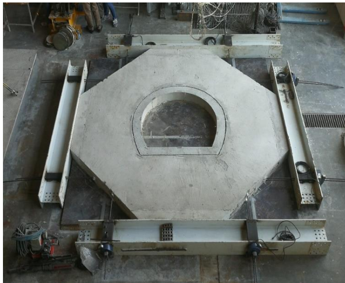
Figure 32. The setup of the third experiment with full rock confinement
